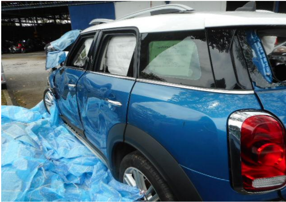
Photo 13 shows a general view of the Motor Car's left body at the time of my inspection. The Motor car was observed to have sustained damage at its right portion. Its left doors (circled) was amongst the body parts damaged as a result of the accident.
