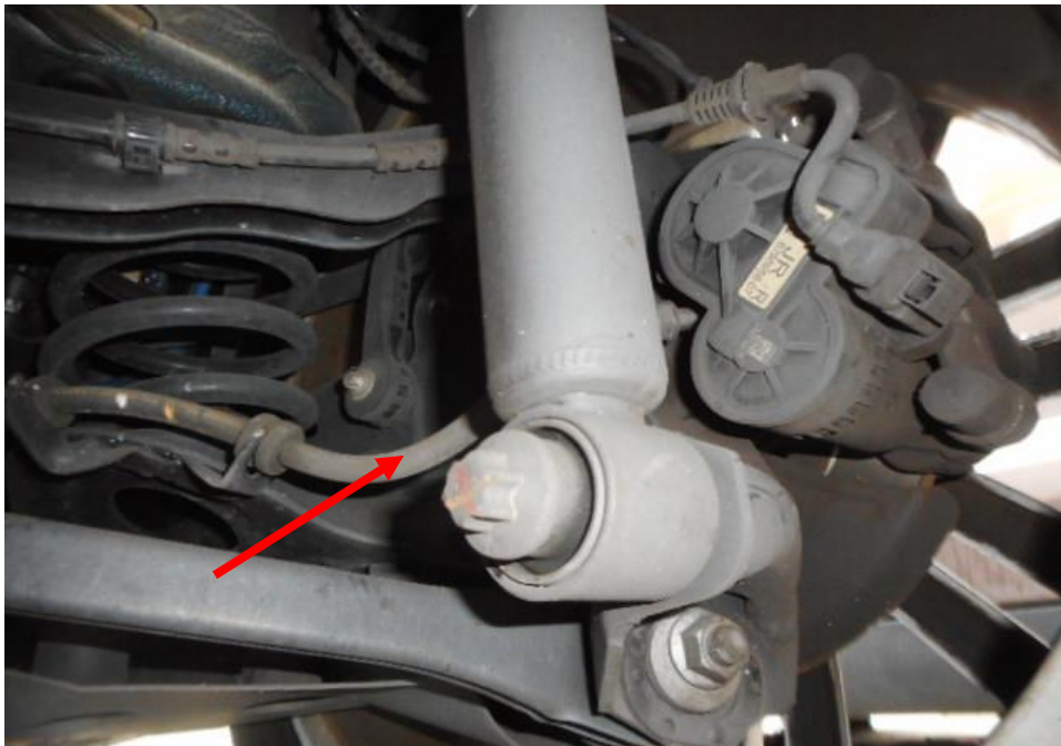
Photo 28 shows the brake hose/pipe (arrowed) at the rear right wheel of the Motor Car. No leakage of brake fluid was observed. Visual examination of the various components of the braking system like the brake caplier to be intact and without visible damage.
