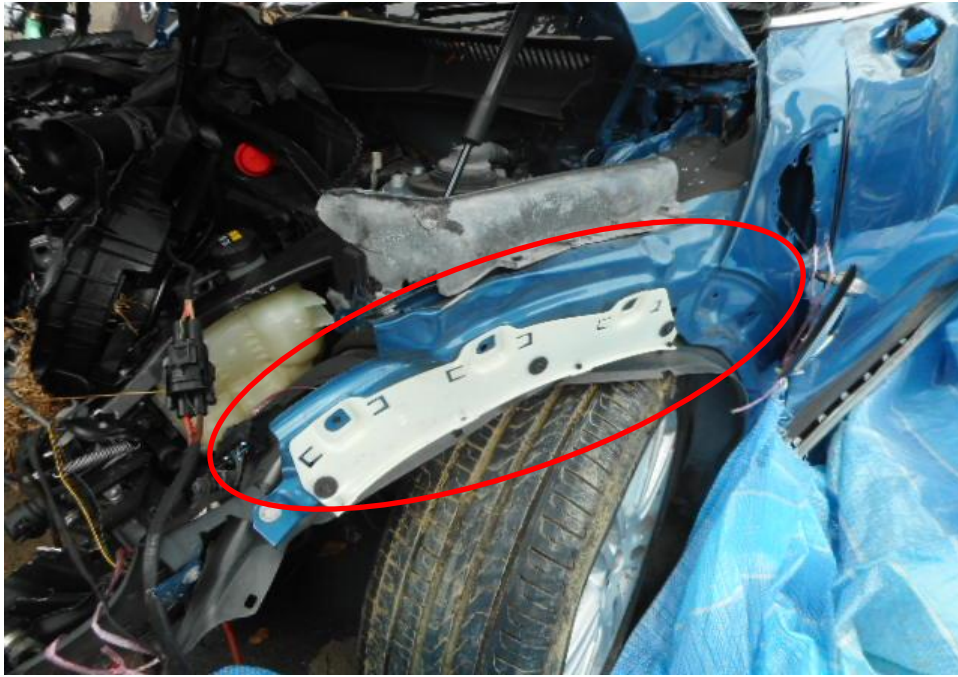
Photo 9 shows the close up view of the Motor Car's front body at the time of my inspection. The Motor car was observed to have sustained damage at its front portion. Its front left fender (circled) was amongst the body part damaged as a result of the accident.
