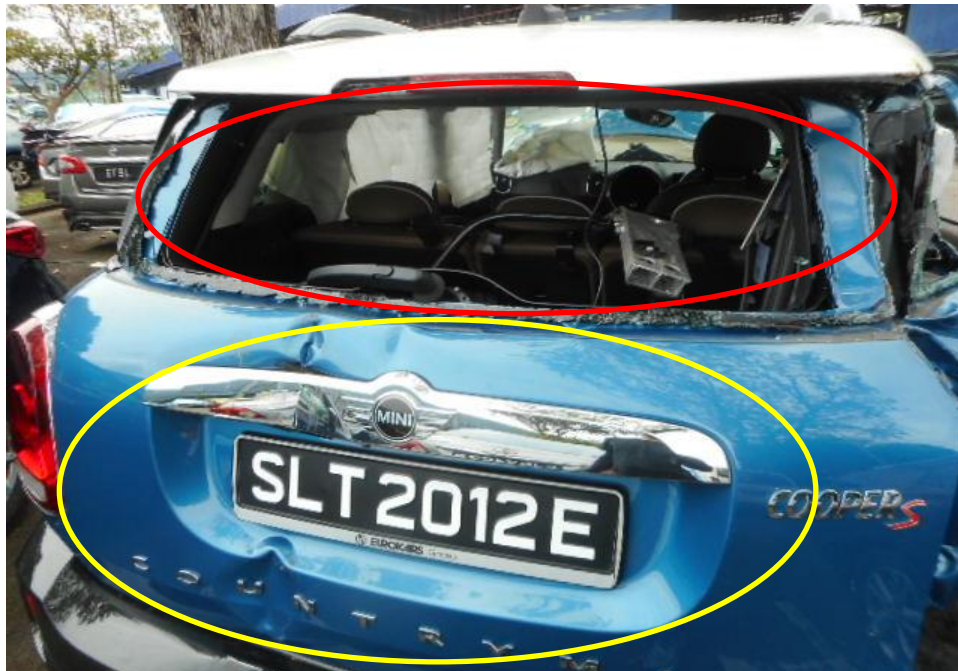
Photo 2 shows a close up view of the Motor Car's rear body at the time of my inspection. The rear portion of the Motor Car was observed to sustain damages as a result of the accident. Its rear windscreen (red circle) and rear boot (yellow arrow) were damaged as a result of the accident.
