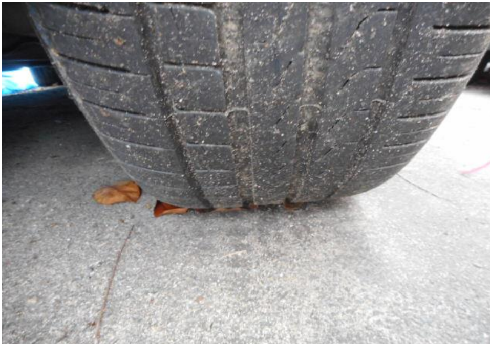
Photo 16 shows the condition of the rear right tyre of the Motor Car, which was observed to be in serviceable condition with remaining tread depth of approximately 4.3mm. The tyre was also observed to be sufficiently inflated for vehicular operation with no tear, cut or burst mark(s).
