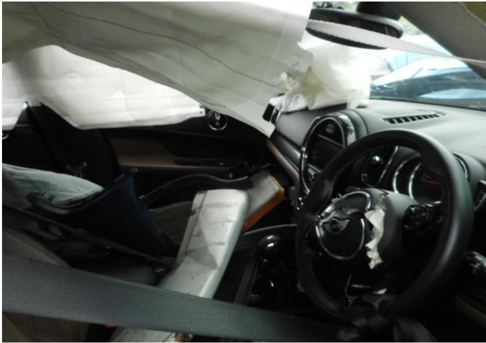
Photo 19 shows the deployment of the Supplemental Restraint System (SRS) airbag in the Motor Car as a result of the accident.
