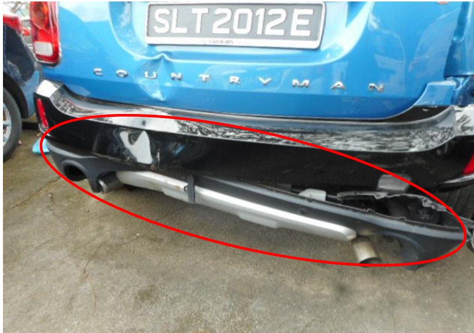
Photo 3 shows a close up view of the Motor Car's rear body at the time of my inspection. The rear portion of the Motor Car was observed to sustain damages as a result of the accident. Its rear bumper (circled) were damaged as a result of the accident.
