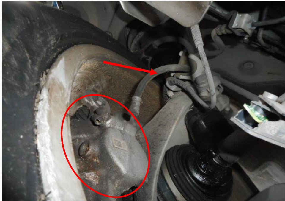
Photo 29 shows the brake hose/pipe (arrowed) at the front right wheel of the Motor Car. I did not observe any leakage of brake fluid at the time of my inspection of the Motor Car. Visual examination of the various components of the braking system the brake caliper (circled) to be intact and without visible damage.
