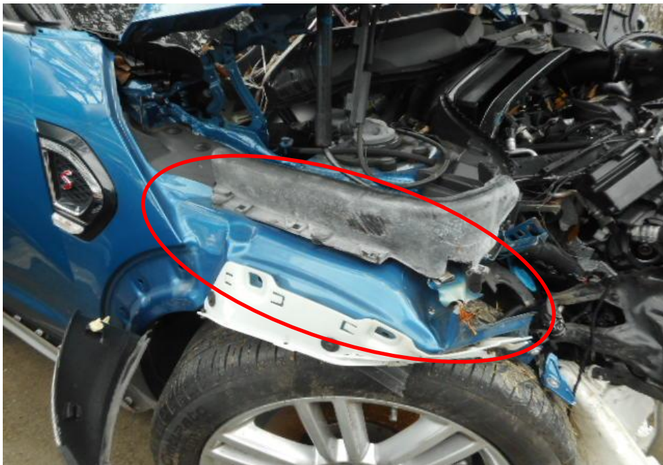
Photo 8 shows the close up view of the Motor Car's front body at the time of my inspection. The Motor car was observed to have sustained damage at its front portion. Its front right fender (circled) was amongst the body part damaged as a result of the accident.
