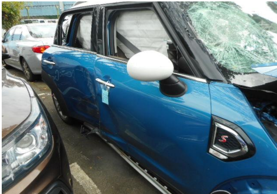
Photo 10 shows a general view of the Motor Car's right body at the time of my inspection. The Motor car was observed to have sustained damage at its right portion. Its right doors (circled) was amongst the body parts damaged as a result of the accident.
