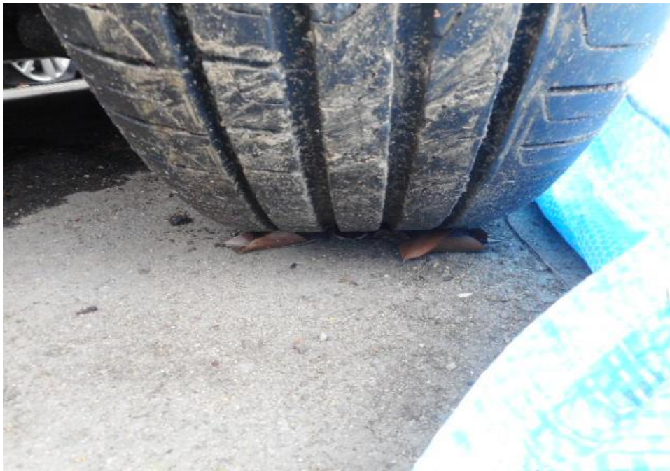
Photo 18 shows the condition of the front left tyre of the Motor Car, which was observed to be in serviceable condition with remaining tread depth of approximately 5.5mm. The tyre was also observed to be sufficiently inflated for vehicular operation with no tear, cut or burst mark(s).
