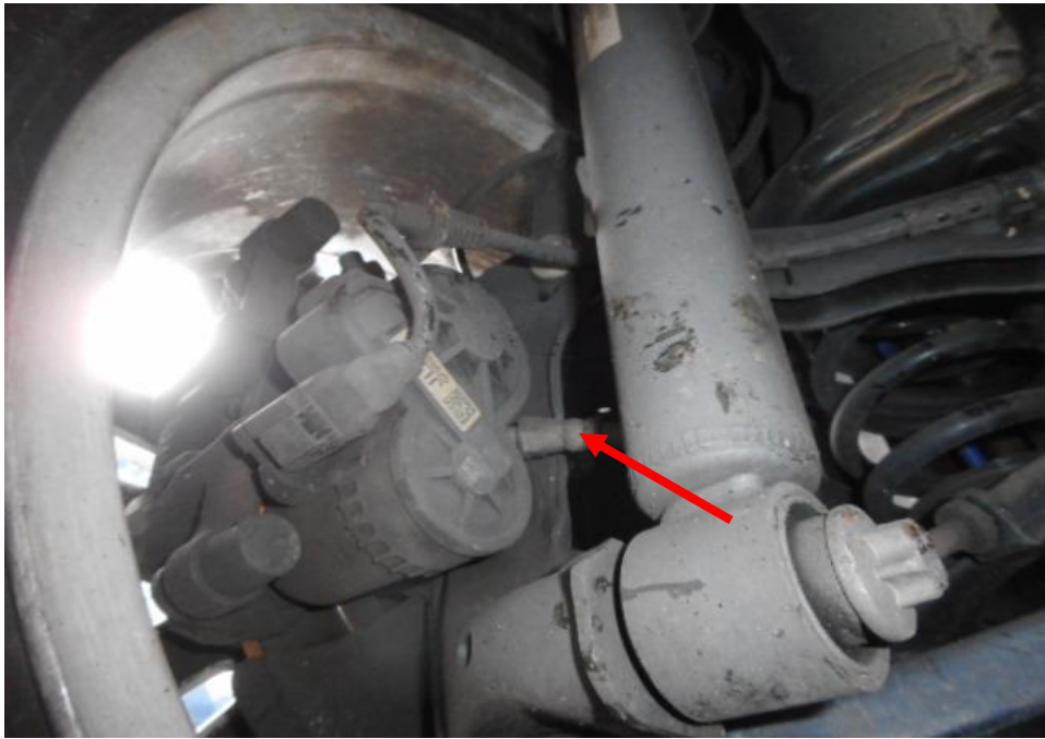
Photo 27 shows the brake hose/pipe (arrowed) at the rear left wheel of the Motor Car. No leakage of brake fluid was observed. Visual examination of the various components of the braking system like the brake caplier to be intact and without visible damage.
