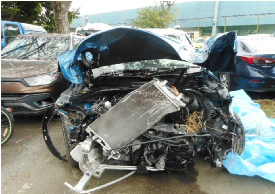
Photo 5 shows a general view of the Motor Car's front body at the time of my inspection. The Motor car was observed to have sustained damage at its front portion. Its front windscreen, front bonnet, front left and right fender, was amongst the body parts that were damaged as a result of the accident. The Supplemental Restraint System (SRS) was activated as a result of the accident.
