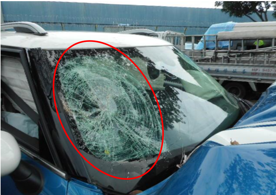
Photo 6 shows the close up view of the Motor Car's front body and roof panel at the time of my inspection. The Motor car was observed to have sustained damage at its front portion. Its front windscreen (circled) was damaged as a result of the accident.
