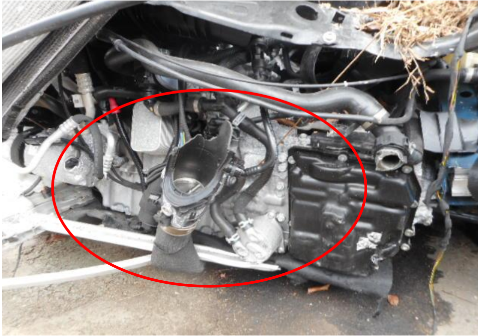
Photo 22 shows the close up view of the Motor Car's front body at the time of my inspection. The Motor car was observed to have sustained damage at its front portion. Its engine components (circled) was amongst the various components in the engine compartments were also damaged as a result of the accident.
