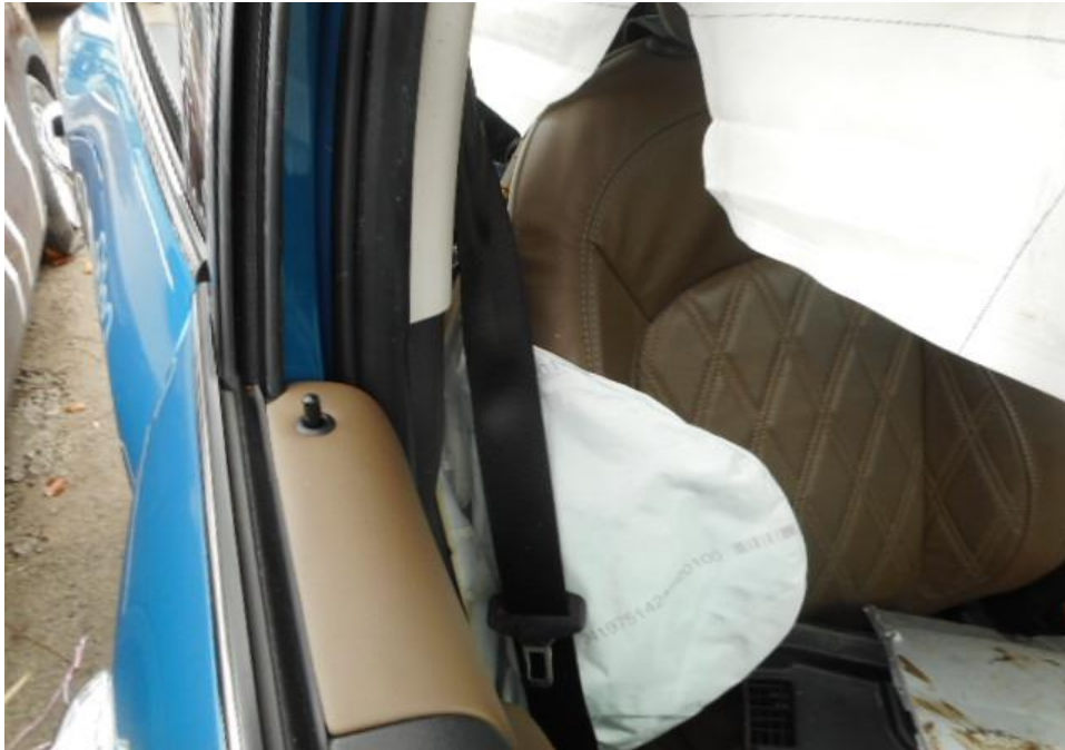
Photo 34 shows that the seat belt on the right seat was worn at the material time of accident as the safety pre-tensioners was activated at the moment of impact and caused the seat belt to be locked into the last position.
