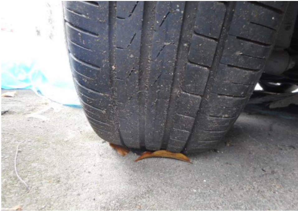
Photo 17 shows the condition of the rear left tyre of the Motor Car, which was observed to be in serviceable condition with remaining tread depth of approximately 4.4mm. The tyre was also observed to be sufficiently inflated for vehicular operation with no tear, cut or burst mark(s).
