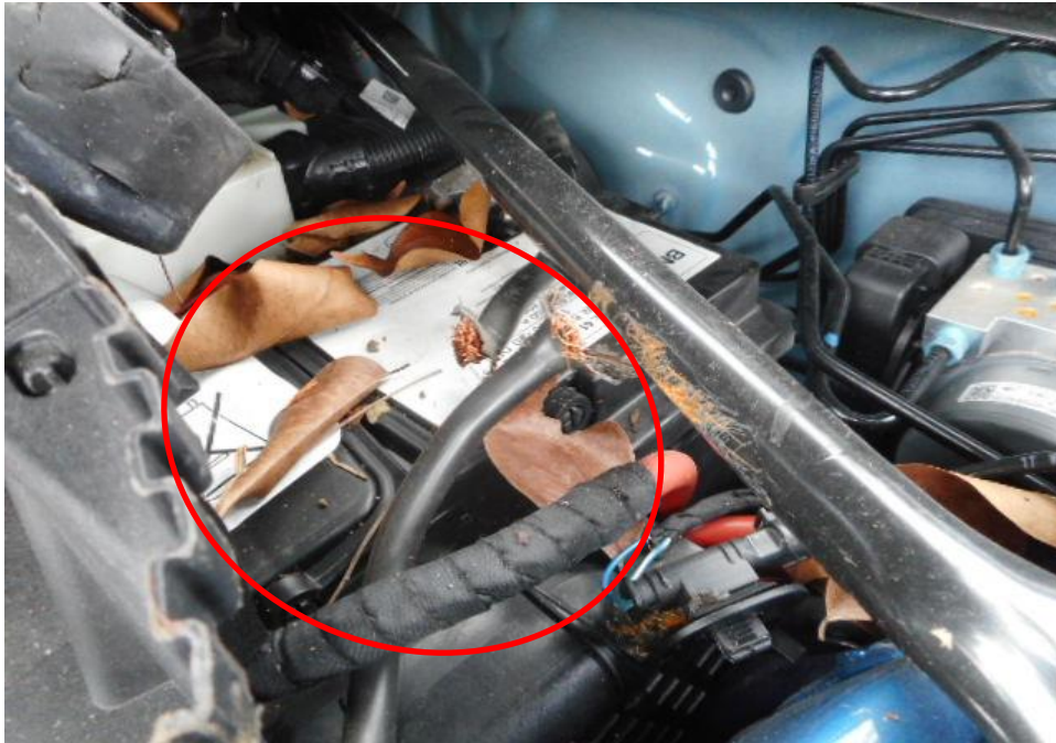
Photo 24 shows the close up view of the Motor Car's front body at the time of my inspection. The Motor car was observed to have sustained damage at its front portion. Its ignition system battery (circled) was amongst the various components in the engine compartments were also damaged as a result of the accident.
