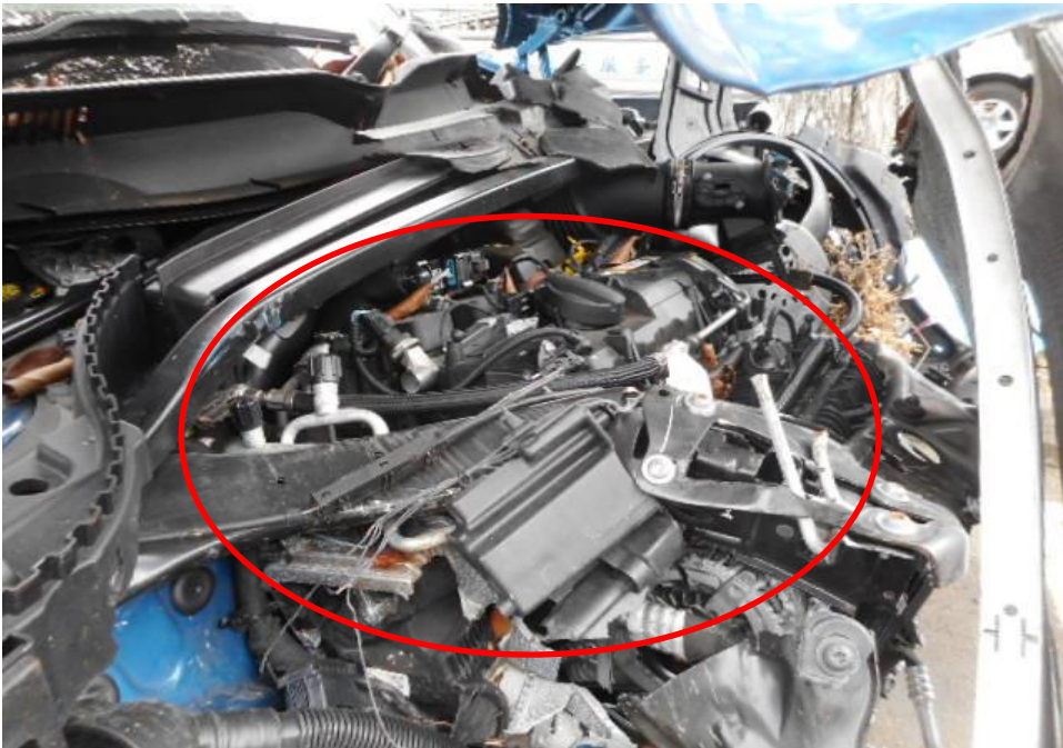
Photo 21 shows the close up view of the Motor Car's front body at the time of my inspection. The Motor car was observed to have sustained damage at its front portion. Its engine components (circled) was amongst the various components in the engine compartments were also damaged as a result of the accident.
