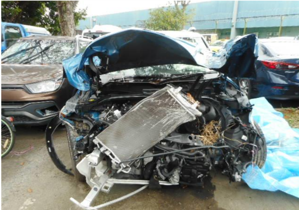
Photo 20 shows a general view of the Motor Car's engine compartment. The various parts and components inside the engine compartment were observed that the engine and ignition system was damaged as a result of the induced impact from the accident.
