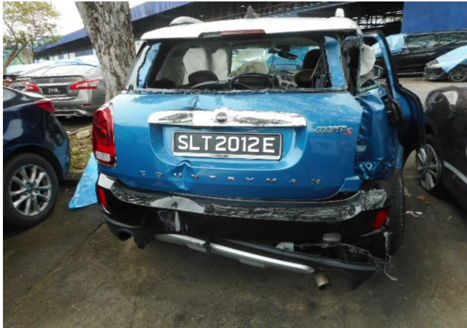
Photo 1 shows a general view of the Motor Car's rear body at the time of my inspection. The rear portion of the Motor Car was observed to sustain damages as a result of the accident. Its rear windscreen, rear boot, rear bumper and right rear brake lamp were damaged as a result of the accident.
