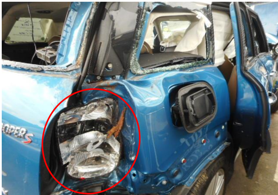
Photo 4 shows a close up view of the Motor Car's rear body at the time of my inspection. The rear portion of the Motor Car was observed to sustain damages as a result of the accident. Its rear right brake lamp (circled) were damaged as a result of the accident.
