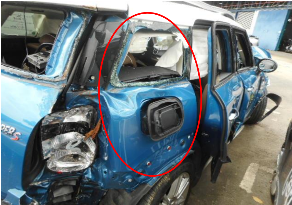
Photo 12 shows a close up view of the Motor Car's right body at the time of my inspection. The Motor car was observed to have sustained damage at its right portion. Its right door panel (circled) was amongst the body parts damaged as a result of the accident.
