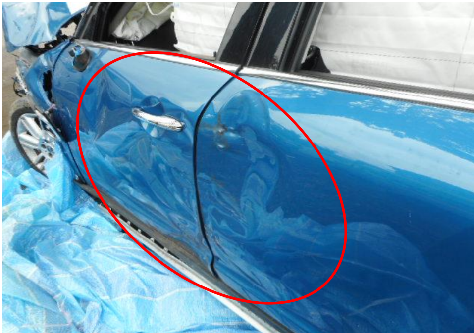
Photo 14 shows a close up view of the Motor Car's left body at the time of my inspection. The Motor car was observed to have sustained damage at its right portion. Its left doors (circled) was amongst the body parts damaged as a result of the accident.
