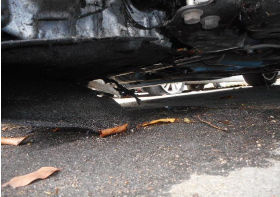
Photo 26 shows the undercarriage of the Motor Car, at the area where the engine housing and transmission housing are located. I found engine oil leakage on the underside of the Motor Car as a result of the accident.
