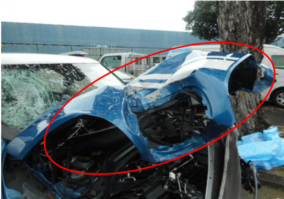
Photo 7 shows the close up view of the Motor Car's front body at the time of my inspection. The Motor car was observed to have sustained damage at its front portion. Its front bonnet (circled) was damaged as a result of the accident.
