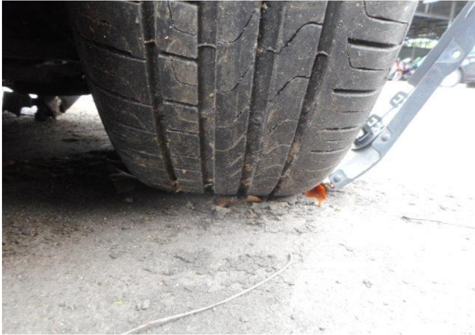
Photo 15 shows the condition of the front right tyre of the Motor Car, which was observed to be in serviceable condition with remaining tread depth of approximately 6.1mm. The tyre, which was wrapped around alloy wheel rim, was also observed to be sufficiently inflated for vehicular operation.
