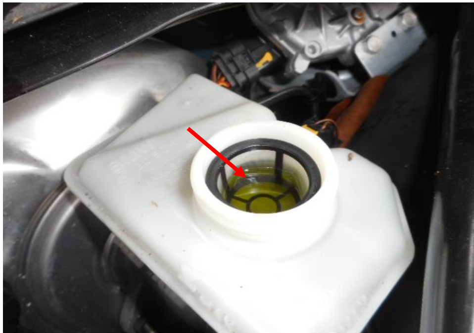
Photo 25 shows the brake fluid reservoir of the Motor Car at the time of my inspection. The brake fluid was observed to be of sufficient level (arrowed) and without any visible contamination.
