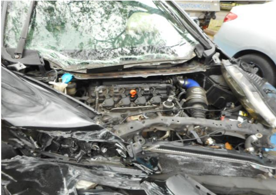
Photo 14 shows a general view of the Motor Car's engine compartment. The various parts and components inside the engine compartment were observed that the engine and ignition system was damaged as a result of the induced impact from the accident.
