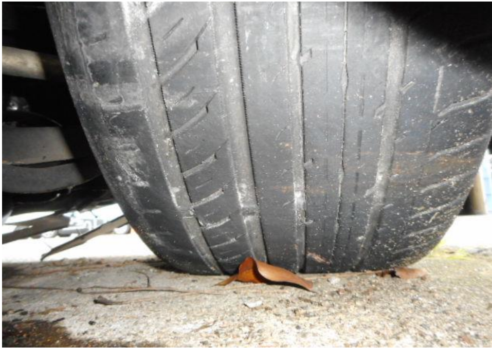
Photo 9 shows the condition of the front right tyre of the Motor Car, which was observed to be in serviceable condition with remaining tread depth of approximately 2.9mm. The tyre, which was wrapped around alloy wheel rim, was also observed to be sufficiently inflated for vehicular operation.
