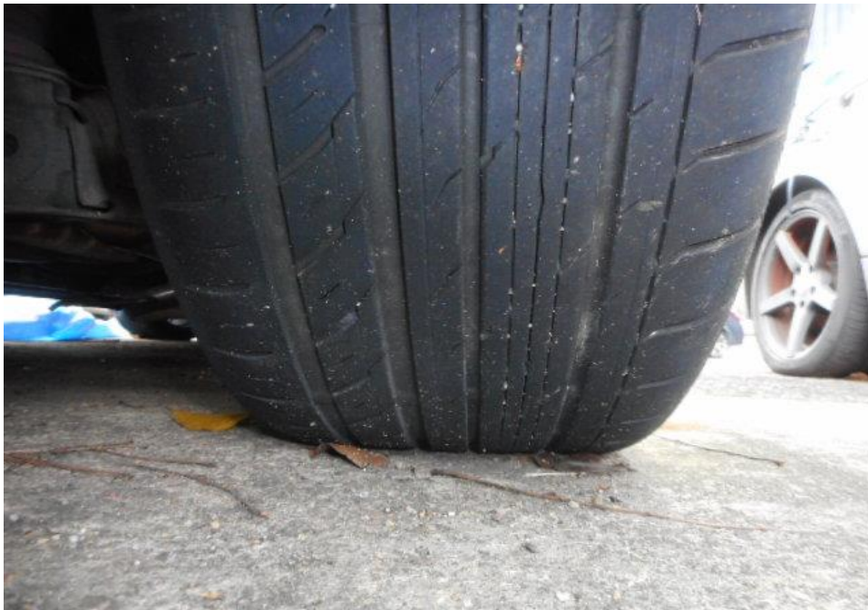
Photo 10 shows the condition of the rear right tyre of the Motor Car, which was observed to be in serviceable condition with remaining tread depth of approximately 5.4mm. The tyre was also observed to be sufficiently inflated for vehicular operation with no tear, cut or burst mark(s).
