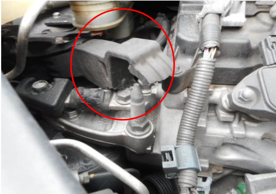
Photo 18 shows the close up view of the Motor Car's front body at the time of my inspection. The Motor car was observed to have sustained damage at its front portion. Its engine mounting (circled) was amongst the various components in the engine compartments were also damaged as a result of the accident.
