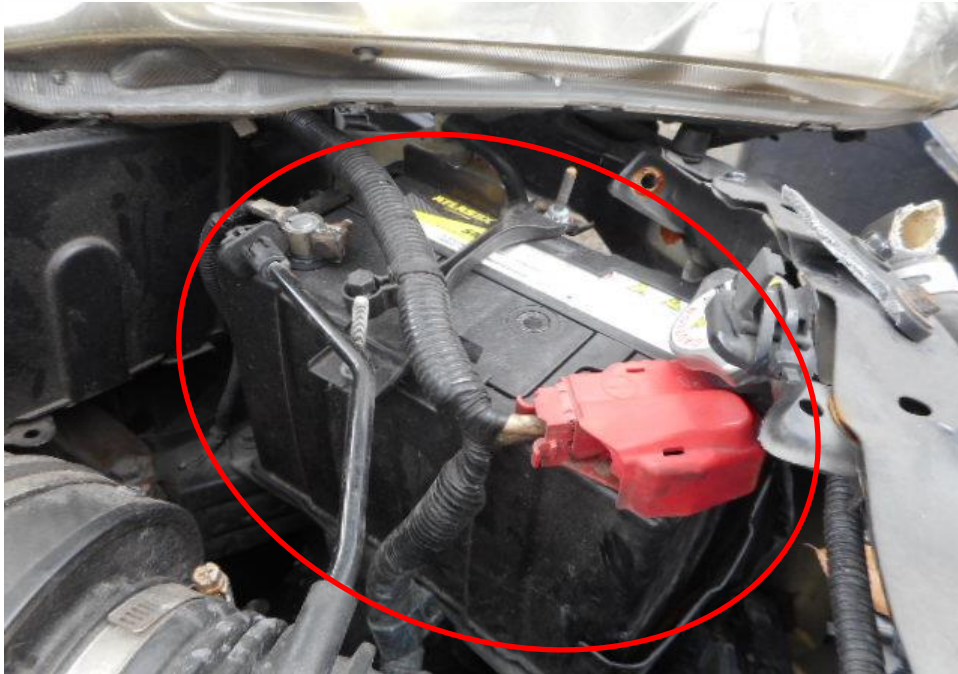
Photo 20 shows the close up view of the Motor Car's front body at the time of my inspection. The Motor car was observed to have sustained damage at its front portion. Its ignition system battery (circled) was amongst the various components in the engine compartments were also damaged as a result of the accident.
