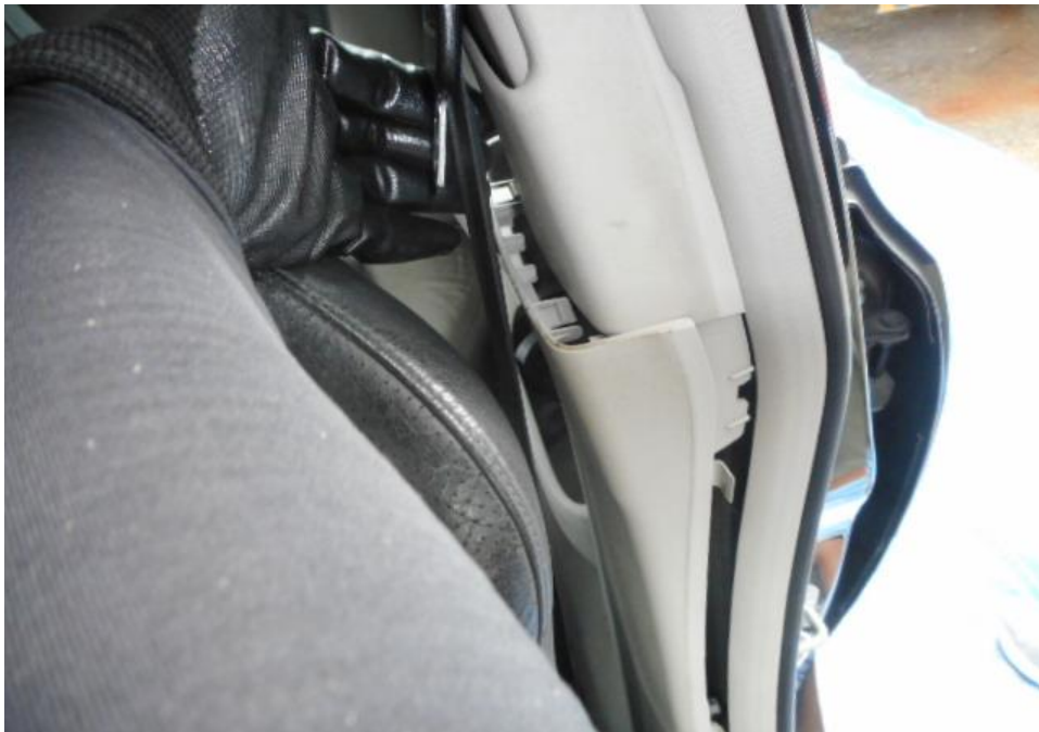
Photo 29 shows that the seat belt on the left seat was not worn at the material time of accident as the safety pre-tensioners was activated at the moment of impact and caused the seat belt to be locked into the last position.
