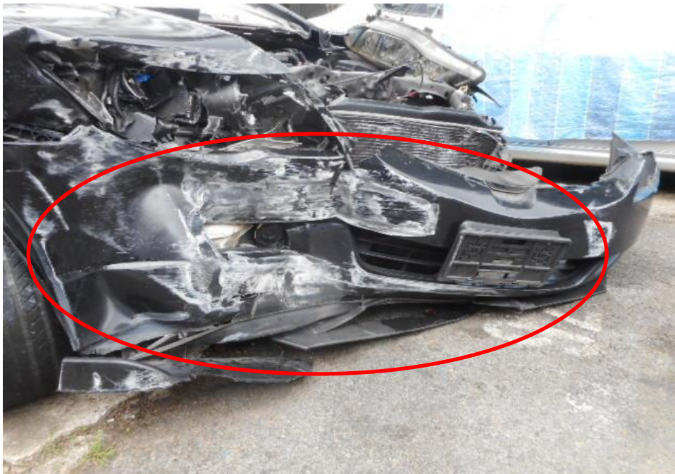
Photo 4 shows the close up view of the Motor Car's front body at the time of my inspection. The Motor car was observed to have sustained damage at its front portion. Its front bumper (circled) was damaged as a result of the accident.
