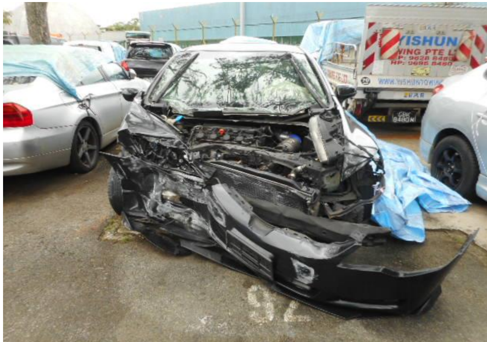
Photo 2 shows a general view of the Motor Car's front body at the time of my inspection. The Motor car was observed to have sustained damage at its front portion. Its front windscreen, front bumper, both front fender and both front headlamp was amongst the body parts and various engine components were also damaged as a result of the accident. The Supplemental Restraint System (SRS) was activated as a result of the accident.
