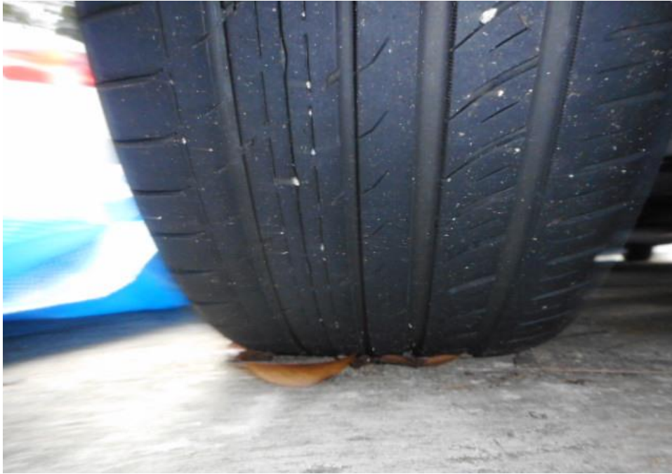
Photo 11 shows the condition of the rear left tyre of the Motor Car, which was observed to be in serviceable condition with remaining tread depth of approximately 4.9mm. The tyre was also observed to be sufficiently inflated for vehicular operation with no tear, cut or burst mark(s).
