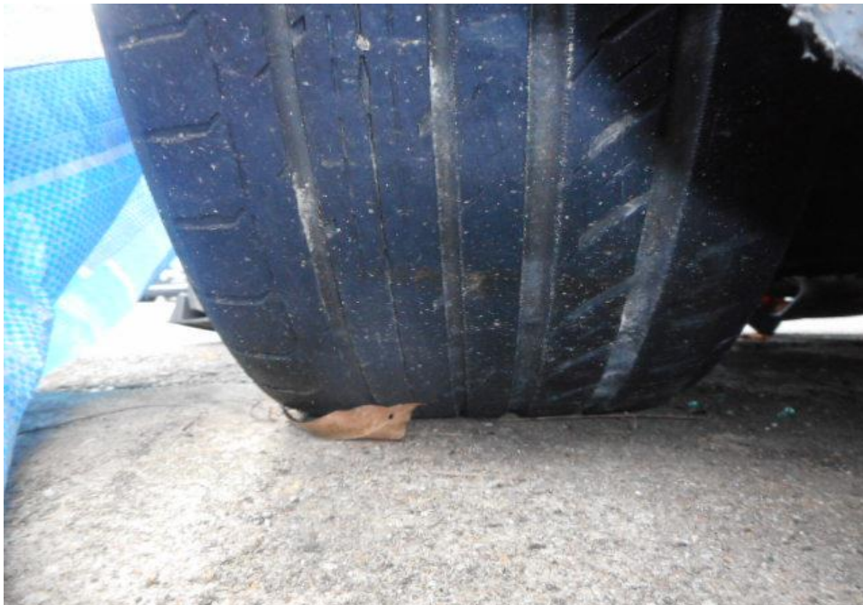
Photo 12 shows the condition of the front left tyre of the Motor Car, which was observed to be in serviceable condition with remaining tread depth of approximately 2.7mm. The tyre was also observed to be sufficiently inflated for vehicular operation with no tear, cut or burst mark(s).
