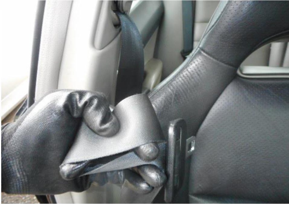
Photo 28 shows that the seat belt on the right seat was worn at the material time of accident as the safety pre-tensioners was activated at the moment of impact and caused the seat belt to be locked into the last position.
