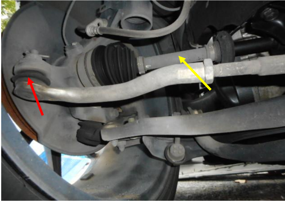
Photo 27 shows the various undercarriage components at the front left wheel of the Motor Car, in particular the steering tie rod end (red arrow) and the driveshaft (yellow arrow). The various undercarriage components of the Motor Car were all found to be intact without any visible damage. There was also no sign of fluid stain(s) observed on the various undercarriage components.
