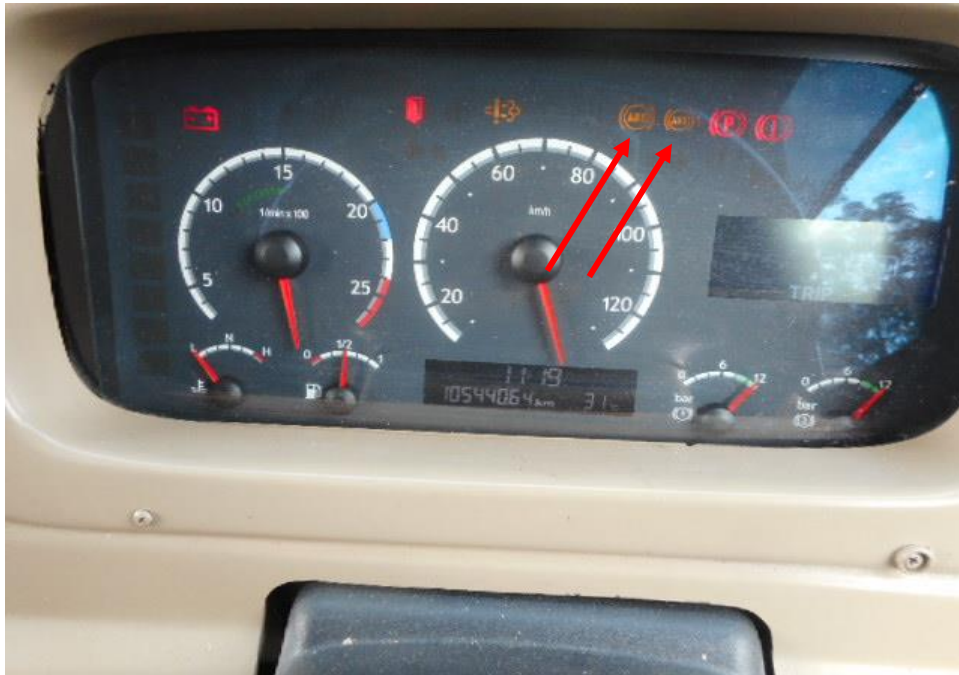
Photo 25 shows the warning light for Anti-Lock Braking System (ABS) and Anti-Slip Regulation (ASR) appearing on the instrument panel of the Motor Bus during the self-test of its various electronic operating systems when its engine was cranked.
