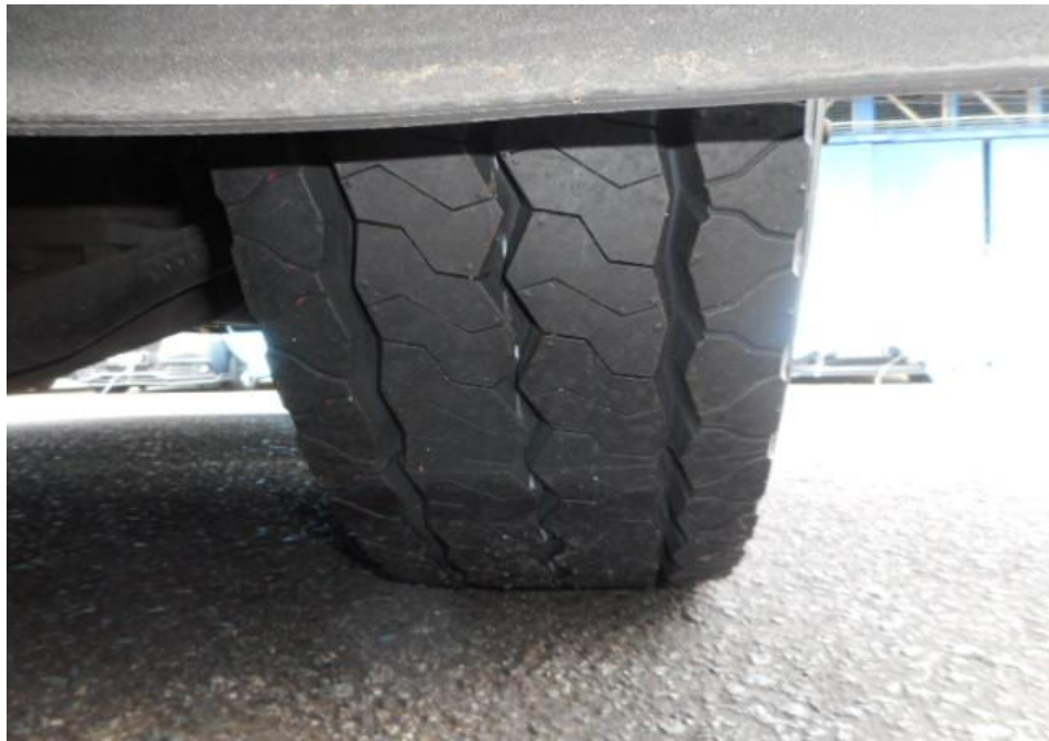
Photo 7 shows the condition of the front right tyre of the Motor Bus, which was observed to be in serviceable condition with remaining tread depth of approximately 14.1mm. The tyre, which was wrapped around standard steel wheel rim, was also observed to be sufficiently inflated for vehicular operation. There was no tear, cut or burst mark(s) on the outer and the inner sidewalls as well as across the tread of the 6 tyres that were fitted on the Motor Bus.
