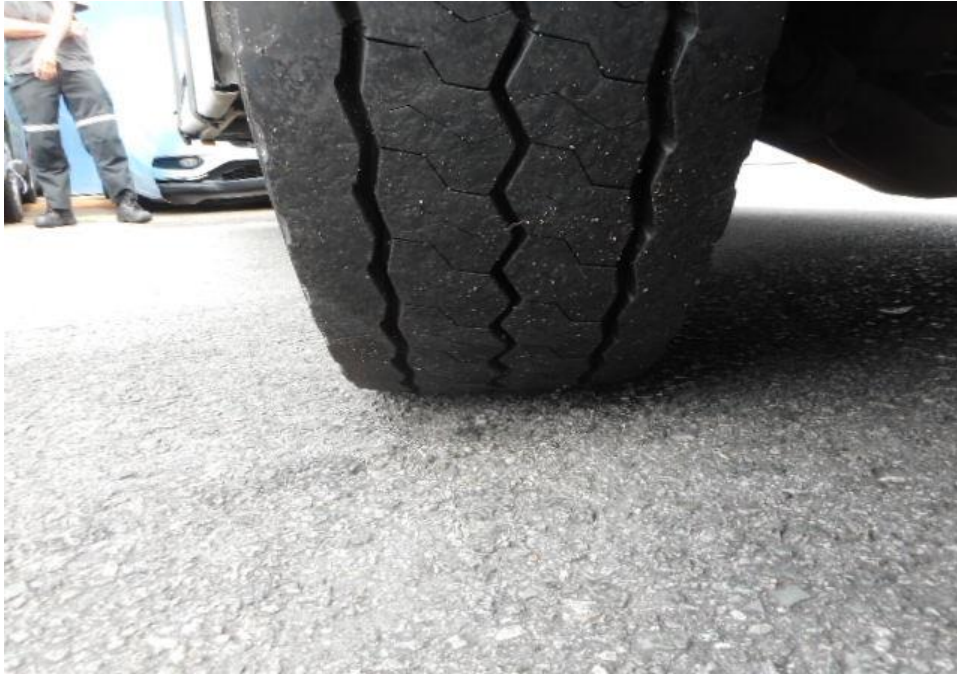
Photo 10 shows the condition of the front left tyres of the Motor Bus, which were observed to be in serviceable condition with remaining tread depth of approximately 12.3mm. There was also no tear, cut or burst mark(s) on the outer and the inner sidewalls as well as across the tread of the 6 tyres that were fitted on the Motor Bus.
