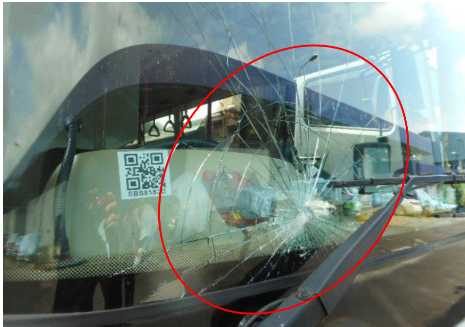
Photo 3 shows a close up view of the front body of the Motor Bus at the time of my inspection. The Motor Bus was observed to have sustained damages at its front windscreen was observed to be damaged at time of our inspection.
