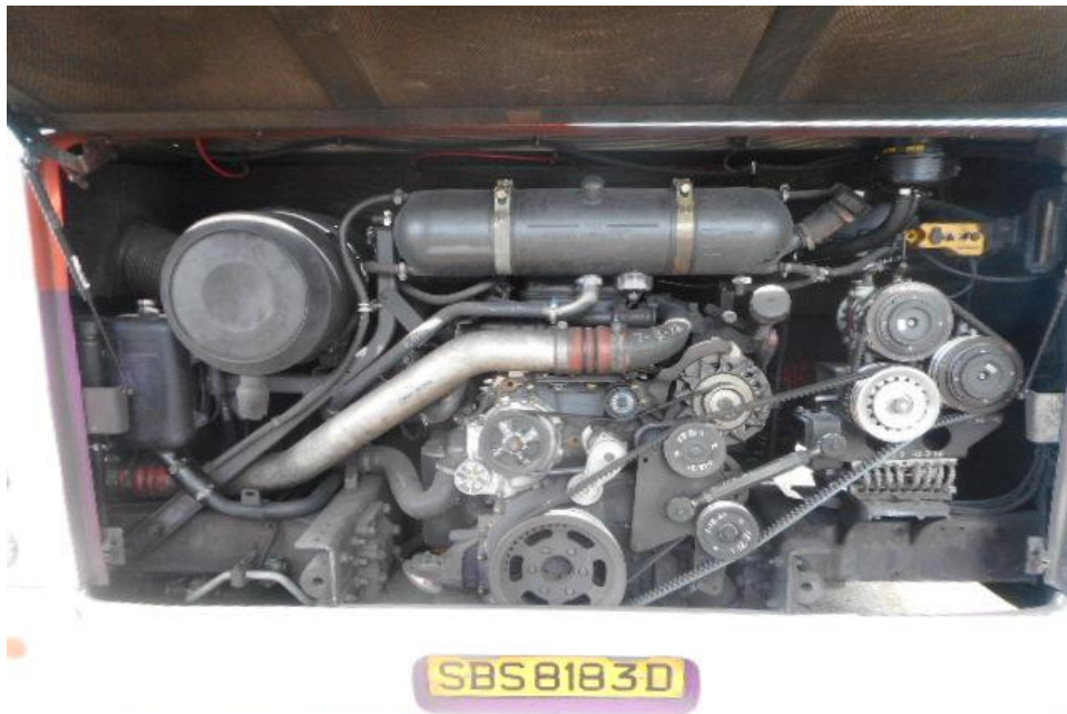
Photo 11 shows a general view of the Motor Bus's engine compartment, which was accessed by lifting the rear of the Motor Bus. The various parts and components inside the engine compartment were unaffected by the accident. There was also no sign(s) or indication(s) of fresh fluid leakage and/or fluid stain within the engine compartment
