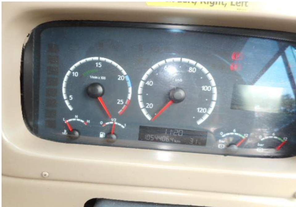
Photo 26 shows no warning lights illuminated on the instrument panel of the Motor Bus after the engine was cranked. This would suggest that there was no abnormality to the various electronic operating systems of the Motor Bus, like the ABS, ASR and etc.
