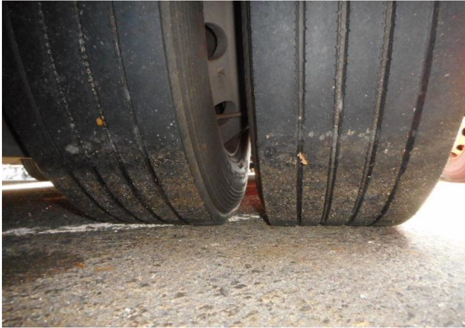
Photo 8 shows the condition of the rear right tyre of the Motor Bus, which was observed to be in serviceable condition with remaining tread depth of approximately 8mm. The tyre, which was wrapped around standard steel wheel rim, was also observed to be sufficiently inflated for vehicular operation.
