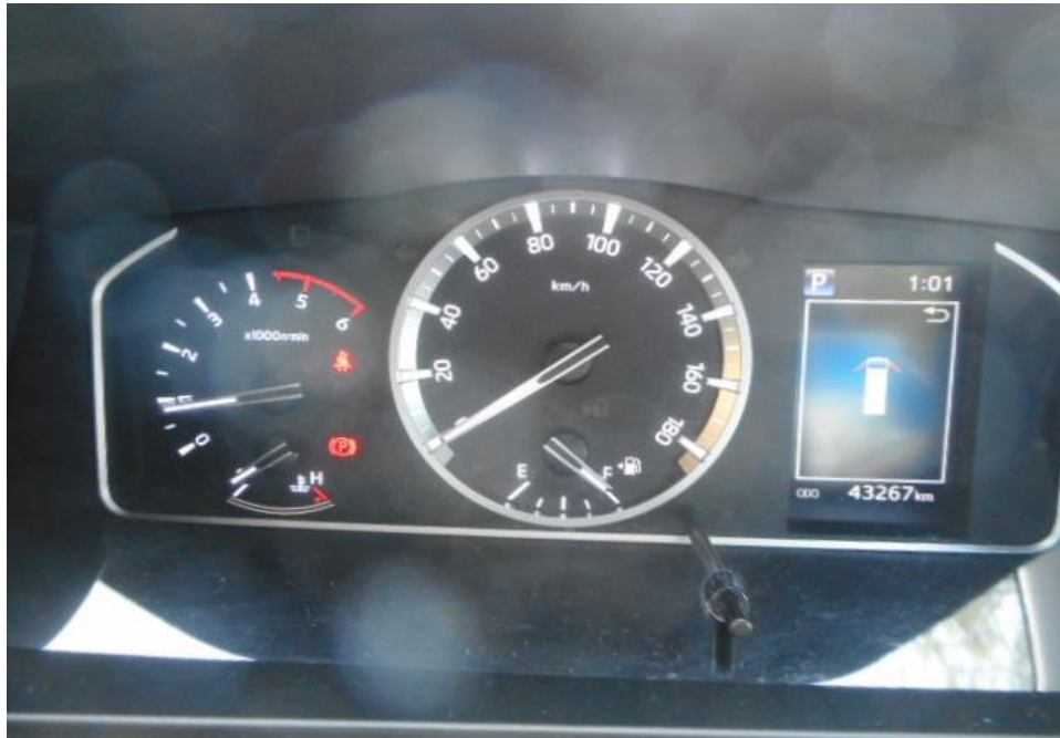
Photo 24 shows no warning lights illuminated on the instrument panel of the Motor Van after the engine was cranked. This would suggest that there was no abnormality to the electronic operating system of the Motor Van, like the SRS, TCS, ABS and etc.
