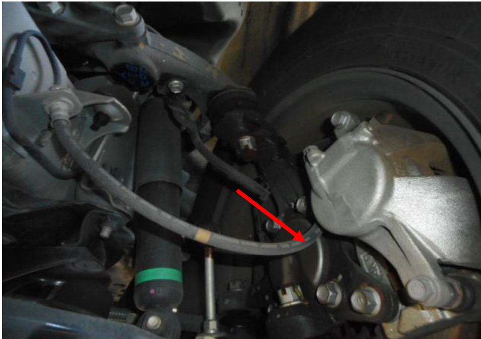
Photo 18 shows the brake hose/pipe (arrowed) at the front right wheel of the Motor Van. I did not observe any leakage of brake fluid at the time of my inspection of the Motor Van. Static tests of the Motor Van's braking system had indicated that there was no internal leakage of pressure/vacuum. The undercarriage components of the Motor Van were also all found to be intact and without any visible damage.
