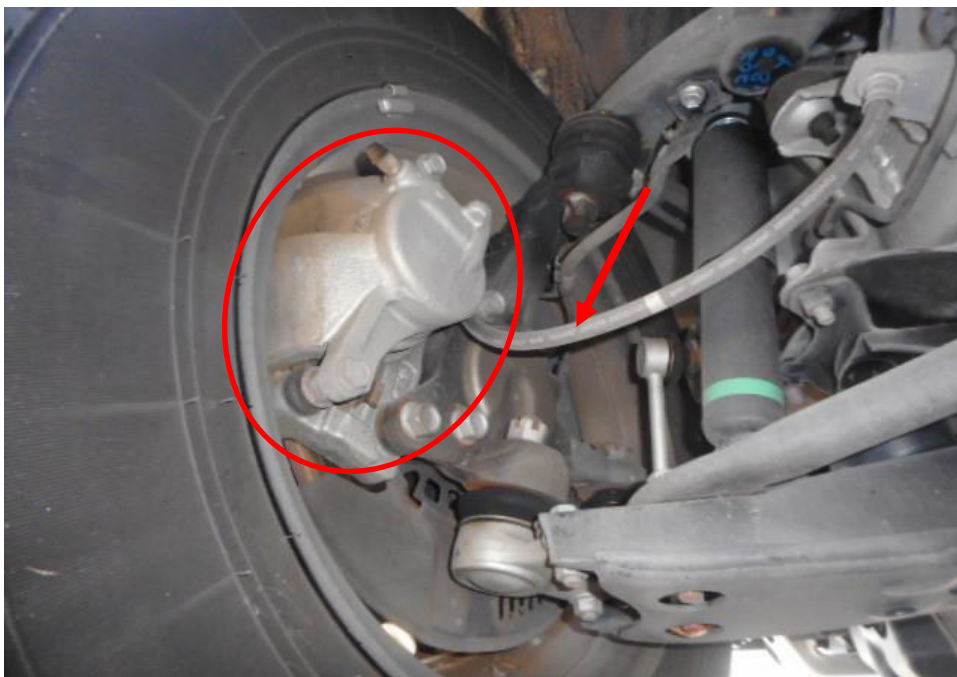
Photo 19 shows the brake hose/pipe (arrowed) at the front left wheel of the Motor Van. No leakage of brake fluid was observed. Visual examination of the various components of the braking system like the brake caliper (circled), brake booster, brake pedal etc had revealed all to be intact and without visible damage.
