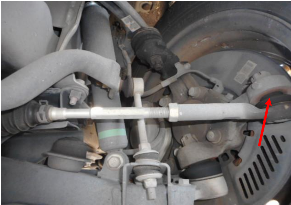
Photo 22 shows the various undercarriage components at the front left wheel of the Motor Van, which had included the steering tie rod (arrowed). The various undercarriage components of the Motor Van were all found to be intact without any visible damage.
