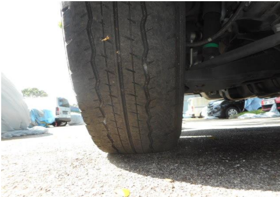
Photo 9 shows the condition of the front left tyre of the Motor Van, which was observed to be in serviceable condition with remaining tread depth of approximately 5mm. There was also no tear, cut or burst mark(s) on the outer and the inner sidewalls as well as across the tread of the Motor Van's 4 tyres.
