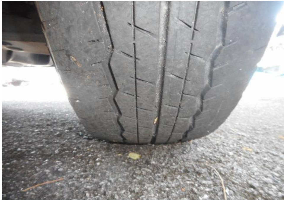
Photo 6 shows the condition of the front right tyre of the Motor Van, which was observed to be in serviceable condition with remaining tread depth of approximately 5.4mm. The tyre was sufficiently inflated for vehicular operation with no tear, cut or burst mark(s) on the outer and the inner sidewalls as well as across the tread. The 4 tyres of the Motor Van were wrapped around standard steel wheel rims without any damage.
