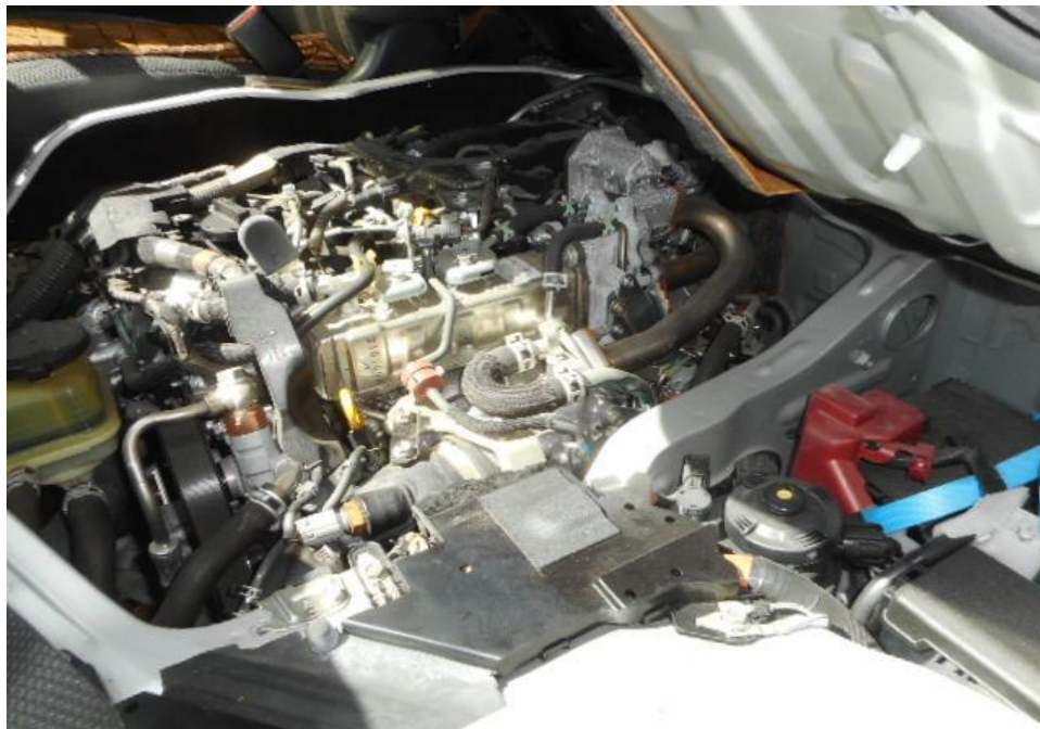
Photo 10 shows a general view of the Motor Van's engine compartment. The various parts and components inside the engine compartment were unaffected by the accident. There was also no sign(s) or indication(s) of fluid leakage and/or fluid stain within the engine compartment.
