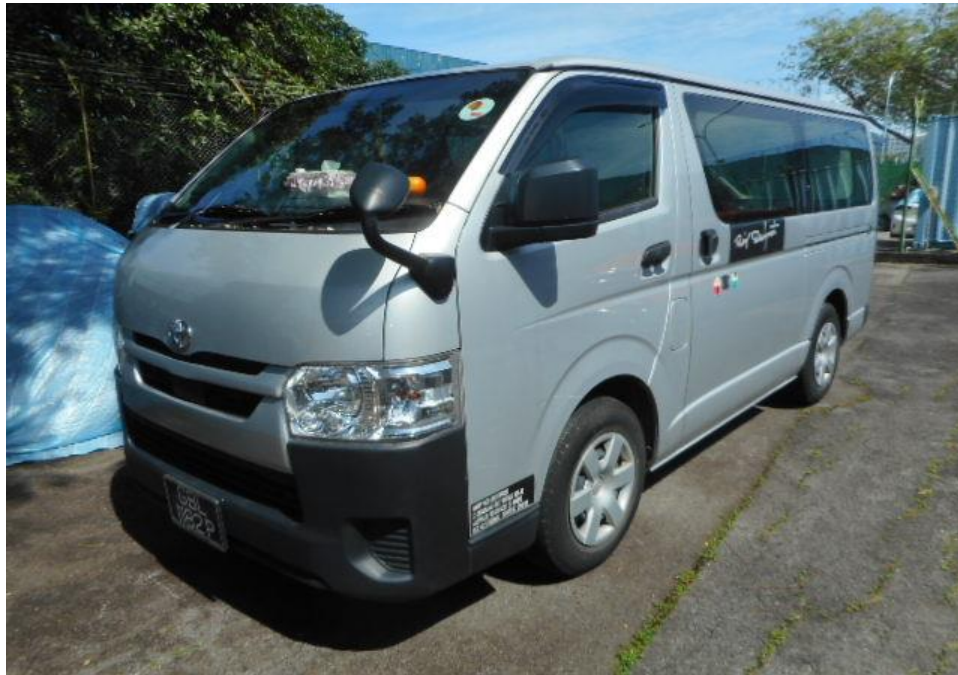
Photo 4 shows a general view of the Motor Van's left body at the time of my inspection. The left portion of the Motor Van was observed to have been unaffected by the accident.
