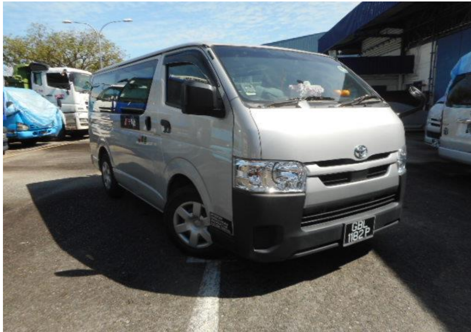
Photo 20 shows the front right wheel of the Motor Van turned to its full left. During my steering system test, I did not experience any abnormal free play and/or resistance when I had turned the steering wheel towards the left and right. This would suggest that the steering system of the Motor Van was likely to be in serviceable condition at the material time of accident.
