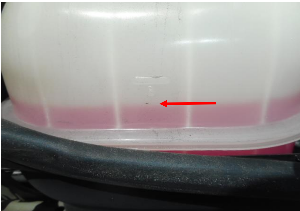
Photo 12 shows checks being carried out to the engine coolant of the Motor Van at the time of my inspection. The engine coolant was observed to be of sufficient level (arrowed) and without any visible contamination.
