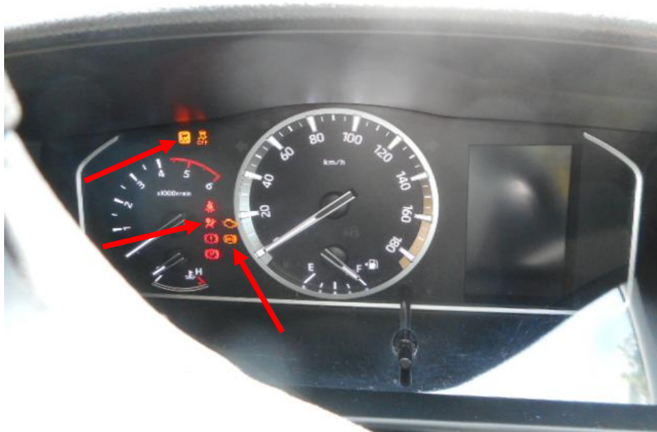
Photo 23 shows the warning light for Supplemental Restraint System (SRS), Traction Control System (TCS) and Anti-Lock Braking System (ABS) (arrowed) appearing on the instrument panel of the Motor Van during the self-test of its various electronic operating systems when its engine was cranked.
