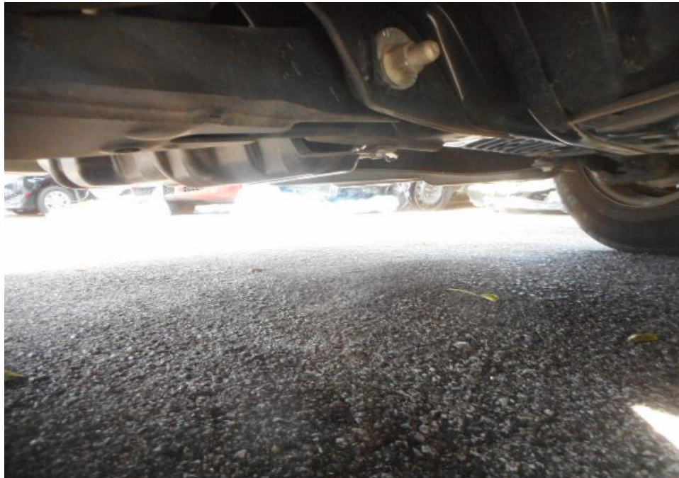
Photo 15 shows the undercarriage of the Motor Van, at the area where the engine housing and transmission housing are located. I did not find any sign(s) or indication(s) of fluid leak and/or fluid stain(s) on the underside of the Motor Van.
