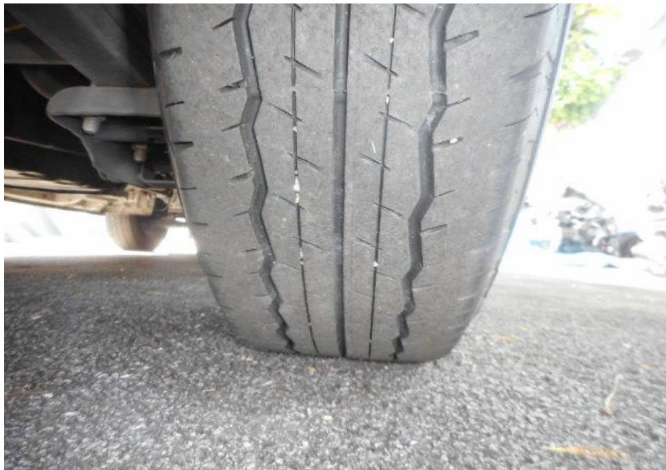
Photo 7 shows the condition of the rear right tyre of the Motor Van, which was observed to be in serviceable condition with remaining tread depth of approximately 4.5mm. The tyre was also observed to be sufficiently inflated for vehicular operation with no tear, cut or burst mark(s).
