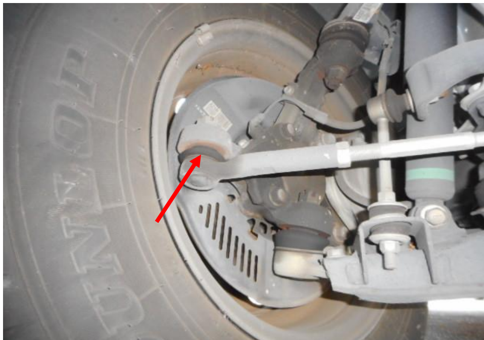
Photo 21 shows the various undercarriage components at the front right wheel of the Motor Van, in particular the steering tie rod (arrowed). The various steering components were all found to be intact, suggesting that the steering system of the Motor Van was likely to be in serviceable condition at the material time of accident. There was also no sign of fluid stain observed on the various undercarriage components at the front right wheel of the Motor Van.
