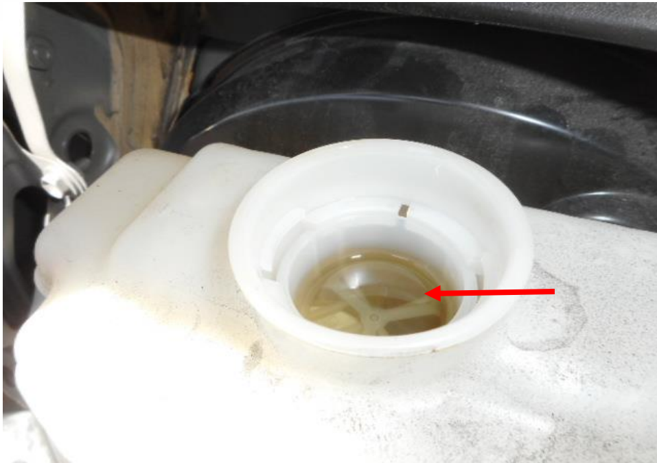
Photo 11 shows the brake fluid reservoir of the Motor Van at the time of my inspection. The brake fluid was observed to be of sufficient level (arrowed) and without any visible contamination.
