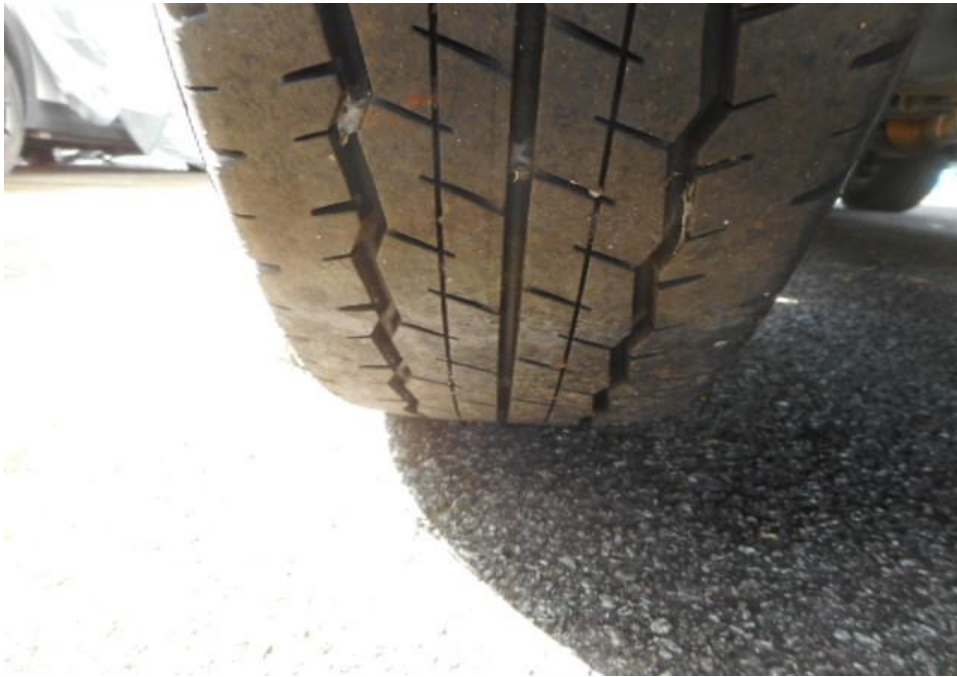
Photo 8 shows the condition of the rear left tyre of the Motor Van, which was observed to be in serviceable condition with remaining tread depth of approximately 5.6mm. The tyre, which was wrapped around steel wheel rim, was also observed to be sufficiently inflated for vehicular operation. The 4 tyres of the Motor Van were wrapped around standard steel wheel rims.
