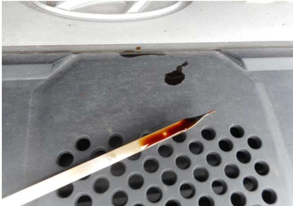
Photo 13 shows the engine oil level dipstick of the Motor Car at the time of my inspection. The engine oil was observed to be of sufficient level and without any visible contamination.
