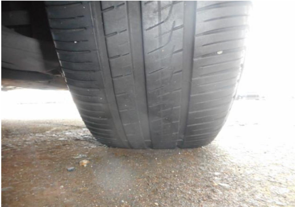
Photo 6 shows the condition of the front right tyre of the Motor Car, which was observed to be in serviceable condition with remaining tread depth of approximately 4.8mm. The tyre was also observed to be sufficiently inflated for vehicular operation with no tear, cut or burst mark(s).
