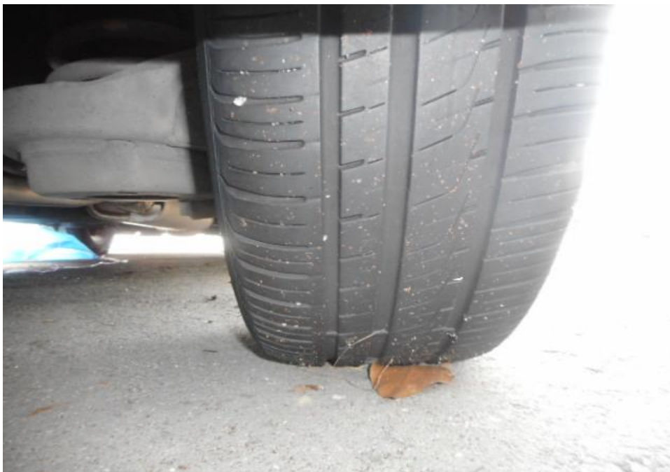
Photo 7 shows the condition of the rear right tyre of the Motor Car, which was observed to be in serviceable condition with remaining tread depth of approximately 4.8mm. The tyre was also observed to be sufficiently inflated for vehicular operation with no tear, cut or burst mark(s).
