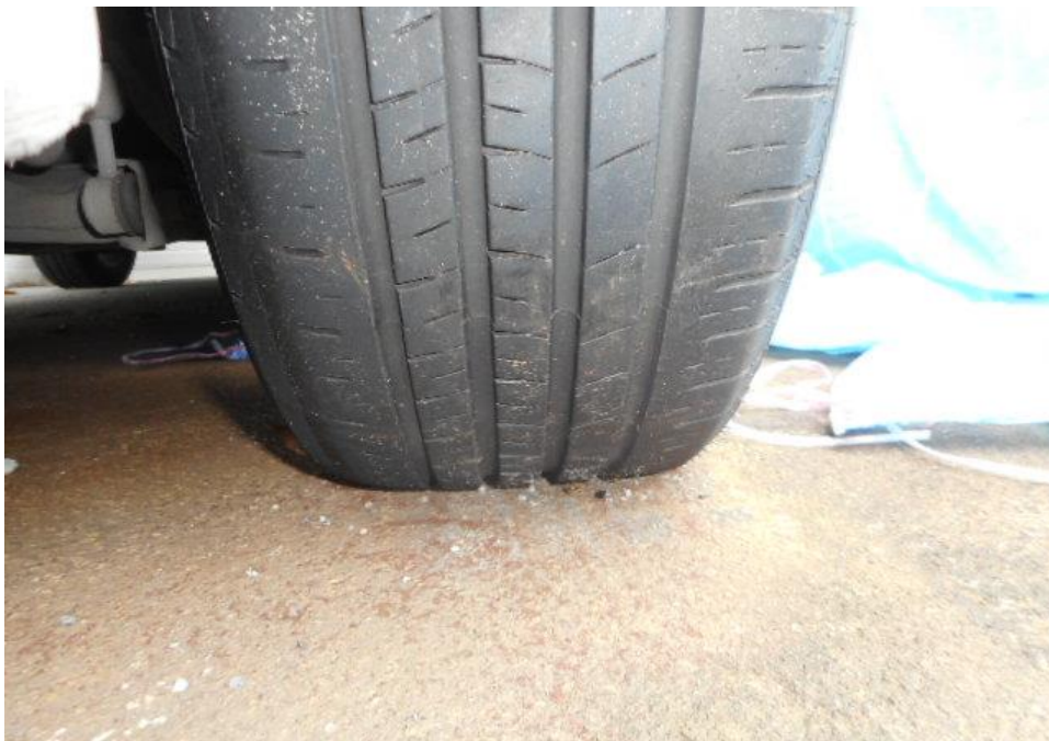
Photo 9 shows the condition of the front left tyre of the Motor Car, which was observed to be in serviceable condition with remaining tread depth of approximately 5mm. There was also no tear, cut or burst mark(s) on the outer and the inner sidewalls as well as across the tread of the Motor Car's 4 tyres.
