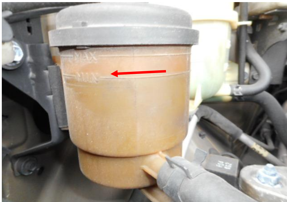
Photo 14 shows the power steering fluid level dipstick of the Motor Car at the time of my inspection. The power steering fluid was observed to be of sufficient level and without any visible contamination.
