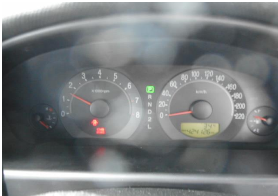
Photo 24 shows no warning lights illuminated on the instrument panel of the Motor Car after the engine was cranked. This would suggest that there was no abnormality to the electronic operating system of the Motor Car, like the ABS etc.
