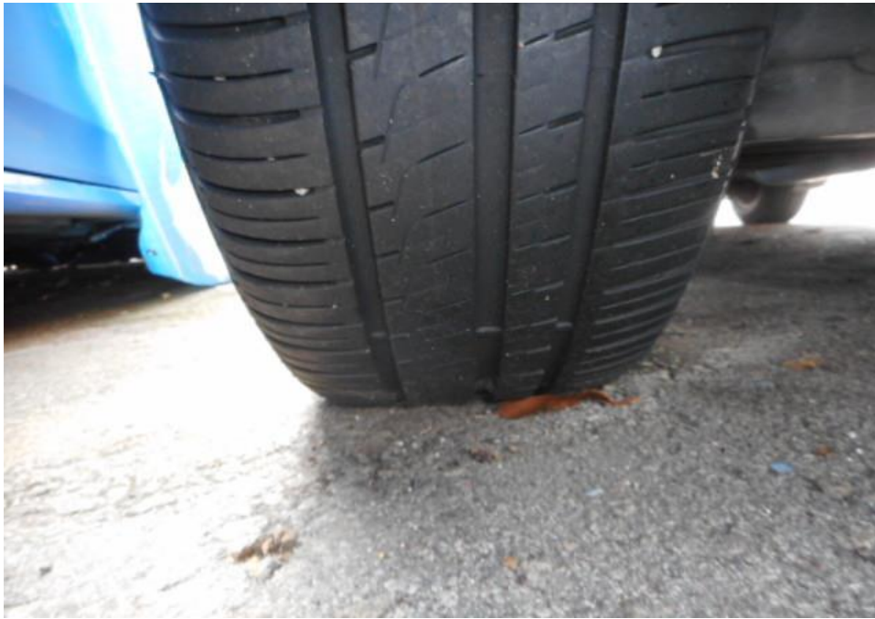
Photo 8 shows the condition of the rear left tyre of the Motor Car, which was observed to be in serviceable condition with remaining tread depth of approximately 4.8mm. The tyre, which was wrapped around alloy wheel rim, was also observed to be sufficiently inflated for vehicular operation. The 4 tyres of the Motor Car were wrapped around standard alloy wheel rims.
