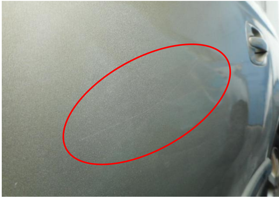
Photo 4 shows a close up view of the Motor Car's left body at the time of my inspection. The left portion of the Motor Car was observed to have sustained damage. Its left rear door (circled) was the body part that were damaged as a result of the accident.
