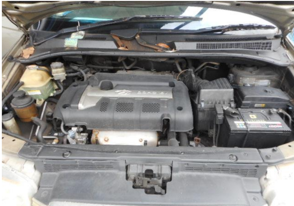
Photo 10 shows a general view of the Motor Car's engine compartment. The various parts and components inside the engine compartment were unaffected by the accident. There was also no sign(s) or indication(s) of fluid leakage and/or fluid stain within the engine compartment.
