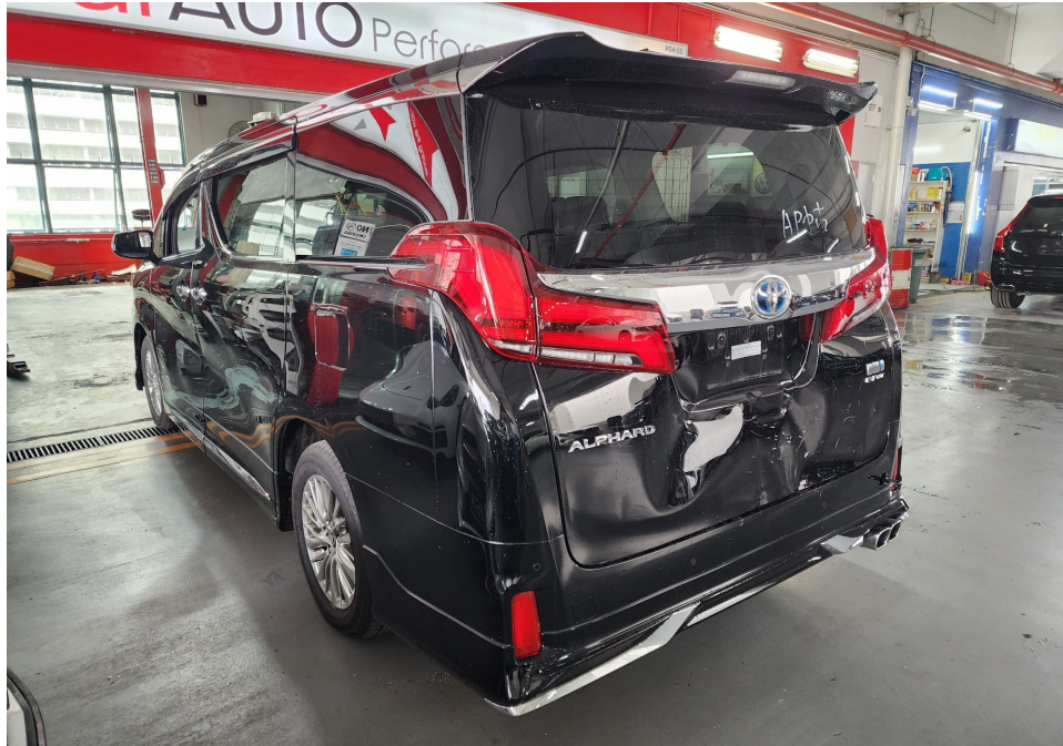
Photo 3 shows the rear left body of the Motor Car (photograph provided to me). The Motor Car was observed to have sustained damage at its rear portion. The rear bumper, rear tailgate, rear tailgate upper chrome moulding, rear tailgate left reflector lamp, rear tailgate right reflector lamp and rear tailgate emblems were amongst the body parts that were observed to have been damaged.
