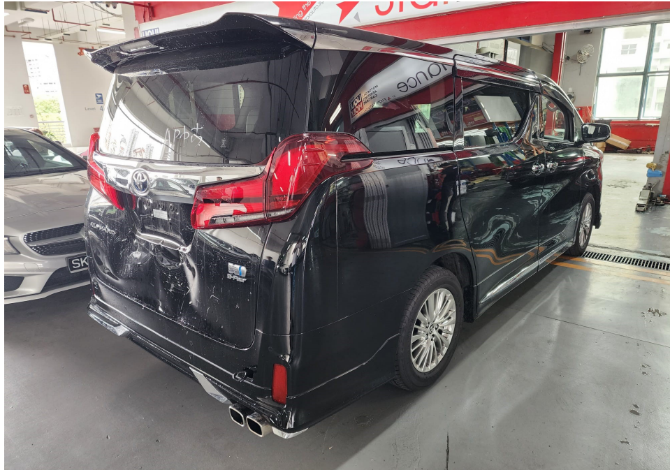
Photo 1 shows the rear right body of the Motor Car (photograph provided to me). The Motor Car was observed to have sustained damage at its rear portion. The rear bumper, rear tailgate, rear tailgate upper chrome moulding, rear tailgate left reflector lamp, rear tailgate right reflector lamp and rear tailgate emblems were amongst the body parts that were observed to have been damaged.
