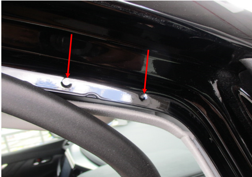
Photo 34 shows the right side "A" pillar of the Motor Car. I did not find any weld marks other than original spot weld marks (arrowed) on the right side "A" pillar of the Motor Car, which indicates that there was no re-welding works carried out. In general, I had found all the non-detachable body panels of the Motor Car to be originally fitted at the time of my inspection.
