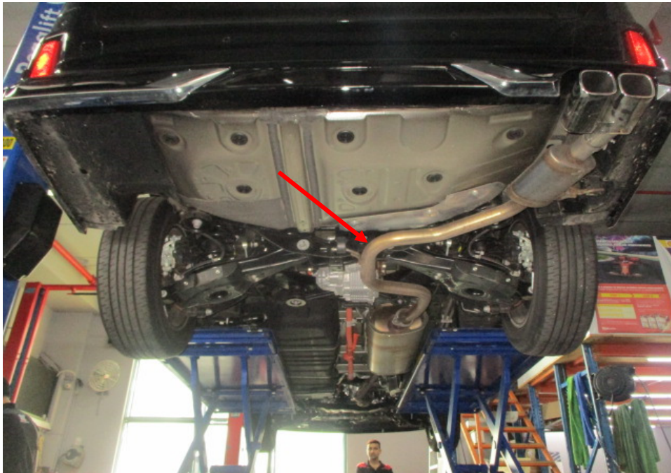
Photo 27 shows a general view of the rear section of the Motor Car's exhaust system. My examination of the Motor Car's exhaust system revealed no sign(s) or indication(s) of any cut or weld marks along its exhaust pipe (arrowed), on its catalytic converter, on its centre resonator box and on its rear muffler.
