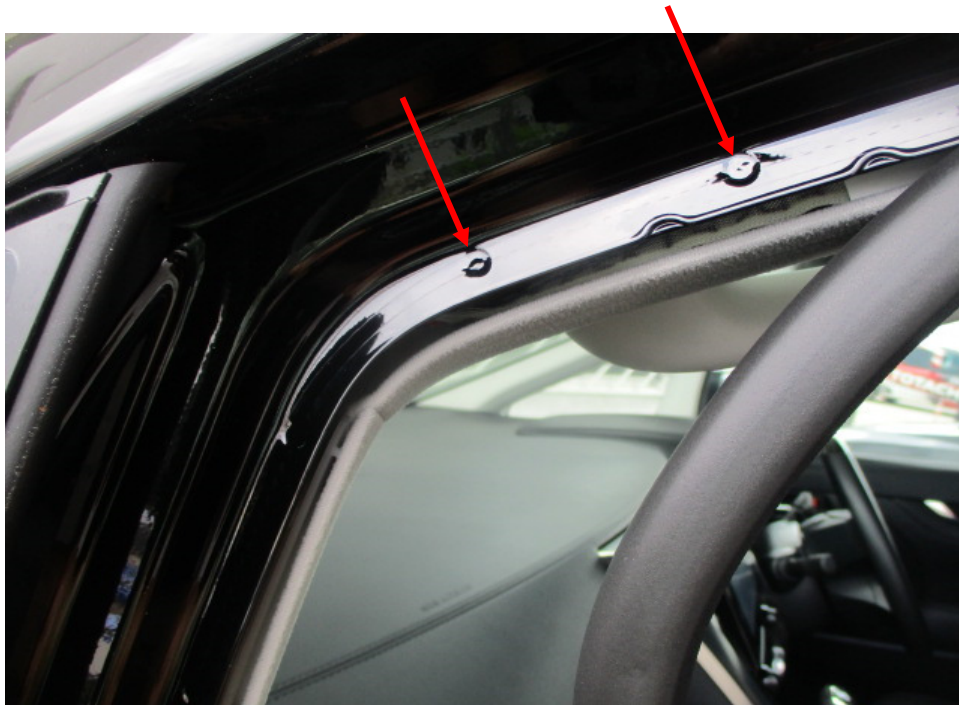
Photo 35 shows the left side "A" pillar of the Motor Car. I did not find any weld marks other than original spot weld marks (arrowed) on the left side "A" pillar of the Motor Car, which indicates that there was no re-welding works carried out. In general, I had found all the non-detachable body panels of the Motor Car to be originally fitted at the time of my inspection.
