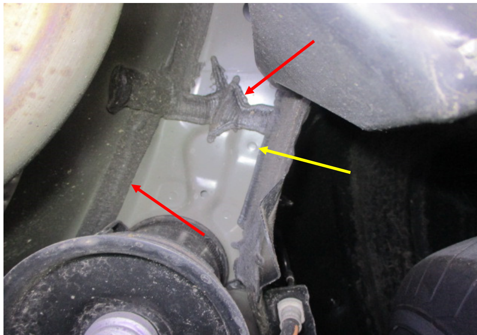
Photo 29 shows the chassis/structural body at the underside rear right of the Motor Car. I did not find any weld marks other than original spot weld marks (yellow arrow) on the chassis/structural body of the Motor Car. The original factory sealant (red arrow) at the joints along the chassis/structural body was untouched, indicating no work was done on the chassis/structural body of the Motor Car and that the chassis/structural body was originally fitted.
