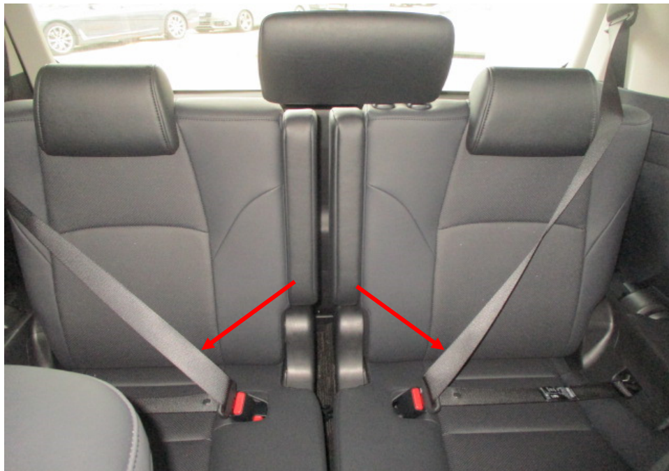
Photo 19 shows the rear seats at the 2 nd row of the Motor Car. All the seats of the Motor Car were secured via seat rails to the floorboard. They were also fitted with a retractable seat belt reel and a pre-tensioner. The seat belts (arrowed) were tested and were able to be fastened into the respective pre-tensions that were fitted on the side of each individual seat.
