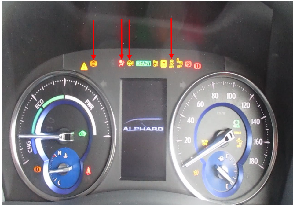
Photo 20 shows the warning lights for the various electronic safety features appearing on the instrument panel of the Motor Car during its self-test when the engine is cranked, in particular the lights for the ABS, SRS, EPS, VSC (arrowed) and the various collision prevention systems.
