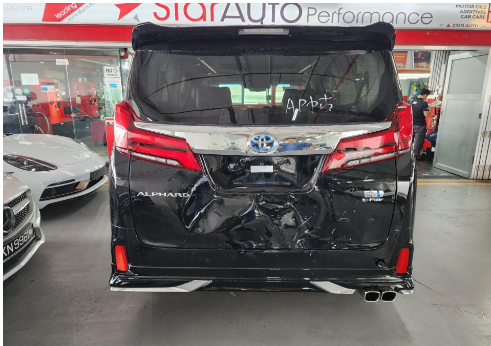
Photo 2 shows the rear body of the Motor Car (photograph provided to me). The Motor Car was observed to have sustained damage at its rear portion. The rear bumper, rear tailgate, rear tailgate upper chrome moulding, rear tailgate left reflector lamp, rear tailgate right reflector lamp and rear tailgate emblems were amongst the body parts that were observed to have been damaged.
