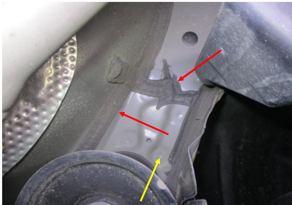
Photo 27 shows the chassis/structural body at the underside rear right of the Motor Car. I did not find any weld marks other than original spot weld marks (yellow arrow) on the chassis/structural body of the Motor Car. The original factory sealant (red arrow) at the joints along the chassis/structural body was untouched, indicating no work was done on the chassis/structural body of the Motor Car and that the chassis/structural body was originally fitted.
