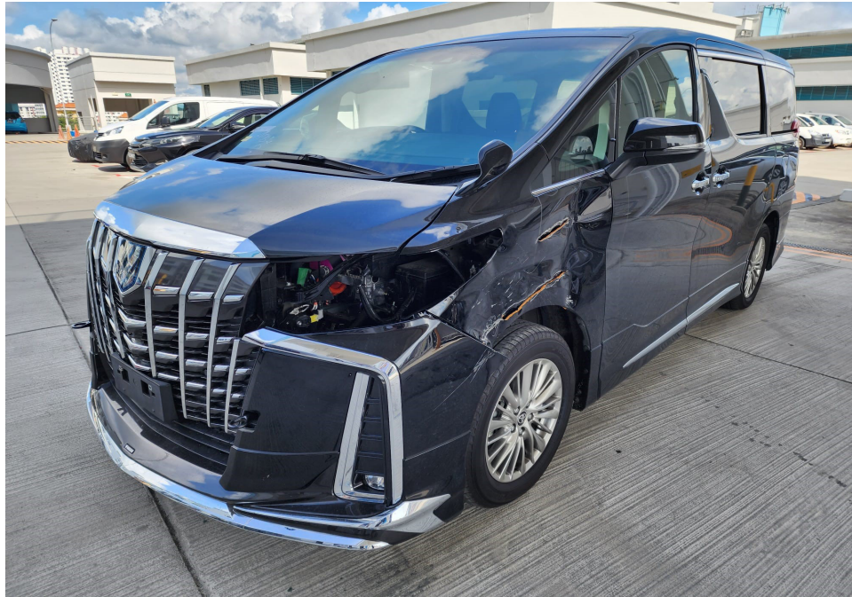
Photo 1 shows the front left body of the Motor Car (photograph provided to me). The Motor Car was observed to have sustained damage at its left side front portion. The front bumper, front left fender and front left fender inner shield were amongst the body parts that were observed to have been damaged. The front left headlamp and front left headlamp chrome moulding were observed to be missing/dislodged/damaged.
