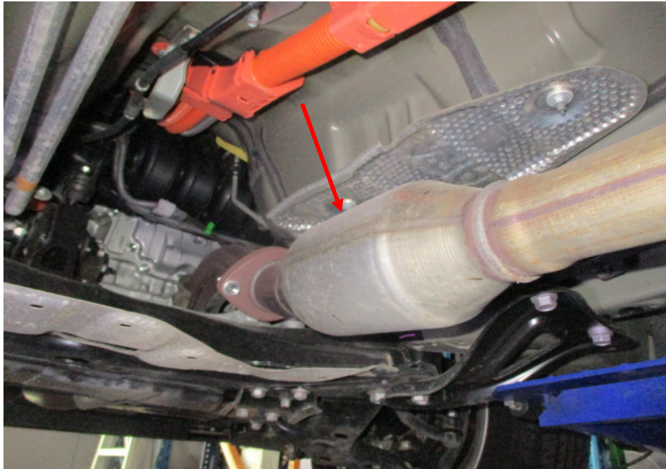
Photo 26 shows a general view of the front section of the Motor Car's exhaust system. My examination of the Motor Car's exhaust system revealed no sign(s) or indication(s) of any cut or weld marks along its exhaust pipe, on its catalytic converter (arrowed), on its centre resonator box and on its rear muffler.
