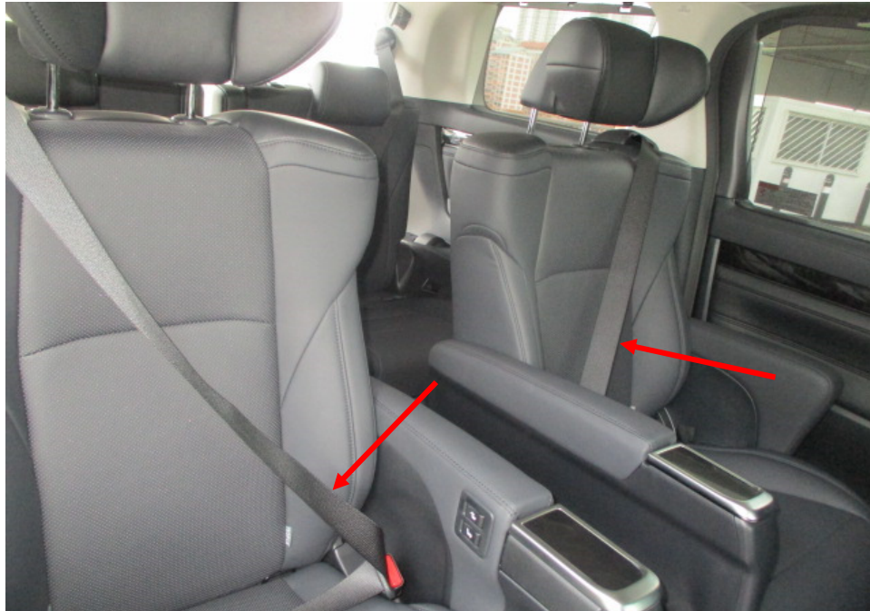
Photo 16 shows the rear seats at the 1 st row of the Motor Car. All the seats of the Motor Car were secured via seat rails to the floorboard. They were also fitted with a retractable seat belt reel and a pre-tensioner. The seat belts (arrowed) were tested and were able to be fastened into the respective pre-tensions that were fitted on the side of each individual seat.
