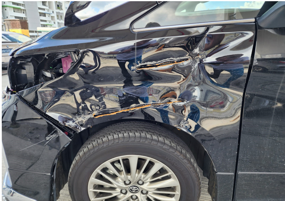
Photo 2 shows another view of the damage at the left side front portion of the Motor Car (photograph provided to me). The front bumper, front left fender and front left fender inner shield were amongst the body parts that were observed to have been damaged. The front left headlamp and front left headlamp chrome moulding were observed to be missing/dislodged/damaged.
