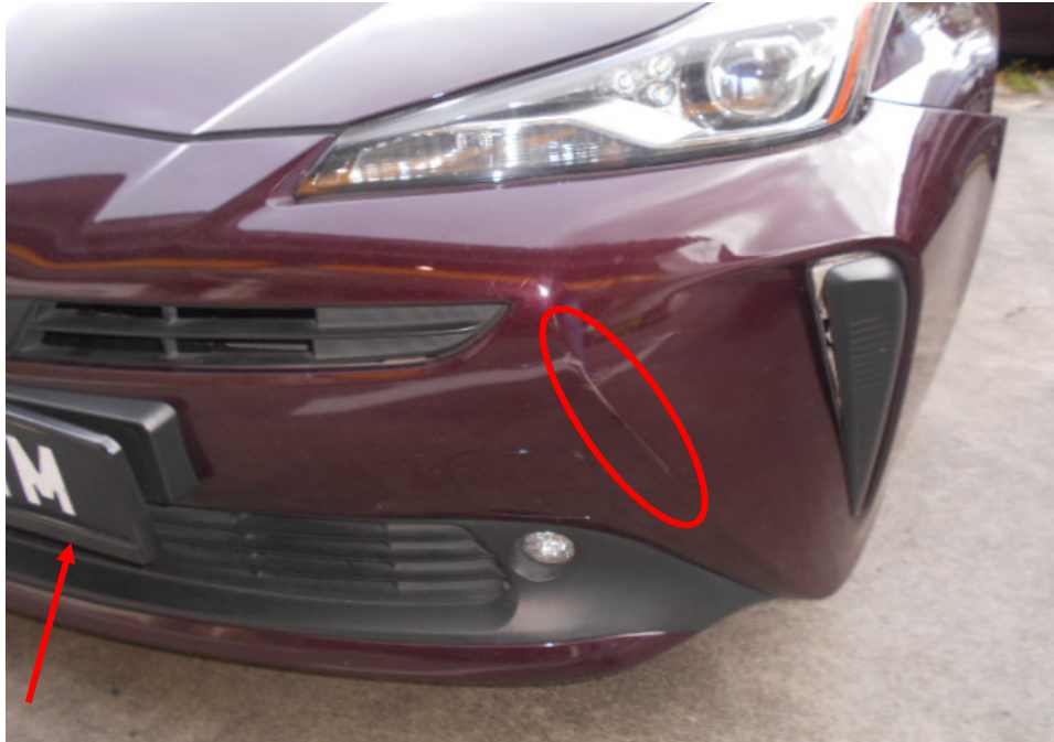
Photo 2 shows a closer view of the damaged area of the Motor Taxi at the time of inspection by LKK Auto Consultants Pte Ltd. The Motor Taxi was observed to have sustained damage at its front left portion. Marks of grazing nature was observed at the left side of its front bumper (circled). It was further observed that the front number plate was bent (arrowed).
