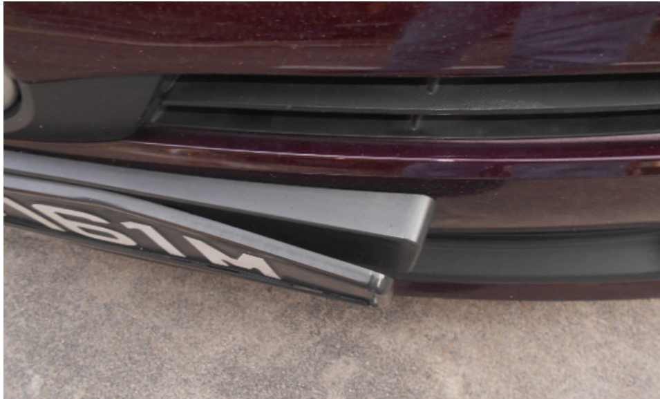
Photo 4 shows a closer view of the bent front number plate of the Motor Taxi at the time of inspection by LKK Auto Consultants Pte Ltd.
