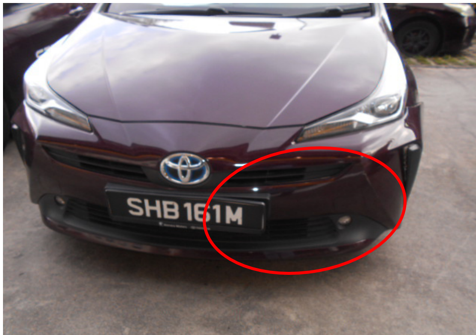
Photo 1 shows a general view of the frontal portion of the Motor Taxi at the time of inspection by LKK Auto Consultants Pte Ltd. The Motor Taxi was observed to have sustained damage at its front left portion (circled). The area of damage to the Motor Taxi corresponds to the area where the Motor Car came into very close proximity.
