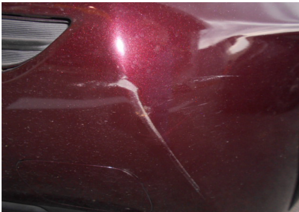
Photo 3 shows a closer view of the marks of grazing nature that was observed at the left side of the Motor Taxi's front bumper.
