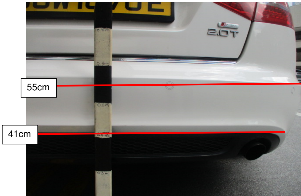
Photo 7 shows height measurement being conducted on the Motor Car. The height above ground level of the Motor Car's damaged area (refer to photograph 5 above) was approximately 41cm to 55cm. The Motor Car's damaged area was within the height above ground level of the Motor Taxi's damaged area (refer to photograph 1 & 2 above).
