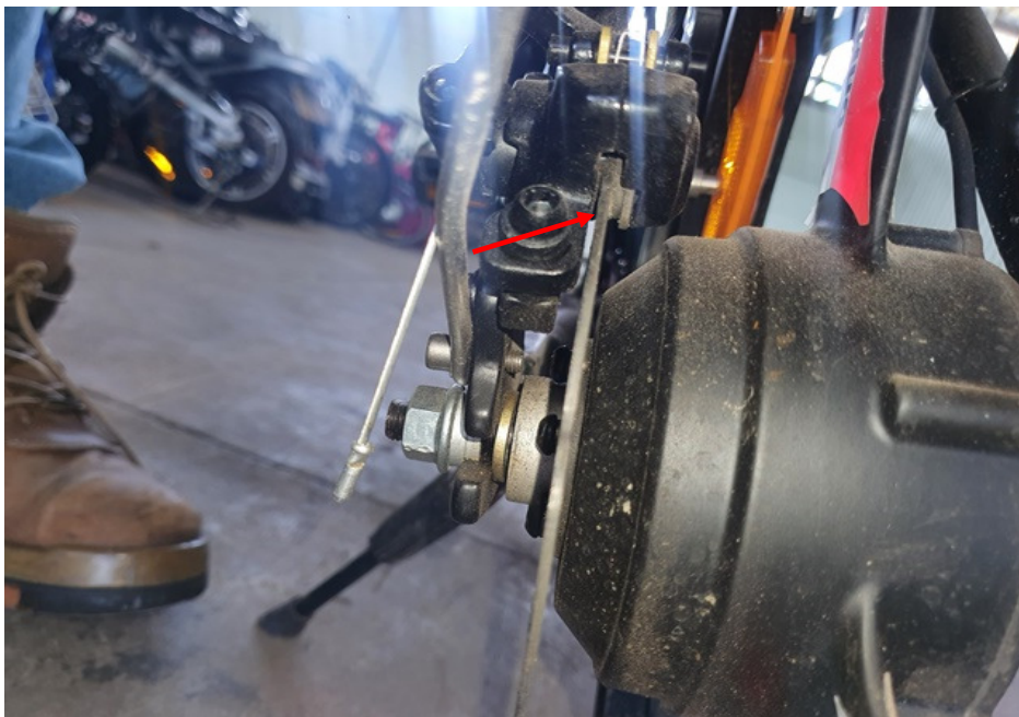
Photo 23 shows a close up view of the rear brake pads responding to the gripping action. The rear brake pads pressed against the rear brake disc (arrowed) upon depressing the left hand brake lever. This had appeared to indicate that the rear brake of the PAB was in serviceable condition.
