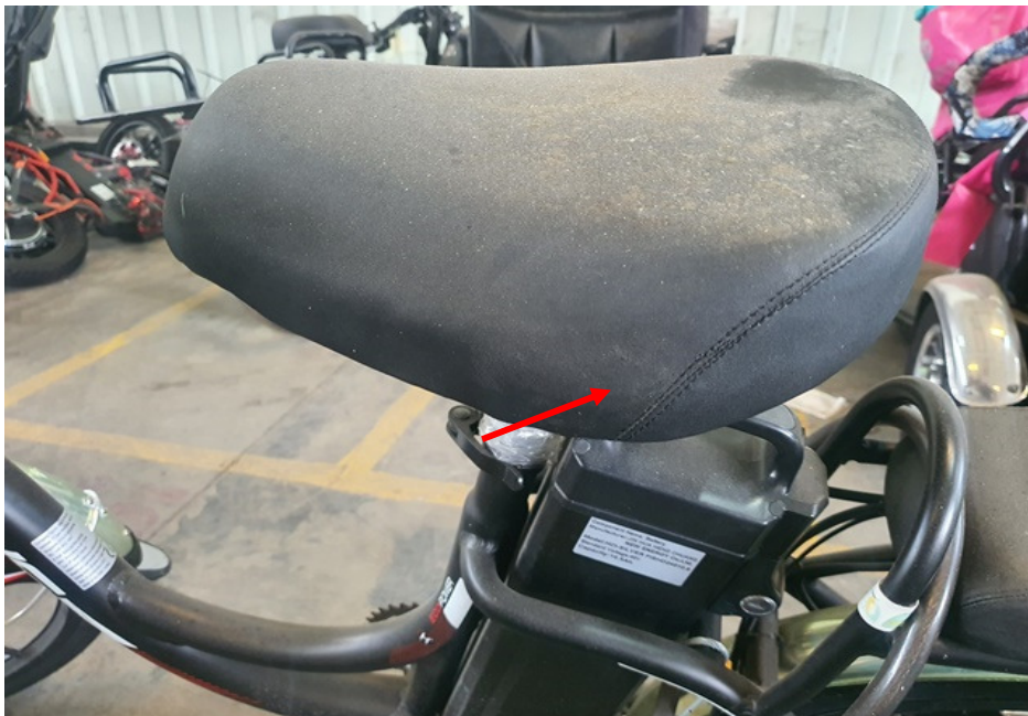
Photo 10 shows the damages of grazing nature on the seat (arrowed) of the PAB as a result of the accident.
