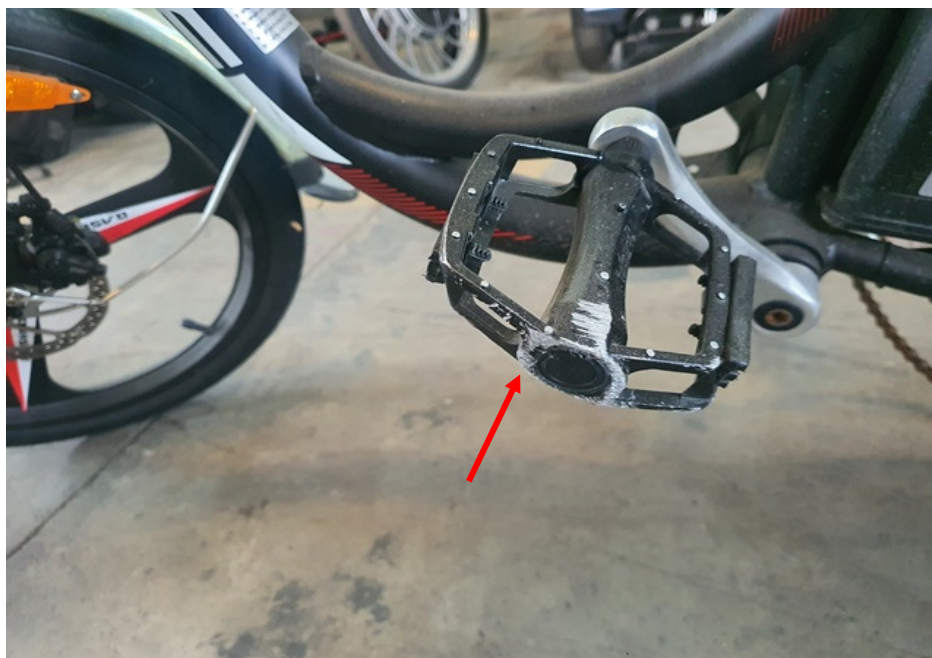
Photo 8 shows the damages of grazing nature on the left pedal (arrowed) of the PAB as a result of the accident.
