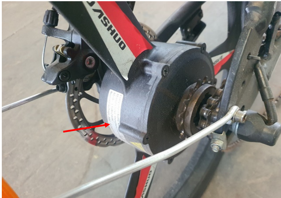
Photo 14 shows the general view of the drive motor (arrowed) of the PAB which was observed to be intact with no misalignment.
