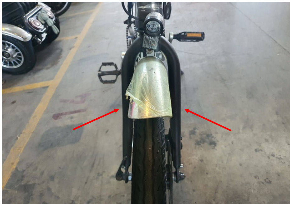
Photo 17 shows the front fork assembly (arrowed) of the PAB. The front forks and fork bracket of the PAB were both found to be intact and undamaged. Turning the PAB's handle bar towards the left and right did not produce any abnormal free play. The steering system of the PAB was in serviceable condition at the time of our inspection.
