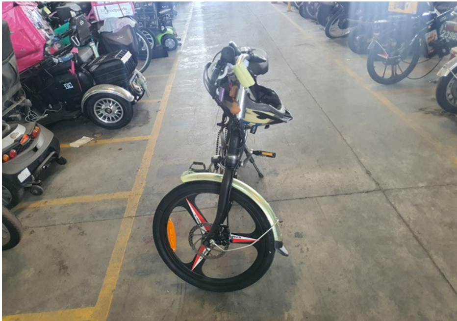
Photo 18 shows the front wheel of the PAB turned towards its full right. Turning the PAB's handle bar towards the right did not produce any abnormal free play and/or resistance. This would indicate that the steering system of the PAB was in serviceable condition at the time of our inspection.
