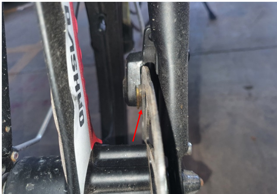
Photo 21 shows a close up view of the front brake pads responding to the gripping action. The front brake pads pressed against the front brake disc (arrowed) upon depressing the right hand brake lever. This had appeared to indicate that the front brake of the PAB was in serviceable condition.
