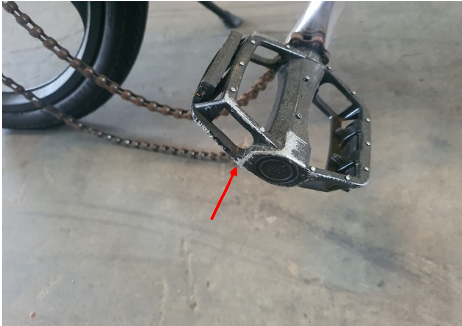
Photo 9 shows the damages of grazing nature on the right pedal (arrowed) of the PAB as a result of the accident.
