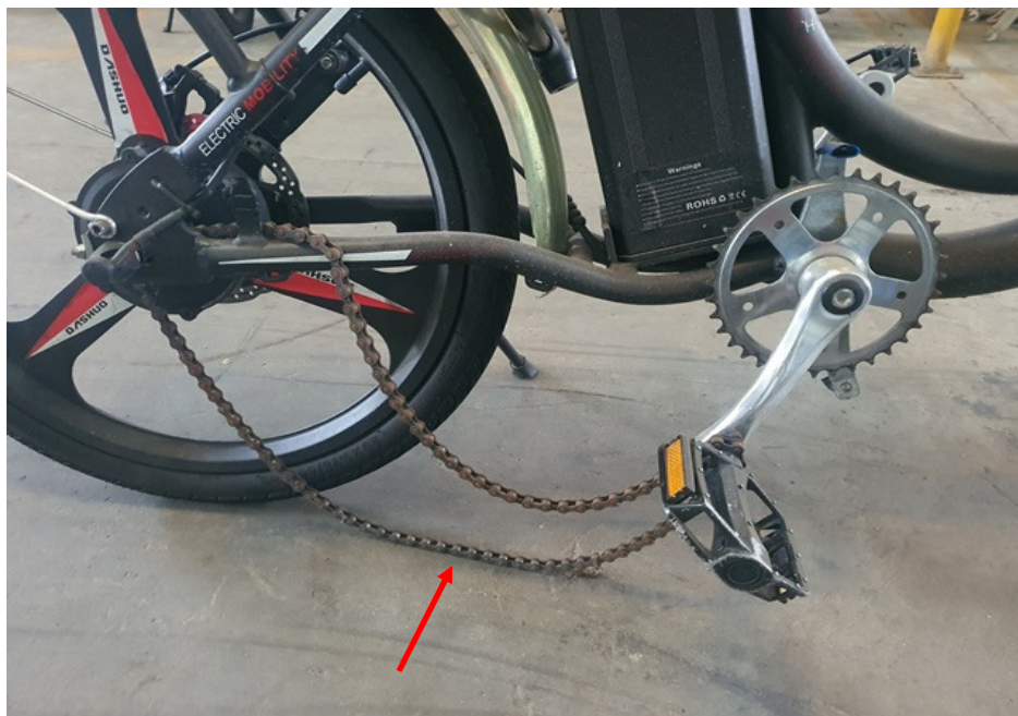
Photo 15 shows the general view of the gear train of the PAB, which was observed to be intact with no misalignment. It was also adequately lubricated for operating purposes. However the chain was observed to be dislodged from the gear train most likely as a result of the accident (arrowed).
