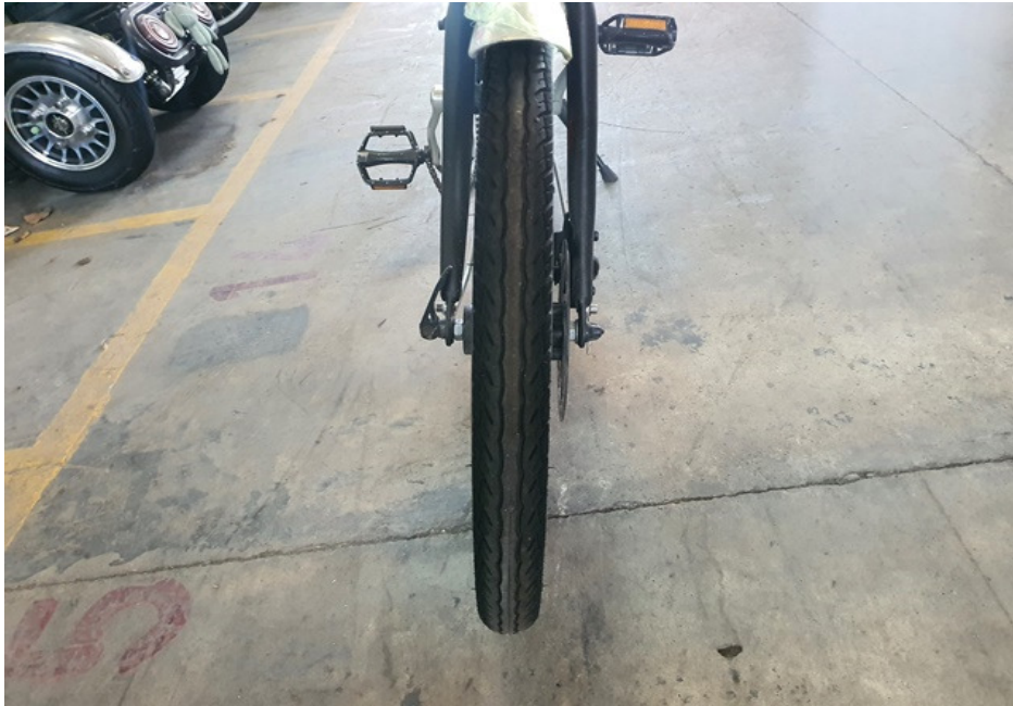
Photo 12 shows the front tyre of the PAB at the time of our inspection. The front tyre was observed to be in serviceable condition with remaining tread depth of approximately 3mm. The tyre was also observed to be sufficiently inflated for vehicular operation. We did not observe any tear, burst mark(s) and/or punctured hole(s) on the sidewalls as well as across the tread of the front tyre.
