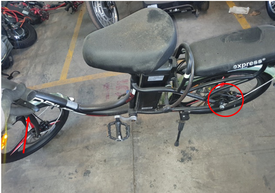
Photo 22 shows a static brake test conducted on the PAB's rear brake. There was some resistance felt upon pressing the left hand brake lever (arrowed). It also shows that the rear brake pads responded to the gripping action (circled) after depressing the left hand brake lever.
