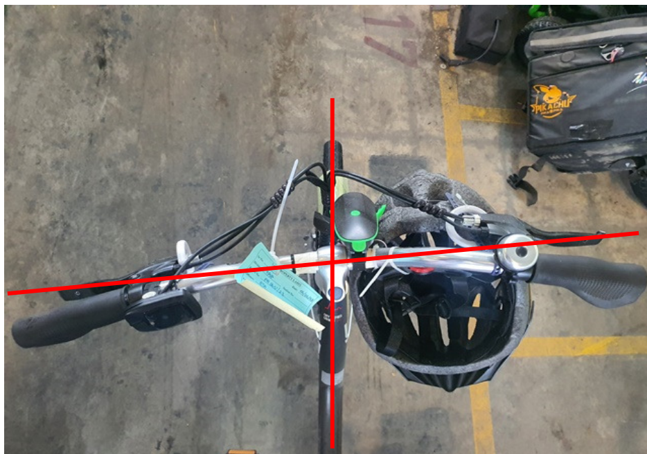
Photo 6 shows the frontal portion of the PAB (top view) at the time of our inspection. There was a misalignment of the handlebar & front tyre observed.
