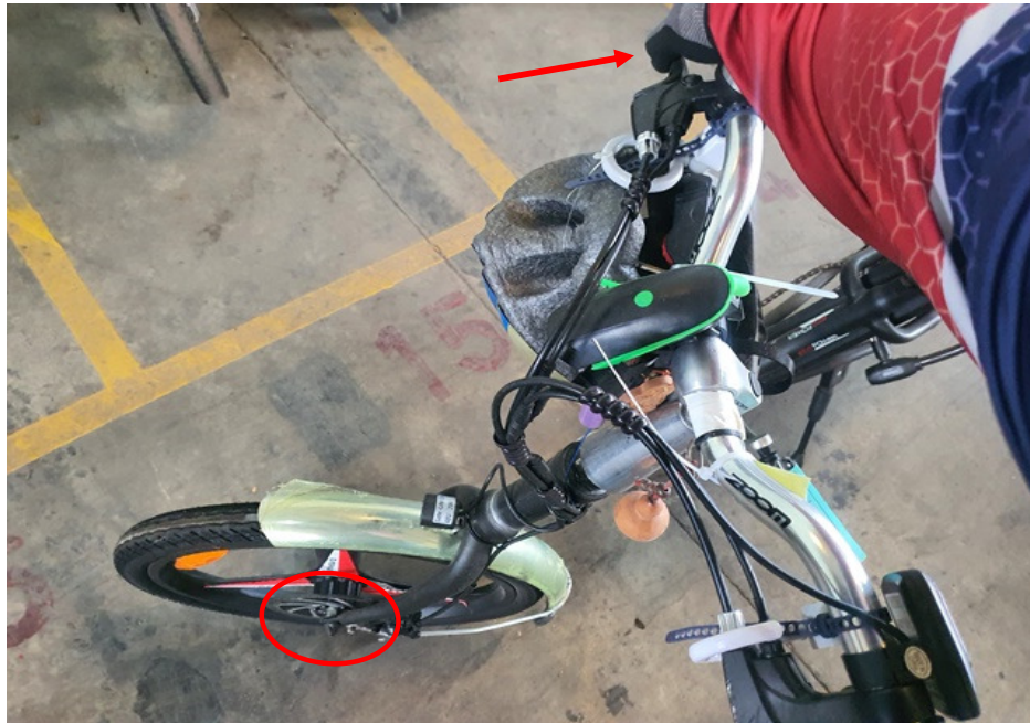
Photo 20 shows a static brake test conducted on the PAB's front brake. There was some resistance felt upon pressing the right hand brake lever (arrowed). It also shows that the front brake pads responded to the gripping action (circled) after depressing the right hand brake lever.
