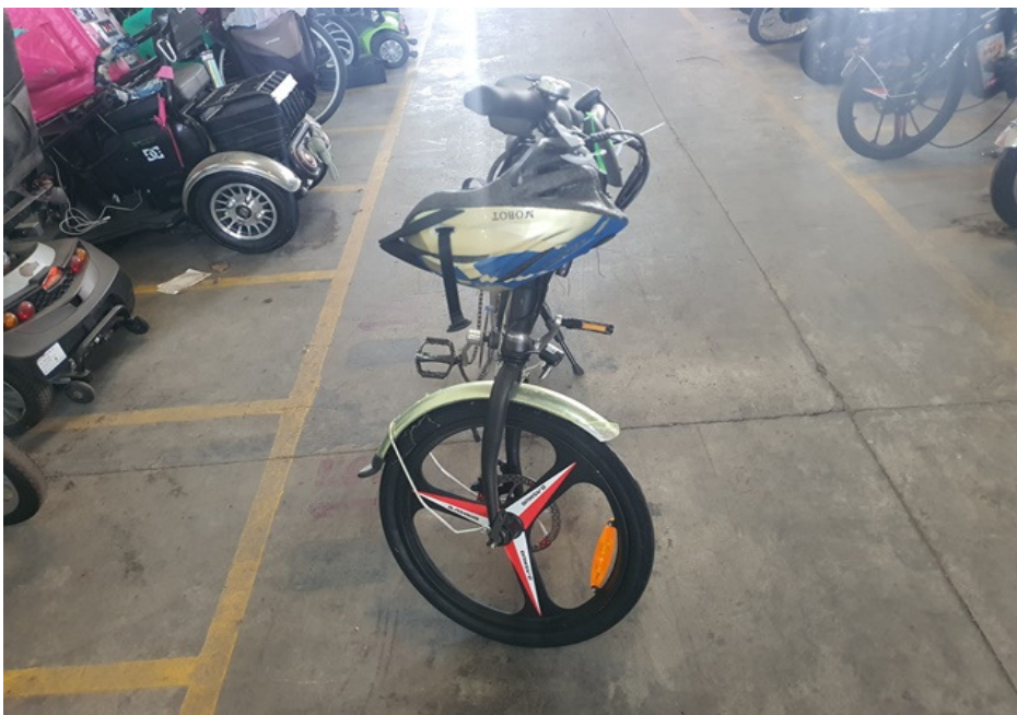
Photo 19 shows the front wheel of the PAB turned towards its full left. Turning the PAB's handle bar towards the left did not produce any abnormal free play and/or resistance. This would indicate that the steering system of the PAB was in serviceable condition at the time of our inspection.
