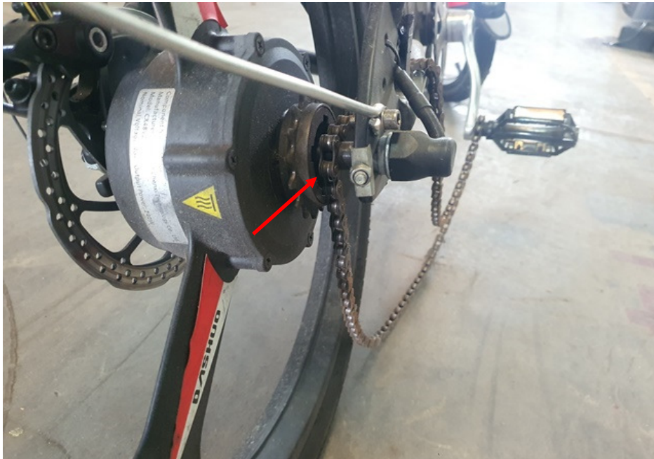
Photo 16 shows a closer view of the dislodged chain from the gear train of the PAB, most likely as a result of the accident (arrowed). It was found to be adequately lubricated for operating purposes.
