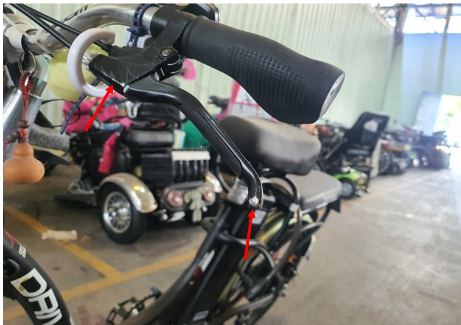
Photo 7 shows the damages on the left hand brake lever (arrowed) of the PAB as a result of the accident.
