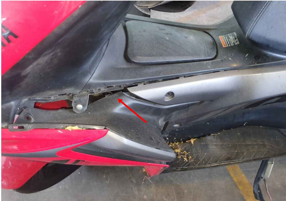
Photo 11 show a closer view of the left inner panel of the Motorcycle which was observed to be damaged due to the accident (arrowed).
