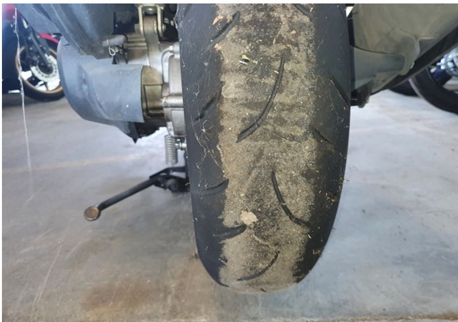
Photo 14 shows the condition of the Motorcycle's rear tyre. The rear tyre was observed to be in serviceable condition with remaining tread depth of approximately 2mm. The tyre was also observed to be sufficiently inflated for vehicular operation. We did not observe any tear, burst mark(s) and/or punctured hole(s) on the sidewalls as well as across the tread of the rear tyre.
