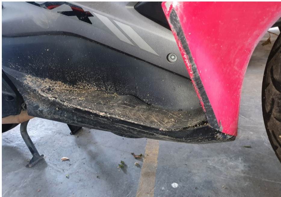
Photo 10 shows a closer view of the right bottom cowling of the Motorcycle which was observed to be damaged due to the accident.
