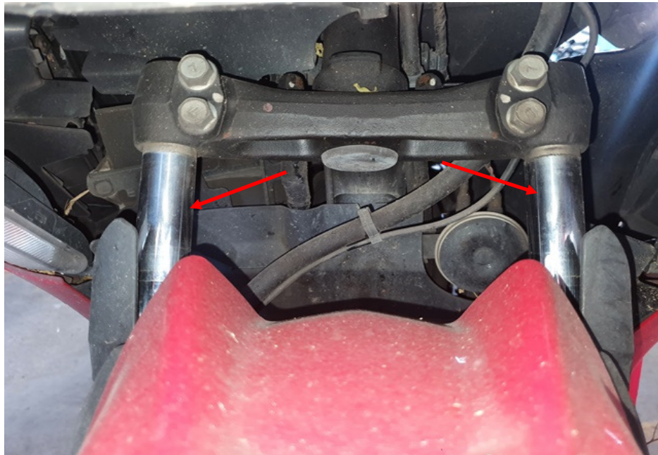
Photo 20 shows the front forks (arrowed) of the Motorcycle. The front forks and fork brackets of the Motorcycle were both found to be intact and undamaged. Turning the Motorcycle's handle bar towards the left and right did not produce any abnormal free play and/or resistance. The steering system of the Motorcycle was in serviceable condition at the time of our inspection.
