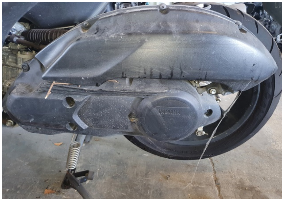
Photo 17 shows the drive train of the Motorcycle which was found to be intact without any misalignment.
