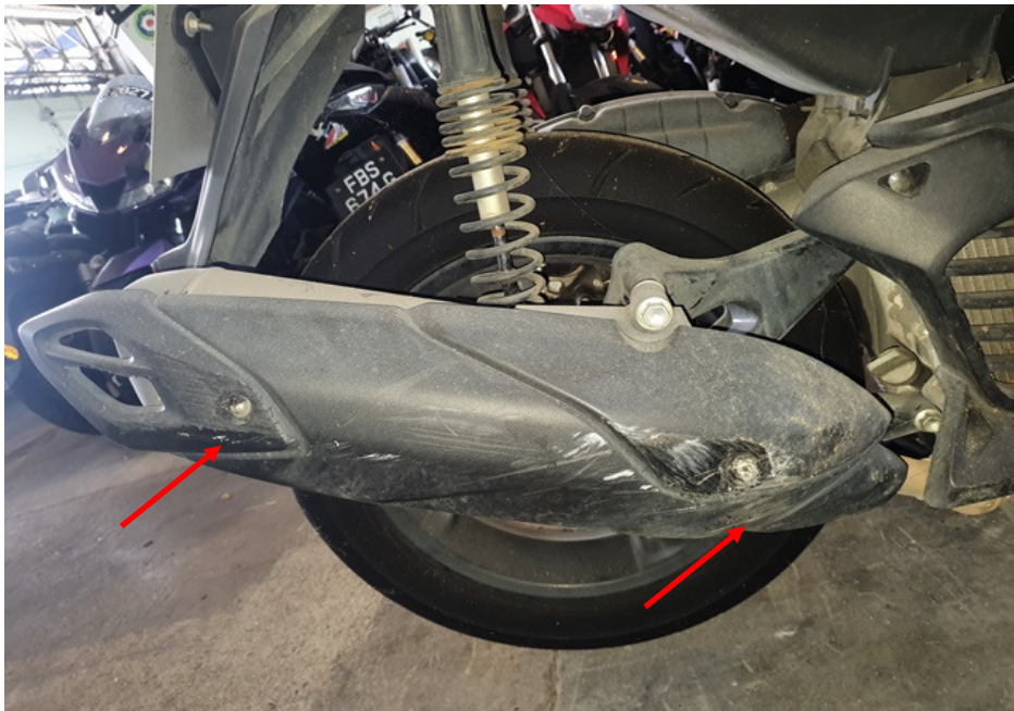
Photo 12 shows a closer view of the grazed exhaust muffler heat shield (arrowed) of the Motorcycle as a result of the accident.
