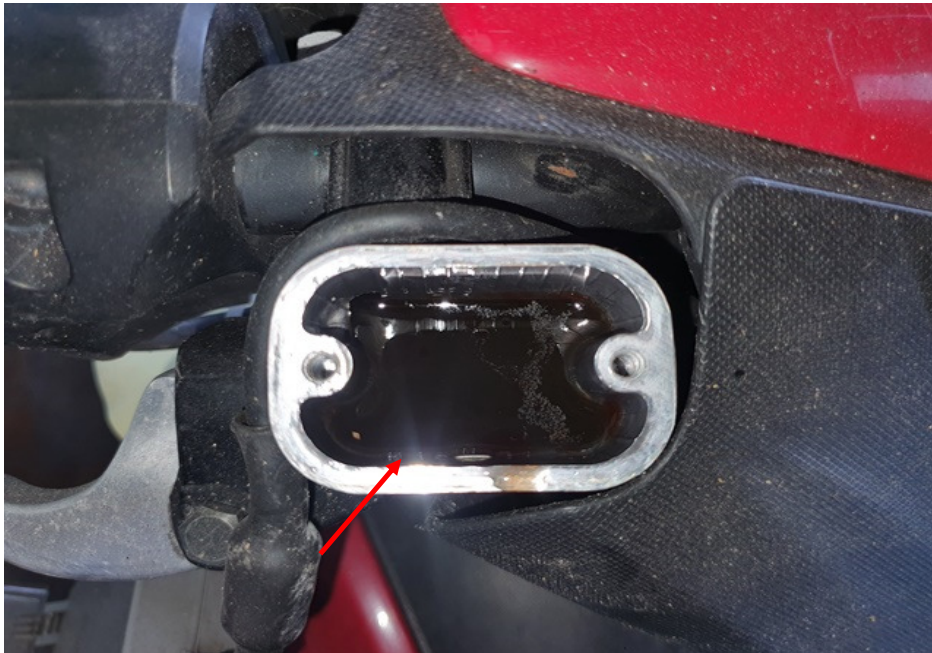
Photo 24 shows a close up view of the brake fluid reservoir for the front brake of the Motorcycle. The brake fluid was observed to be of sufficient level for operational purposes. However it was found to be slightly contaminated (arrowed).
