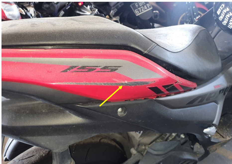
Photo 5 shows a closer view of the grazed right rear side cover (arrowed) of the Motorcycle at the time of our inspection.
