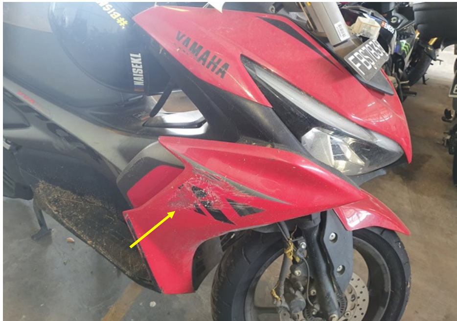
Photo 9 shows a closer view of the grazed right cowling (arrowed) of the Motorcycle as a result of the accident.
