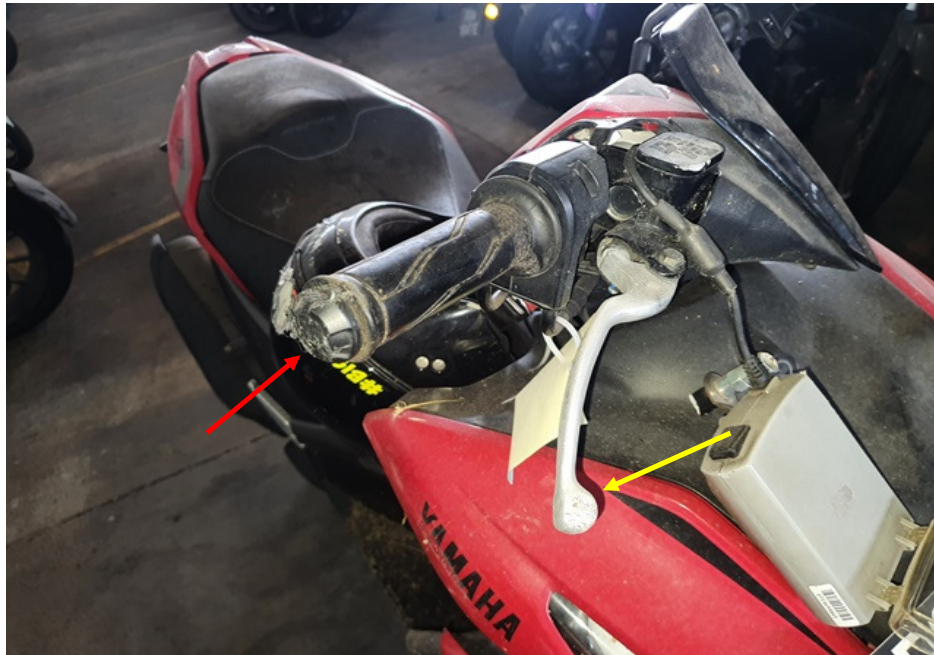
Photo 7 shows a closer view of the grazed front brake lever and right handlebar end (arrowed) of the Motorcycle as a result of the accident.
