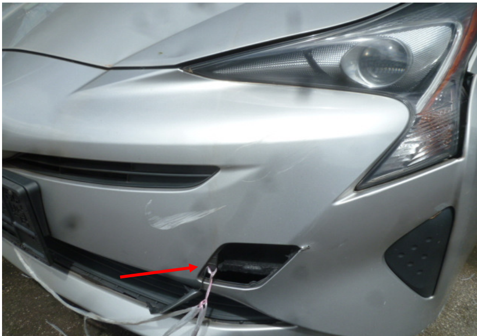
Photo 5 shows a closer view of the missing front left tow cover (arrowed) of the Motor Car at the time of our inspection
