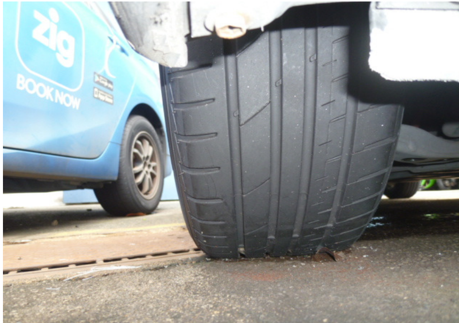
Photo 8 shows the condition of the front right tyre of the Motor Car, which was observed to be in serviceable condition with remaining tread depth of approximately 6mm. The tyre, which was wrapped around alloy wheel rim, was also observed to be sufficiently inflated for vehicular operation.
