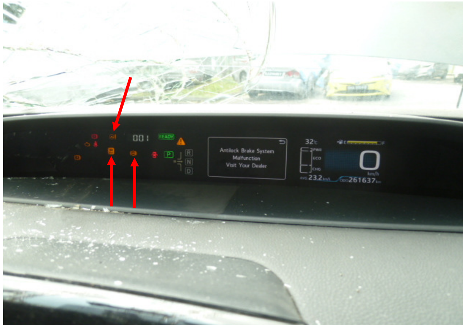
Photo 23 shows no SRS warning light illuminated on the instrument panel of the Motor Car after the engine was cranked. This would suggest that there was no abnormality to the SRS of the Motor Car. The ABS warning light, VSC warning light and EPS warning light had however remained illuminated after the self-test (arrowed).
