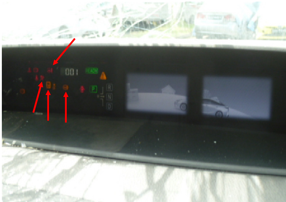
Photo 22 shows the warning lights for the various electronic operating systems of the Motor Car appearing on its instrument panel during the self-test when the engine is cranked, in particular the SRS light, ABS light, EPS light and VSC light (arrowed).
