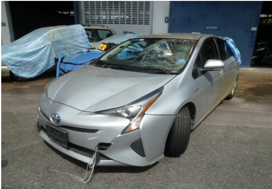
Photo 20 shows the front left wheel of the Motor Car turned to its full left. During our steering system test, we did not experience any abnormal free play and/or resistance when we had turned the steering wheel towards the left and right. This would suggest that the steering system of the Motor Car was likely to be in serviceable condition at the material time of accident.
