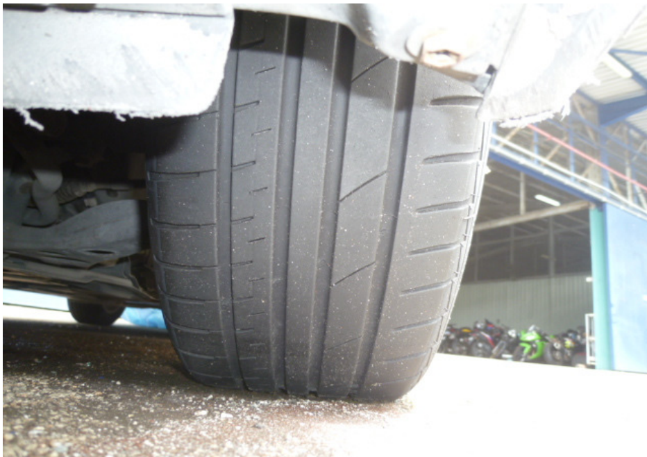
Photo 7 shows the condition of the front left tyre of the Motor Car, which was observed to be in serviceable condition with remaining tread depth of approximately 7mm. The tyre, which was wrapped around alloy wheel rim, was also observed to be sufficiently inflated for vehicular operation. There was no tear, cut or burst mark(s) on the outer and the inner sidewalls as well as across the tread of the 4 tyres.
