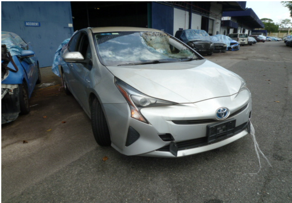
Photo 21 shows the front right wheel of the Motor Car turned to its full right. During our steering system test, we did not experience any abnormal free play and/or resistance when we had turned the steering wheel towards the left and right. This would suggest that the steering system of the Motor Car was likely to be in serviceable condition at the material time of accident.
