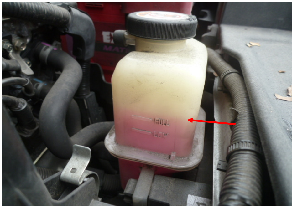
Photo 14 shows the coolant reservoir for the hybrid system of the Motor Car at the time of our inspection. The hybrid system coolant was observed to be of sufficient level for operating purposes and without any visible contamination (arrowed).
