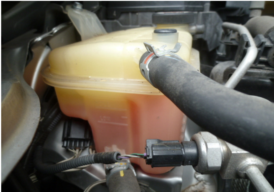
Photo 13 shows checks being carried out to the engine coolant of the Motor Car at the time of our inspection. The engine coolant was observed to be of sufficient level for operating purposes and without any visible contamination.
