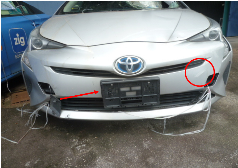
Photo 4 shows a closer view of the cracked front bumper (circled) and missing front number plate (arrowed) of the Motor Car at the time of our inspection
