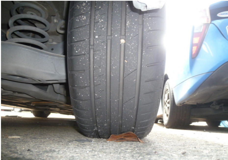
Photo 10 shows the condition of the rear right tyre of the Motor Car, which was observed to be in serviceable condition with remaining tread depth of approximately 8mm. There was also no tear, cut or burst mark(s) on the outer and the inner sidewalls as well as across the tread of the 4 tyres.
