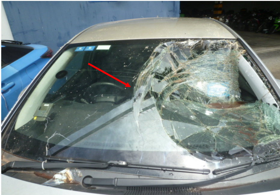
Photo 6 shows a closer view of the shattered front windscreen (arrowed) of the Motor Car at the time of our inspection.
