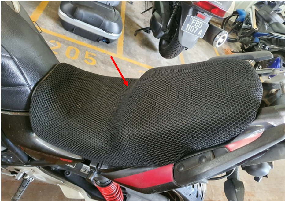
Photo 8 shows the deformed seat of the Motorcycle as a result of the accident (arrowed).
