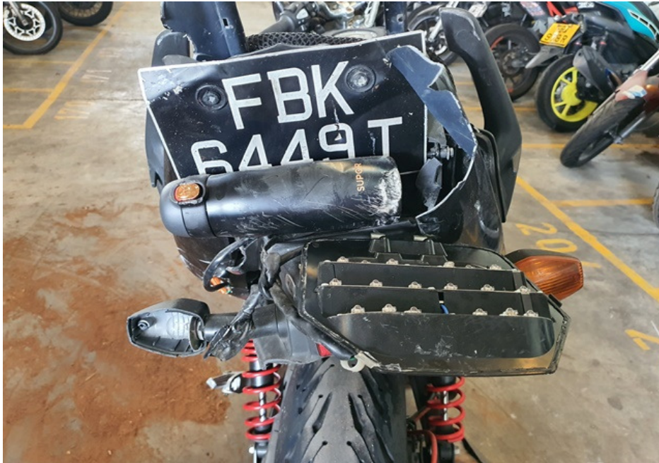
Photo 12 shows a closer view of the broken tail light assembly of the Motorcycle as a result of the accident.
