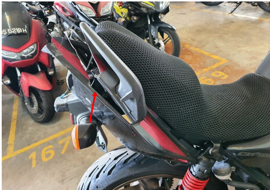
Photo 11 shows the cracked right rear side cover (arrowed) of the Motorcycle as a result of the accident.
