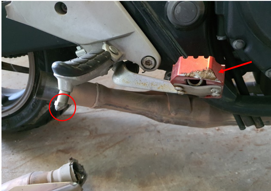
Photo 10 shows a closer view of the right front footrest (circled) and rear brake pedal (arrowed) which were amongst the body parts of the Motorcycle that had sustained damage as a result of the accident.
