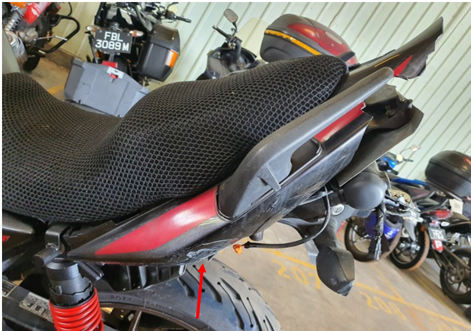
Photo 9 shows the grazed left rear side cover of the Motorcycle as a result of the accident (arrowed).
