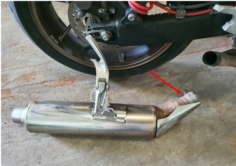
Photo 13 shows a closer view of the dislodged exhaust muffler (arrowed) which was amongst the body parts at the rear body of the Motorcycle that had sustained damage as a result of the accident.
