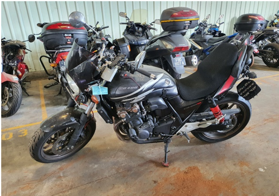
Photo 3 shows a general view of the left body of the Motorcycle at the time of our inspection. The Motorcycle was observed to have sustained damages all around. The body parts that were found to have been damaged include its head cowling, front mudguard, right handlebar end and exhaust muffler, amongst others.
