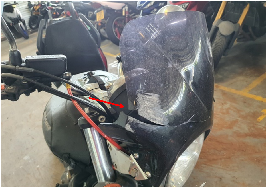
Photo 4 shows a closer view of the cracked head cowling (arrowed) of the Motorcycle as a result of the accident.
