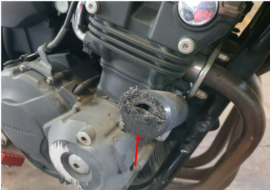
Photo 7 shows the grazed right frame slider of the Motorcycle as a result of the accident (arrowed).
