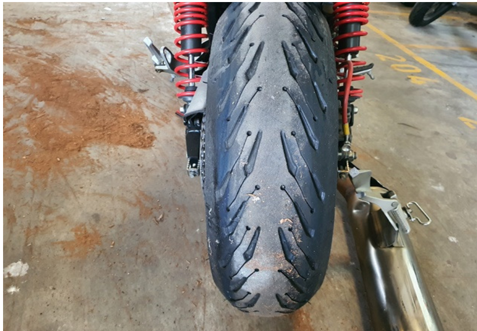
Photo 15 shows the condition of the Motorcycle's rear tyre. The rear tyre was observed to be in serviceable condition with remaining tread depth of approximately 6mm. The tyre was also observed to be sufficiently inflated for vehicular operation. We did not observe any tear, burst mark(s) and/or punctured hole(s) on the sidewalls as well as across the tread of the rear tyre.
