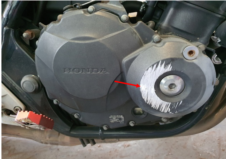
Photo 17 shows the right side of the engine of the Motorcycle at the time of our inspection. The various right engine components had sustained damage of grazing nature as a result of the accident (arrowed) however the engine components were still intact. There was also no fluid leak and/or fluid stain found around the right engine area of the Motorcycle.
