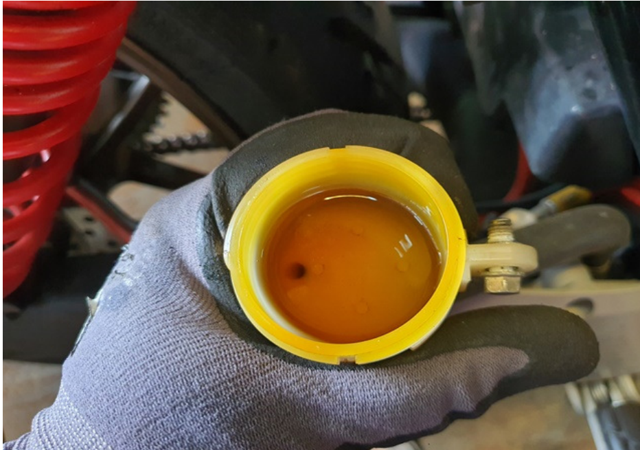
Photo 28 shows the brake fluid reservoir for the rear brake of the Motorcycle. The brake fluid was observed to be of sufficient level for operational purposes and without any contamination.
