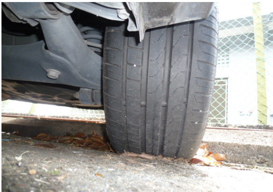
Photo 9 shows the condition of the rear left tyre of the Motor Car, which was observed to be in serviceable condition with remaining tread depth of approximately 8mm. The tyre, which was wrapped around alloy wheel rim, was also observed to be sufficiently inflated for vehicular operation. There was also no damage found on the 4 wheel rims of the Motor Car.
