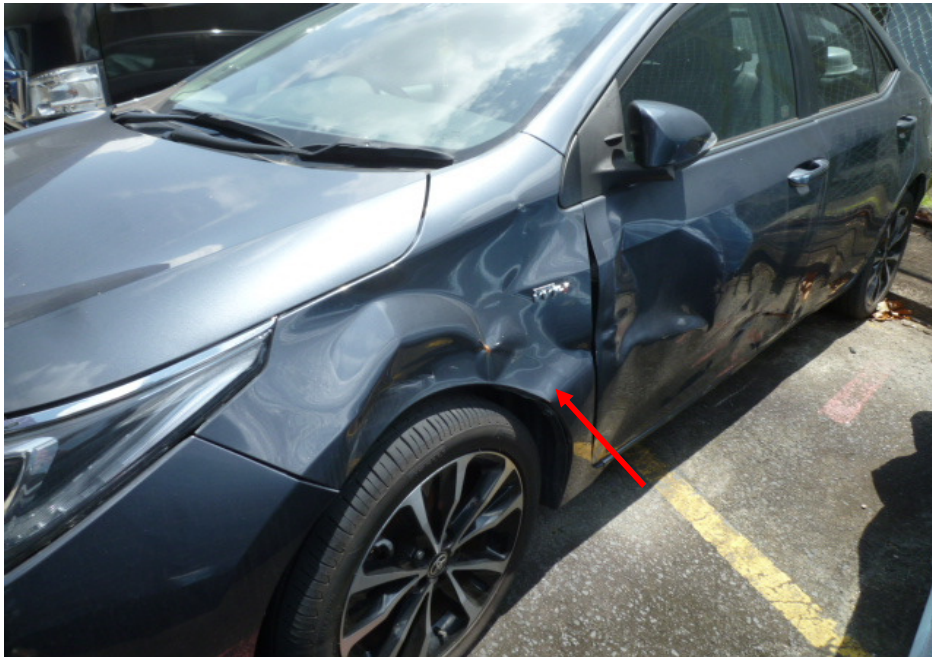
Photo 4 shows a closer view of the dented left front fender of the Motor Car at the time of our inspection (arrowed).
