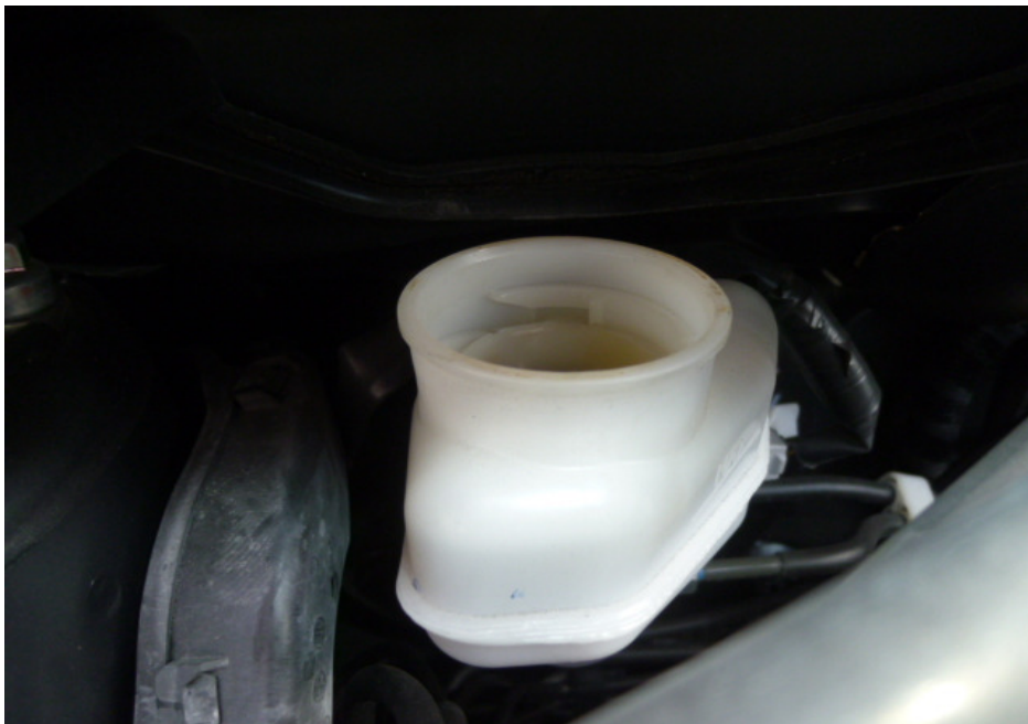
Photo 12 shows the brake fluid reservoir of the Motor Car at the time of our inspection. The brake fluid was observed to be of sufficient level for operating purposes and without any visible contamination.
