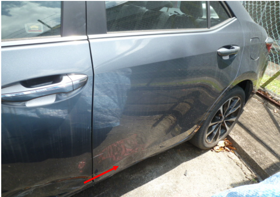
Photo 6 shows a closer view of the dented left rear door of the Motor Car at the time of our inspection (arrowed).
