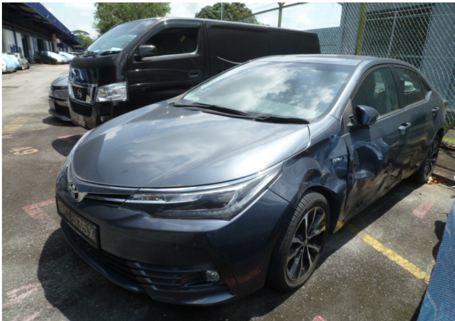
Photo 3 shows a general view of the front left body of the Motor Car at the time of our inspection. The Motor Car was observed to be in good general condition. However we had observed relatively minor impact damage that was confined to its left portion. Its front left fender, left front door and left rear door were observed to have been dented.
