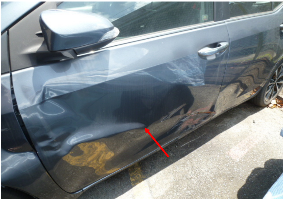
Photo 5 shows a closer view of the dented left front door of the Motor Car at the time of our inspection (arrowed).
