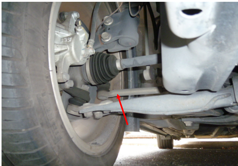
Photo 17 shows the various undercarriage components at the front right wheel of the Motor Car, in particular the steering tie rod (arrowed). The various steering components were all found to be intact, suggesting that the steering system of the Motor Car was likely to be in serviceable condition at the material time of accident. There was also no sign of fluid stain observed on the various undercarriage components at the front right wheel of the Motor Car.
