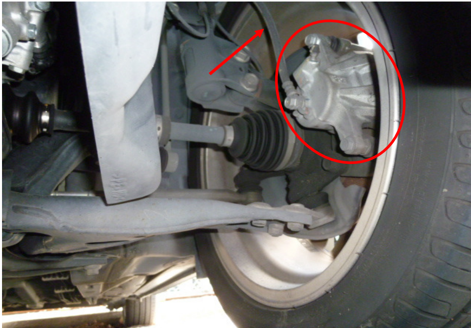
Photo 16 shows the brake hose/pipe (arrowed) at the front left wheel of the Motor Car. No leakage of brake fluid was observed. Visual examination of the various components of the braking system like the brake caliper (circled), brake pedal etc. had revealed all to be intact and without visible damage.
