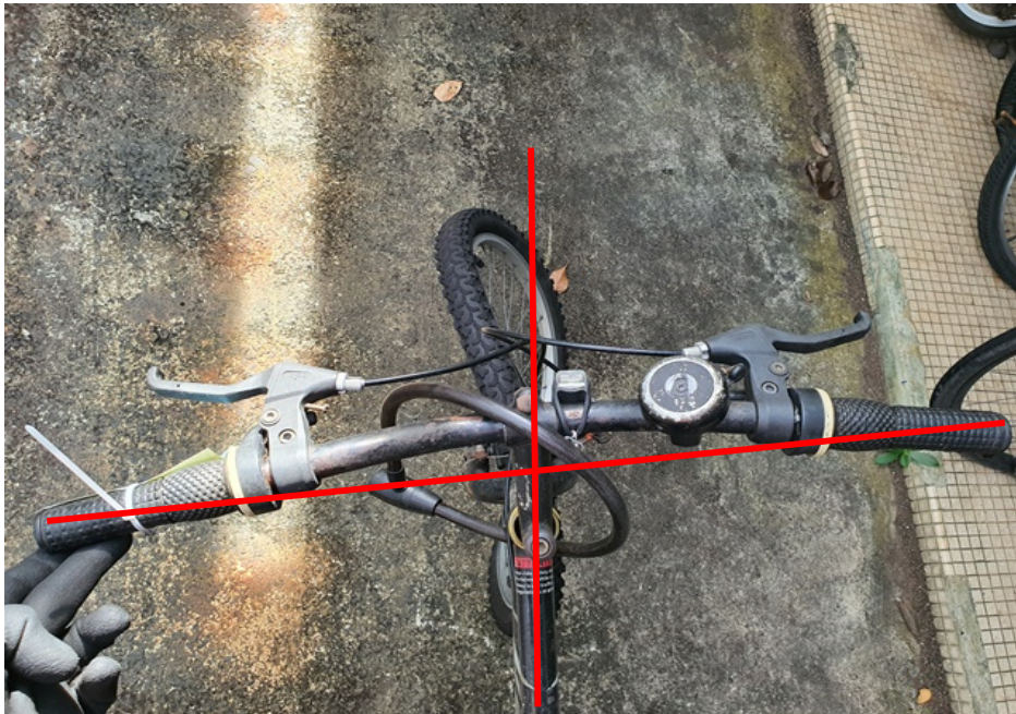
Photo 5 shows the frontal portion of the Bicycle (top view) at the time of our inspection. There was a misalignment of the handle bar & front tyre observed as a result of the accident.
