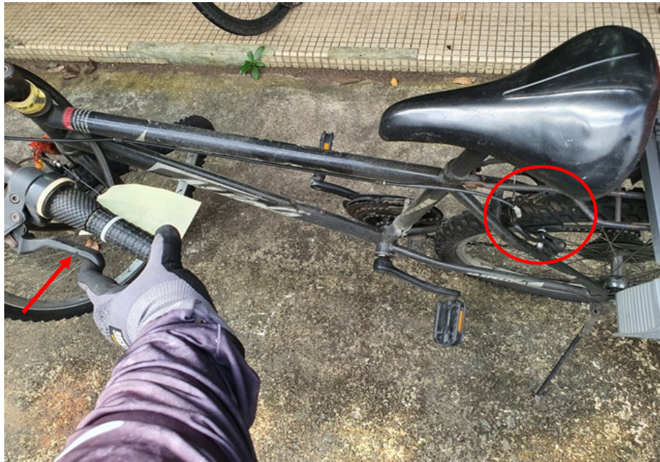
Photo 17 shows a static brake test conducted on the Bicycle's rear brake. There was some resistance felt upon pressing the left hand brake lever (arrowed). It also shows that the rear brake clamps responded to the gripping action (circled) after depressing the left hand brake lever.
