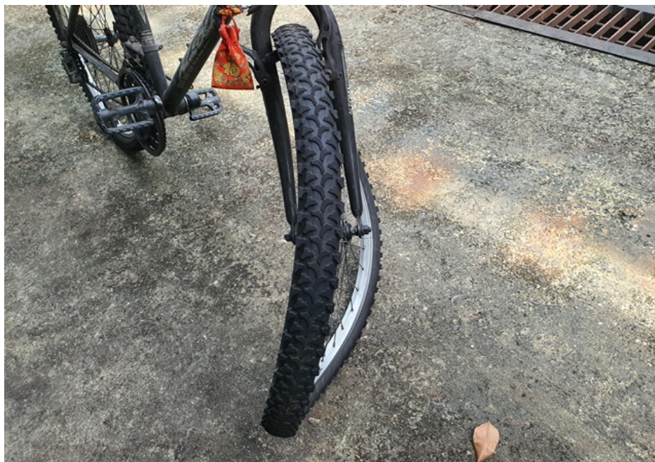
Photo 9 shows the front tyre of the Bicycle. The pattern of the tread was clearly visible. There was no tear, burst mark(s) and/or punctured hole(s) on the sidewalls as well as across the tread of the front tyre. However the front tyre was observed to be deflated at the time of our inspection.
