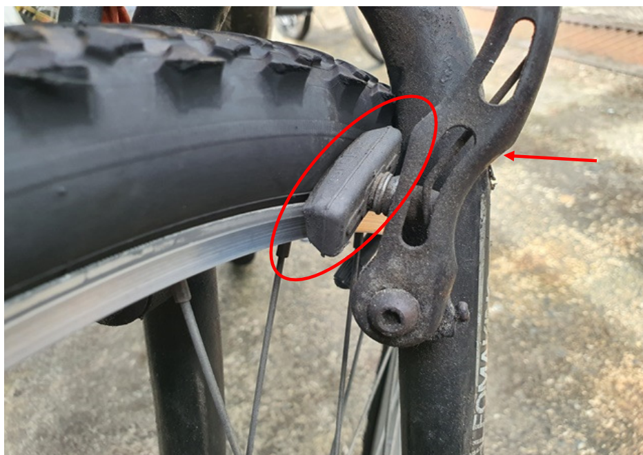
Photo 16 shows a close up view of the front brake clamp assembly of the Bicycle. There was some resistance felt upon pressing the right hand brake lever. However the front brake clamp had not responded to the gripping action. Upon closer examination, we observed that the front brake clamp assembly was misaligned as a result of the accident (circled). Hence the rubber brake blocks had pressed against the front tyre instead of the front wheel rim (arrowed). This had appeared to indicate that the front brake of the Bicycle was not in serviceable condition.
