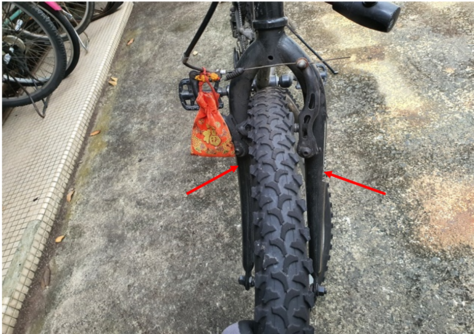
Photo 14 shows the front forks (arrowed) of the Bicycle. The front forks of the Bicycle were found to be bent as a result of the accident, hence causing the whole steering system to be out of alignment and rendering the Bicycle immobile for any static or operational tests.
