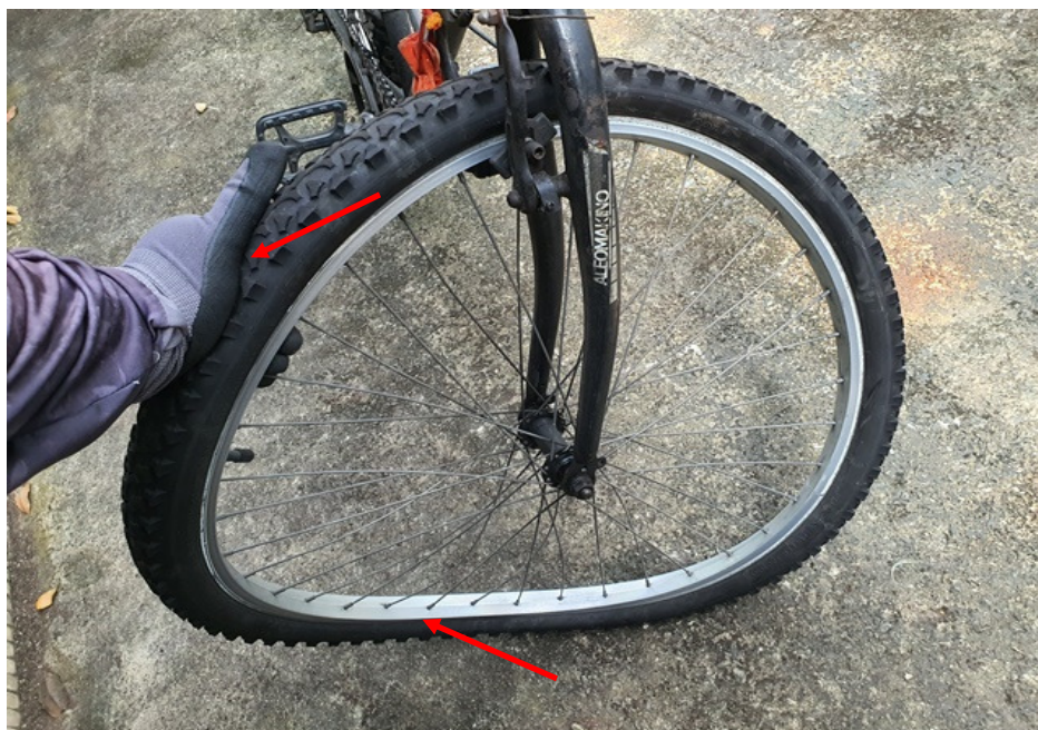
Photo 10 shows the deflated front tyre and bent front wheel rim of the Bicycle (arrowed).
