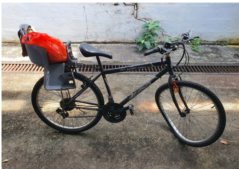
Photo 4 shows the right body of the Bicycle at time of our inspection. The Bicycle had sustained damages at its right body. The body parts that were found to have been damaged include its front brake clamp assembly, right handlebar grip, right pedal and baby seat, amongst others as a result of the accident.
