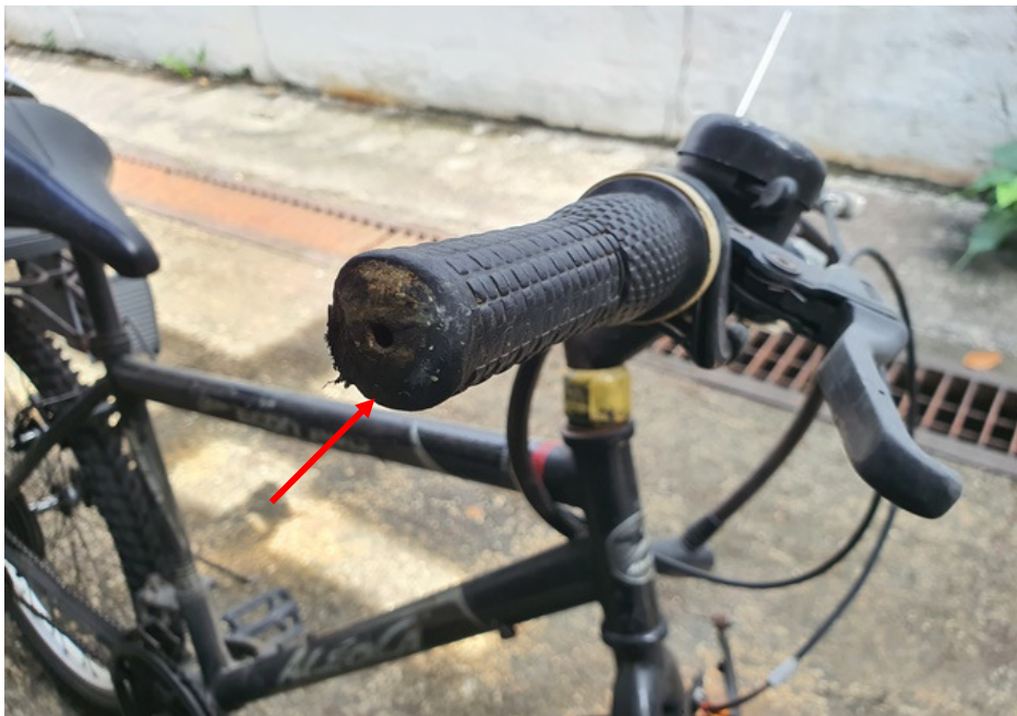
Photo 6 shows the damaged right handlebar grip (arrowed) of the Bicycle at the time of our inspection.
