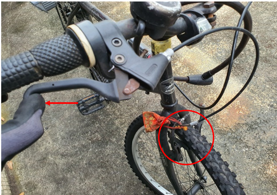
Photo 15 shows a static brake test conducted on the Bicycle's front brake. There was some resistance felt upon pressing the right hand brake lever (arrowed). However the front brake clamps had not responded to the gripping action (circled) after depressing the right hand brake lever.
