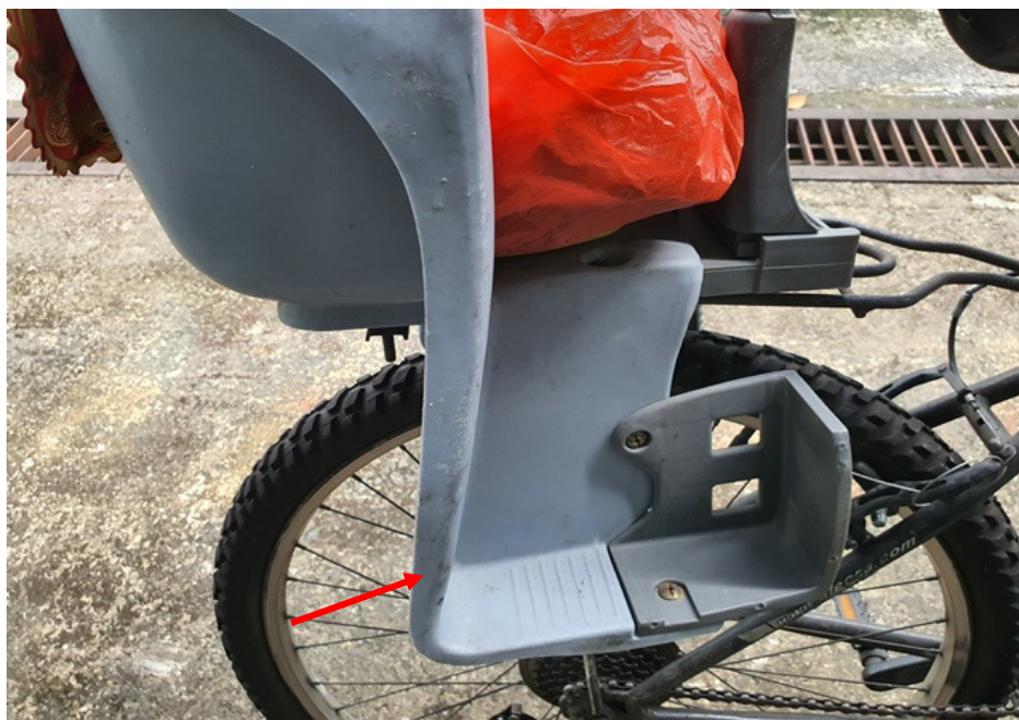
Photo 8 shows a close-up view of the damaged baby seat (arrowed) of the Bicycle as a result of the accident.
