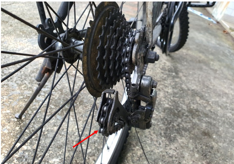
Photo 13 shows a closer view of the gear train of the Bicycle, which was observed to be intact with no misalignment (arrowed). It was also adequately lubricated for operating purposes.
