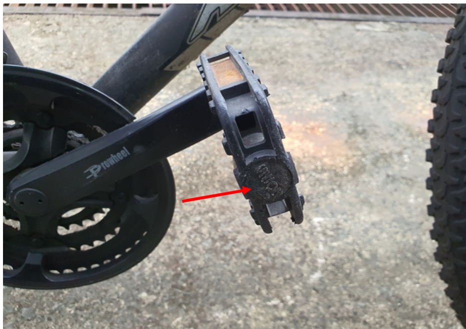
Photo 7 shows the damages of grazing nature on the right pedal of the Bicycle at the time of our inspection (arrowed).
