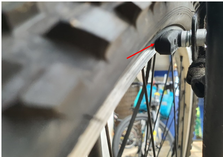
Photo 18 shows a close up view of the rear brake clamps responding to the gripping action. The rubber brake blocks pressed against the rear wheel rim upon depressing the left hand brake lever (arrowed). This had appeared to indicate that the rear brake of the Bicycle was in serviceable condition.
