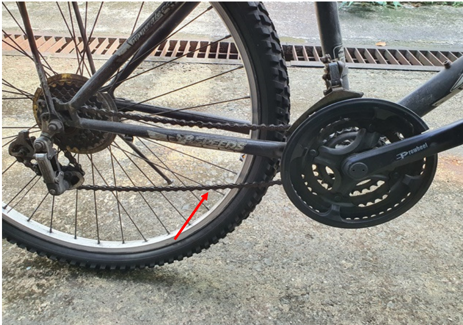
Photo 12 shows the general view of the gear train of the Bicycle, which was observed to be intact with no misalignment. It was also adequately lubricated for operating purposes. However the chain was observed to be dislodged from the gear train most likely as a result of the accident (arrowed).
