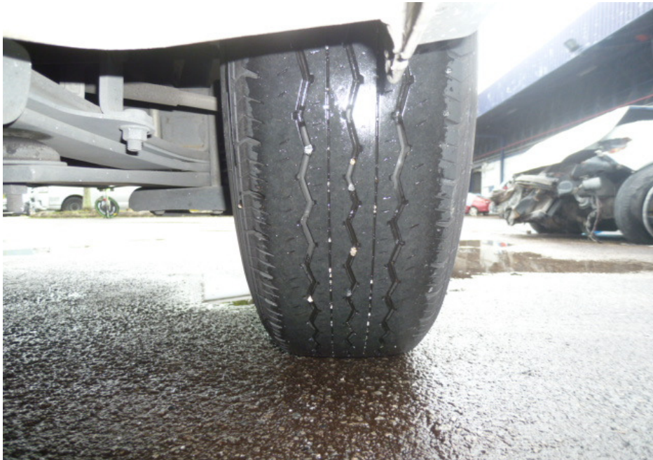
Photo 6 shows the condition of the rear left tyre of the Motor Van, which was observed to be in serviceable condition with remaining tread depth of approximately 7mm. The tyre, which was wrapped around standard steel wheel rim, was also observed to be sufficiently inflated for vehicular operation. There was also no damage found on the 4 wheel rims of the Motor Van.
