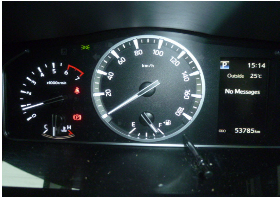
Photo 20 shows no warning lights illuminated on the instrument panel of the Motor Van after the engine was cranked. This would suggest that there was no abnormality to the various electronic operating systems of the Motor Van, like the VSC, SRS and ABS.
