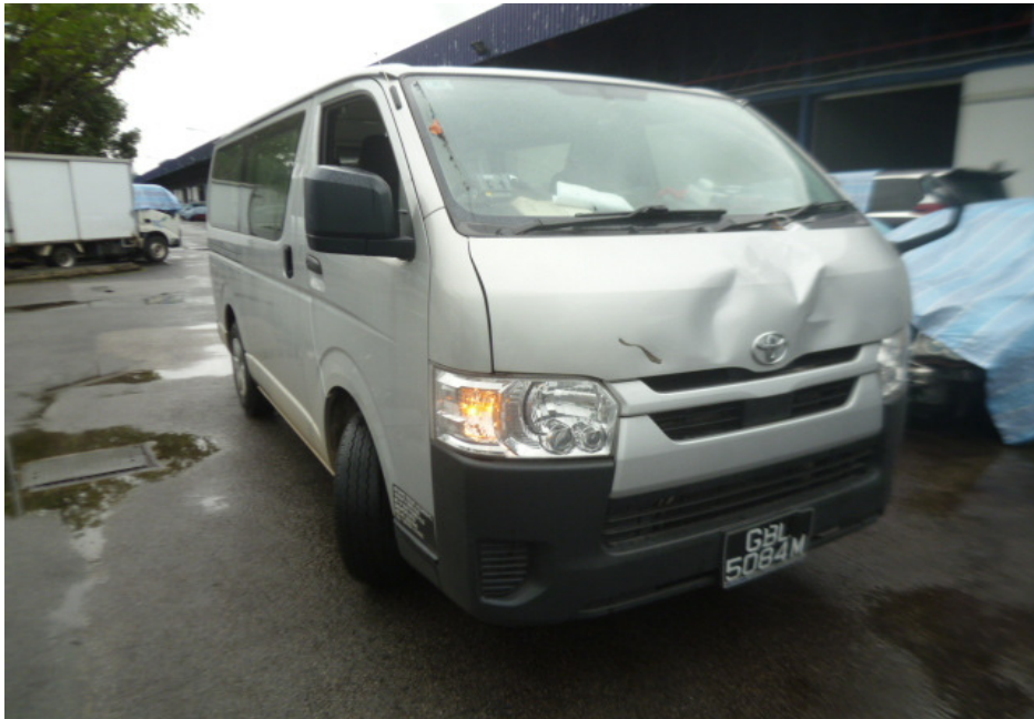
Photo 15 shows the front right wheel of the Motor Van turned to its full right. During our steering system test, we did not experience any abnormal free play and/or resistance when we had turned the steering wheel towards the left and right. This would suggest that the steering system of the Motor Van was likely to be in serviceable condition at the material time of accident.
