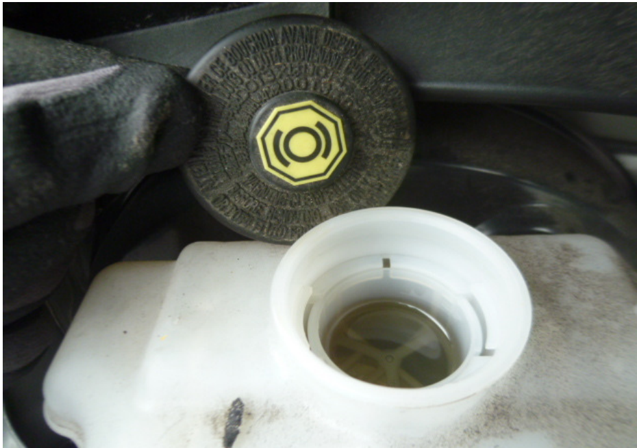
Photo 9 shows the brake fluid reservoir of the Motor Van at the time of our inspection. The brake fluid was observed to be of sufficient level for operating purposes and without any visible contamination.
