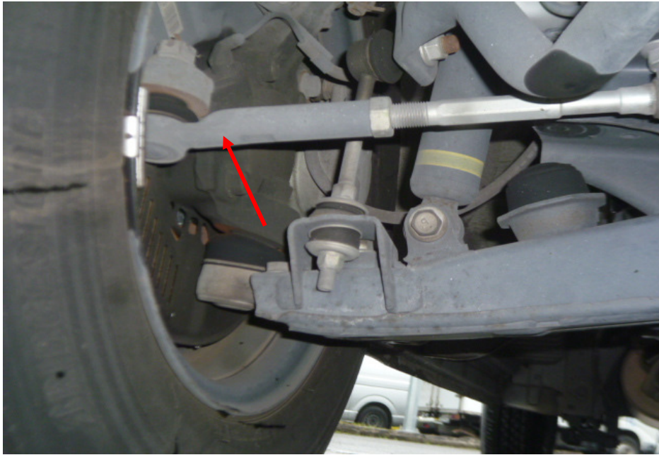
Photo 17 shows the various undercarriage components at the front right wheel of the Motor Van, in particular the steering tie rod (arrowed). The various steering components were all found to be intact, suggesting that the steering system of the Motor Van was likely to be in serviceable condition at the material time of accident. There was also no sign of fluid stain(s) observed on the various undercarriage components.
