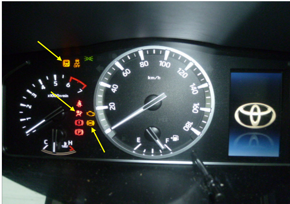
Photo 19 shows the warning lights for the various electronic operating systems of the Motor Van appearing on its instrument panel during the self-test when the engine is cranked, in particular the Vehicle Stability Control (VSC) light, Supplemental Restraint System (SRS) light and Antilock Braking System (ABS) light (arrowed).
