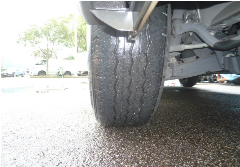
Photo 5 shows the condition of the front right tyre of the Motor Van, which was observed to be in serviceable condition with remaining tread depth of approximately 6mm. The tyre, which was wrapped around standard steel wheel rim, was also observed to be sufficiently inflated for vehicular operation.
