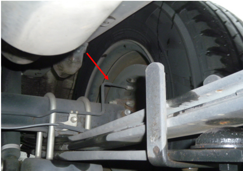
Photo 14 shows the brake pipe (arrowed) at the rear right wheel of the Motor Van. We did not observe any leakage of brake fluid at the time of our inspection of the Motor Van. Our static tests of the Motor Van's braking system had indicated that there was no internal leakage of pressure/vacuum. Hence the braking system was likely to be in serviceable condition at the material time of accident.
