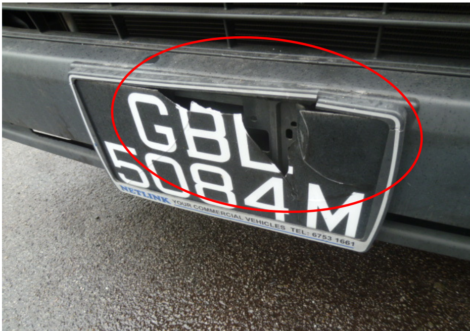
Photo 3 shows a close up view of the cracked front number plate and front number plate holder of the Motor Van at the time of our inspection (circled).
