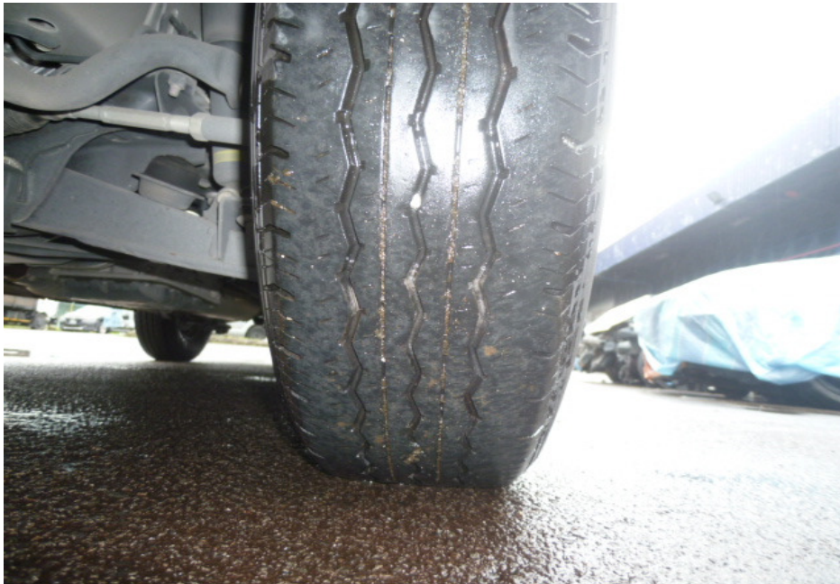
Photo 4 shows the condition of the front left tyre of the Motor Van, which was observed to be in serviceable condition with remaining tread depth of approximately 5mm. The tyre, which was wrapped around standard steel wheel rim, was also observed to be sufficiently inflated for vehicular operation. There was no tear, cut or burst mark(s) on the outer and the inner sidewalls as well as across the tread of the 4 tyres.
