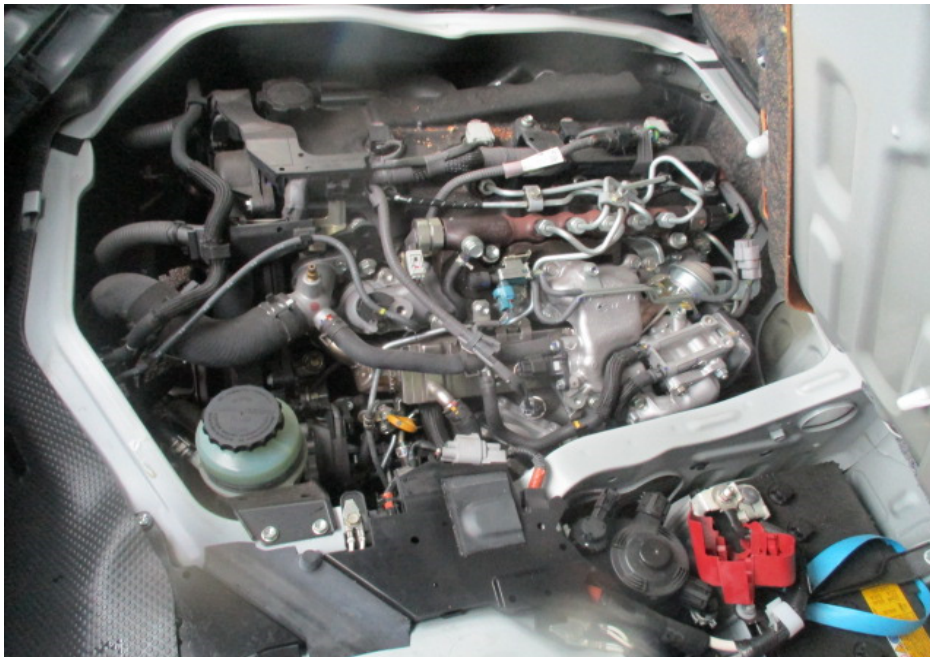
Photo 8 shows a general view of the Motor Van's engine compartment. The various parts and components inside the engine compartment were unaffected by the accident. There was also no sign(s) or indication(s) of fluid leakage and/or fluid stain within the engine compartment. The wirings and cables were all observed to be intact and adequately secured to their respective connectors and/or connecting ports.
