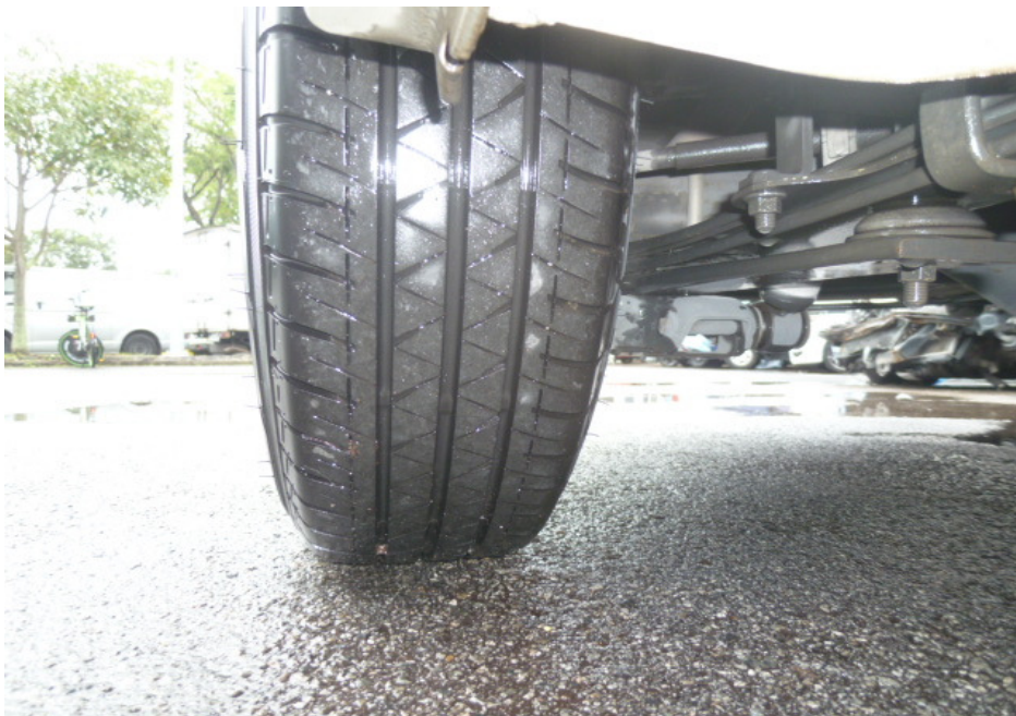
Photo 7 shows the condition of the rear right tyre of the Motor Van, which was observed to be in serviceable condition with remaining tread depth of approximately 7.5mm. There was also no tear, cut or burst mark(s) on the outer and the inner sidewalls as well as across the tread of the 4 tyres.
