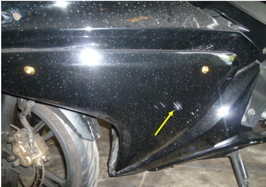
Photo 8 shows a closer view of the left cowling of the Motorcycle that had sustained damages of grazing nature as a result of the accident (arrowed).
