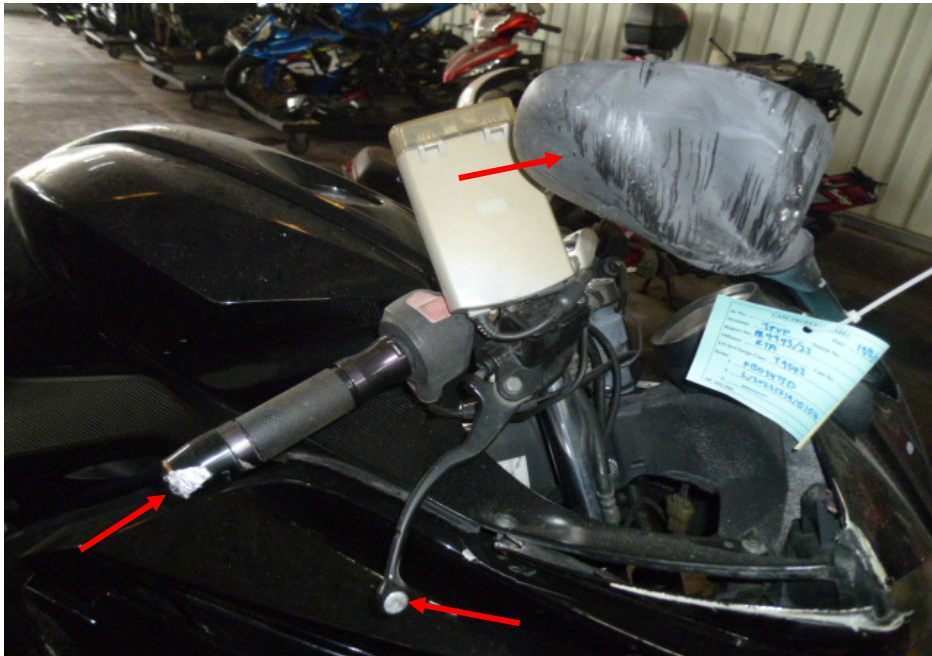
Photo 7 shows a closer view of right handlebar end, right side mirror and front brake lever (arrowed) which were amongst the body parts at the front body of the Motorcycle that had sustained damage as a result of the accident.
