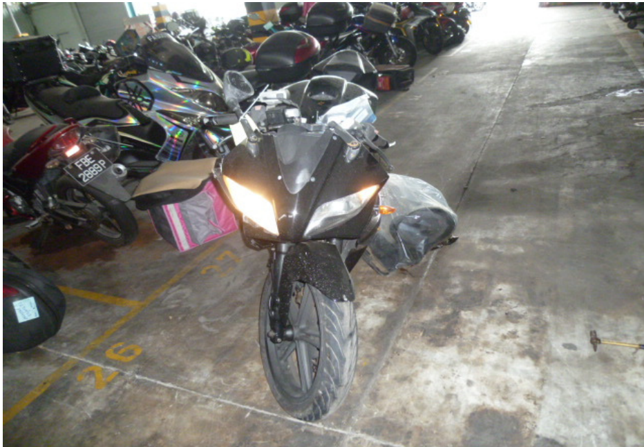
Photo 23 shows the front wheel of the Motorcycle turned towards its full left. Turning the Motorcycle's handle bar towards the left and right did not produce any abnormal free play and/or resistance. This would indicate that the steering system of the Motorcycle was in serviceable condition at the time of our inspection.
