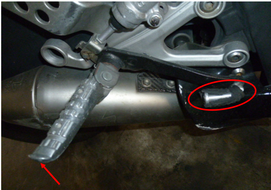
Photo 11 shows a closer view of the rear brake pedal (circled) and right front footrest (arrowed) which were amongst the body parts of the Motorcycle that had sustained damage as a result of the accident
