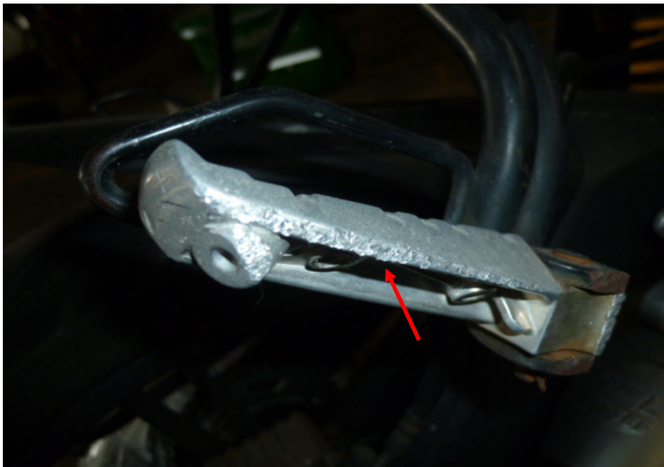
Photo 13 shows a closer view of the grazed right pillion foot peg of the Motorcycle as a result of the accident (arrowed).
