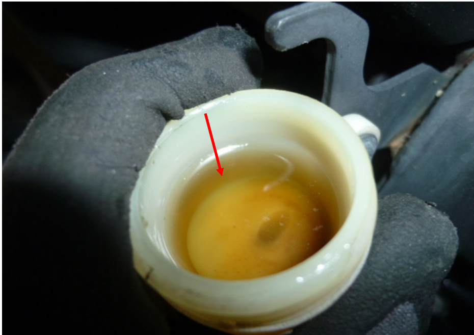
Photo 29 shows a close up view of the brake fluid reservoir for the rear brake of the Motorcycle. The brake fluid for the rear brake was observed to be of sufficient level for operational purposes. However it was found to be slightly contaminated (arrowed).
