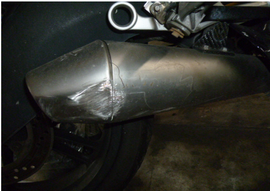
Photo 15 shows a closer view of the dented exhaust muffler of the Motorcycle as a result of the accident.
