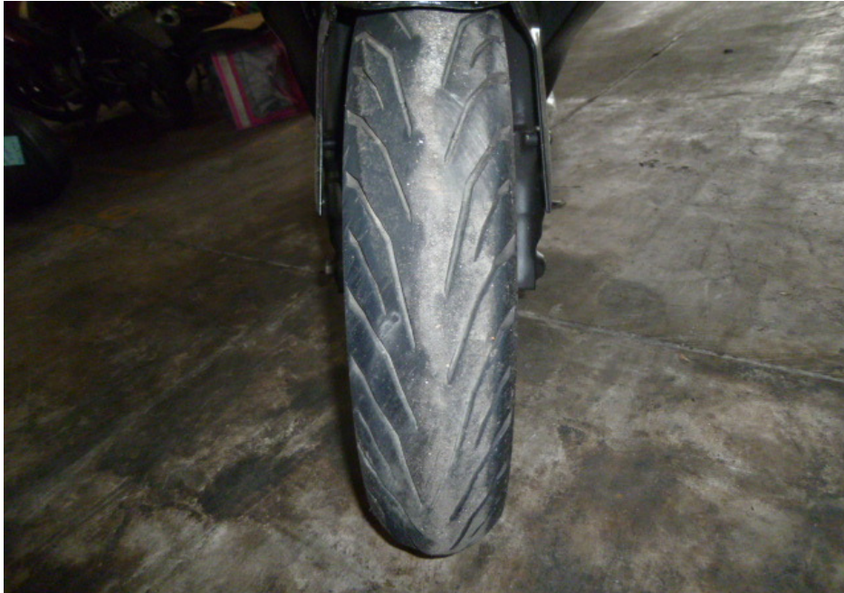
Photo 16 shows the condition of the Motorcycle's front tyre. The front tyre was observed to be in serviceable condition with remaining tread depth of approximately 4mm. There was no tear, burst mark(s) and/or punctured hole(s) on the sidewalls as well as across the tread of the front tyre.
