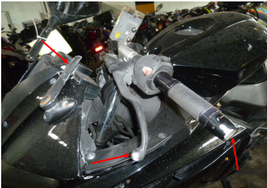
Photo 9 shows a closer view of the left handlebar end, left side mirror and clutch lever (arrowed) which were amongst the body parts of the Motorcycle that had sustained damage as a result of the accident.
