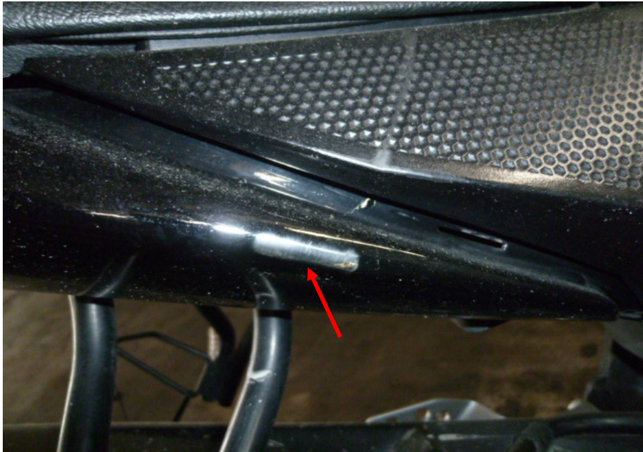
Photo 12 shows the grazed right rear side cover of the Motorcycle as a result of the accident.
