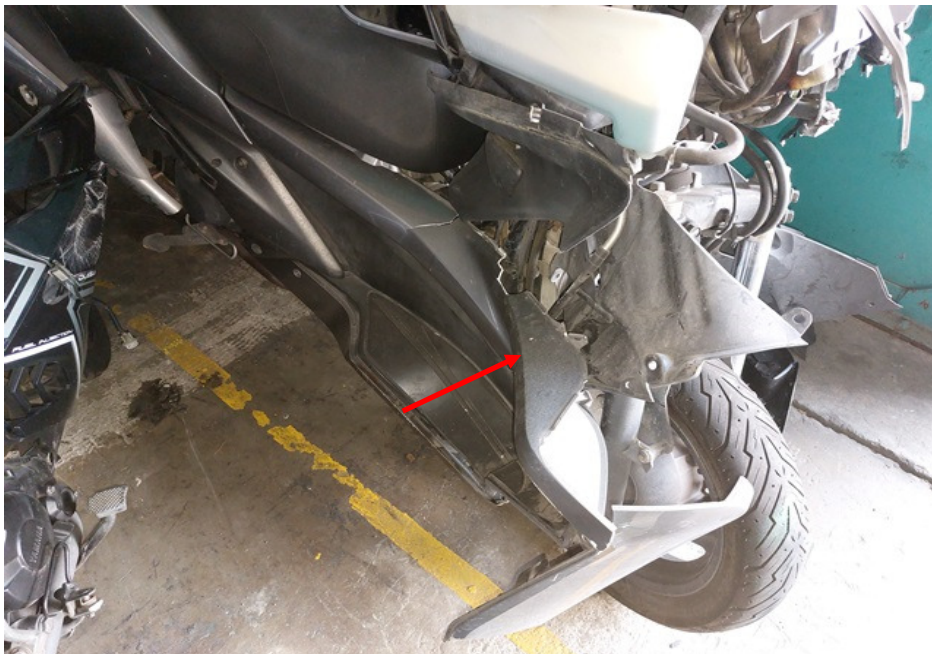
Photo 10 shows the cracked right side cowling of the Motorcycle as a result of the accident (arrowed).
