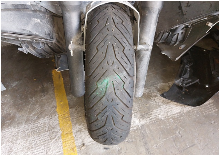
Photo 16 shows the condition of the Motorcycle's front tyre. The front tyre was observed to be in serviceable condition with remaining tread depth of approximately 4mm. There was no tear, burst mark(s) and/or punctured hole(s) on the sidewalls as well as across the tread of the front tyre. The tyre was also observed to be sufficiently inflated for vehicular operation.
