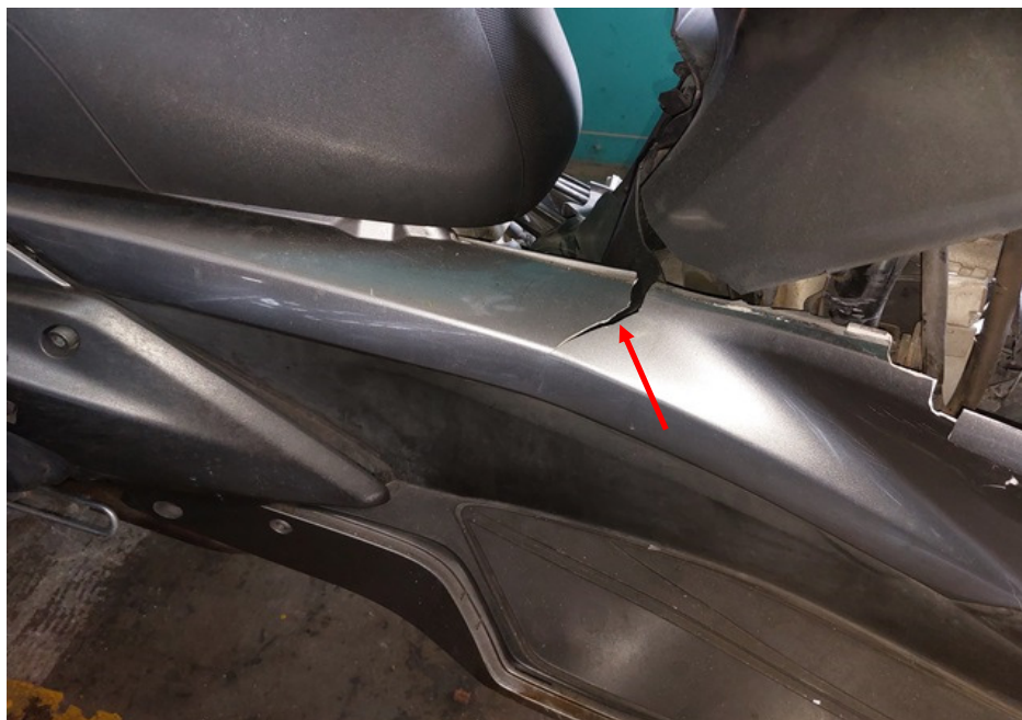
Photo 13 shows a general view of the cracked right centre cover of the Motorcycle as a result of the accident (arrowed).
