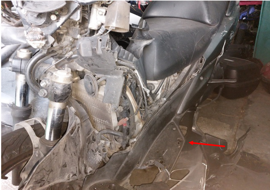
Photo 9 shows the cracked left side cowling of the Motorcycle as a result of the accident (arrowed).
