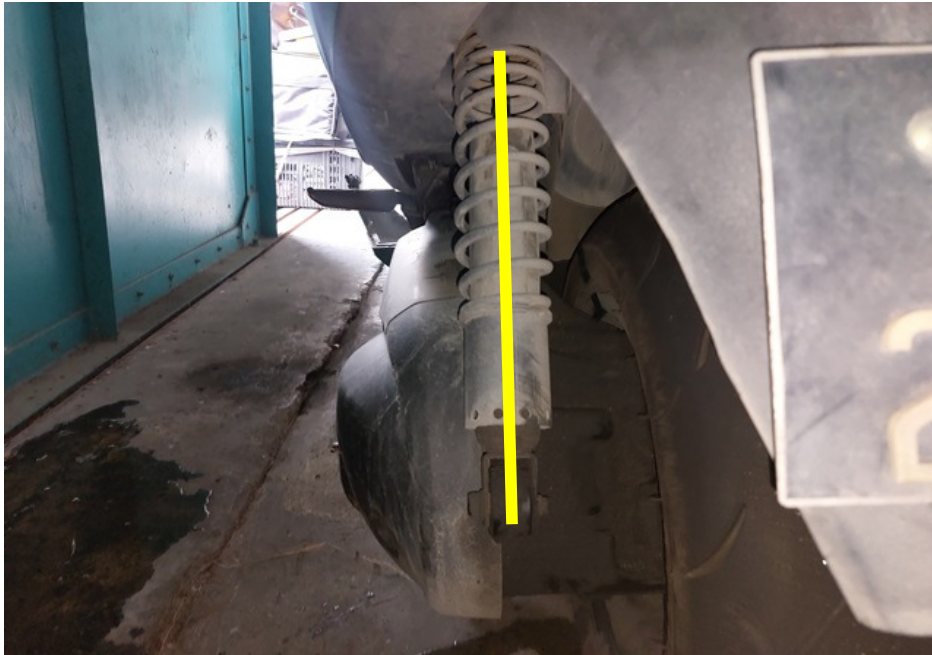
Photo 20 shows the left shock absorber of the Motorcycle which was found to be intact without any misalignment.
