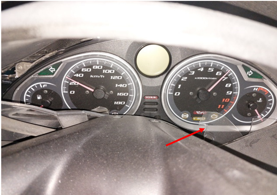
Photo 1 shows the speedometer of the Motorcycle. The mileage of the Motorcycle could not be recorded at the time of our inspection due to damages sustained to the speedometer gauge (arrowed).
