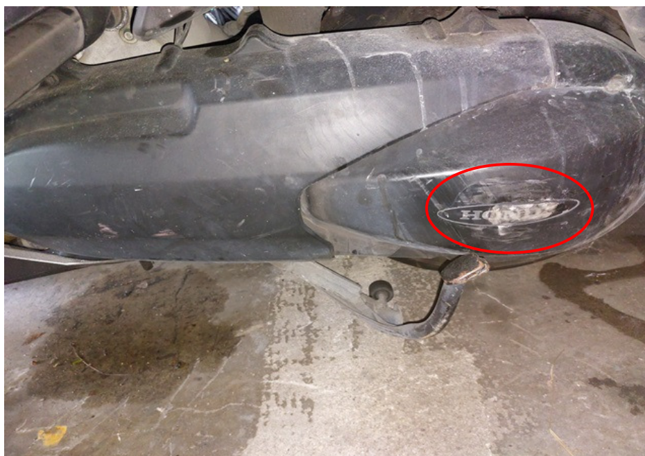
Photo 19 shows the drive train of the Motorcycle which was found to be intact without any misalignment. However the drive train cover had sustained damages of grazing nature as a result of the accident (circled).
