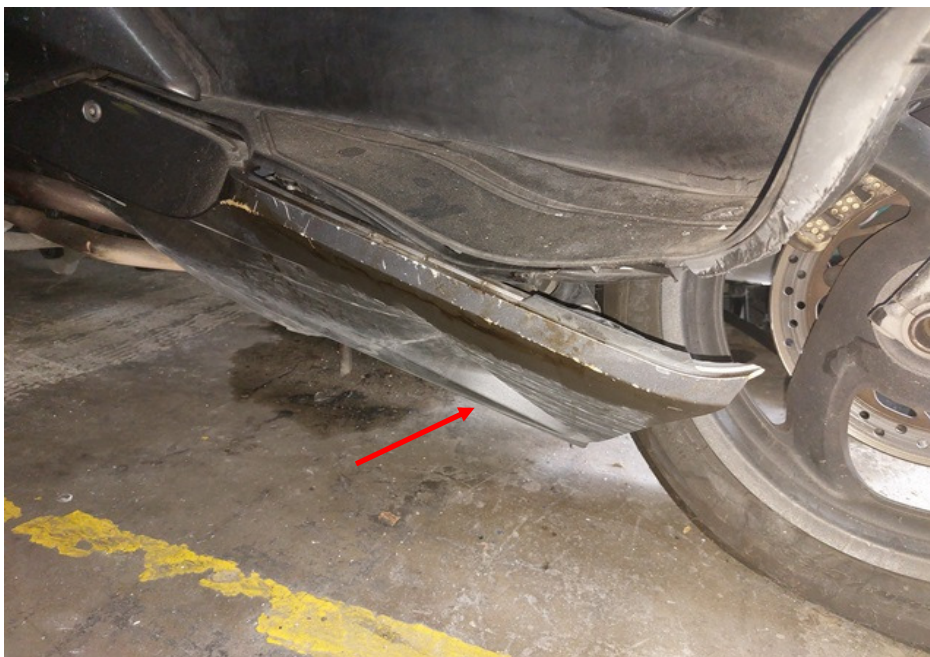
Photo 11 shows a close-up view of the cracked right lower side cowling of the Motorcycle as a result of the accident.
