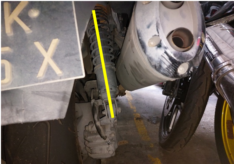
Photo 21 shows the right shock absorber of the Motorcycle which was found to be intact without any misalignment.
