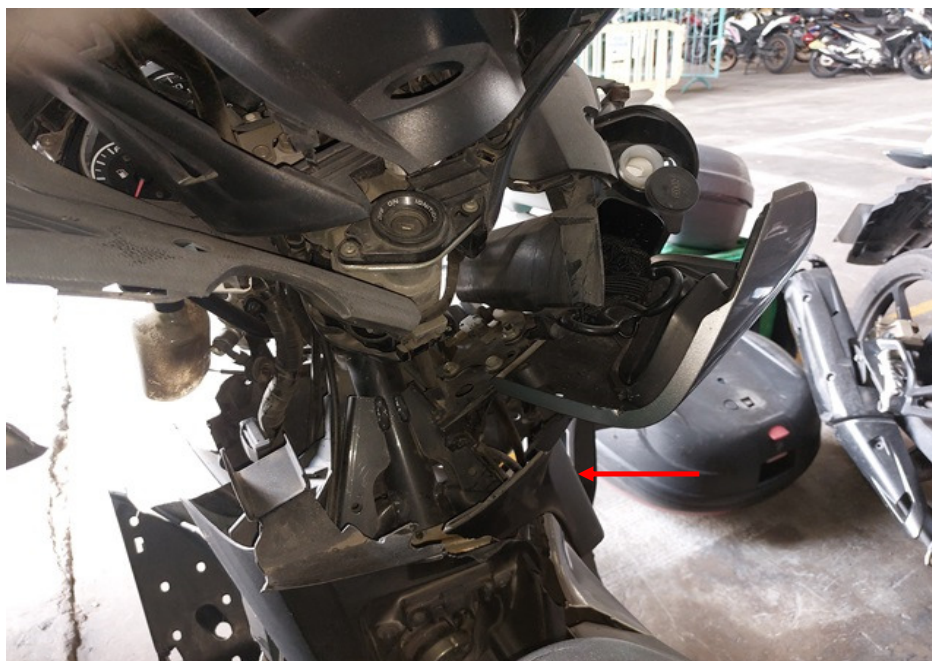
Photo 6 shows a closer view of the cracked inner centre cowling of the Motorcycle as a result of the accident (arrowed).
