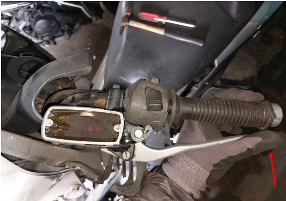
Photo 27 shows the rear brake lever being depressed. There was some resistance felt (spongy like feel) upon pressing the front brake lever (arrowed). This would indicate that there is no leakage of pressure/vacuum in the rear brake system.
