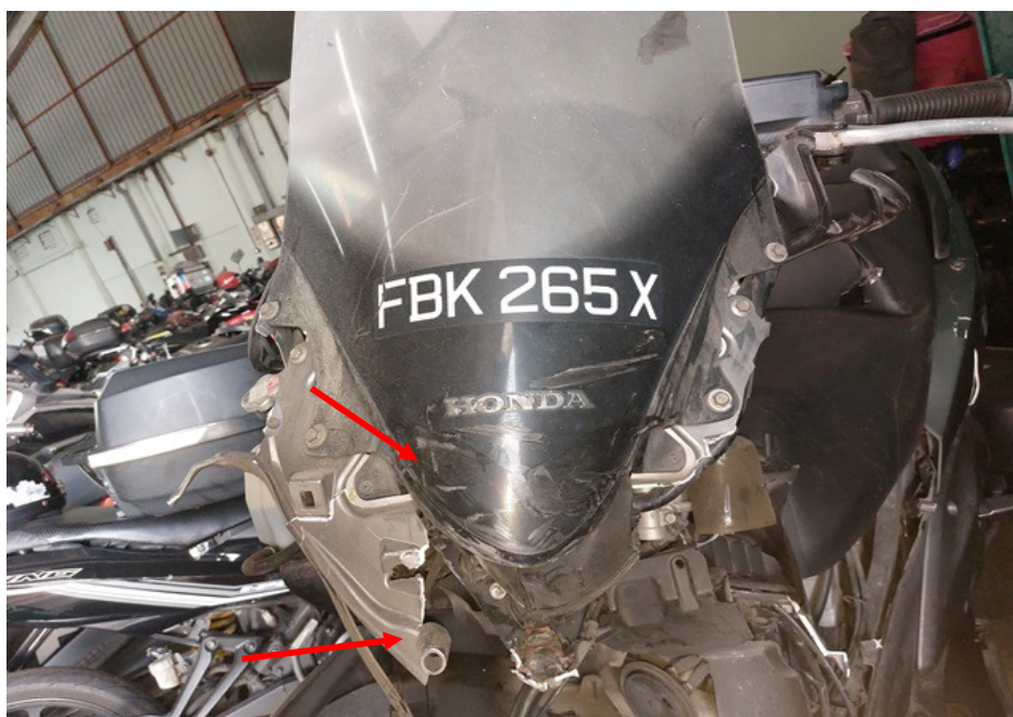
Photo 5 shows a closer view of the cracked windshield and head cowling of the Motorcycle at the time of our inspection (arrowed).
