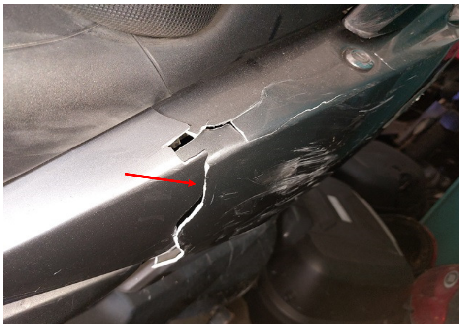
Photo 14 shows a close-up view of the cracked left rear side cover of the Motorcycle as a result of the accident (arrowed).
