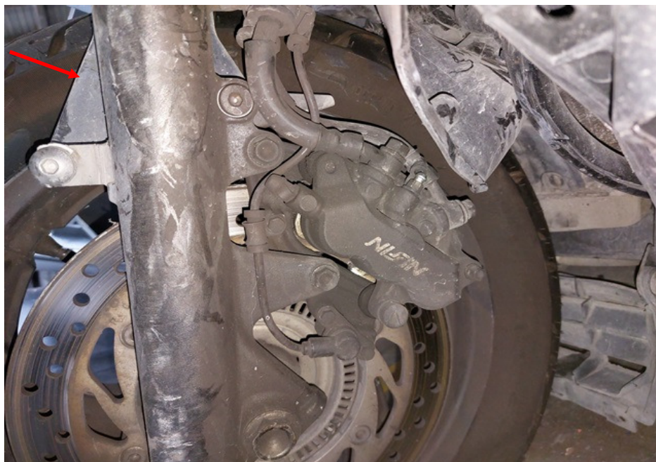
Photo 7 shows a closer view of the cracked front mudguard of the Motorcycle as a result of the accident (arrowed).
