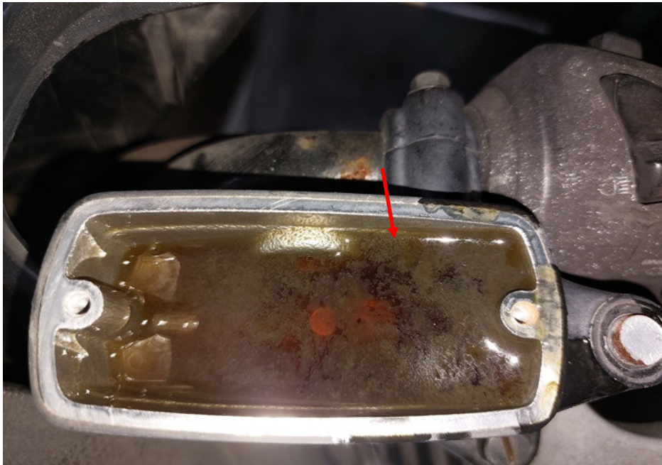
Photo 26 shows the brake fluid reservoir for the rear brake of the Motorcycle. The brake fluid was observed to be of sufficient level for operational purposes. However it was found to be contaminated (arrowed).
