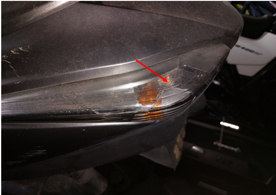
Photo 15 shows a close-up view of the cracked left rear signal lamp of the Motorcycle as a result of the accident (arrowed).
