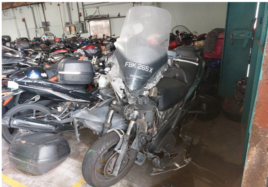
Photo 4 shows a general view of the left frontal portion of the Motorcycle at the time of our inspection. The Motorcycle was observed to have sustained damages all around. The body parts that were found to have been damaged include its windshield, head cowl, front mudguard, steering stem, right side mirror, side cowlings, inner centre cowl, lower side cowlings, right centre side cover, left rear side cover and left rear signal lamp, amongst others as a result of the accident.
