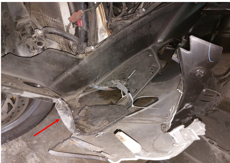
Photo 12 shows a close-up view of the cracked left lower side cowling of the Motorcycle as a result of the accident (arrowed).
