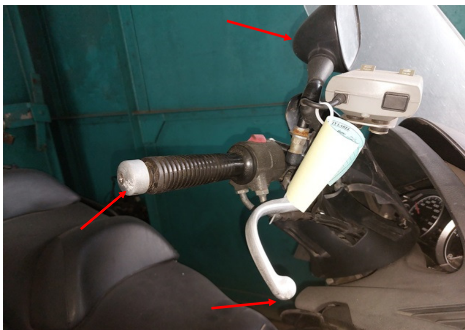
Photo 8 shows a closer view of the right side mirror, right handlebar end and front brake lever of the Motorcycle which were observed to be damaged due to the accident (arrowed).
