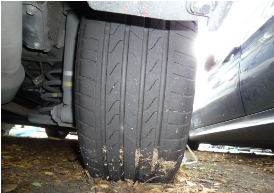
Photo 10 shows the condition of the right rear tyre of the Motor Car, which was observed to be in serviceable condition with remaining tread depth of approximately 5mm. There was also no tear, cut or burst mark(s) on the outer and the inner sidewalls as well as across the tread of the 4 tyres.
