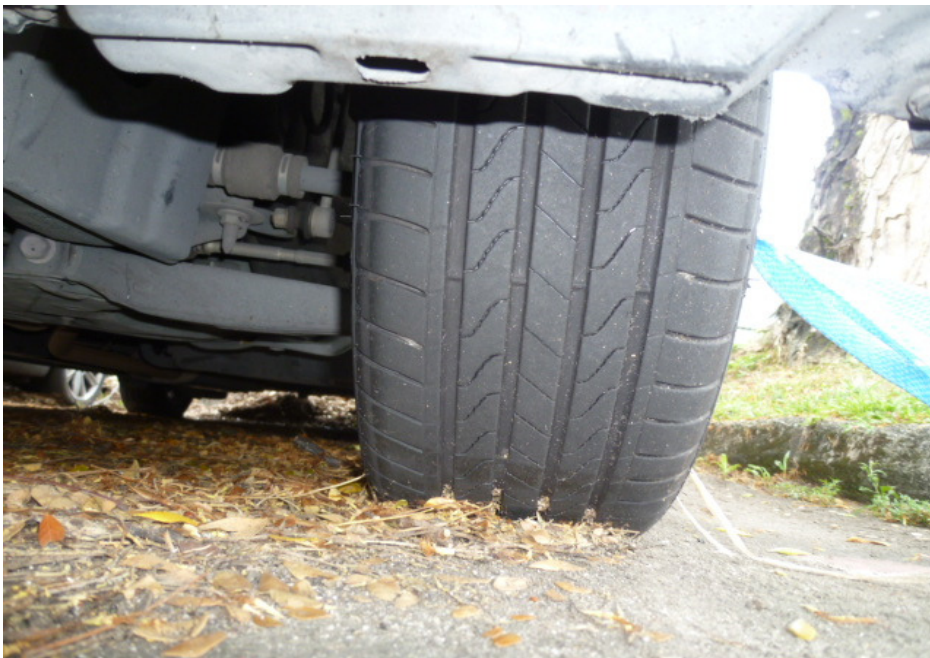
Photo 7 shows the condition of the left front tyre of the Motor Car, which was observed to be in serviceable condition with remaining tread depth of approximately 7mm. The tyre, which was wrapped around alloy wheel rim, was also observed to be sufficiently inflated for vehicular operation. There was no tear, cut or burst mark(s) on the outer and the inner sidewalls as well as across the tread of the 4 tyres.
