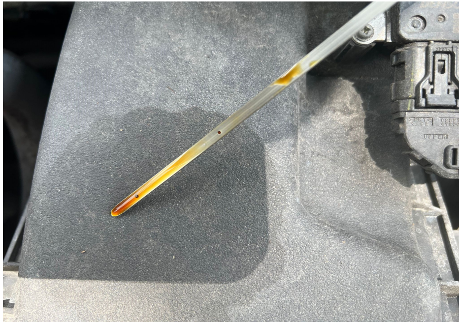
Photo 15 shows the engine oil dip stick of the Motor Car at the time of our inspection. The engine oil was observed to be of sufficient level for operating purposes and without any visible contamination.
