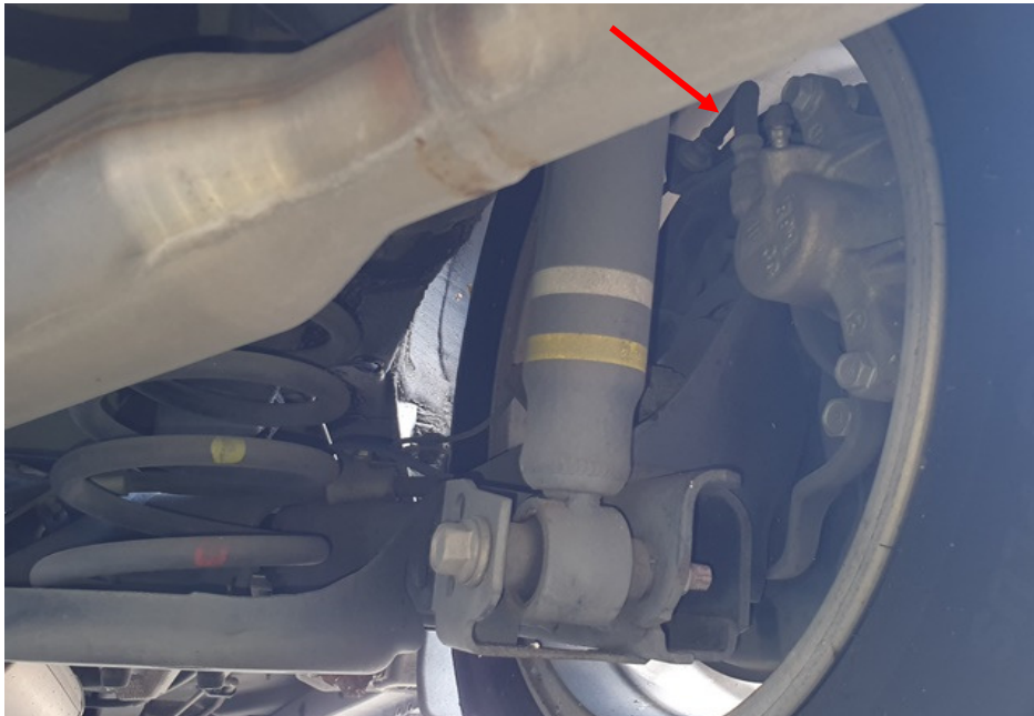
Photo 16 shows the brake hose/pipe (arrowed) at the rear right wheel of the Motor Car. We did not observe any leakage of brake fluid at the time of our inspection of the Motor Car. Static tests of the Motor Car's braking system had indicated that there was no internal leakage of pressure/vacuum. Hence the braking system was likely to be in serviceable condition at the material time of accident. The undercarriage components of the Motor Car were also all found to be intact and without any visible damage.
