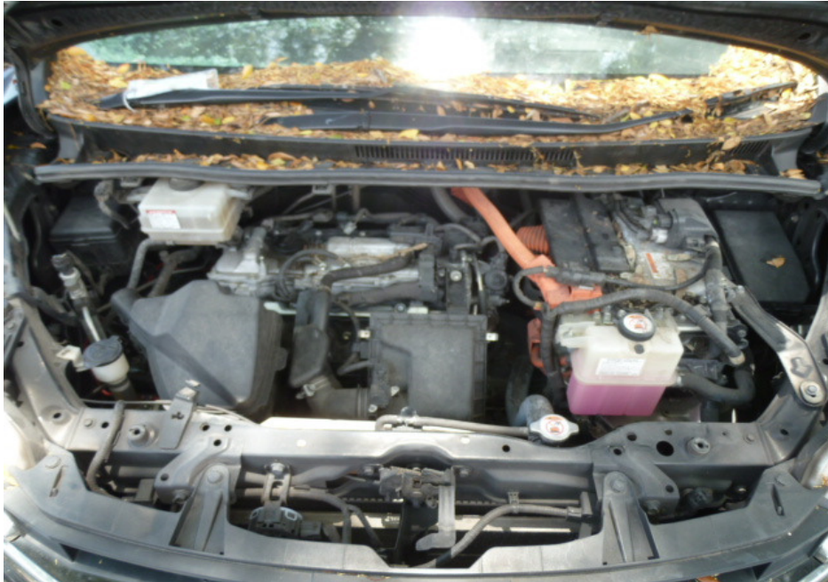
Photo 11 shows a general view of the Motor Car's engine compartment. The various parts and components inside the engine compartment were unaffected by the accident. The wirings and cables for the hybrid system were all further observed to be intact and adequately secured to their respective terminals and/or connecting ports. There was also no sign(s) or indication(s) of fluid leakage and/or fluid stain within the engine compartment.
