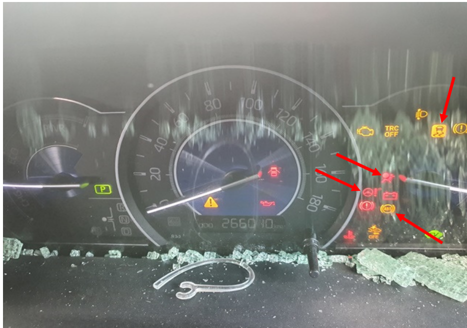
Photo 22 shows the warning lights for the various electronic operating systems of the Motor Car appearing on its instrument panel during the self-test when the engine is cranked, in particular the ABS light, EPS light, ESC light and SRS light (arrowed).
