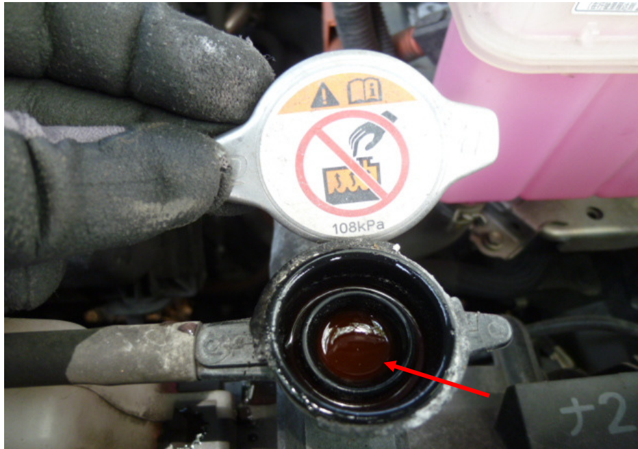
Photo 13 shows checks being carried out to the engine coolant of the Motor Car at the time of our inspection. The engine coolant was observed to be of sufficient level for operating purposes and without any visible contamination (arrowed).
