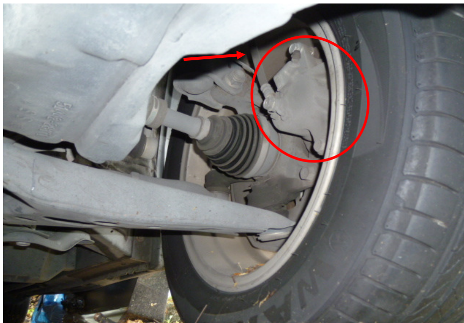
Photo 17 shows the brake hose/pipe (arrowed) at the front left wheel of the Motor Car. No leakage of brake fluid was observed. Visual examination of the various components of the braking system like the brake caliper (circled), brake pedal etc. had revealed all to be intact and without visible damage.
