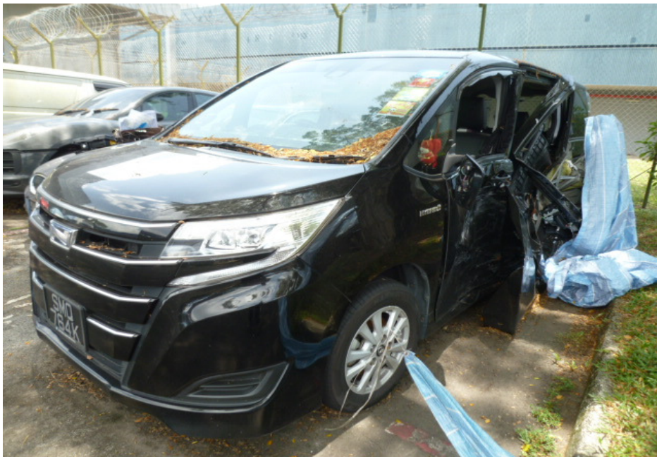
Photo 3 shows a general view of the left body of the Motor Car at the time of our inspection. The Motor Car was observed to be in good general condition. However we had observed impact damage that was confined to its left body. Its left front fender and left front door were observed to be dented. Its left rear door was found to be dislodged. Its left side mirror was observed to be broken.
