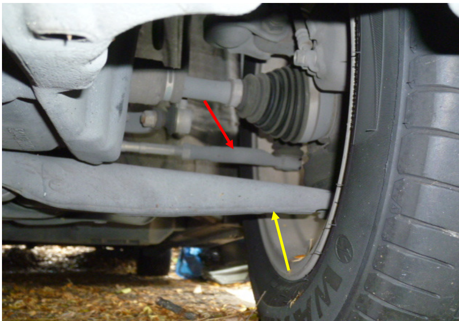
Photo 19 shows the various undercarriage components at the front left wheel of the Motor Car, which had included the steering tie rod (red arrow) and left drive shaft (yellow arrow). The various undercarriage components of the Motor Car were all found to be intact without any visible damage.
