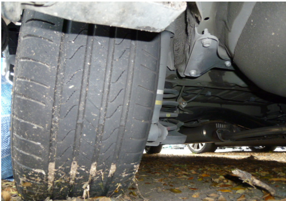
Photo 9 shows the condition of the left rear tyre of the Motor Car, which was observed to be in serviceable condition with remaining tread depth of approximately 5mm. The tyre, which was wrapped around alloy wheel rim, was also observed to be sufficiently inflated for vehicular operation. There was also no damage found on the 4 wheel rims of the Motor Car.
