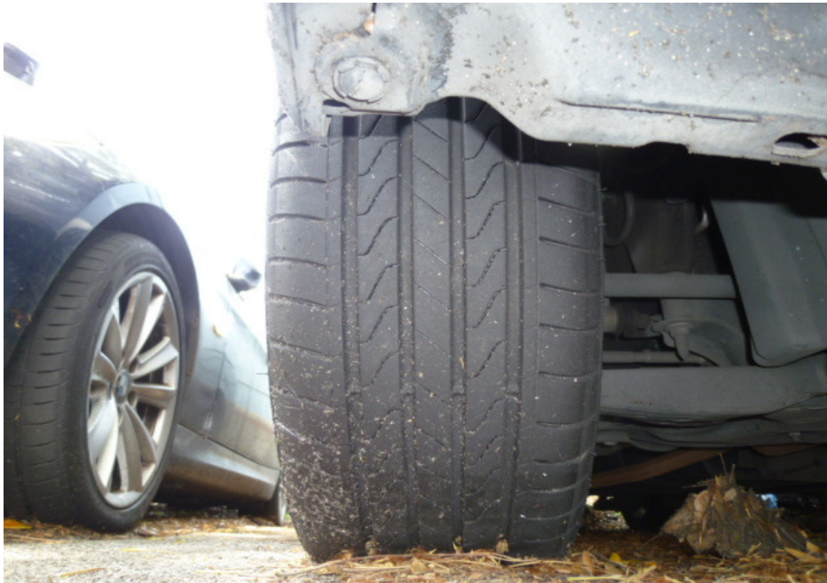
Photo 8 shows the condition of the right front tyre of the Motor Car, which was observed to be in serviceable condition with remaining tread depth of approximately 7mm. The tyre, which was wrapped around alloy wheel rim, was also observed to be sufficiently inflated for vehicular operation.
