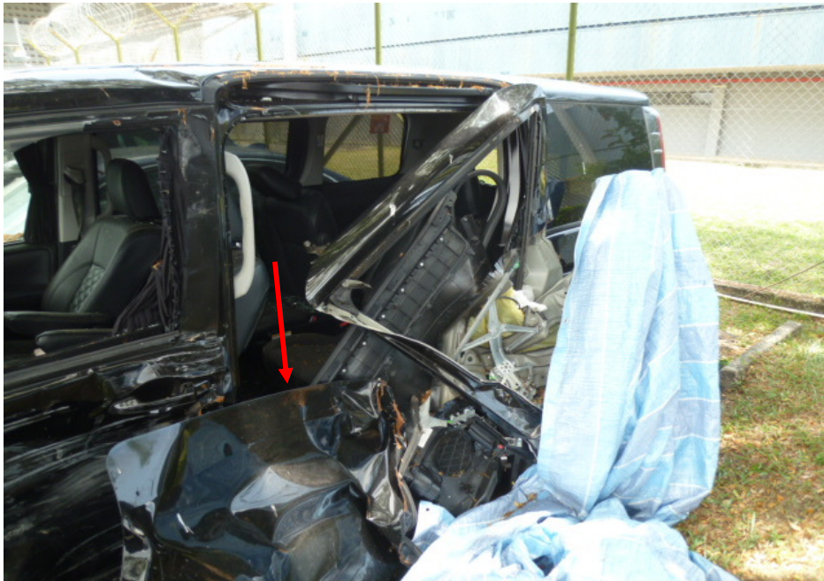
Photo 6 shows the dislodged left rear door (arrowed) of the Motor Car at the time of our inspection.
