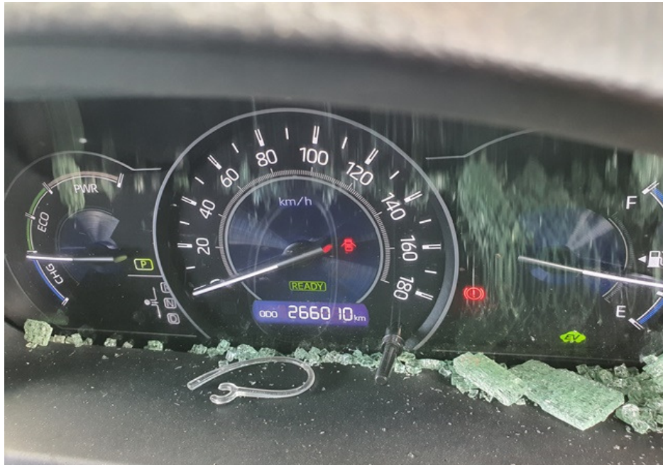
Photo 23 shows no warning lights illuminated on the instrument panel of the Motor Car after the engine was cranked. This would suggest that there was no abnormality to the various electronic operating systems of the Motor Car, like the ABS, EPS, ESC and SRS etc.
