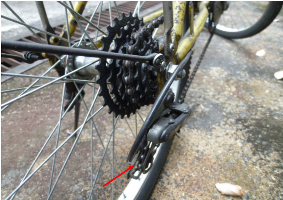
Photo 14 shows a closer view of the dislodged chain from the gear train of the Bicycle, most likely as a result of the accident. It was found to be adequately lubricated for operating purposes (arrowed).
