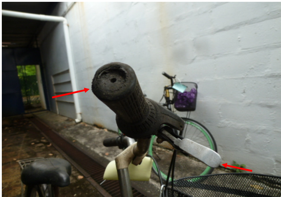
Photo 6 shows the damaged right handlebar grip and right hand brake lever (arrowed) of the Bicycle at the time of our inspection.
