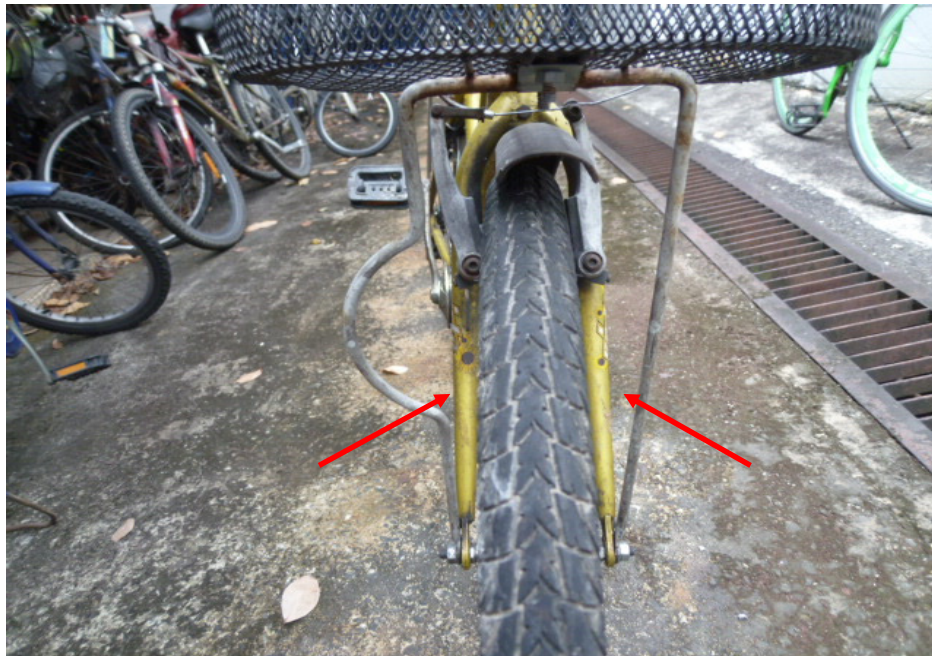
Photo 15 shows the front forks (arrowed) of the Bicycle. The front forks and fork bracket of the Bicycle were both found to be intact and undamaged. Turning the Bicycle's handle bar towards the left and right did not produce any abnormal free play. The steering system of the Bicycle was in serviceable condition at the time of our inspection.
