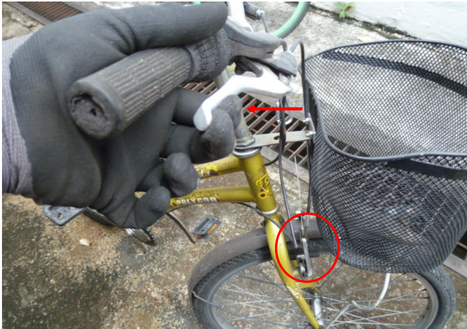
Photo 18 shows a static brake test conducted on the Bicycle's front brake. There was some resistance felt upon pressing the right hand brake lever (arrowed). It also shows that the front brake clamps responded to the gripping action (circled) after depressing the right hand brake lever.
