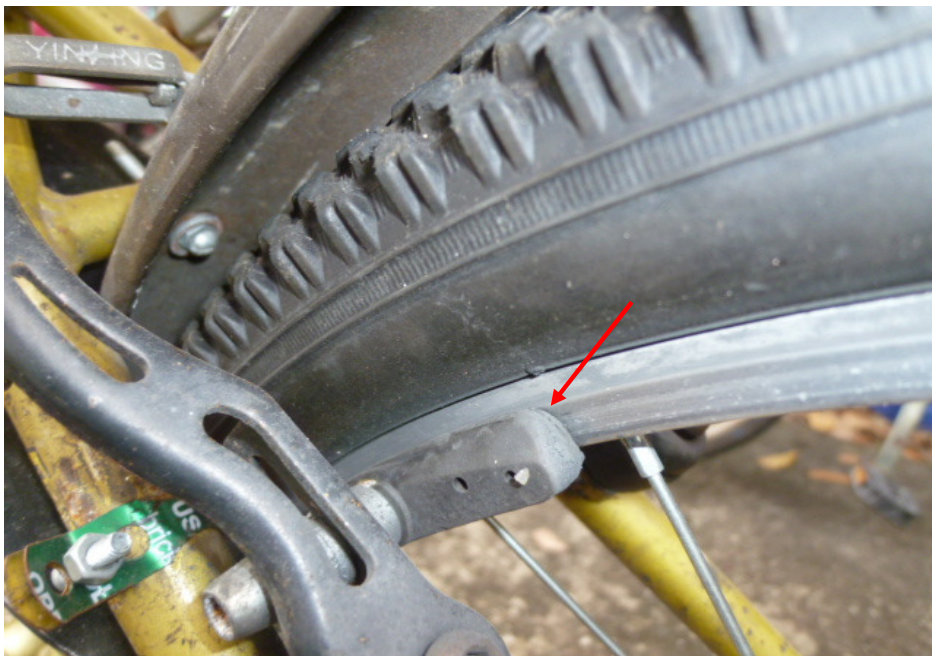
Photo 21 shows a close up view of the rear brake clamps responding to the gripping action. The rubber brake blocks pressed against the rear wheel rim upon depressing the left hand brake lever (arrowed). This had appeared to indicate that the rear brake of the Bicycle was in serviceable condition.
