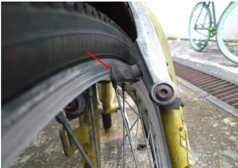
Photo 19 shows a close up view of the front brake clamps responding to the gripping action. The rubber brake blocks pressed against the front wheel rim upon depressing the right hand brake lever (arrowed). This had appeared to indicate that the front brake of the Bicycle was in serviceable condition.
