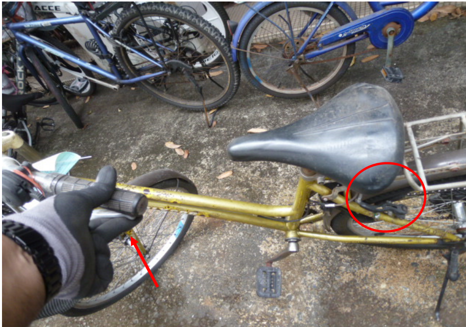
Photo 20 shows a static brake test conducted on the Bicycle's rear brake. There was some resistance felt upon pressing the left hand brake lever (arrowed). It also shows that the rear brake clamps responded to the gripping action (circled) after depressing the left hand brake lever.
