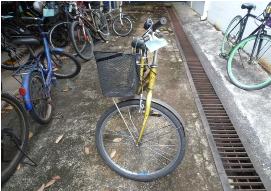
Photo 16 shows the front wheel of the Bicycle turned towards its full right. Turning the Bicycle's handle bar towards the right did not produce any abnormal free play and/or resistance. This would indicate that the steering system of the Bicycle was in serviceable condition at the time of our inspection.
