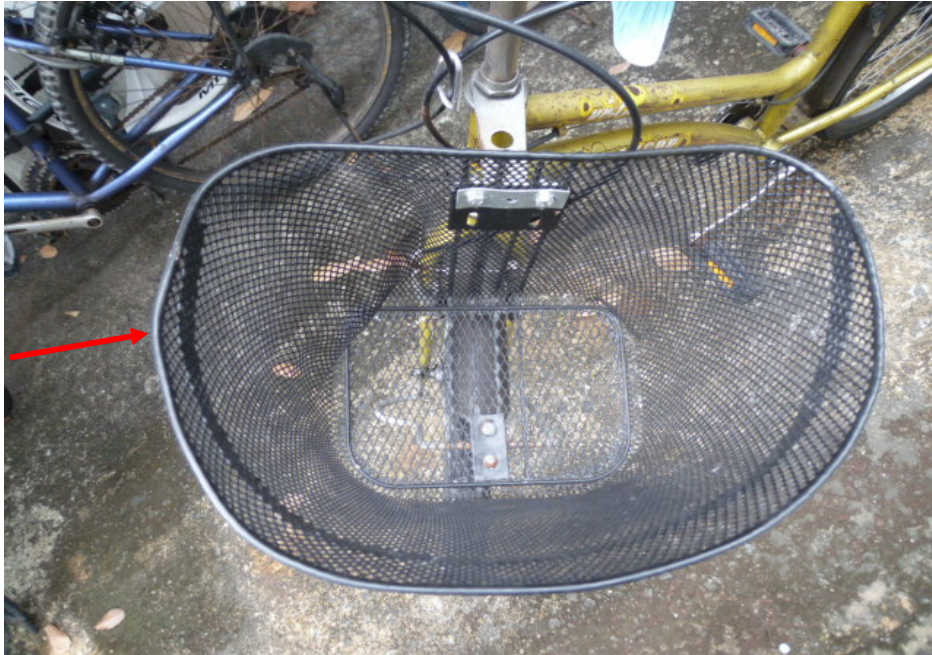
Photo 9 shows the deformed front basket of the Bicycle at the time of our inspection (arrowed).
