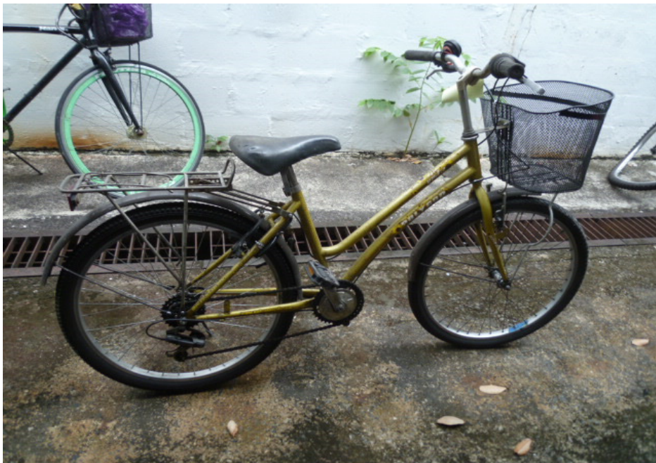
Photo 4 shows the right body of the Bicycle at time of our inspection. The Bicycle had sustained damages at its right body. The body parts that were found to have been damaged include its front basket, right handlebar grip, front mudguard, right hand brake lever, right pedal and seat, amongst others as a result of the accident.
