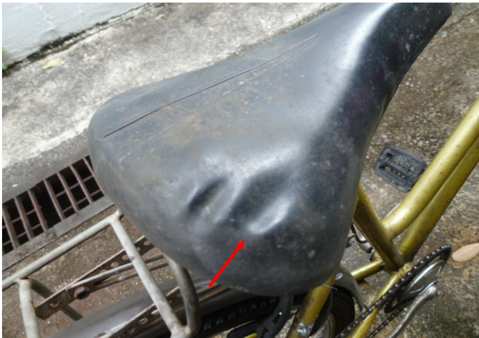
Photo 10 shows a close-up view of the deformed seat (arrowed) of the Bicycle as a result of the accident.
