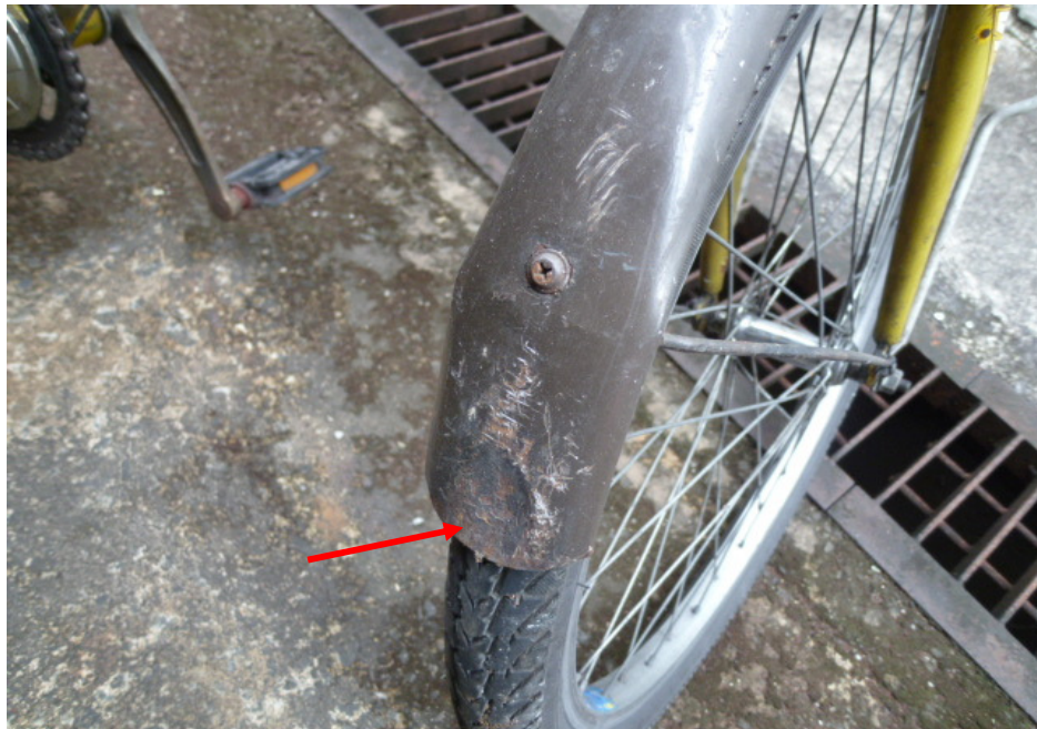
Photo 7 shows the damaged front mudguard (arrowed) of the Bicycle at the time of our inspection.
