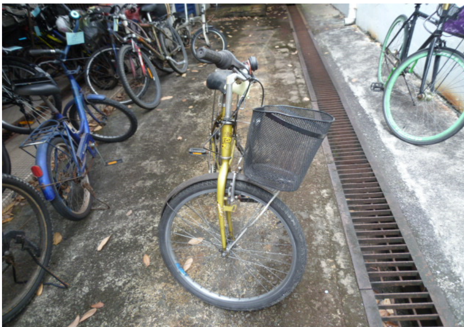
Photo 17 shows the front wheel of the Bicycle turned towards its full left. Turning the Bicycle's handle bar towards the left did not produce any abnormal free play and/or resistance. This would indicate that the steering system of the Bicycle was in serviceable condition at the time of our inspection.
