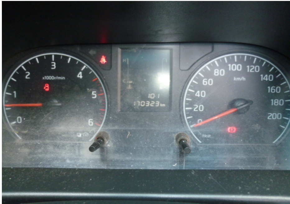
Photo 18 shows no warning lights illuminated on the instrument panel of the Motor Van after the engine was cranked. This would suggest that there was no abnormality to the various electronic operating systems of the Motor Van, like the ABS.
