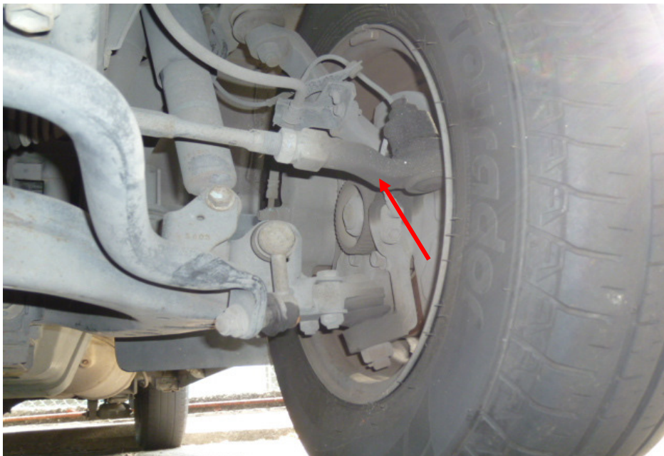
Photo 16 shows the various undercarriage components at the front left wheel of the Motor Van, in particular the steering tie rod (arrowed). The various undercarriage components of the Motor Van were all found to be intact without any visible damage. There was also no sign of fluid stain(s) observed on the various undercarriage components.
