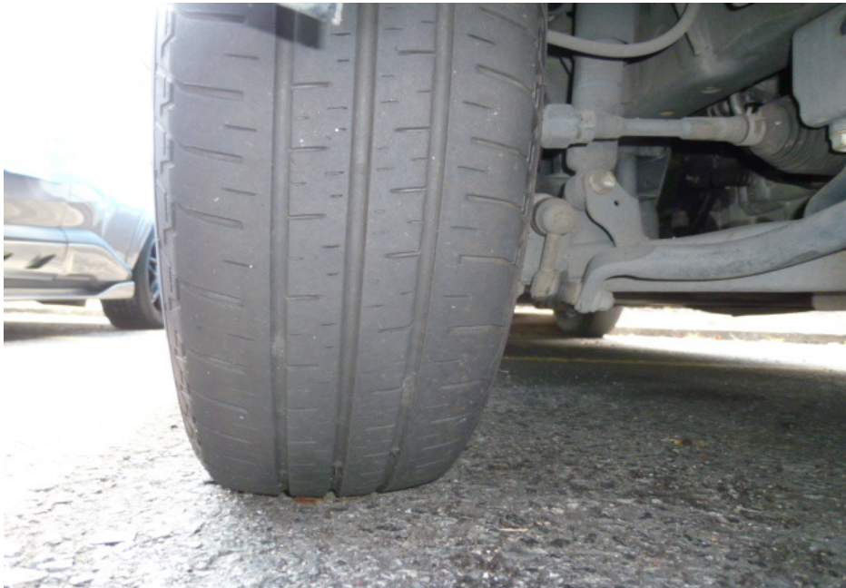
Photo 5 shows the condition of the front right tyre of the Motor Van, which was observed to be in serviceable condition with remaining tread depth of approximately 4mm. The tyre, which was wrapped around a standard steel wheel rim, was also observed to be sufficiently inflated for vehicular operation.
