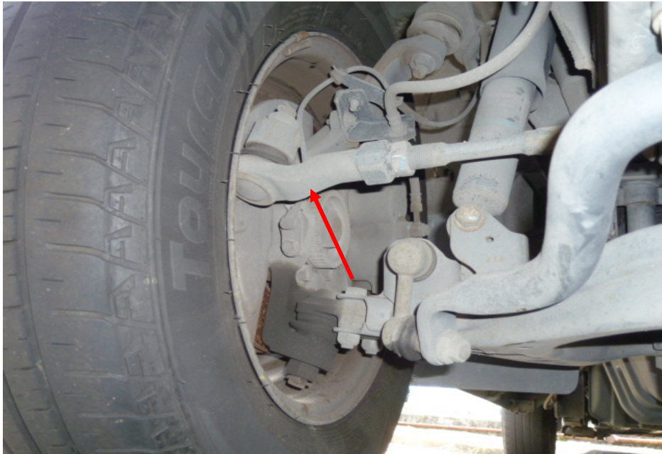
Photo 15 shows the various undercarriage components at the front right wheel of the Motor Van, in particular the steering tie rod (arrowed). The various steering components were all found to be intact, suggesting that the steering system of the Motor Van was likely to be in serviceable condition at the material time of accident. There was also no sign of fluid stain(s) observed on the various undercarriage components.
