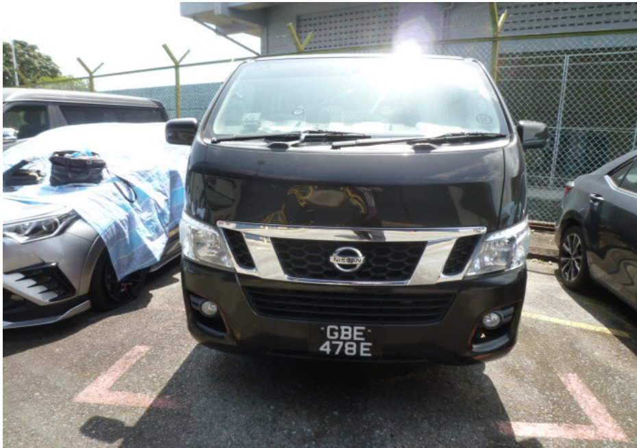
Photo 1 shows a general view of the frontal portion of the Motor Van at the time of our inspection. The Motor Van was observed to have sustained minimal impact damage that was confined to its frontal portion. The mileage of the Motor Van was recorded to be 170, 323km.
