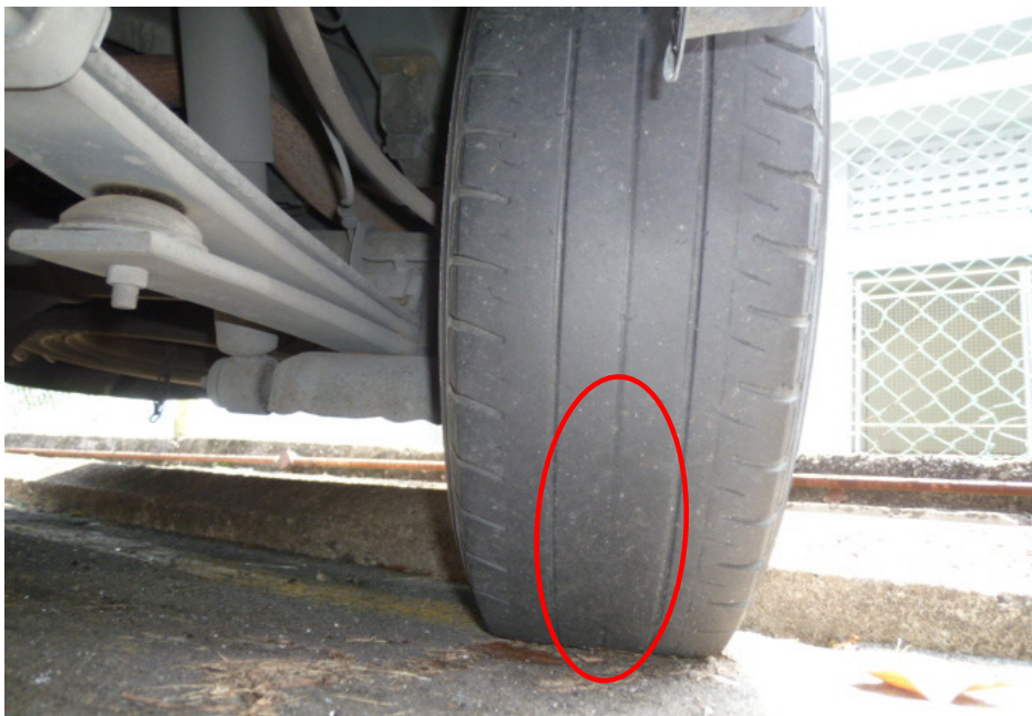
Photo 6 shows the condition of the rear left tyre of the Motor Van, which was observed to be in serviceable condition with remaining tread depth of approximately 7mm. However the pattern at the centre portion of the tread was observed to be flushed with the tyre wear indicator (circled). The tyre, which was wrapped around standard steel wheel rim, was also observed to be sufficiently inflated for vehicular operation.
