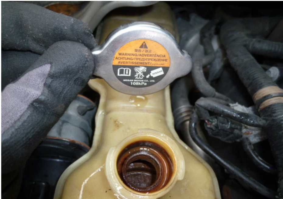
Photo 10 shows the engine coolant reservoir of the Motor Van at the time of our inspection. The engine coolant was observed to be of sufficient level for operating purposes and without any visible contamination.
