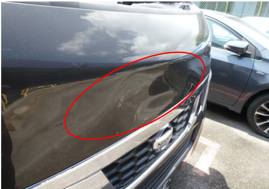
Photo 2 shows a closer view of the frontal portion of the Motor Van at the time of our inspection. The Motor Van was observed to have sustained minimal impact damage that was confined to its frontal portion. Its front bonnet was dented as a result of the accident (circled).
