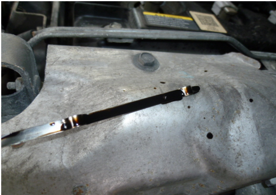
Photo 11 shows the engine dip stick of the Motor Van at the time of our inspection. The engine oil was observed to be of sufficient level for operating purposes and without any visible contamination.
