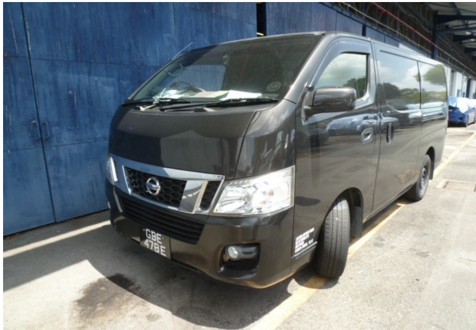
Photo 14 shows the front left wheel of the Motor Van turned to its full left. During our steering system test, we did not experience any abnormal free play and/or resistance when we had turned the steering wheel towards the left and right. This would suggest that the steering system of the Motor Van was likely to be in serviceable condition at the material time of accident.
