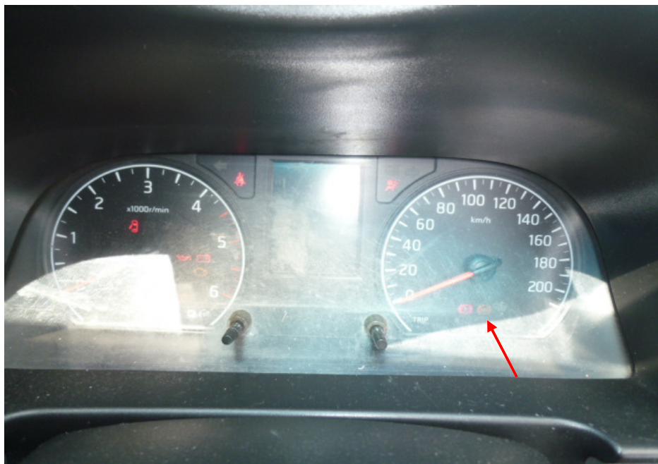
Photo 17 shows the warning lights for the various electronic operating systems of the Motor Van appearing on its instrument panel during the self-test when the engine is cranked, in particular the Antilock Braking System (ABS) light (arrowed).
