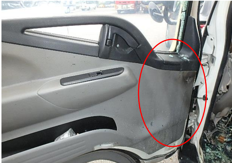
Photo 5 shows the close up view of the interior compartment of the Insured Vehicle at the time of our inspection. Its left door (circled) was observed to sustain smoke and heat damages as a result of the fire.
