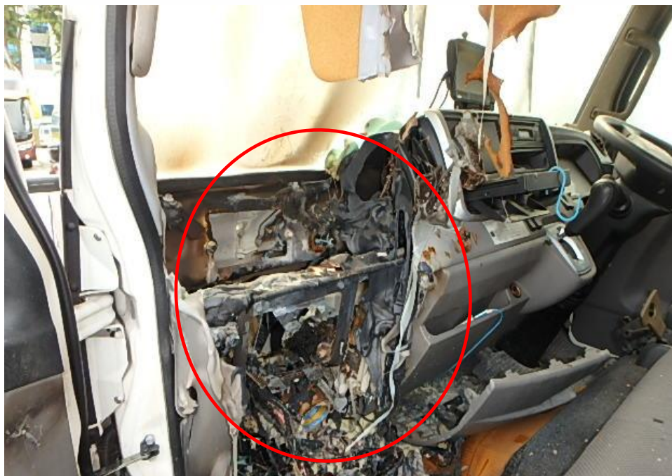
Photo 6 shows the close up view of the interior compartment of the Insured Vehicle at the time of our inspection. The fire was confined to its front left dashboard portion, its front dashboard, electronic components & wirings (circled) were observed to sustain heat and smoke damages as a result of the fire.
