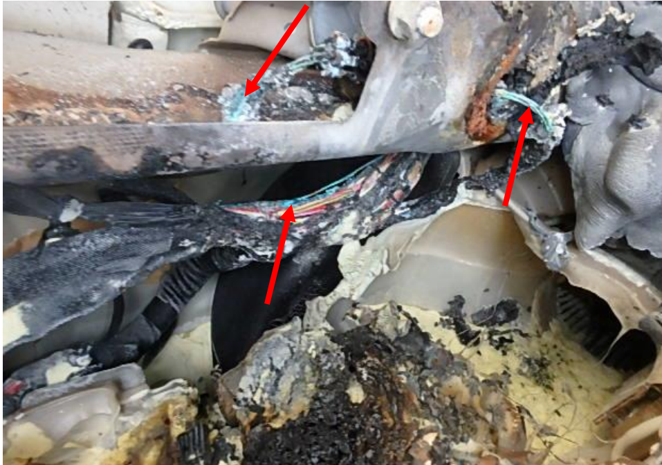
Photo 8 shows a close up view of the original wiring harness leading from the fuse box to the electrical components. The original wiring harness (arrowed) was observed with greenish residue on the surface. The presence of greenish residue indicates internal heating of copper wires, a sign of an electrical short circuit occurring. The greenish residue is normally left behind from oxidation as a result of chemical reaction involving the copper wires. This is likely where the fire had started from.
