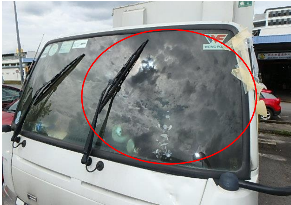
Photo 4 shows the general view of the interior compartment of the Insured Vehicle at the time of our inspection. The fire was confined to its front left dashboard portion, however the fire had resulted in the various components located in the interior of the Insured Vehicle suffer from heat and smoke damages, this includes the front windscreen (circled) and several parts at the front dashboard that were also observed to sustain damages included electronic components & wirings.
