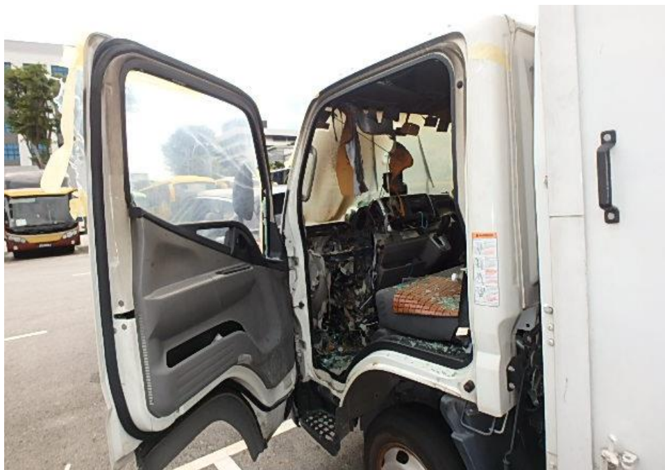
Photo 3 shows the general view of the interior compartment of the Insured Vehicle at the time of our inspection. The fire was confined to its front left dashboard portion, however the fire had resulted in the various components located in the interior of the Insured Vehicle suffer from heat and smoke damages, this includes the front windscreen and several parts at the front dashboard that were also observed to sustain damages included electronic components & wirings.
