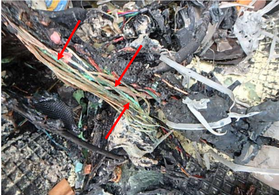
Photo 9 shows a close up view of the original wiring harness leading from the fuse box to the electrical components. The original wiring harness (arrowed) was observed with greenish residue on the surface. The presence of greenish residue indicates internal heating of copper wires, a sign of an electrical short circuit occurring. The greenish residue is normally left behind from oxidation as a result of chemical reaction involving the copper wires. This is likely where the fire had started from.
