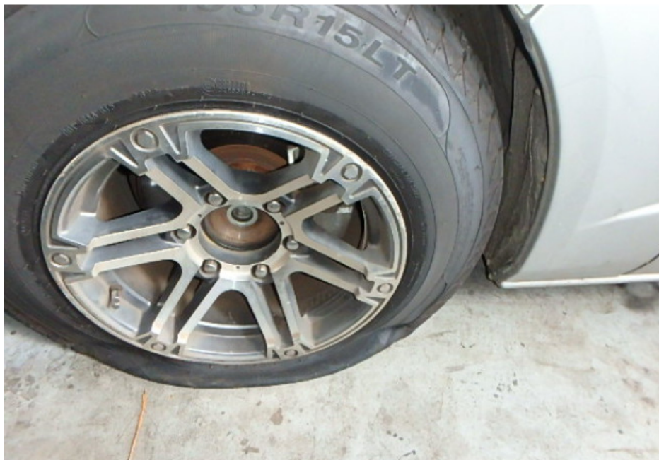
Photo 5 shows a closer view of the non-standard rim found to be fitted on the Insured Vehicle at the time of our inspection. The 15- inch alloy rims fitted on the Insured Vehicle were not the standard type for the Insured Vehicle.
