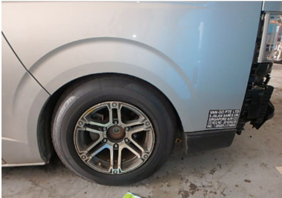
Photo 4 shows the non-standard rim found to be fitted on the Insured Vehicle at the time of our inspection. The 15- inch alloy rims fitted on the Insured Vehicle were not the standard type for the Insured Vehicle.
