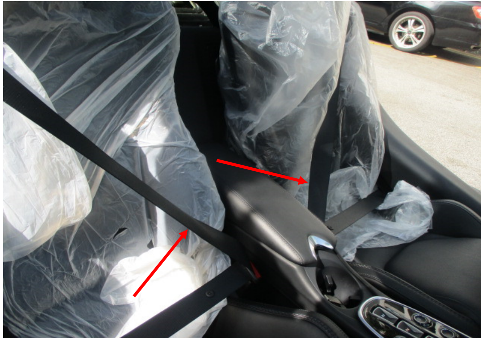
Photo 16 shows the seats of the Motor Car. All the seats of the Motor Car were secured via seat rails to the floorboard. They were also fitted with a retractable seat belt reel and a pre-tensioner. The seat belts (arrowed) were tested and were able to be fastened into the respective pre-tensions that were fitted on the side of each individual seat.
