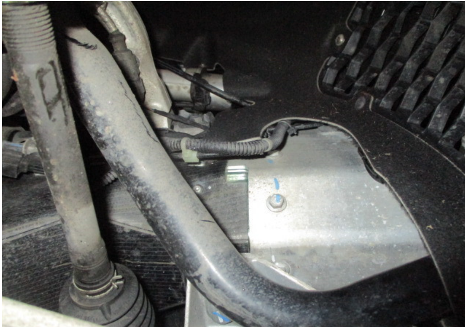
Photo 30 shows the aluminium chassis/structural body at the underside front right of the Motor Car. The original factory sealant at the joints along the chassis/structural body was observed to be untouched. In general, I had found no work was carried out on the chassis/structural body of the Motor Car. The aluminium chassis/structural body of the Motor Car was originally fitted.
