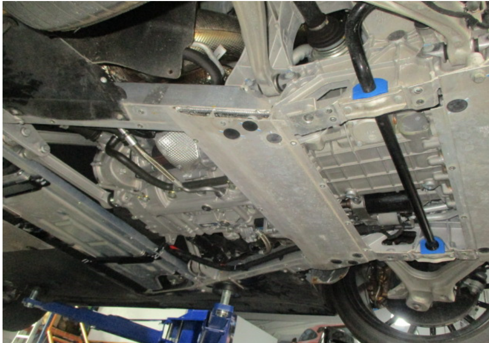
Photo 26 shows another view of the Motor Car's engine compartment as viewed from the rear underside of the Motor Car, after dismantling of the rear undercovers. The various parts and components inside the engine compartment were all observed to be intact and properly fitted. There was also no sign(s) or indication(s) of fluid leak and/or fluid stain found inside the engine compartment.
