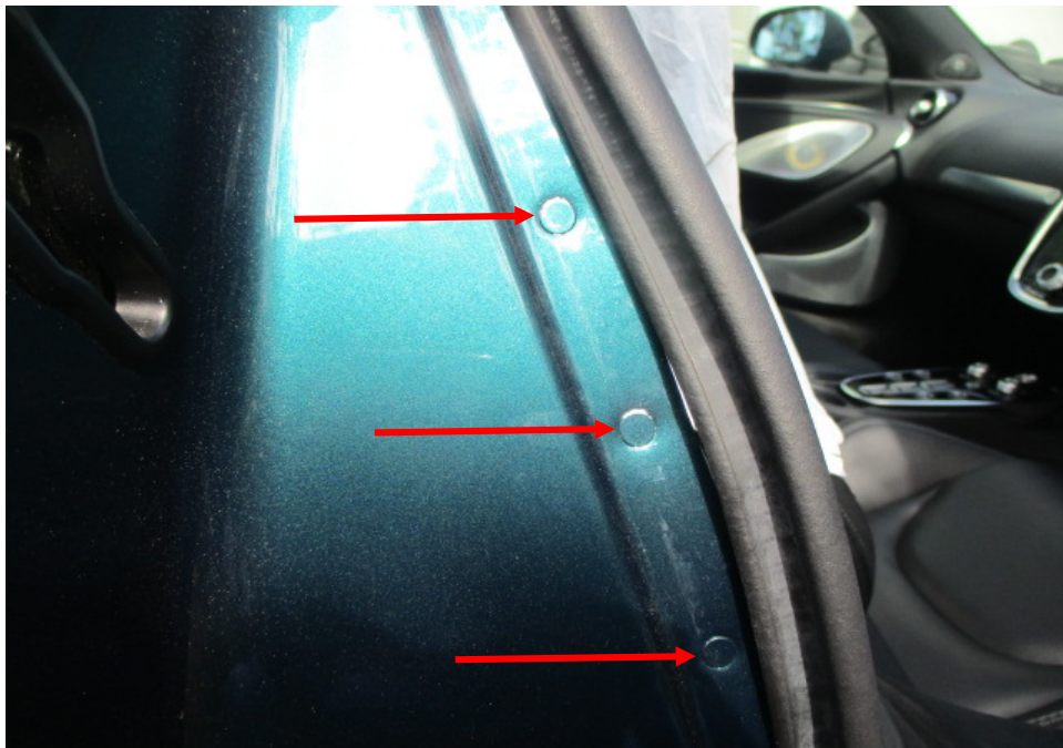
Photo 33 shows the right side rear body panel of the Motor Car. I did not find any weld marks other than original spot weld marks (arrowed) on the right side rear body panel pillar of the Motor Car which, indicates that there was no re-welding works carried out. In general, I had found all the non-detachable body panels of the Motor Car to be originally fitted at the time of my inspection.
