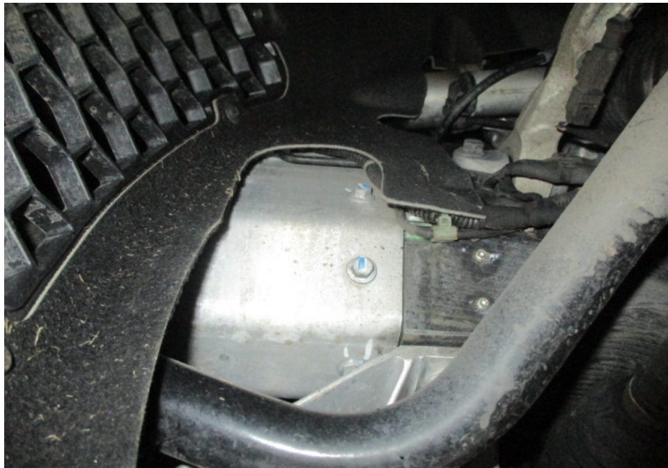
Photo 29 shows the aluminium chassis/structural body at the underside front left of the Motor Car. The original factory sealant at the joints along the chassis/structural body was observed to be untouched. In general, I had found no work was carried out on the chassis/structural body of the Motor Car. The aluminium chassis/structural body of the Motor Car was originally fitted.
