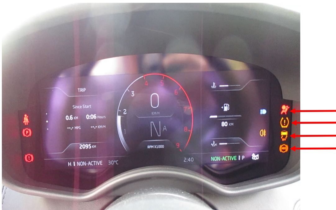
Photo 17 shows the warning lights for the various electronic safety features appearing on the instrument panel of the Motor Car during its self-test when the engine is cranked, in particular the ABS, SRS, TPM and TCS lights (arrowed).
