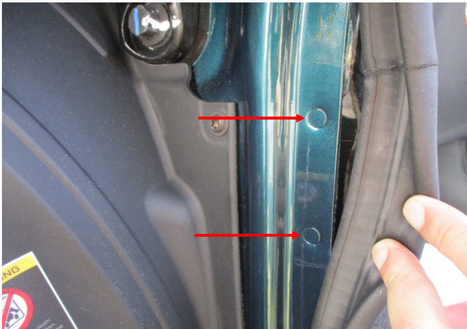
Photo 31 shows the left side "A" pillar of the Motor Car. I did not find any weld marks other than original spot weld marks (arrowed) on the left side "A" pillar of the Motor Car which, indicates that there was no re-welding works carried out. In general, I had found all the non-detachable body panels of the Motor Car to be originally fitted at the time of my inspection.
