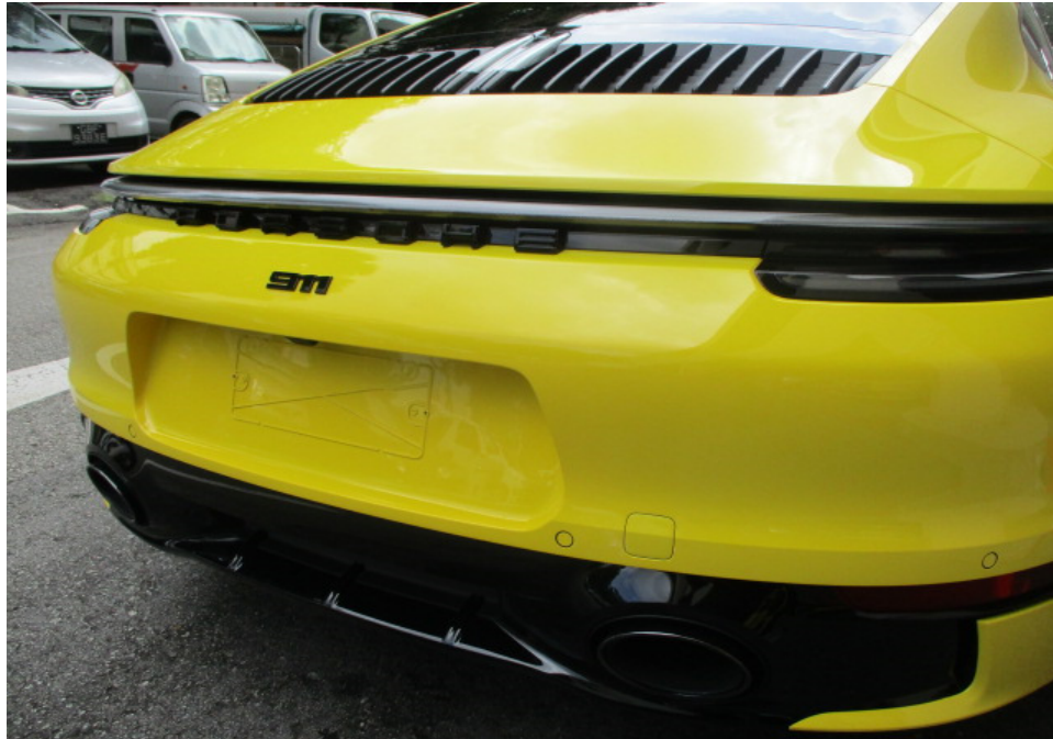
Photo 16 shows a closer view of the Motor Car's rear bumper, rear bumper lower cover, rear right taillamp and rear centre lamp. The body parts at the rear portion of the Motor Car were visually examined and it was observed that the repair/restoration works carried out to the damaged area of the Motor Car (refer to photograph 3 & 4 above) were reasonably adequate and in order.
