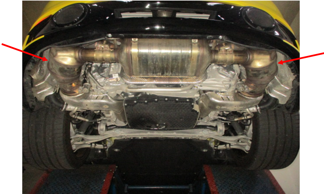
Photo 28 shows the Motor Car's exhaust system. My examination of the Motor Car's exhaust system revealed no sign(s) or indication(s) of any cut or weld marks along its exhaust pipes, on its catalytic converters (arrowed) and on its rear muffler.
