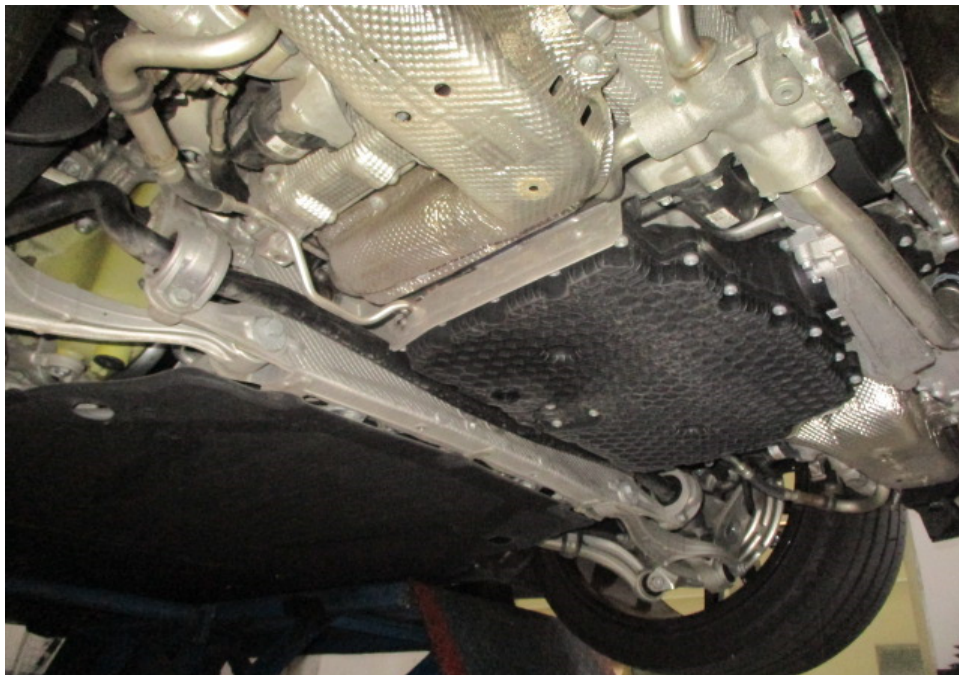
Photo 29 shows a general view of the Motor Car's engine compartment. The engine compartment was at the rear underside of the Motor Car. The various parts and components within the engine compartment were all observed to be intact and properly fitted. There was also no sign(s) or indication(s) of fluid leak and/or fluid stain found inside the engine compartment.
