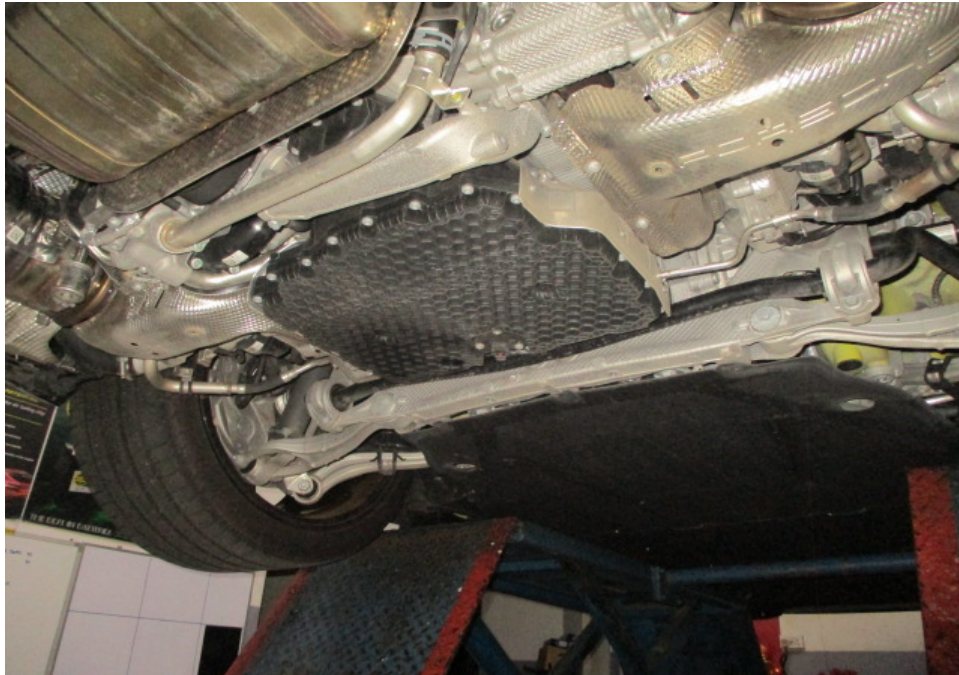
Photo 30 shows another view of the Motor Car's engine compartment. The engine compartment was at the rear underside of the Motor Car. The various parts and components within the engine compartment were all observed to be intact and properly fitted. There was also no sign(s) or indication(s) of fluid leak and/or fluid stain found inside the engine compartment.
