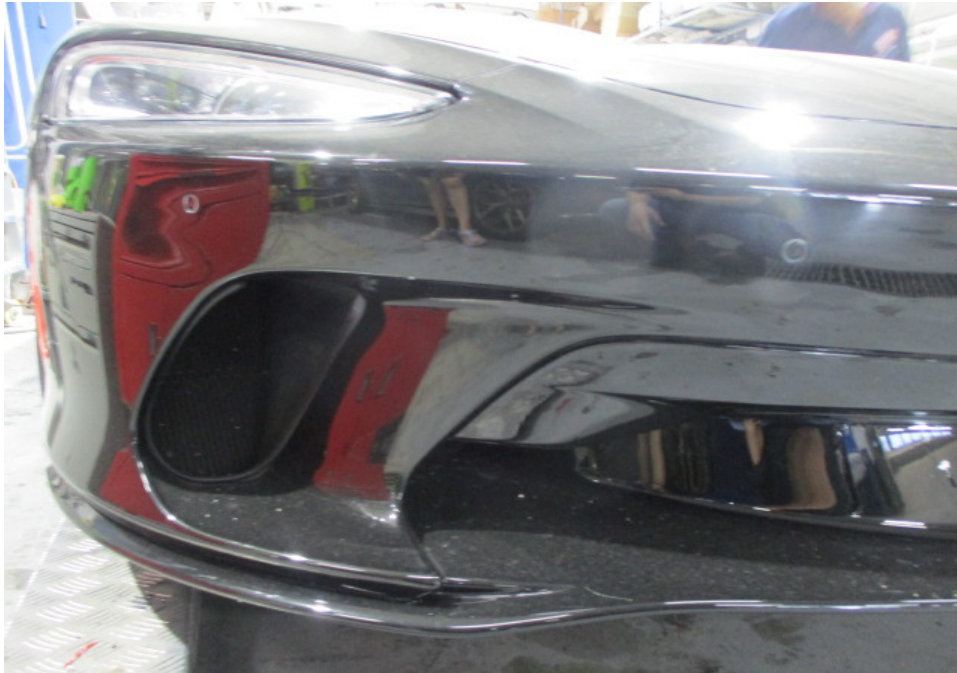
Photo 7 shows a closer view of the Motor Car's front bumper, front bumper lower cover, front bumper sensors, front bumper right air duct and front right headlamp at the time of my inspection. The body parts at the frontal portion of the Motor Car were visually examined and it was observed that the repair/restoration works carried out to the damaged area of the Motor Car (refer to photograph 1 & 2 above) were reasonably adequate and in order.
