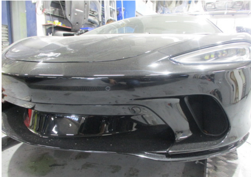
Photo 11 shows a closer view of the Motor Car's front bumper, front bumper lower cover, front bumper sensors, front bonnet and front left headlamp. The body parts at the frontal portion of the Motor Car were visually examined and it was observed that the repair/restoration works carried out to the damaged area of the Motor Car (refer to photograph 1 & 2 above) were reasonably adequate and in order.
