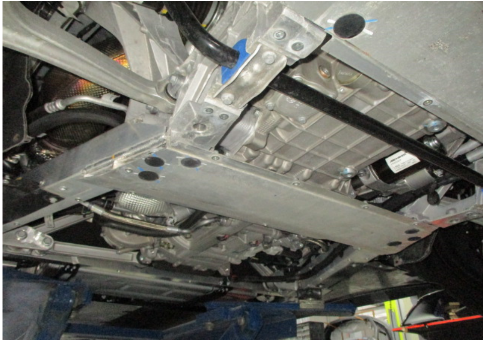
Photo 31 shows another view of the Motor Car's engine compartment as viewed from the rear underside of the Motor Car. The various parts and components inside the engine compartment were all observed to be intact and properly fitted. There was also no sign(s) or indication(s) of fluid leak and/or fluid stain found inside the engine compartment.
