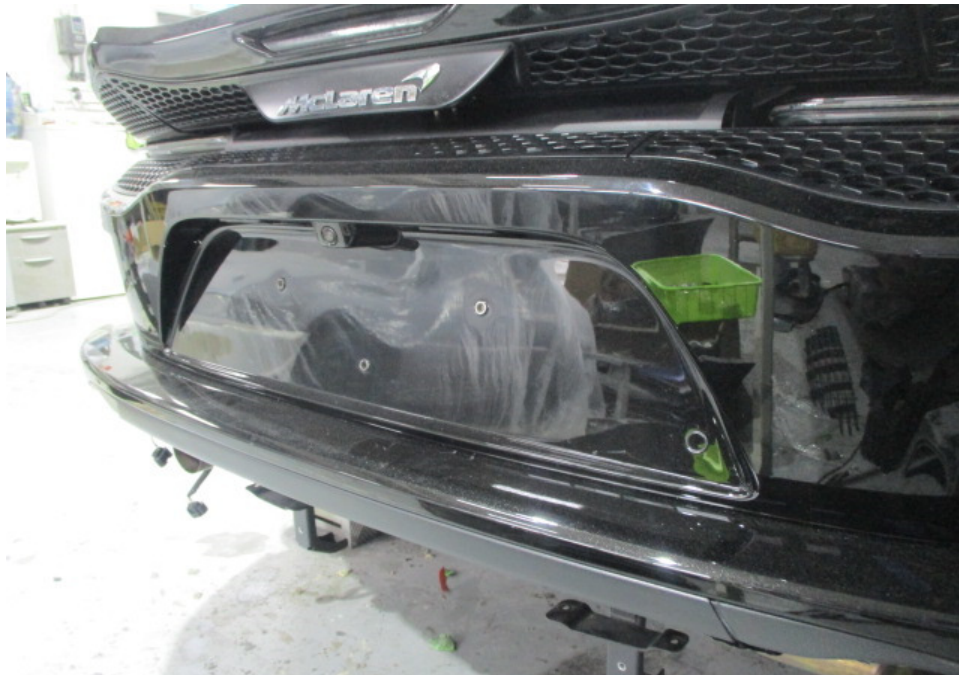
Photo 16 shows a closer view of the Motor Car's rear bumper and rear bumper top centre grille. The body parts at the rear portion of the Motor Car were visually examined and it was observed that the repair/restoration works carried out to the damaged area of the Motor Car (refer to photograph 3 & 4 above) were reasonably adequate and in order.
