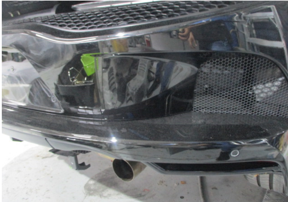
Photo 15 shows a closer view of the Motor Car's rear bumper, rear bumper right grille and rear bumper right sensor. The body parts at the rear portion of the Motor Car were visually examined and it was observed that the repair/restoration works carried out to the damaged area of the Motor Car (refer to photograph 3 & 4 above) were reasonably adequate and in order.
