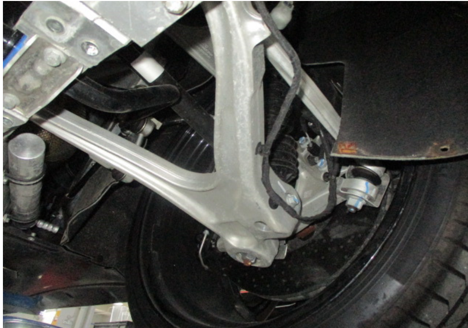
Photo 25 shows a general view of the control arms and linkages at the rear right wheel of the Motor Car. I did not observe any fluid leak and/or fluid stain on the underside of the Motor Car. All of the Motor Car's undercarriage components were observed to be intact and secured in an appropriate manner.
