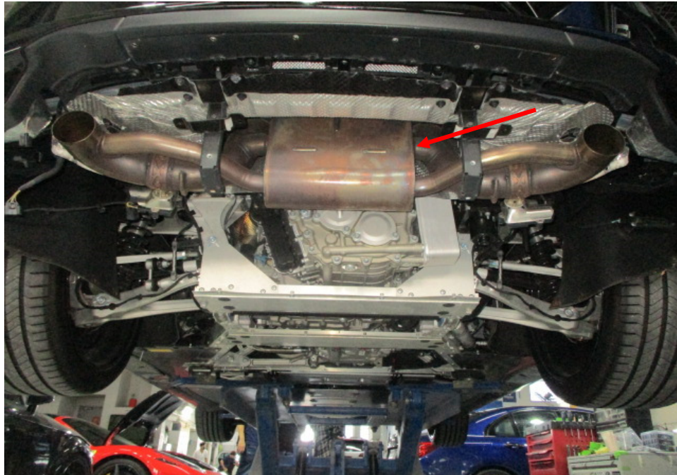
Photo 29 shows the Motor Car's exhaust system. In general, my examination of the Motor Car's exhaust system revealed no sign(s) or indication(s) of any cut or weld marks along its exhaust pipes, on its catalytic converters and on its rear muffler (arrowed).
