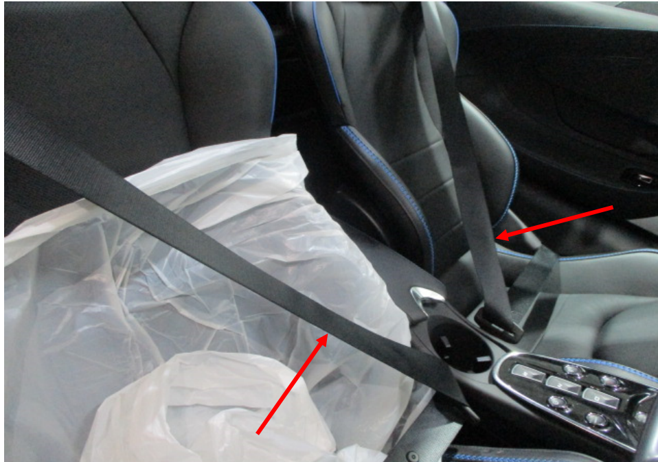
Photo 21 shows the seats of the Motor Car. All the seats of the Motor Car were secured via seat rails to the floorboard. They were also fitted with a retractable seat belt reel and a pre-tensioner. The seat belts (arrowed) were tested and were able to be fastened into the respective pre-tensions that were fitted on the side of each individual seat.
