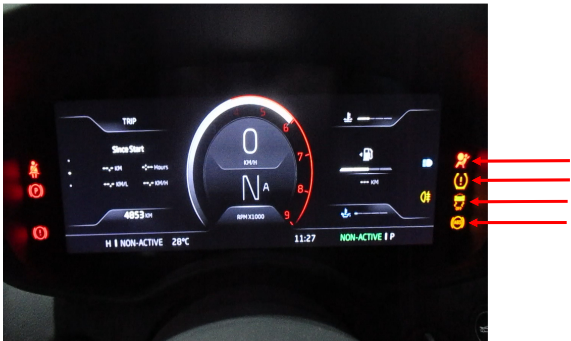
Photo 22 shows the warning lights for the various electronic safety features appearing on the instrument panel of the Motor Car during its self-test when the engine is cranked, in particular the ABS, SRS, TPM and TCS lights (arrowed).
