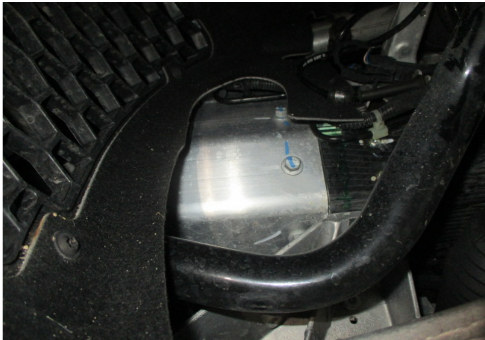
Photo 34 shows the aluminium chassis/structural body at the underside front left of the Motor Car. The original factory sealant at the joints along the chassis/structural body was observed to be untouched. In general, I had found no work was carried out on the chassis/structural body of the Motor Car. The aluminium chassis/structural body of the Motor Car was originally fitted.
