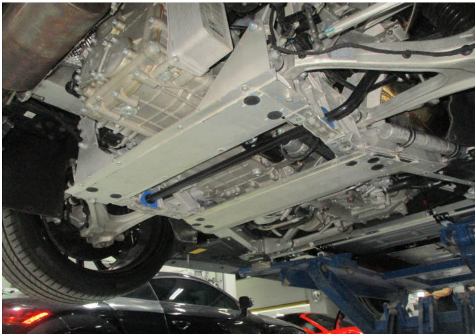
Photo 30 shows the Motor Car's engine compartment as viewed from the rear underside of the Motor Car. The various parts and components inside the engine compartment were all observed to be intact and properly fitted. There was also no sign(s) or indication(s) of fluid leak and/or fluid stain found inside the engine compartment.
