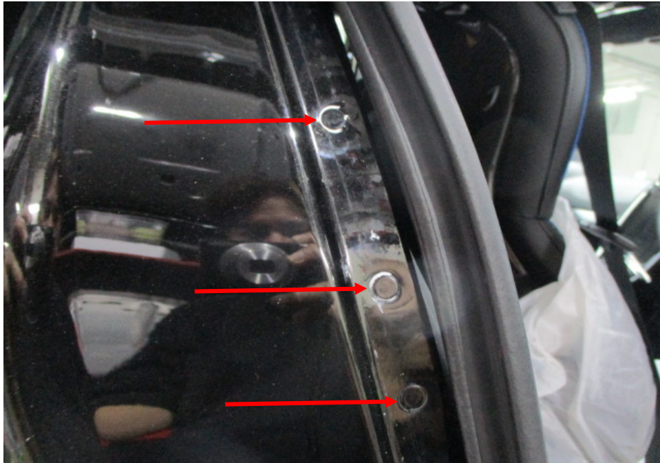
Photo 39 shows the right side rear body panel of the Motor Car. I did not find any weld marks other than original spot weld marks (arrowed) on the right side rear body panel of the Motor Car, which indicates that there was no re-welding works carried out. In general, I had found all the non-detachable body panels of the Motor Car to be originally fitted at the time of my inspection.
