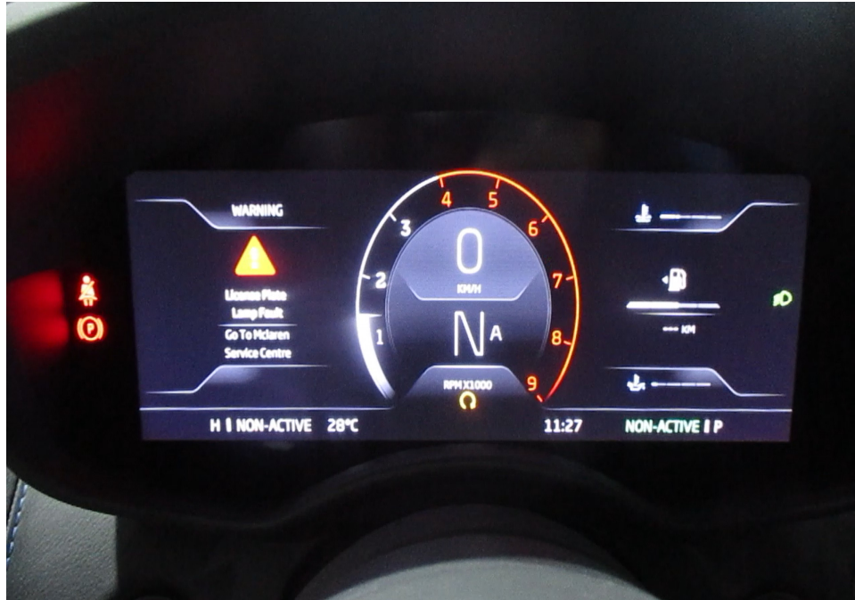
Photo 23 shows the respective warning lights no longer illuminated, indicating that there is no fault detected to the ABS, SRS, TPM and TCS systems of the Motor Car during the self-test. These electronic systems were hence in working condition at the time of my inspection.
