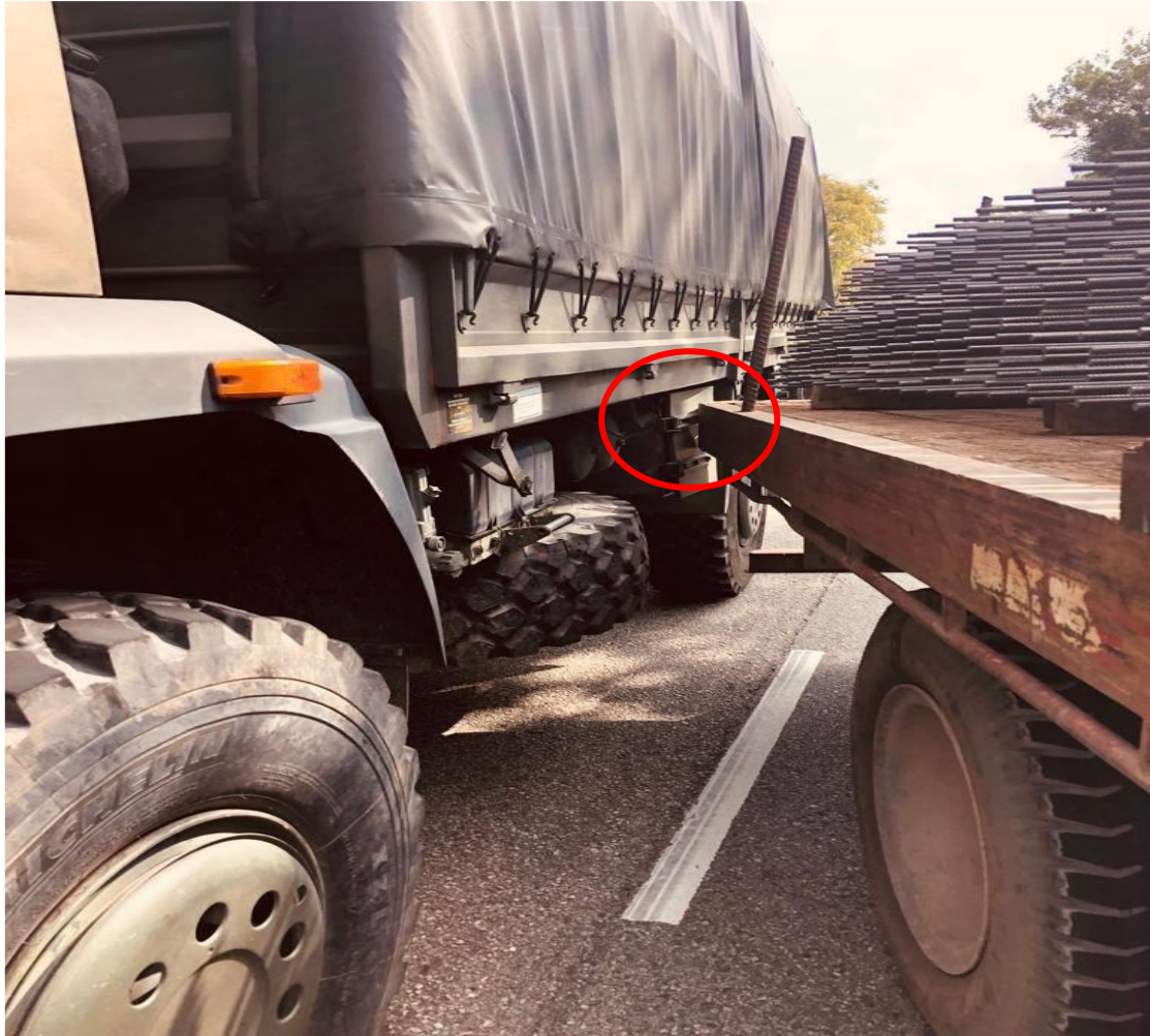
Figure 2I: Zoom in image on civilian flatbed XD4333H damage on 5-TON (MID21383) BII Compartment Box
