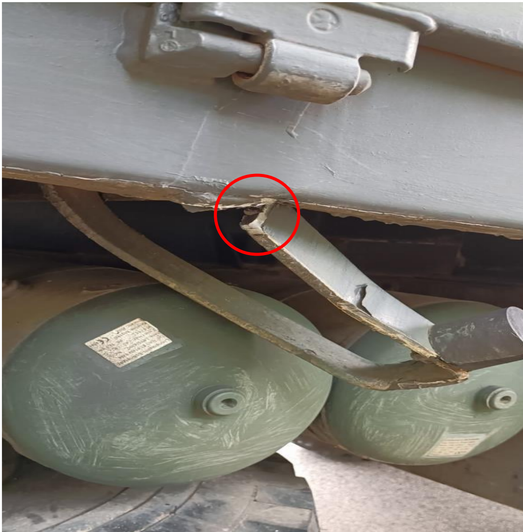
Figure 2F: Close up view of damages to LHS rubber stopper of MID 21383
