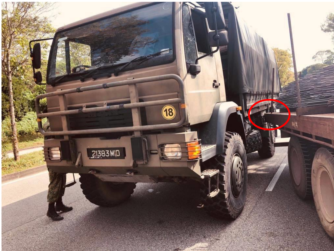
Figure 2H: Civilian flatbed XD4333H protrude out onto 5-TON (MID21383) BII Compartment Box
