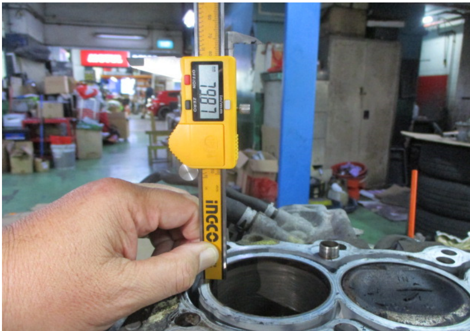
Photo 10 shows the stroke measurement of cylinder 1, which was recorded to be 79.87mm.
