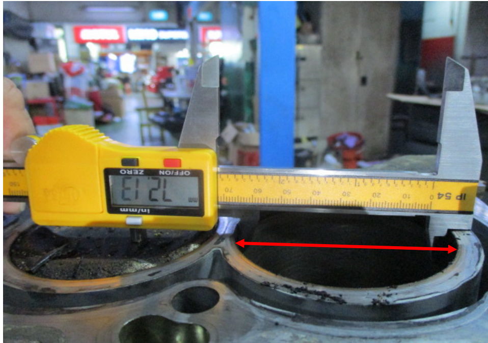
Photo 19 shows measurement being carried out to the bore (arrowed) of cylinder 4 of the Honda engine. The bore measurement of cylinder 4 was recorded to be 72.13mm.
