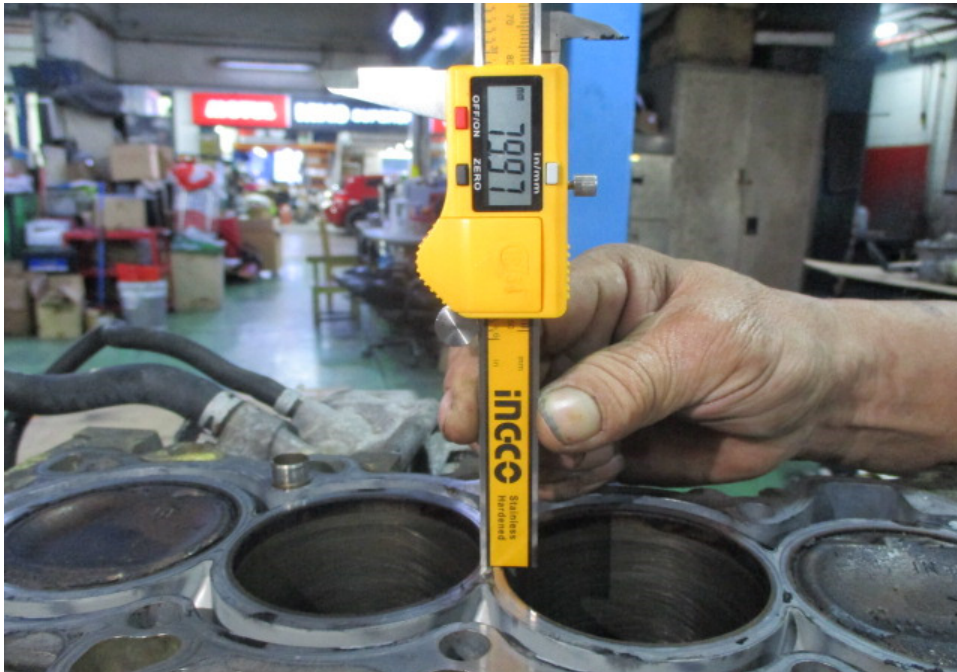
Photo 18 shows the stroke measurement of cylinder 3, which was recorded to be 79.97mm.
