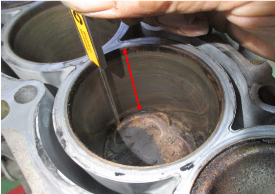
Photo 17 shows measurement being carried out to the stroke (arrowed) of cylinder 3 of the Honda engine. The bore and stroke measurements of the Honda engine were carried out using a digital Vernier Caliper that was calibrated before the start of the measurements.
