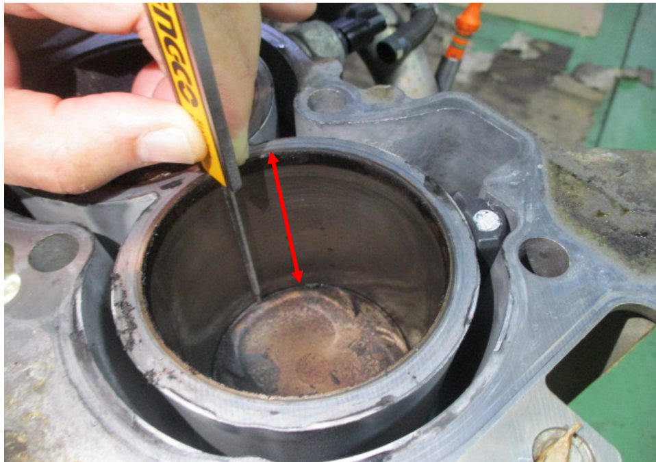
Photo 20 shows measurement being carried out to the stroke (arrowed) of cylinder 4 of the Honda engine. The bore and stroke measurements of the Honda engine were carried out using a digital Vernier Caliper that was calibrated prior to the start of measurements.
