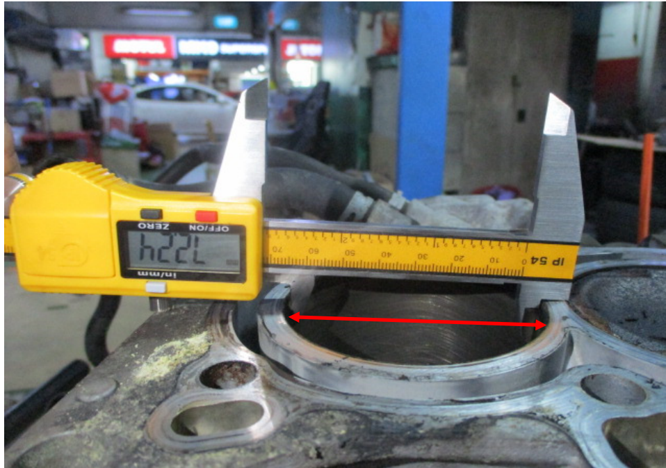
Photo 7 shows measurement being carried out to the bore (arrowed) of cylinder 1 of the Honda engine. The bore measurement of cylinder 1 was recorded to be 72.24mm.
