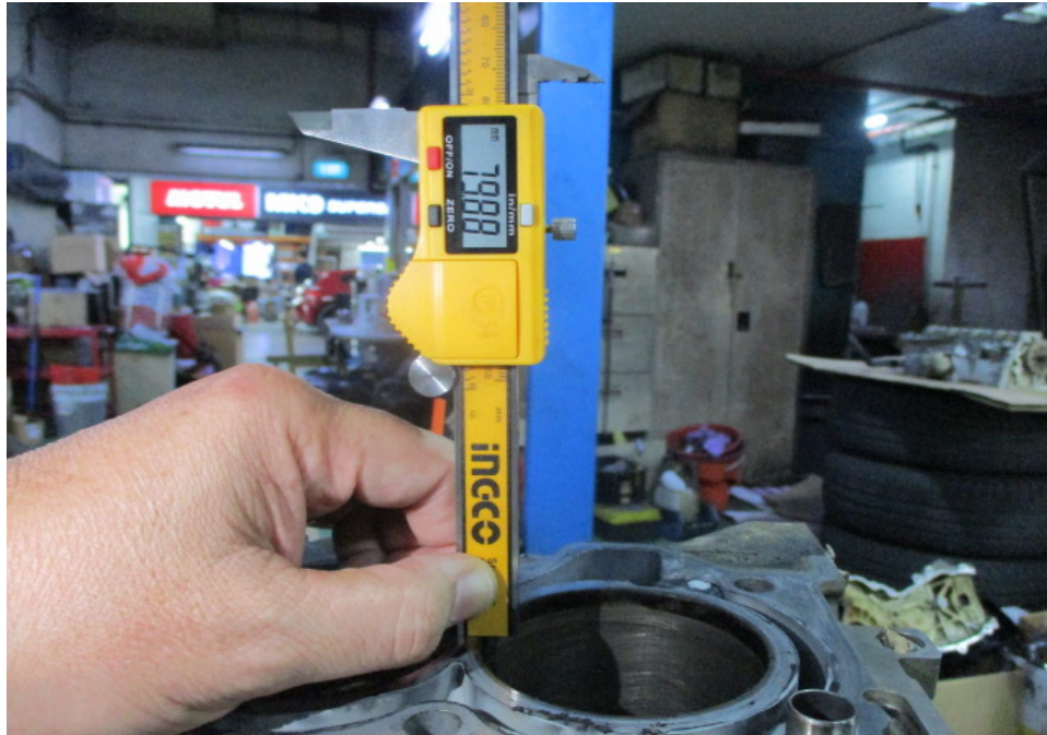
Photo 21 shows the stroke measurement of cylinder 4, which was recorded to be 79.88mm.
