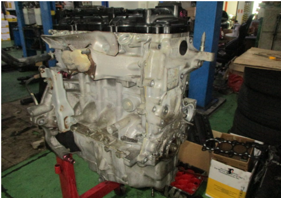
Photo 2 shows another view of the Honda engine that I had inspected. My visual examination of the engine housing revealed the housing to be of serviceable/satisfactory condition. There was no crack and/or hole observed on the engine housing.
