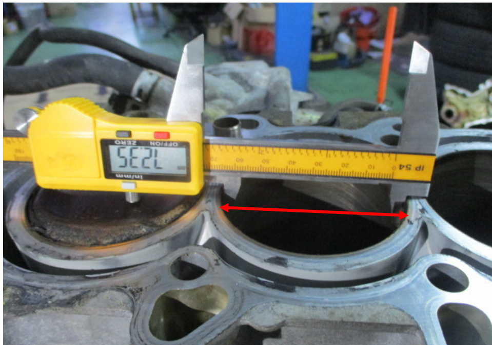
Photo 12 shows measurement being carried out to the bore (arrowed) of cylinder 2 of the Honda engine. The bore measurement of cylinder 2 was recorded to be 72.35mm.
