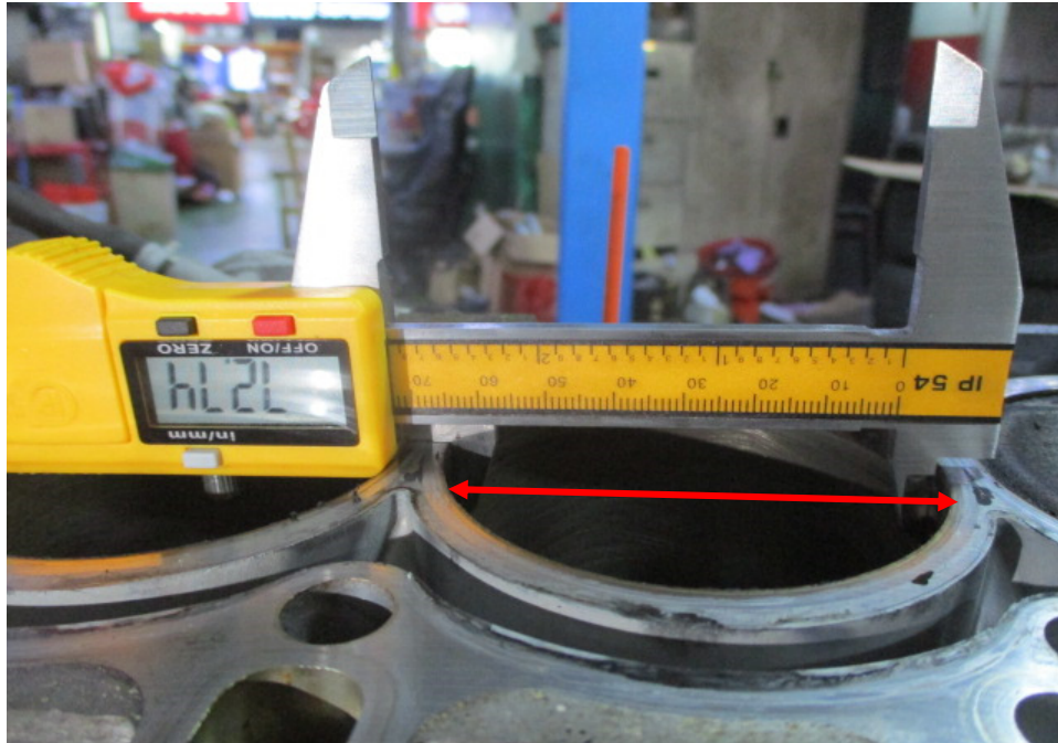
Photo 15 shows measurement being carried out to the bore (arrowed) of cylinder 3 of the Honda engine. The bore measurement of cylinder 3 was recorded to be 72.74mm.
