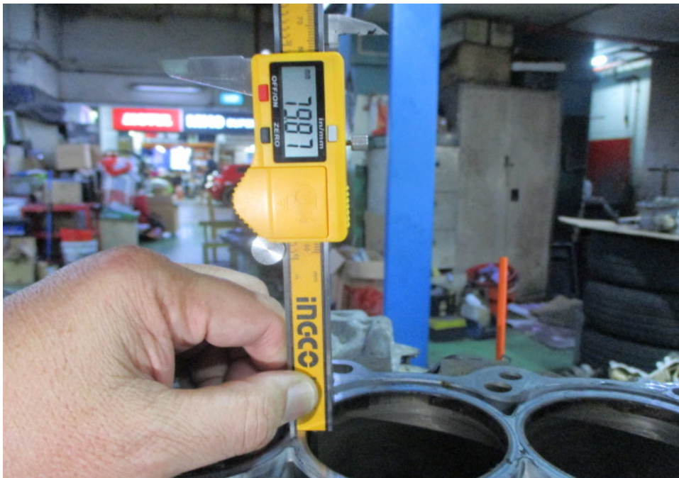
Photo 14 shows the stroke measurement of cylinder 2, which was recorded to be 79.87mm.
