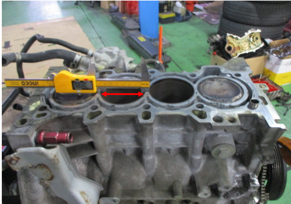
Photo 11 shows measurement being carried out to the bore (arrowed) of cylinder 2 of the Honda engine. The bore and stroke measurements of the Honda engine were carried out using a digital Vernier Caliper that was calibrated before the start of the measurements.
