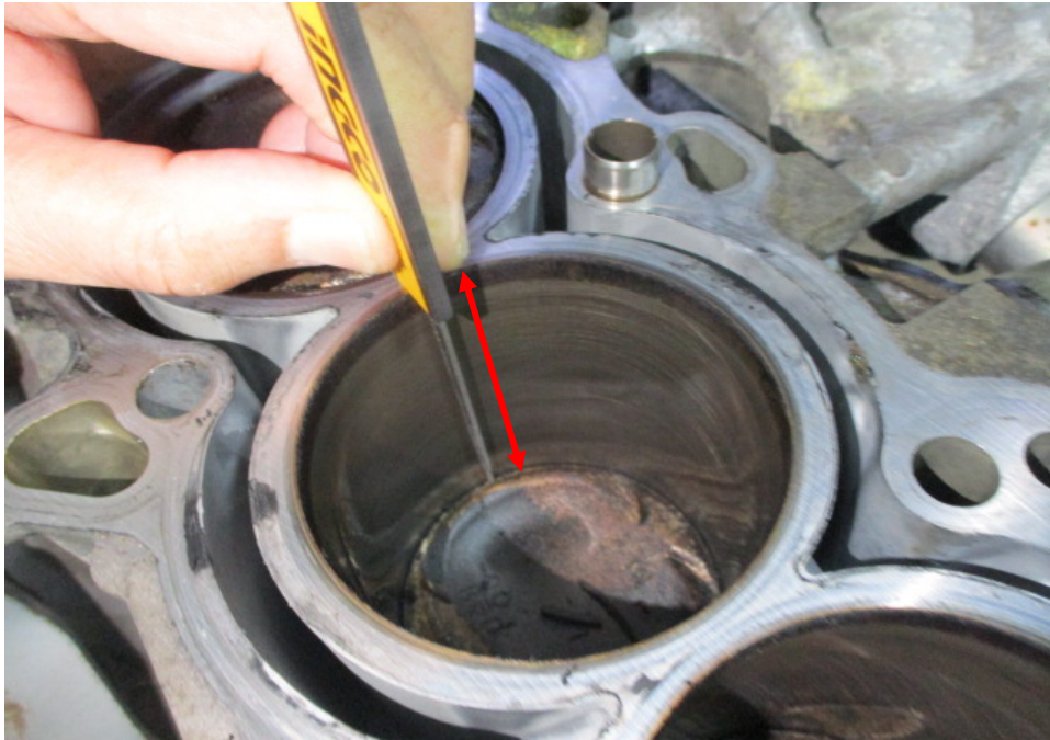
Photo 13 shows measurement being carried out to the stroke (arrowed) of cylinder 2 of the Honda engine. The bore and stroke measurements of the Honda engine were carried out using a digital Vernier Caliper that was calibrated before the start of the measurements.
