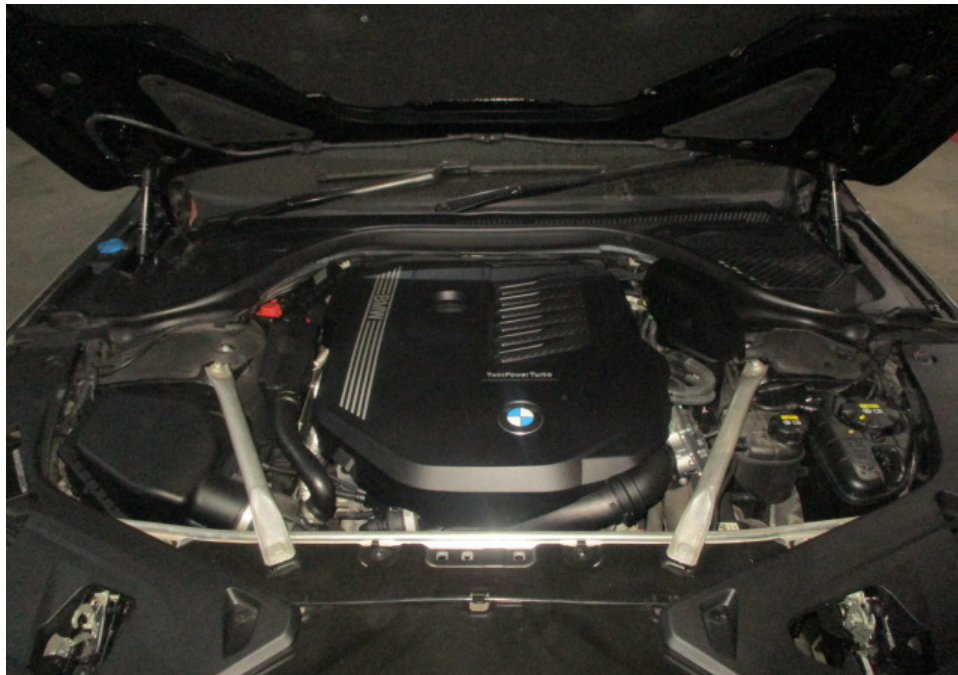
Photo 17 shows a general view of the engine compartment of the Motor Car at the time of my inspection. The various parts and components inside the engine compartment were all observed to be intact and properly fitted. There was also no sign(s) or indication(s) of fluid leak and/or fluid stain found inside the engine compartment.
