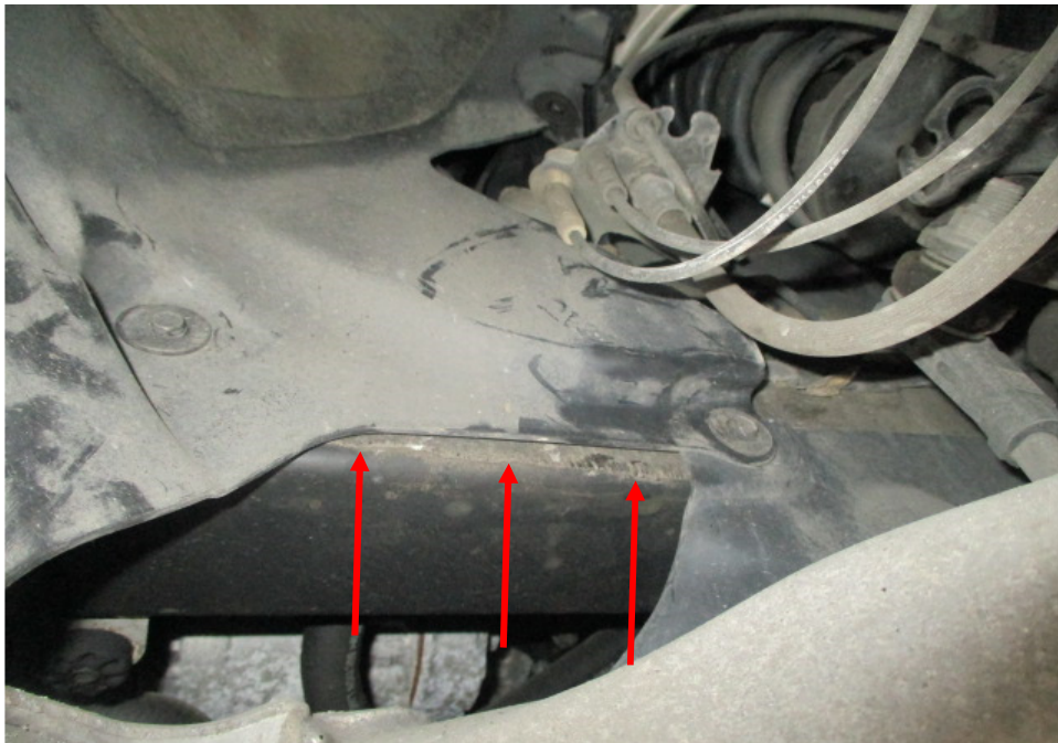
Photo 31 shows the chassis/structural body at the underside front left of the Motor Car. The original factory sealant (arrowed) at the joints along the chassis/structural body was observed to be untouched. In general, I had found no work was carried out on the chassis/structural body of the Motor Car. The chassis/structural body of the Motor Car was originally fitted.
