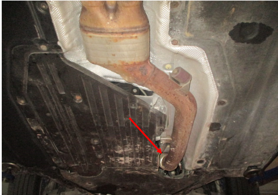
Photo 28 shows the front section of the Motor Car's exhaust system. My examination of the Motor Car's exhaust system revealed no sign(s) or indication(s) of any cut or weld marks along its exhaust pipes, on its rear muffler, on its centre resonator boxes and on its catalytic converter (arrowed).
