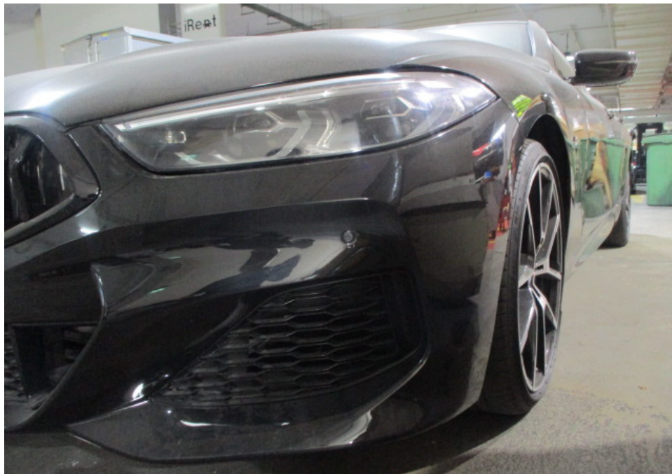
Photo 9 shows a closer view of the Motor Car's front bumper, front bumper left lower grille, front bumper left sensor and front left headlamp. The body parts at the frontal portion of the Motor Car were visually examined and it was observed that the repair/restoration works carried out to the damaged area of the Motor Car (refer to photograph 1 - 3 above) were reasonably adequate and in order.
