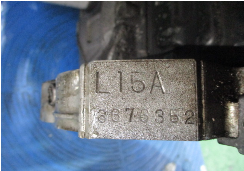
Photo 4 shows the engine number engraved on the housing of the Honda engine that I had inspected. The engine number was L15A3676352.
