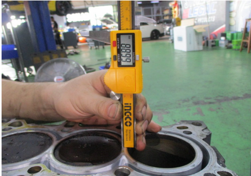
Photo 21 shows the stroke measurement of cylinder 4, which was recorded to be 88.99mm.
