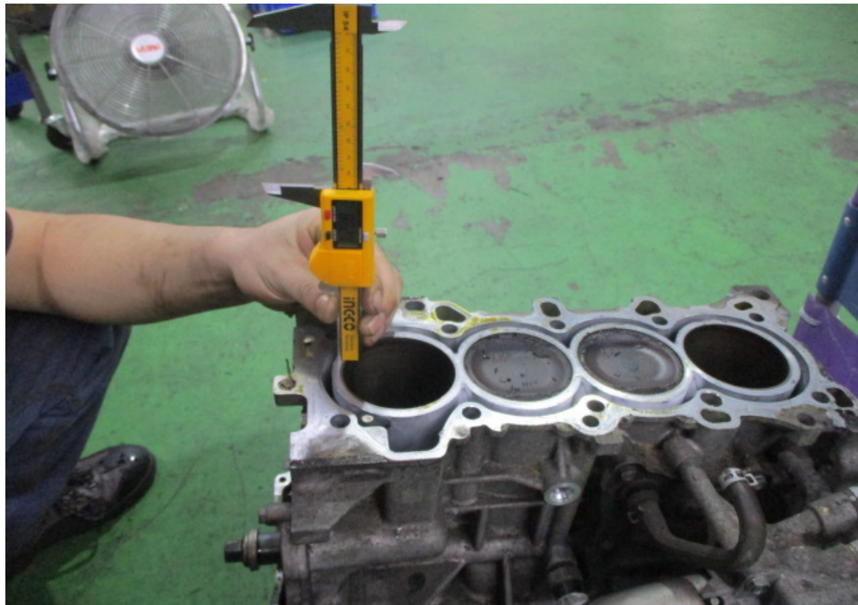
Photo 8 shows measurement being carried out to the stroke of cylinder 1 of the Honda engine. The bore and stroke measurements of the Honda engine were carried out using a digital Vernier Caliper that was calibrated before the start of the measurements.
