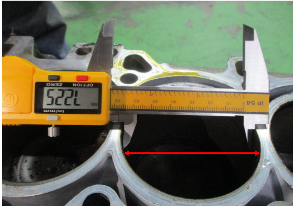
Photo 15 shows measurement being carried out to the bore (arrowed) of cylinder 3 of the Honda engine. The bore measurement of cylinder 3 was recorded to be 72.25mm.
