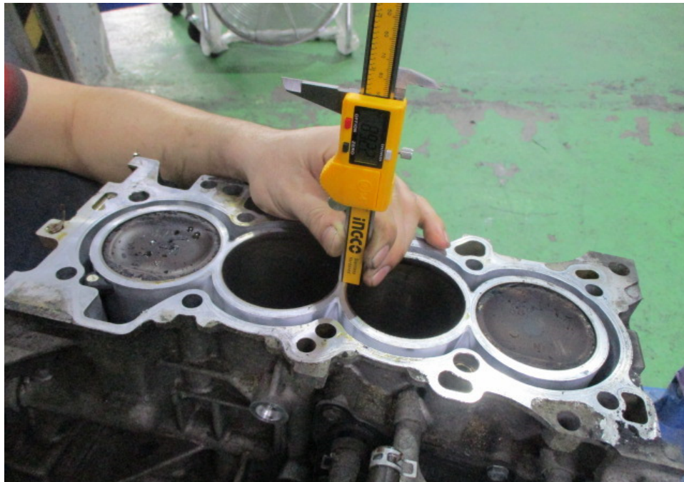
Photo 16 shows measurement of the stroke of cylinder 3 of the Honda engine that I had inspected. The bore and stroke measurements of the Honda engine were carried out using a digital Vernier Caliper that was calibrated before the start of measurements.
