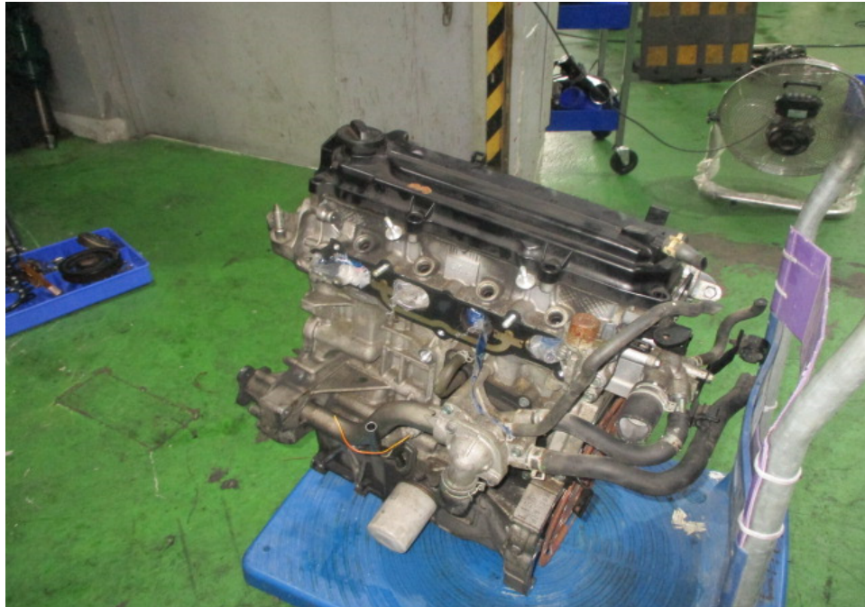
Photo 1 shows a general view of the Honda engine that I had inspected. The Honda engine was observed to be a used engine and was not fitted on any motor car. It was also observed to be a complete assembly with all mechanical parts still intact, within the engine housing.
