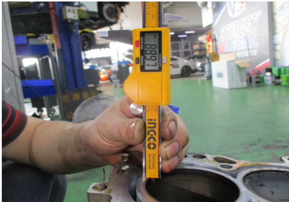
Photo 10 shows the stroke measurement of cylinder 1, which was recorded to be 88.97mm.
