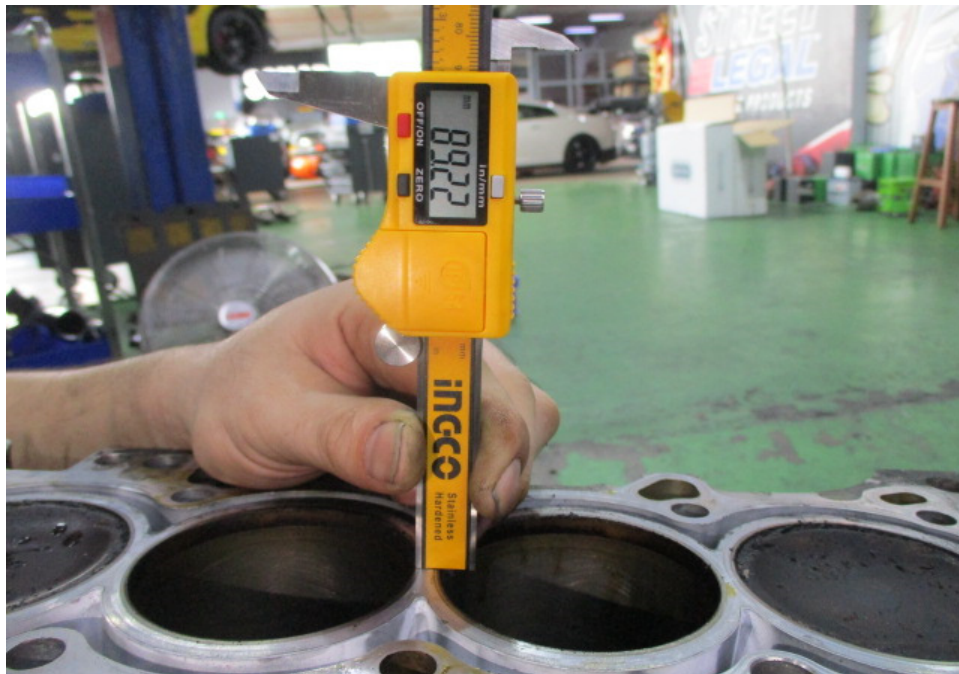
Photo 18 shows the stroke measurement of cylinder 3, which was recorded to be 89.22mm.
