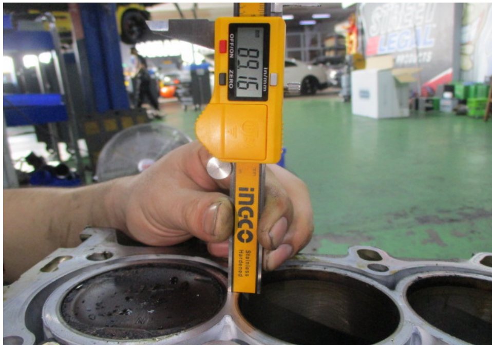
Photo 14 shows the stroke measurement of cylinder 2, which was recorded to be 89.16mm.
