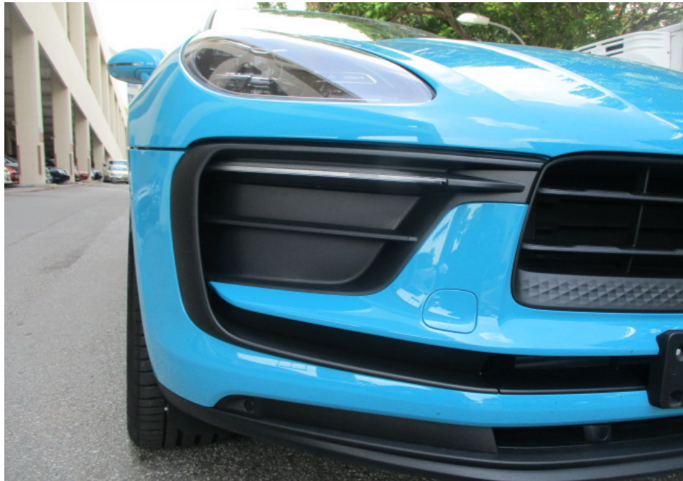
Photo 14 shows a closer view of the Motor Car's front bumper, front bumper lower cover, front bumper right lower grille, front right day light and front right headlamp. The body parts at the frontal portion of the Motor Car were visually examined and it was observed that the repair/restoration works carried out to the damaged area of the Motor Car (refer to photograph 4 & 5 above) were reasonably adequate and in order.
