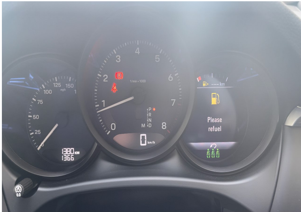
Photo 21 shows the respective warning lights no longer illuminated, indicating that there is no fault detected to the ABS, SRS, TPM and TCS systems of the Motor Car during the self-test. These electronic systems were hence in working condition at the time of my inspection.
