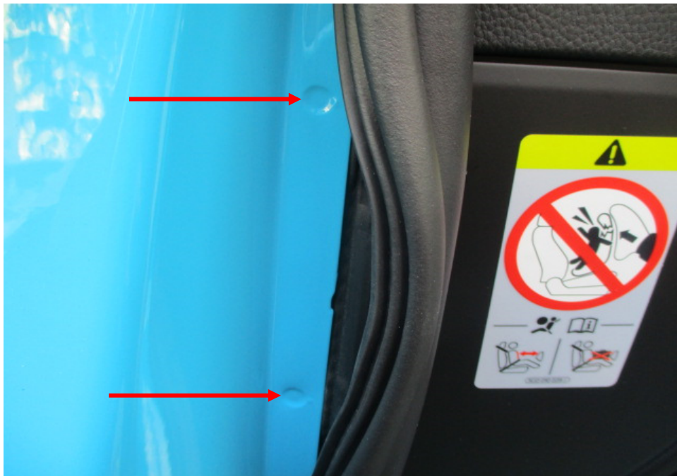
Photo 35 shows the left side "A" pillar of the Motor Car. I did not find any weld marks other than original spot weld marks (arrowed) on the left side "A" pillar of the Motor Car, which indicates that there was no re-welding works carried out. In general, I had found all the non-detachable body panels of the Motor Car to be originally fitted at the time of my inspection.
