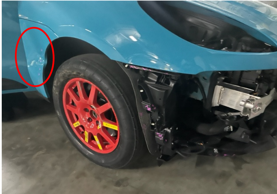
Photo 3 shows the Motor Car's damaged front right fender (circled). The Motor Car's front right wheel rim was observed to be not the original wheel rim (photograph provided to me).
