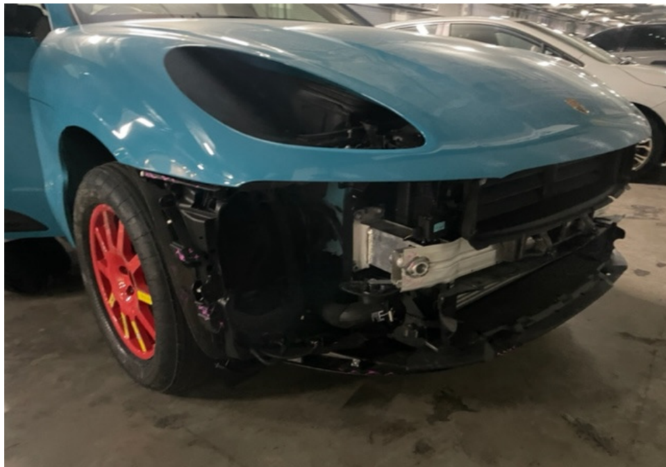
Photo 4 shows the front right body of the Motor Car (photograph provided to me). The Motor Car's front right headlamp, front grille, front bumper and all its related parts and attachments like the front bumper lower cover, front bumper right lower grille, front bumper sensors and front right day light amongst others, were observed to be missing/dislodged/damaged.
