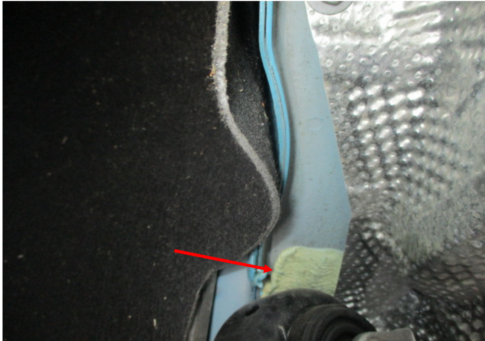
Photo 32 shows the chassis/structural body at the underside front right of the Motor Car. I did not find any weld marks other than original spot weld marks on the chassis/structural body of the Motor Car. The original factory sealant (arrowed) at the joints along the chassis/structural body was untouched, indicating no work was done on the chassis/structural body of the Motor Car and that the chassis/structural body was originally fitted.
