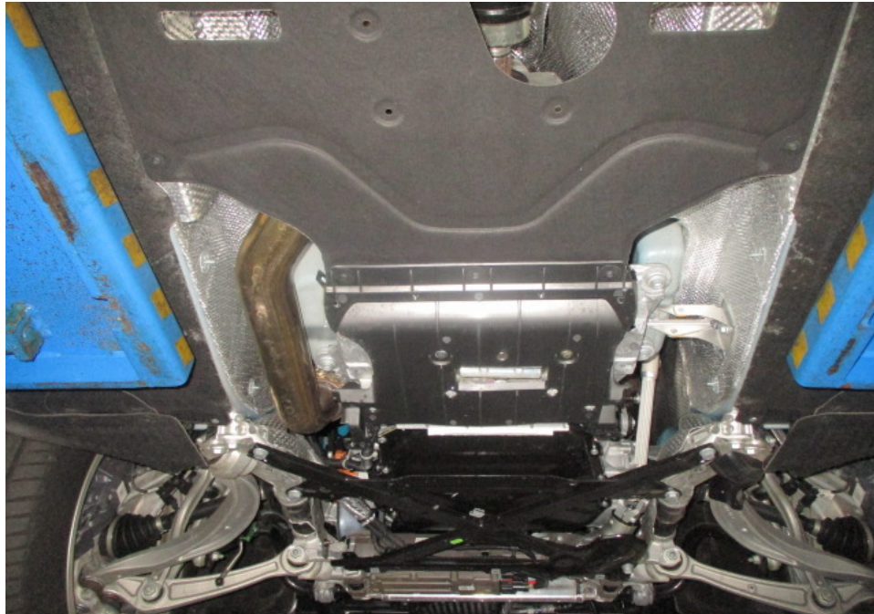
Photo 28 shows the front section of the Motor Car's exhaust system. My examination of the Motor Car's exhaust system revealed no sign(s) or indication(s) of any cut or weld marks along its exhaust pipes, on its rear mufflers, and on its catalytic converter.
