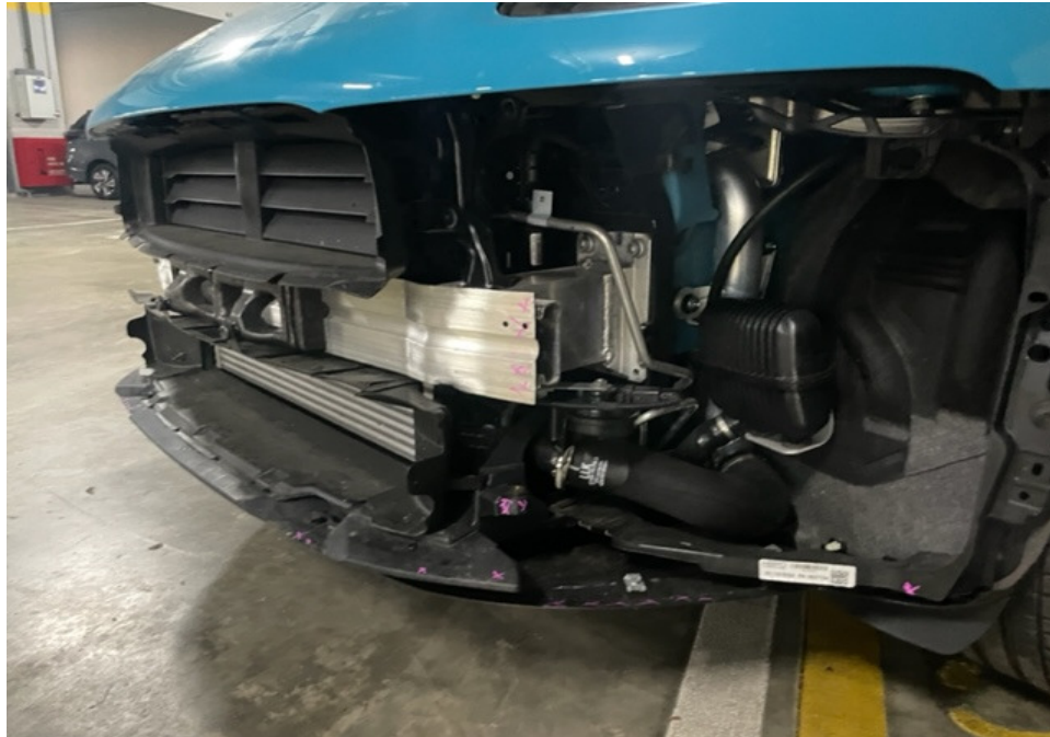
Photo 5 shows another view of the Motor Car's front bumper and all its related parts and attachments like the front bumper lower cover, front bumper left lower grille, front bumper sensors and front left day light amongst other, missing/dislodged/damaged. (photograph provided to me).
