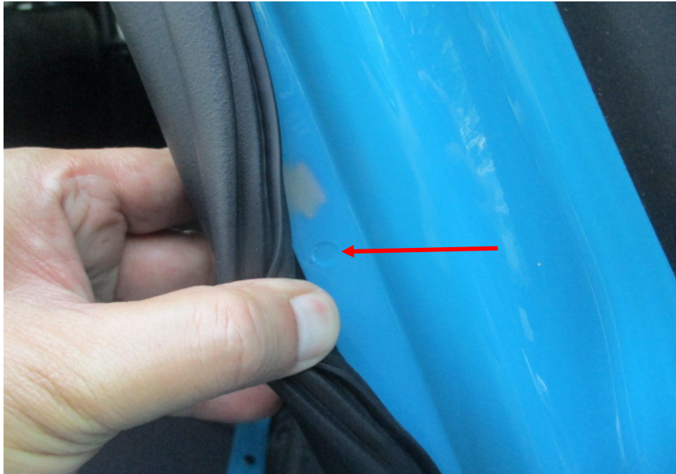
Photo 36 shows the left side “C” pillar of the Motor Car. I did not find any weld marks other than original spot weld marks (arrowed) on the left side “C” pillar of the Motor Car, which indicates that there was no re-welding works carried out. In general, I had found all the non-detachable body panels of the Motor Car to be originally fitted at the time of my inspection.
