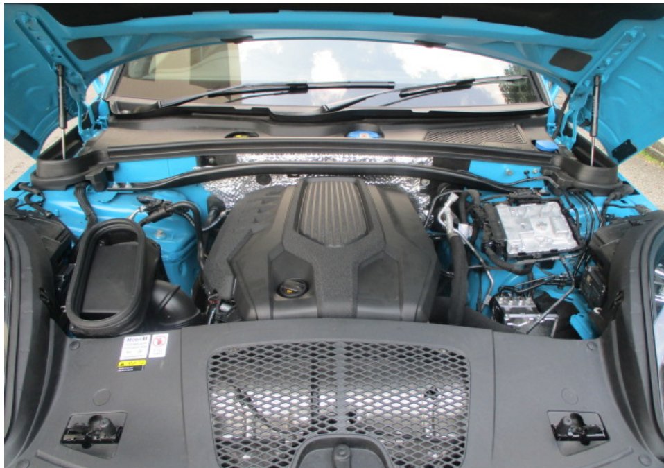
Photo 17 shows a general view of the Motor Car's engine compartment at the time of my inspection. The various parts and components inside the engine compartment were all observed to be intact and properly fitted. There was also no sign(s) or indication(s) of fluid leak and/or fluid stain found inside the engine compartment.
