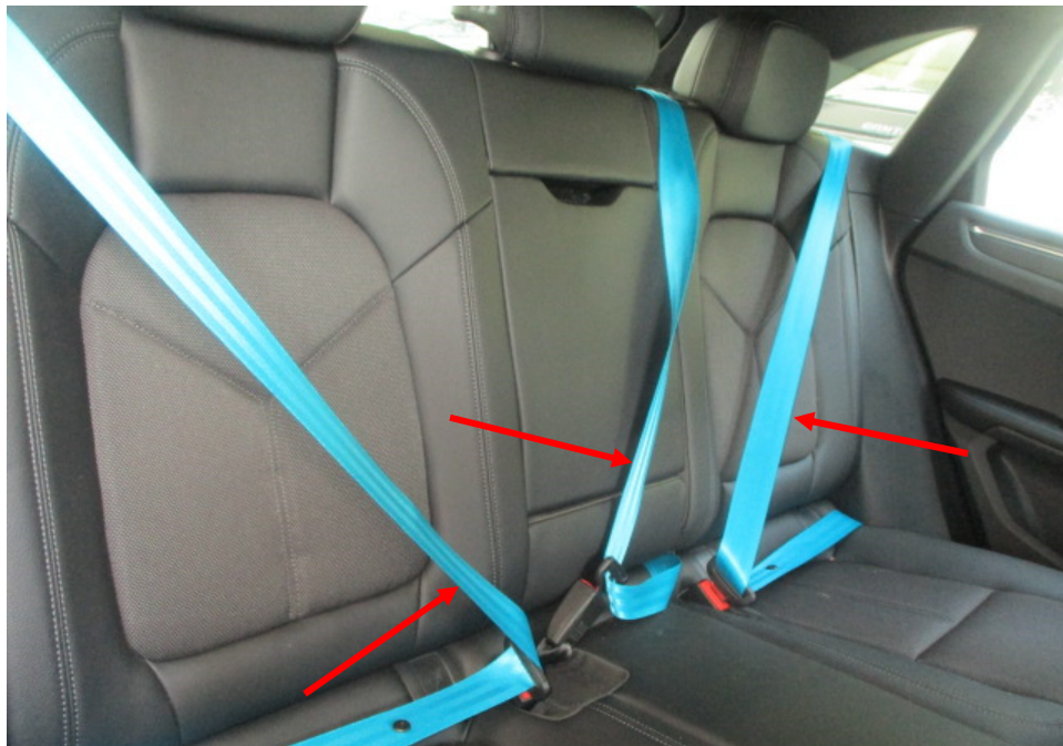
Photo 19 shows the rear seats of the Motor Car. All the seats of the Motor Car were secured via seat rails to the floorboard. They were also fitted with a retractable seat belt reel and a pre-tensioner. The seat belts (arrowed) were tested and were able to be fastened into the respective pre-tensions that were fitted on the side of each individual seat.
