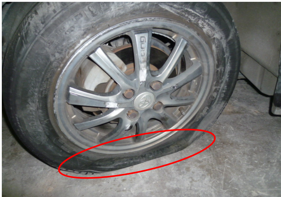
Photo 10 shows the left front tyre of the Insured Vehicle at the time of our inspection. We had observed that the left front tyre was deflated as a result of the accident (circled).
