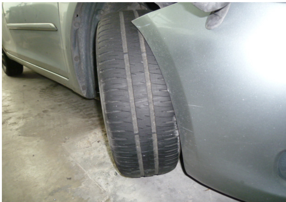
Photo 6 shows the right front tyre of the Insured Vehicle at the time of our inspection. The right front tyre of the Insured Vehicle was observed to be in serviceable condition. The pattern of the tread was generally still visible. The remaining tread depth was measured to be approximately 3mm.
