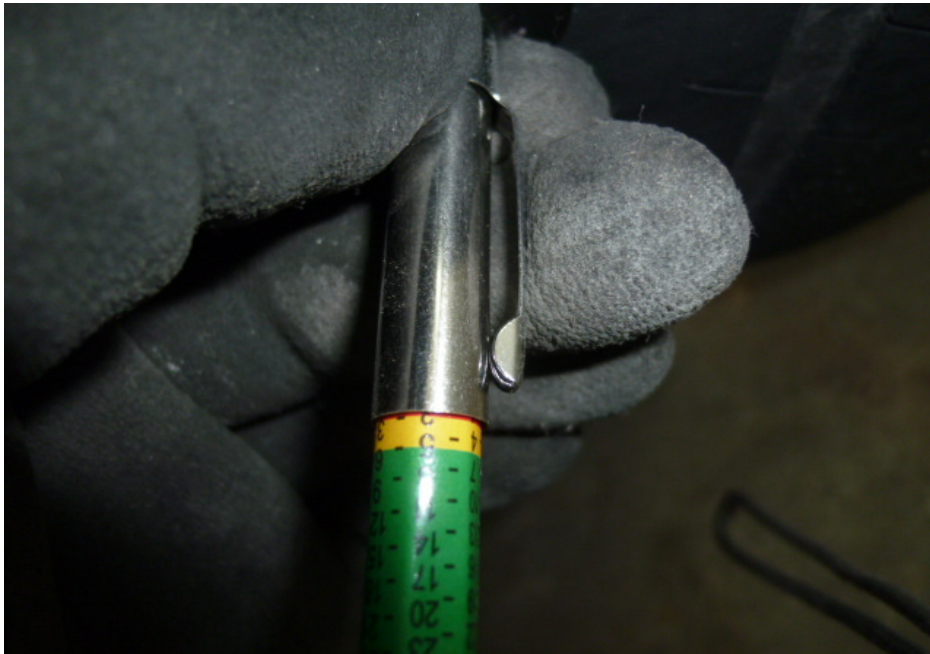
Photo 14 shows measurements being conducted on the remaining tread depth of the left front tyre of the Insured Vehicle. The remaining tread depth at the outer side of the left front tyre was measured to be approximately 2mm.
