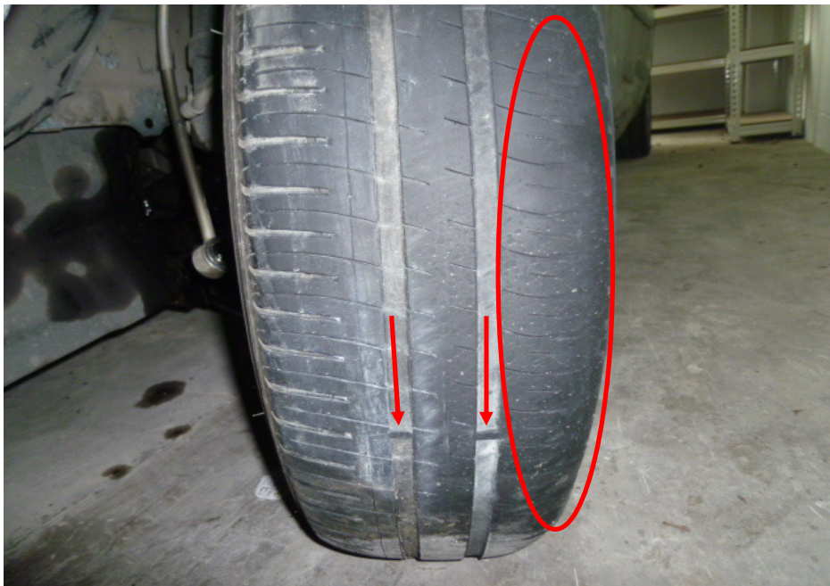
Photo 12 shows a closer view of the left front tyre of the Insured Vehicle at the time of our inspection. The rubber at the outer side of the tread (circled) was partially worn. However the pattern of the tread was generally still visible. The
