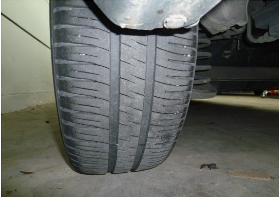
Photo 4 shows the left rear tyre of the Insured Vehicle at the time of our inspection. The left rear tyre of the Insured Vehicle was observed to be in serviceable condition. The pattern of the tread was generally still visible. The remaining tread depth was measured to be approximately 4mm.
