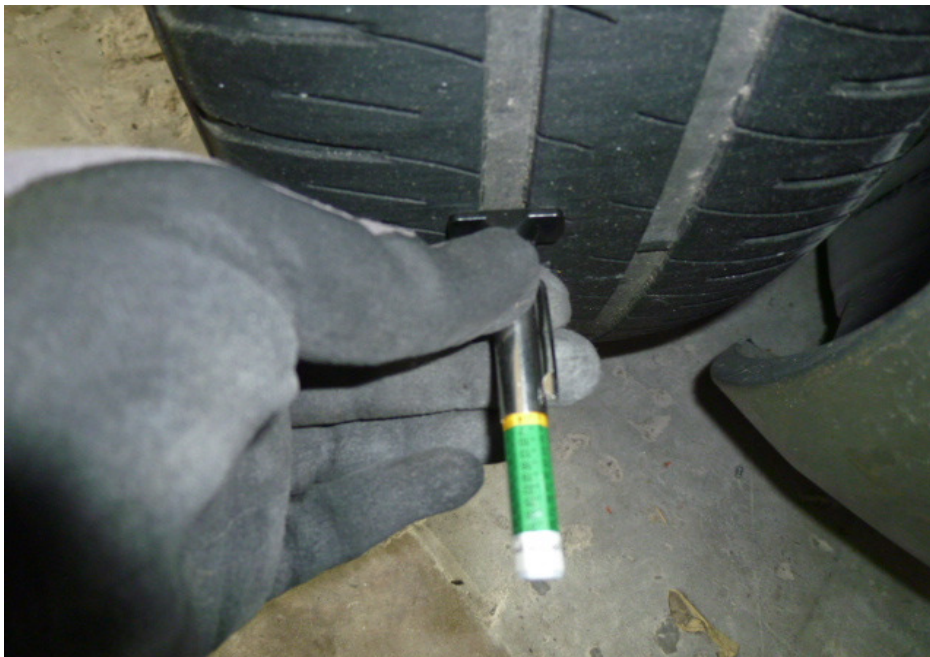
Photo 8 shows measurements being conducted on the remaining tread depth of the front right tyre of the Insured Vehicle. The remaining tread depth was measured to be approximately 3mm.
