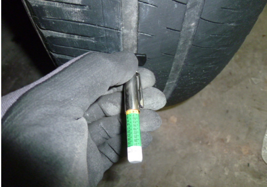
Photo 13 shows measurements being conducted on the remaining tread depth of the left front tyre of the Insured Vehicle. The remaining tread depth was measured to be approximately 2mm.
