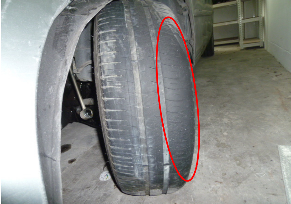
Photo 11 shows the left front tyre of the Insured Vehicle at the time of our inspection. The rubber at the outer side of the tread (circled) was partially worn. The pattern at some areas on the outer side of the tread was vaguely visible due to worn rubber however the reinforcing belts that are found within the tyre were not exposed at the time of our inspection.
