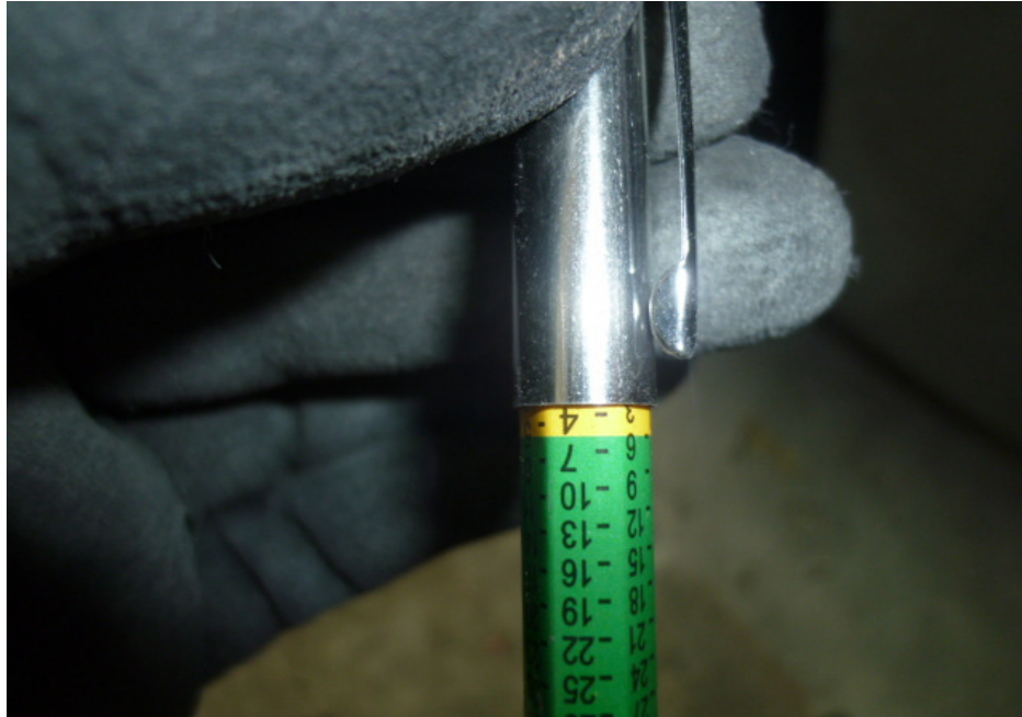
Photo 9 shows measurements being conducted on the remaining tread depth of the right front tyre of the Insured Vehicle. The remaining tread depth was measured to be approximately 3mm.
