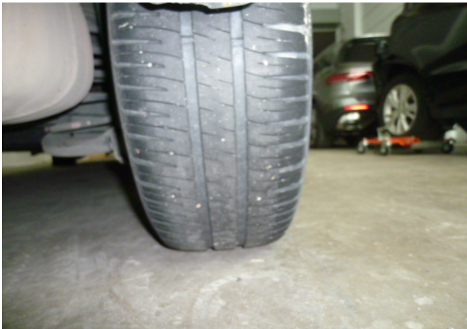
Photo 5 shows the right rear tyre of the Insured Vehicle at the time of our inspection. The right rear tyre of the Insured Vehicle was observed to be in serviceable condition. The pattern of the tread was generally still visible. The remaining tread depth was measured to be approximately 4mm.
