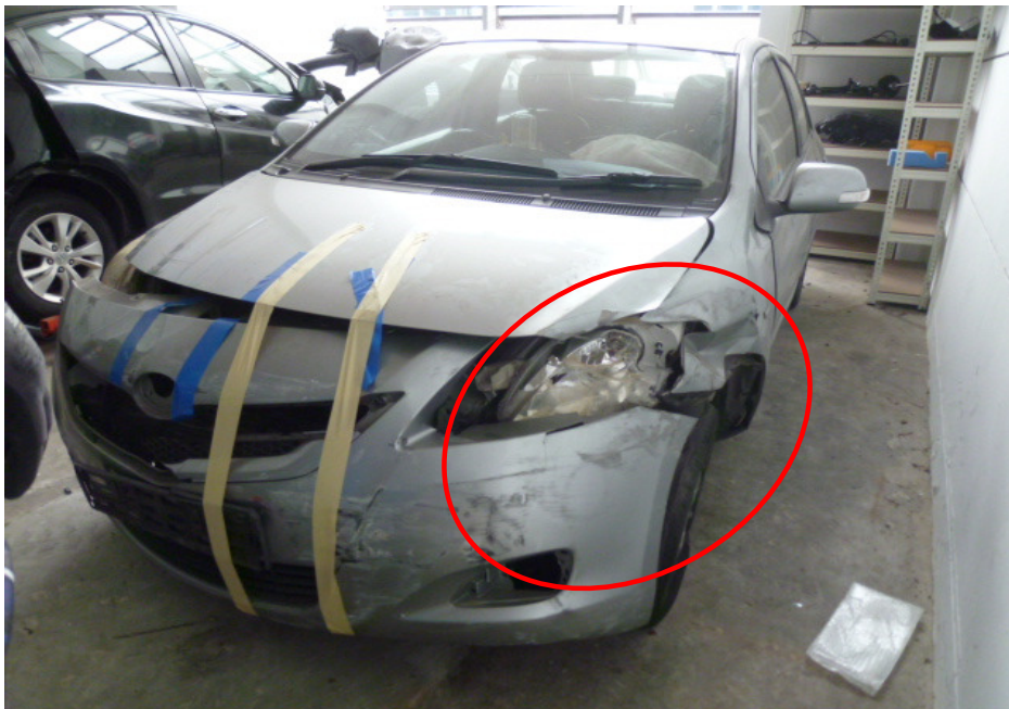
Photo 3 shows the general view of the left front portion of the Insured Vehicle at the time of our inspection. The Insured Vehicle was observed to have sustained impact damage that was confined to its left frontal portion. Its front bumper, front bonnet, front windscreen, left front fender, left headlamp, left front wheel rim and left front tyre were amongst the exterior body parts that were observed to have been damaged as a result of the accident.
