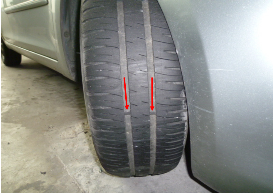
Photo 7 shows a closer view of the right front tyre of the Insured Vehicle at the time of our inspection. The pattern of the tread was generally still visible. The tyre wear indicators (arrowed), normally built into the groove of the tread pattern, were also observed to be not flushed with the tread pattern.
