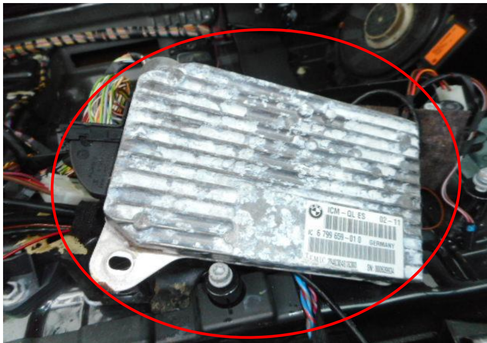
Photo 30 shows a close up view of the Motor Car's electrical Chassis control module component (circled) located at the bottom of the centre console. We have observed mould and rust built up on the electrical component due to damage by direct water intrusion into the interior cabin of the Motor Car.
