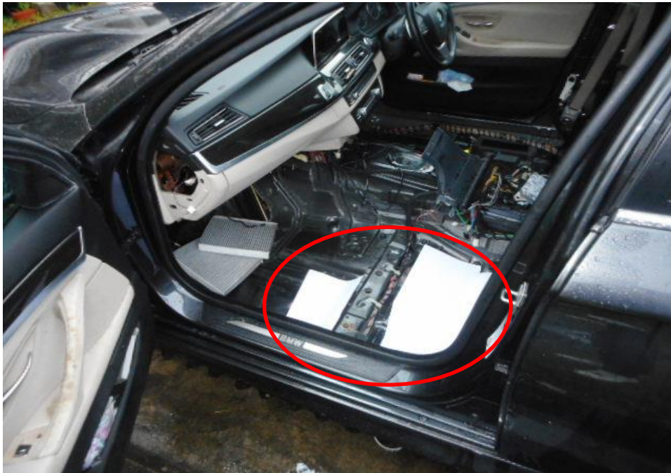
Photo 32 shows dry papers (red circle) that was placed into the floor of the interior cabin where the seats and electrical components was at and before water was poured onto the exterior door seals of the Motor Car to see if there was any water intrusion into the Motor Car
