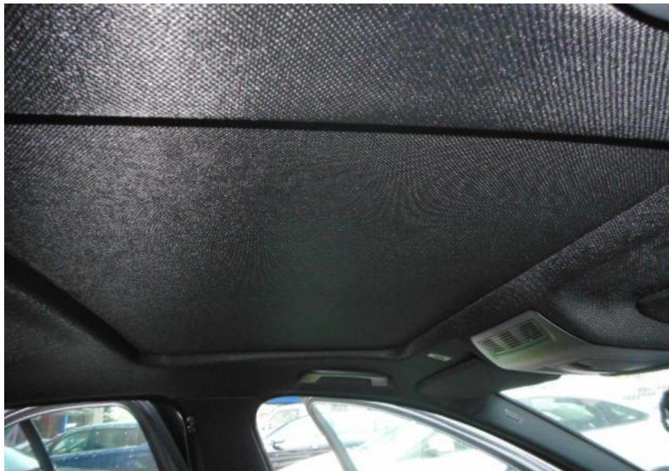
Photo 31 shows a general up view of the Motor Car's interior cabin roof material located at the top of the interior. We have observed no water intrusion damages to the interior cabin roof material of the Motor Car at the time of inspection and also after the water leak test.
