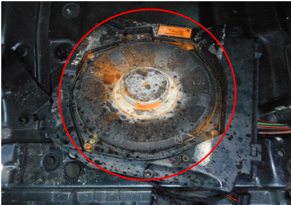
Photo 28 shows a close up view of the Motor Car's electrical audio subwoofer component (circled) located at the bottom of the front left seat. We have observed rust built up on its electrical component due to damage by direct water intrusion into the interior cabin of the Motor Car.
