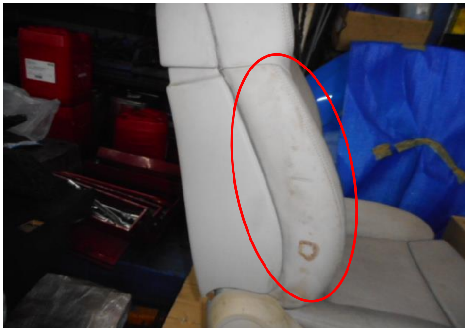
Photo 22 shows a close up view of the Motor Car's front right seat. We have observed mouldy stains on its front right seat (circled) due to indirect water intrusion into the interior cabin of the Motor Car.
