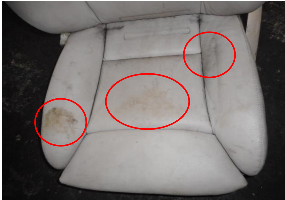
Photo 16 shows a close up view of the Motor Car's front left seat. We have observed mouldy stains on its front left seat (circled) due to indirect water intrusion into the interior cabin of the Motor Car.
