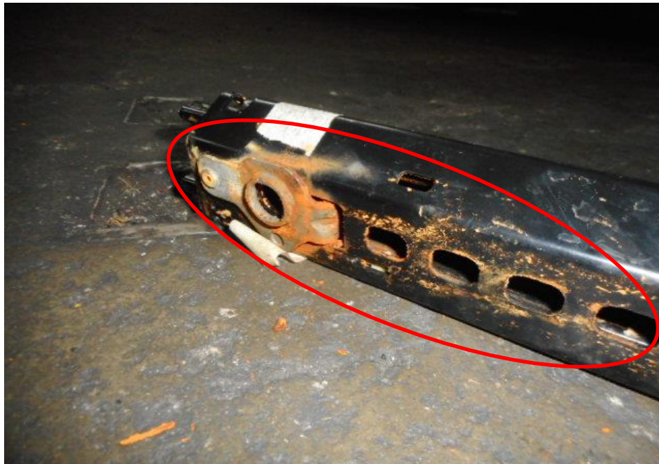
Photo 19 shows a close up view of the Motor Car's front left seat mechanism. We have observed rust built up on its front left seat mechanism due to damage by direct water intrusion into the interior cabin of the Motor Car.
