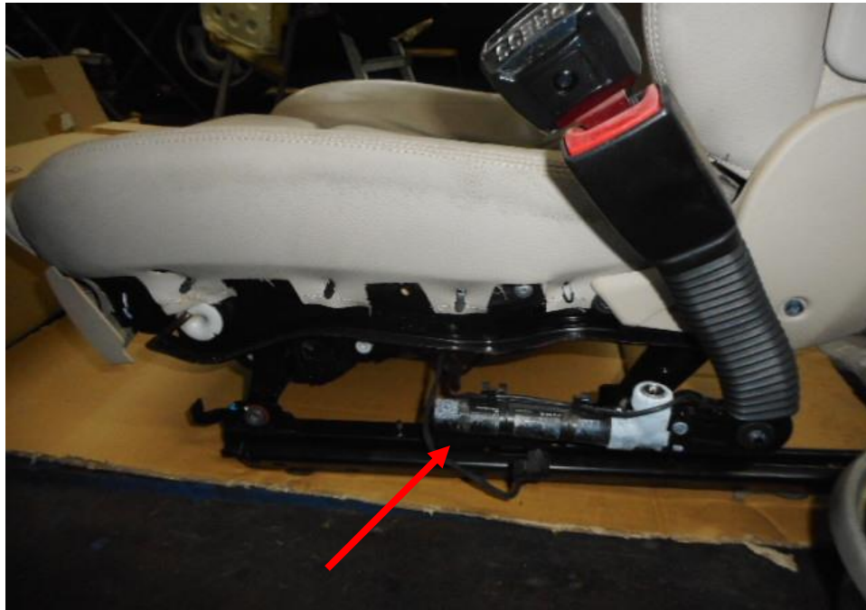
Photo 23 shows a general up view of the Motor Car's front right seat rail mechanism. We have observed that its front right seat mechanism (arrowed) did not sustain any damage by any water intrusion into the interior cabin of the Motor Car.
