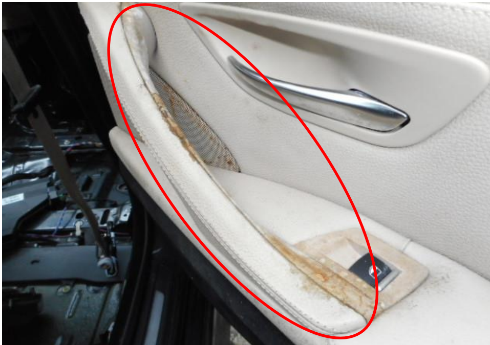
Photo 14 shows a close up view of the Motor Car's rear right door handle. We have observed mouldy stains on its rear right door handle (circled) due to indirect water intrusion into the interior cabin of the Motor Car.
