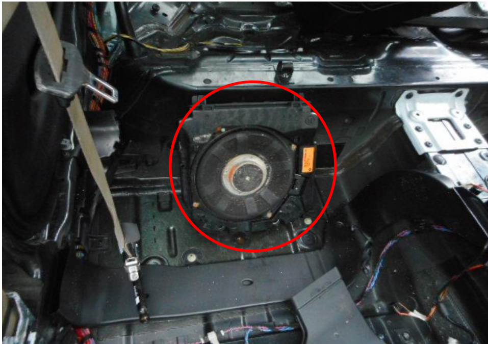
Photo 25 shows a general up view of the Motor Car's electrical audio subwoofer component (circled) located at the bottom of the front right seat. We have observed rust built up on its electrical component due to damage by direct water intrusion into the interior cabin of the Motor Car.
