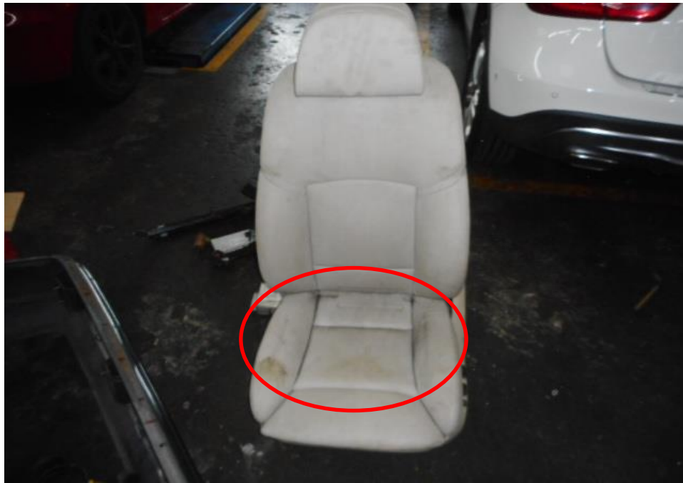
Photo 15 shows a general up view of the Motor Car's front left seat. We have observed mouldy stains on its front left seat (circled) due to indirect water intrusion into the interior cabin of the Motor Car.
