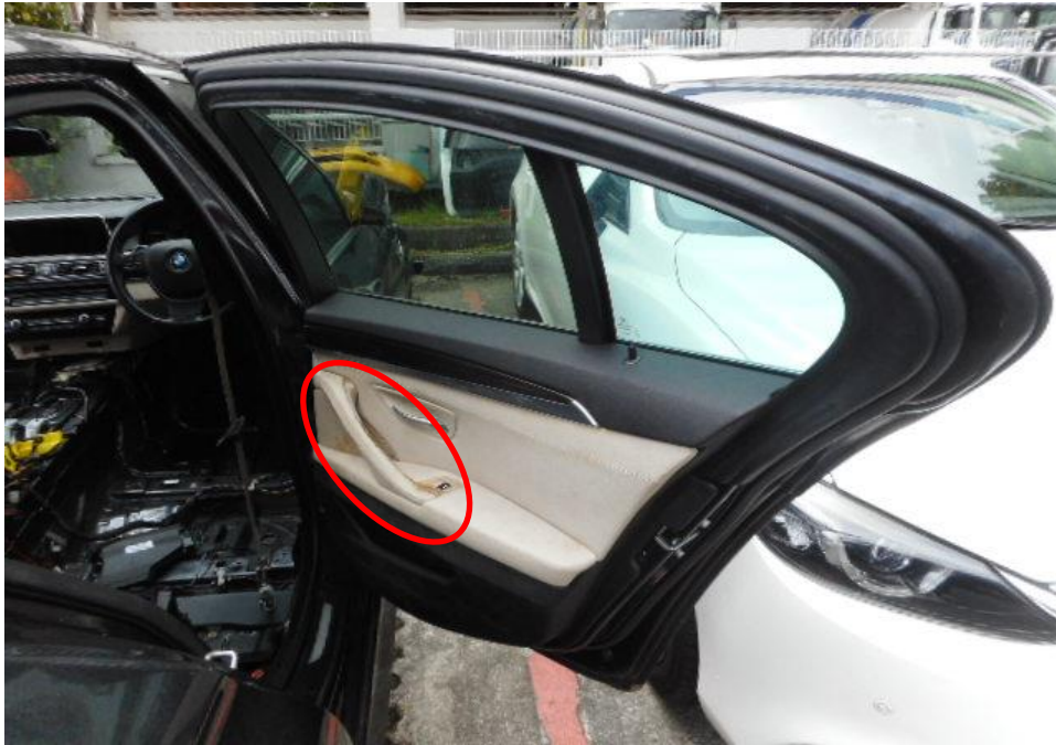
Photo 13 shows a general up view of the Motor Car's rear right door handle. We have observed mouldy stains on its rear right door handle (circled) due to indirect water intrusion into the interior cabin of the Motor Car.
