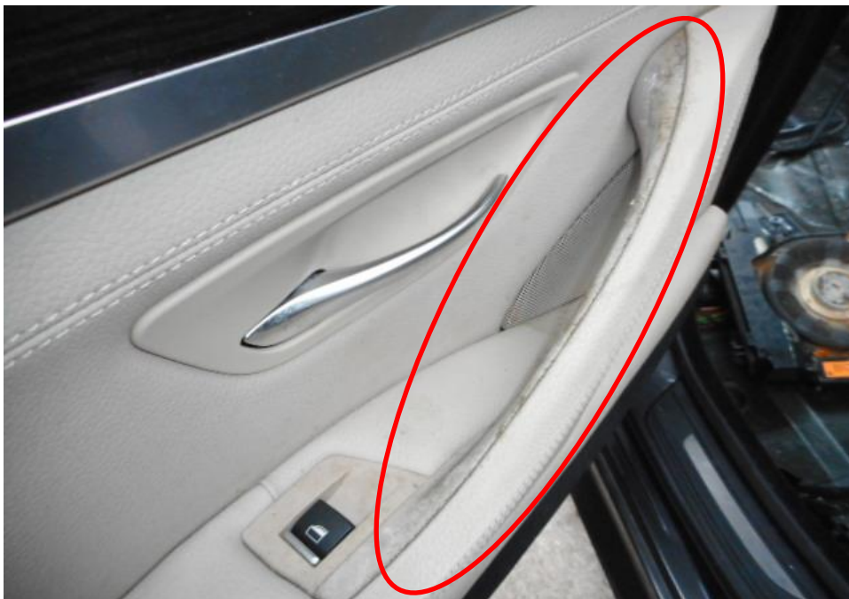
Photo 12 shows a close up view of the Motor Car's rear left door handle. We have observed mouldy stains on its rear left door handle (circled) due to indirect water intrusion into the interior cabin of the Motor Car.
