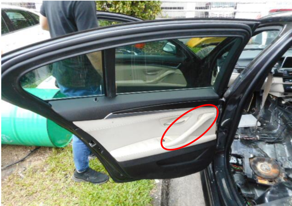
Photo 11 shows a general up view of the Motor Car's rear left door handle. We have observed mouldy stains on its rear left door handle (circled) due to indirect water intrusion into the interior cabin of the Motor Car.
