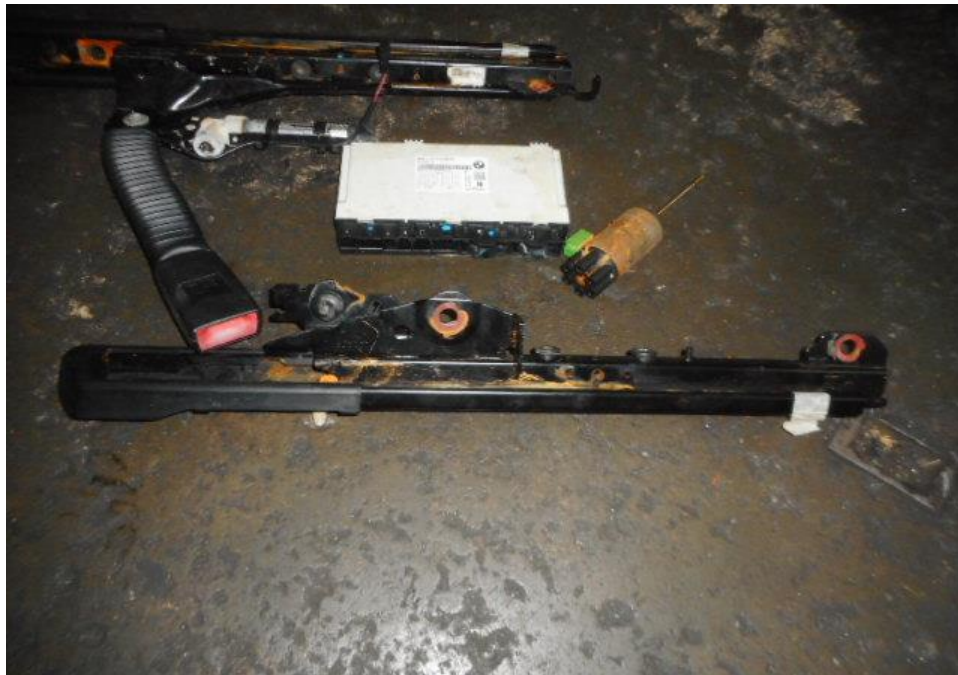
Photo 17 shows a general up view of the Motor Car's front left seat rail mechanism. We have observed rust built up on its front left seat mechanism due to damage by direct water intrusion into the interior cabin of the Motor Car.
