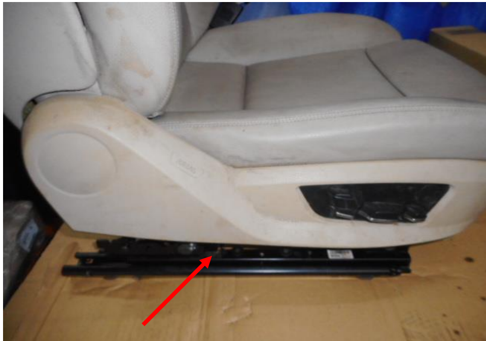
Photo 24 shows a general up view of the Motor Car's front right seat rail mechanism. We have observed that its front right seat mechanism did not sustain any damage by any water intrusion into the interior cabin of the Motor Car.
