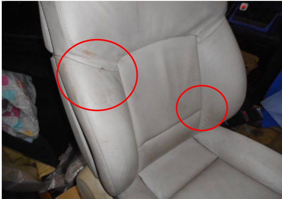
Photo 21 shows a close up view of the Motor Car's front right seat. We have observed mouldy stains on its front right seat (circled) due to indirect water intrusion into the interior cabin of the Motor Car.
