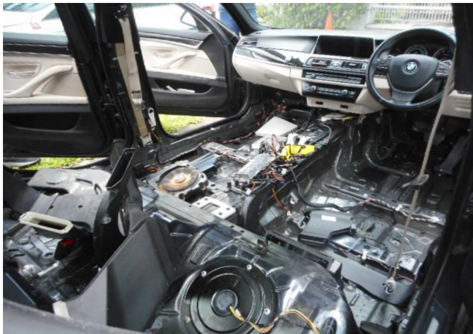
Photo 6 shows a general view of the Motor Car's interior portion at the time of our inspection. The Motor Car was observed to have sustained direct and indirect water intrusion damages in its interior cabin. At the time of our inspection shows that its front left and right seat, interior door handles, left seat rail mechanism and its electrical components were amongst the body parts that had sustained water intrusion damages.
