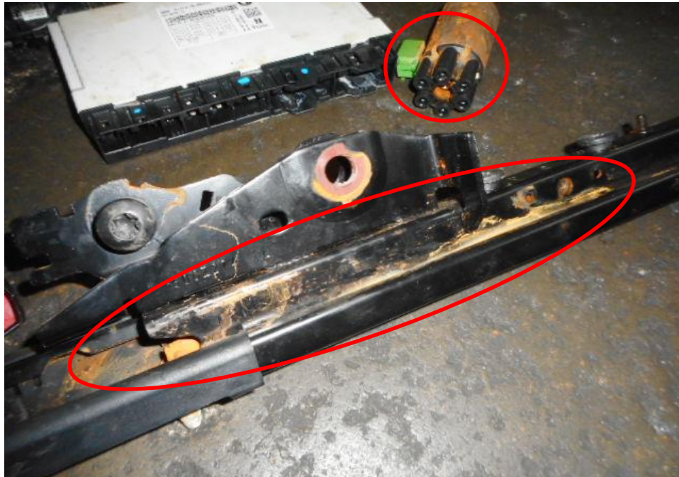
Photo 18 shows a close up view of the Motor Car's front left seat mechanism. We have observed rust built up on its front left seat mechanism due to damage by direct water intrusion into the interior cabin of the Motor Car.
