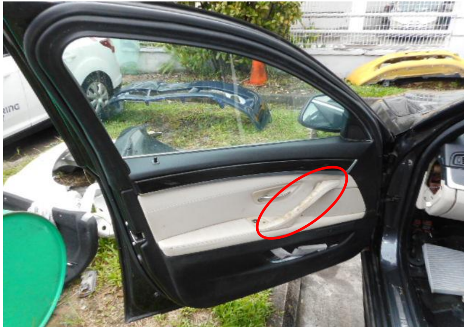
Photo 7 shows a general up view of the Motor Car's front left door handle. We have observed mouldy stains on its front left door handle (circled) due to indirect water intrusion into the interior cabin of the Motor Car.
