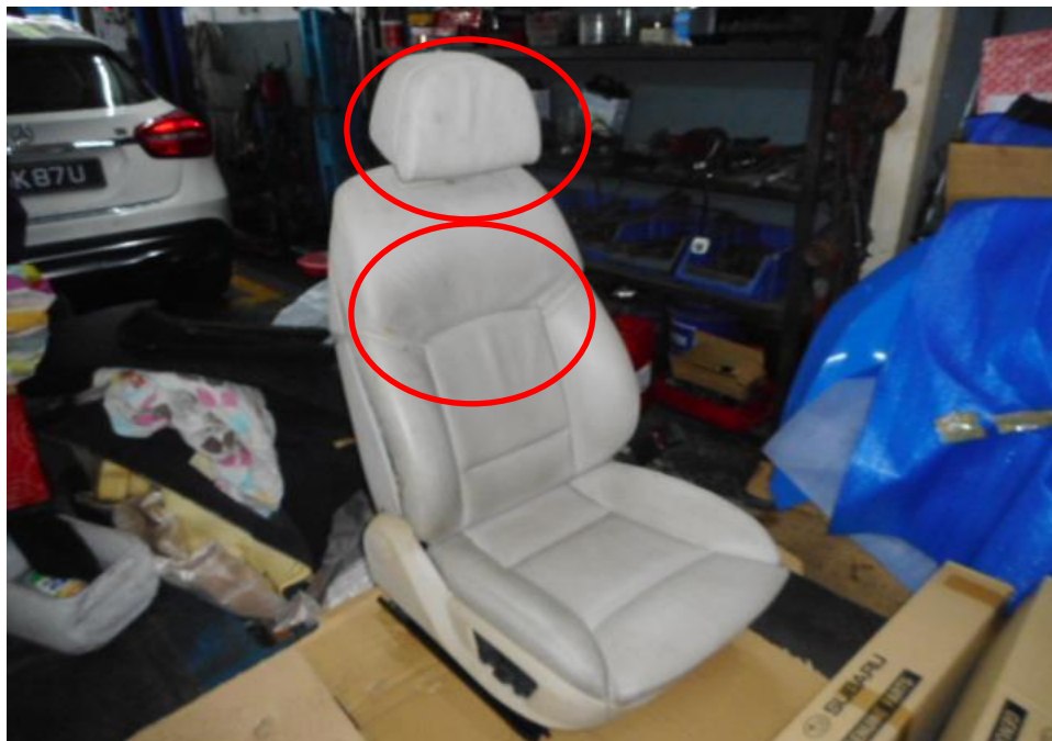
Photo 20 shows a general up view of the Motor Car's front right seat. We have observed mouldy stains on its front right seat (circled) due to indirect water intrusion into the interior cabin of the Motor Car.
