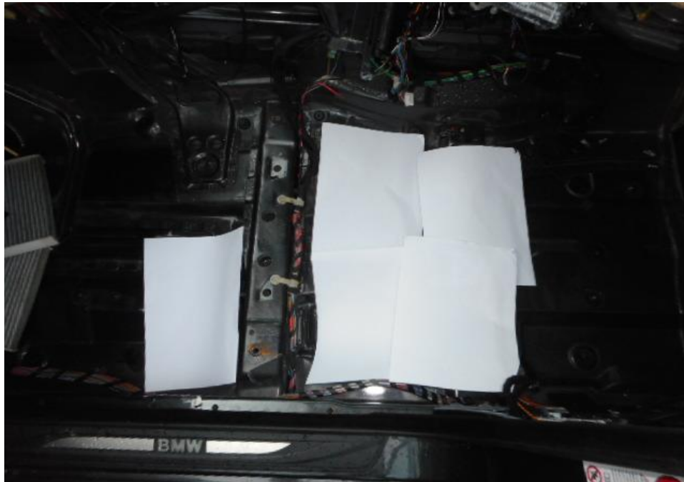
Photo 34 shows dry papers (red circle) that was placed into the floor of the interior cabin where the seats and electrical components was at and after water was poured onto the exterior door seals of the Motor Car and the papers remained dry and there was no water intrusion into the Motor Car
