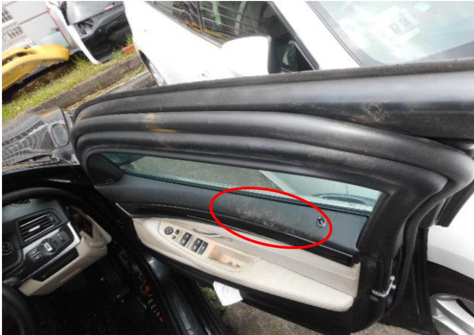
Photo 9 shows a general up view of the Motor Car's front right door panel. We have observed mouldy stains on its front right door panel (circled) due to indirect water intrusion into the interior cabin of the Motor Car.
