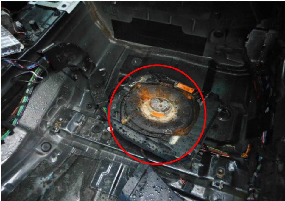
Photo 27 shows a general up view of the Motor Car's electrical audio subwoofer component (circled) located at the bottom of the front left seat. We have observed rust built up on its electrical component due to damage by direct water intrusion into the interior cabin of the Motor Car.
