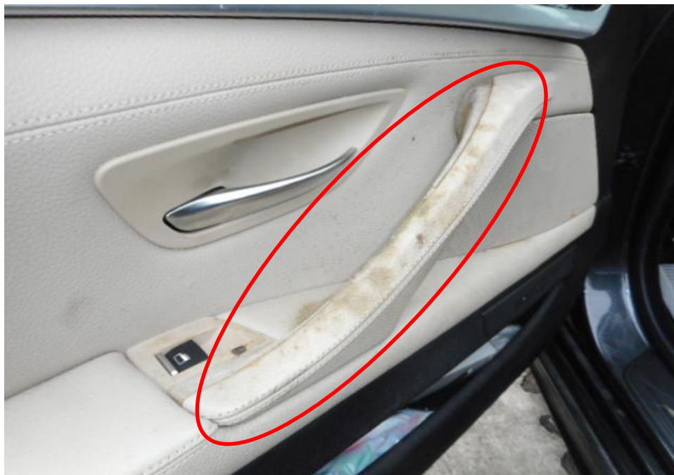
Photo 8 shows a close up view of the Motor Car's front left door handle. We have observed mouldy stains on its front left door handle (circled) due to indirect water intrusion into the interior cabin of the Motor Car.
