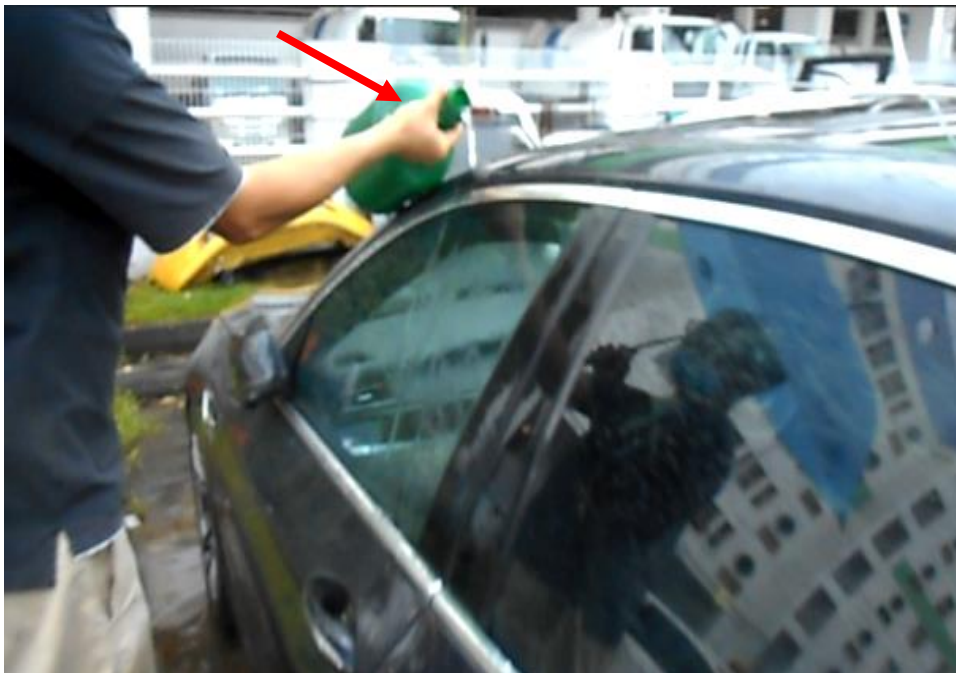
Photo 33 shows water leak test where (arrowed) water was poured onto the exterior door seals of the Motor Car to see if there was any water intrusion into the Motor Car
