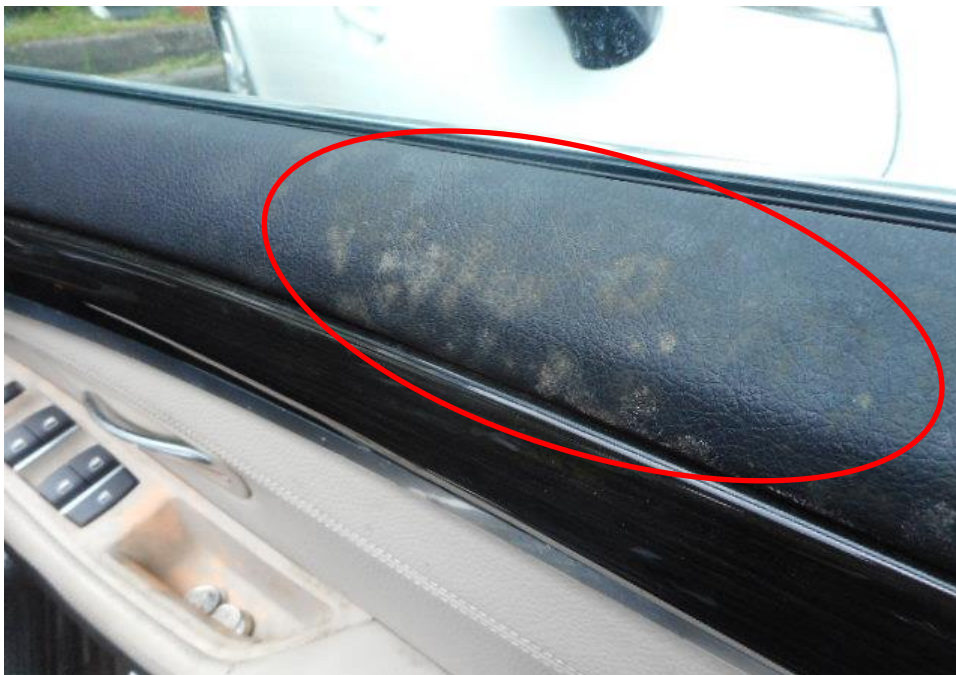
Photo 10 shows a close up view of the Motor Car's front right door panel. We have observed mouldy stains on its front right door panel (circled) due to indirect water intrusion into the interior cabin of the Motor Car.
