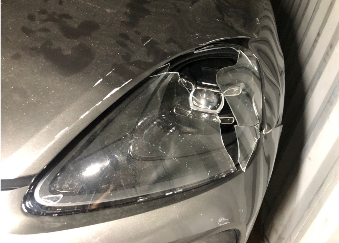
Photo 5 shows the left side front body of the Motor Car (photograph provided to me). Apart for the right side portion, I had also observed damage at the left side front portion of the Motor Car. Body parts damaged include the front left headlamp and front left fender amongst others.
