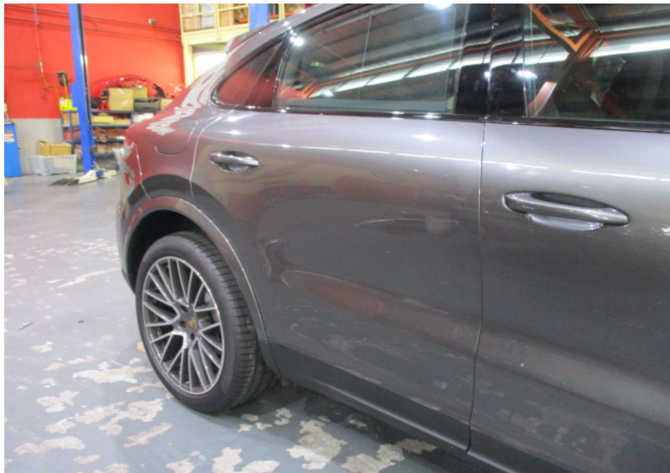
Photo 10 shows a closer view of the Motor Car's front right door, rear right door and rear right fender wheel arc garnish. The body parts at the right side portion of the Motor Car were visually examined and it was observed that the repair/restoration works carried out to the damaged area of the Motor Car (refer to photograph 2 & 3 above) were reasonably adequate and in order.
