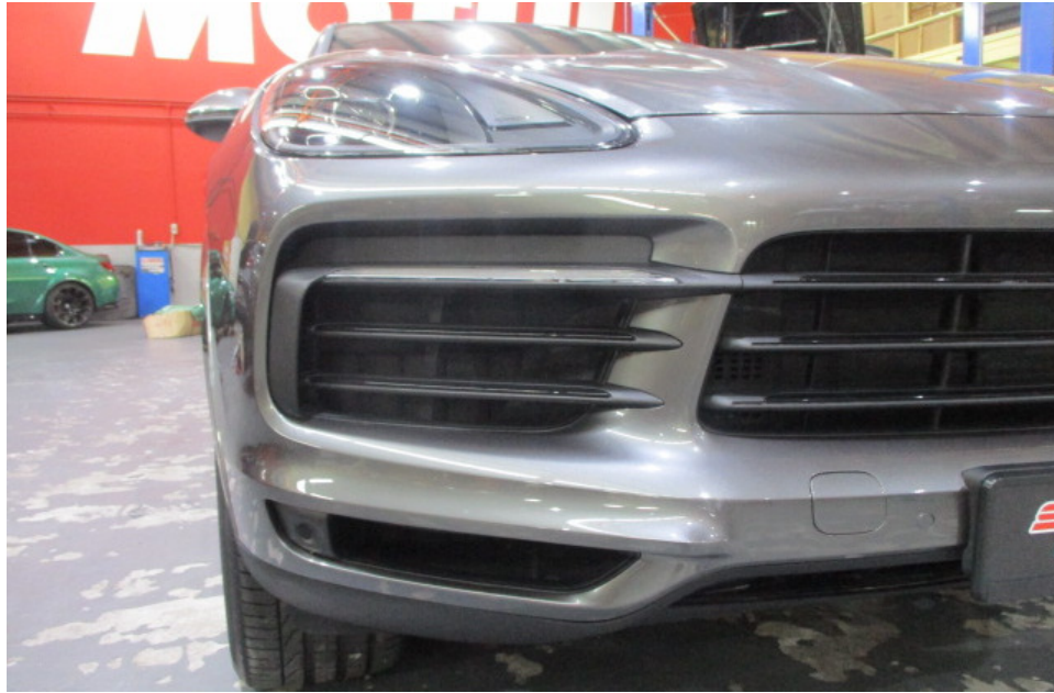
Photo 7 shows a closer view of the Motor Car's front bumper, front bumper lower cover, front bumper right upper grille, front right day light, front right headlamp and front radiator grille. The body parts at the right side front portion of the Motor Car were visually examined and it was observed that the repair/restoration works carried out to the damaged area of the Motor Car (refer to photograph 1 & 2 above) were reasonably adequate and in order.
