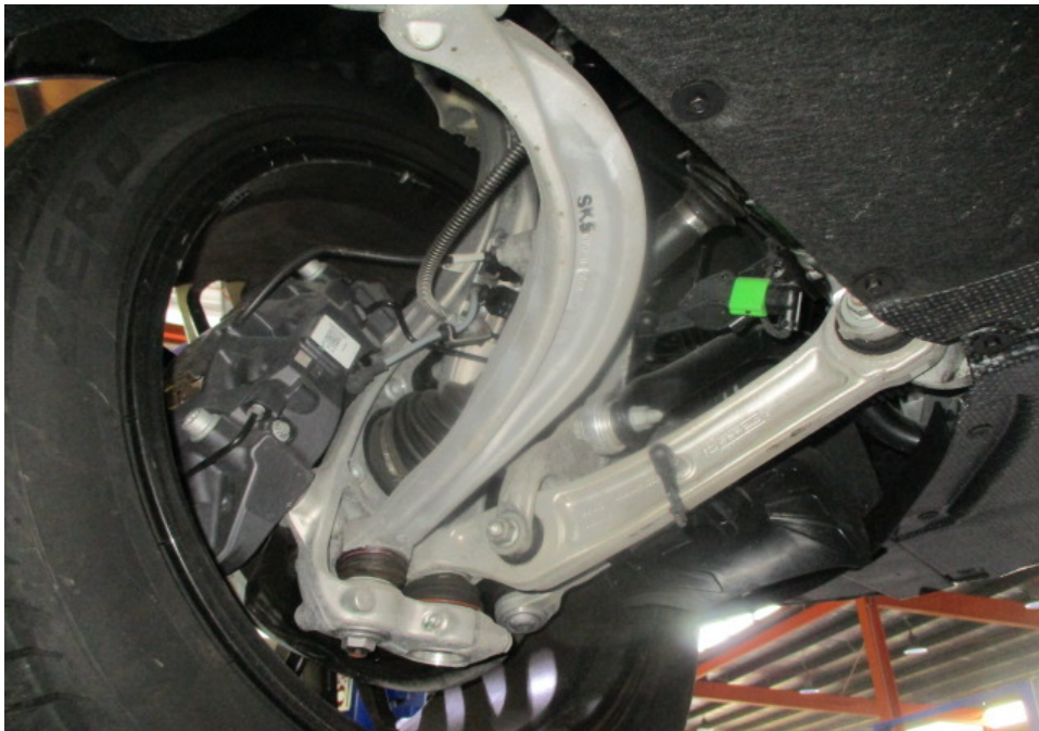
Photo 26 shows a general view of the control arms and linkages at the front left wheel of the Motor Car. I did not observe any fluid leak and/or fluid stain on the underside of the Motor Car. All of the Motor Car's undercarriage components were observed to be intact and secured in an appropriate manner.
