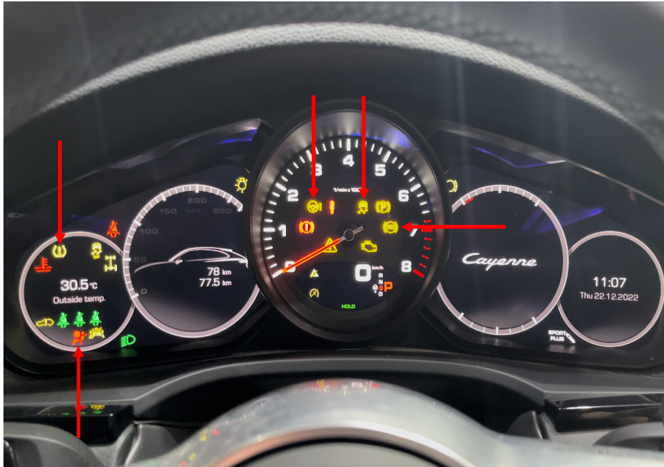
Photo 21 shows the warning lights for the various electronic safety features appearing on the instrument panel of the Motor Car during its self-test when the engine is cranked, in particular the ABS, SRS, TPM, EPS and TCS lights (arrowed).
