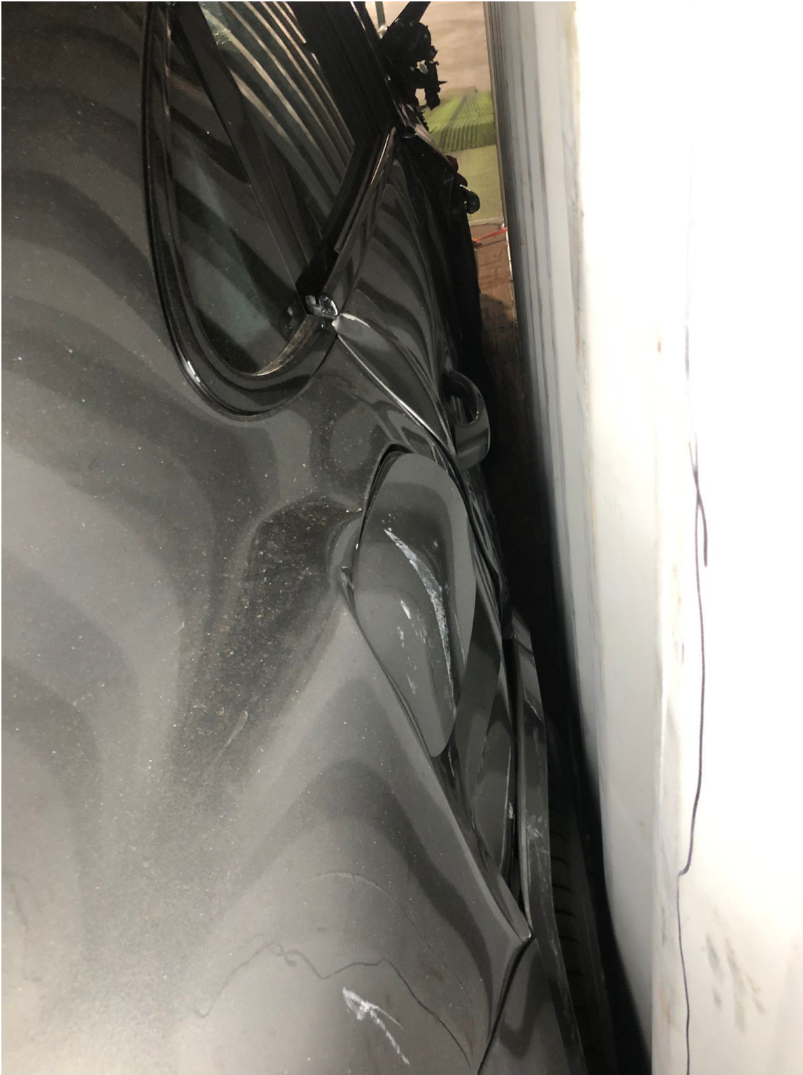
Photo 3 shows the right side rear portion of the Motor Car (photograph provided to me). The Motor Car was observed to have sustained damage at its right side portion and left side front portion. Body parts damaged at the right side portion include the rear bumper, rear right fender, rear right fender wheel arc garnish, rear right door, fuel filler outer cover and right side wing mirror amongst others.
