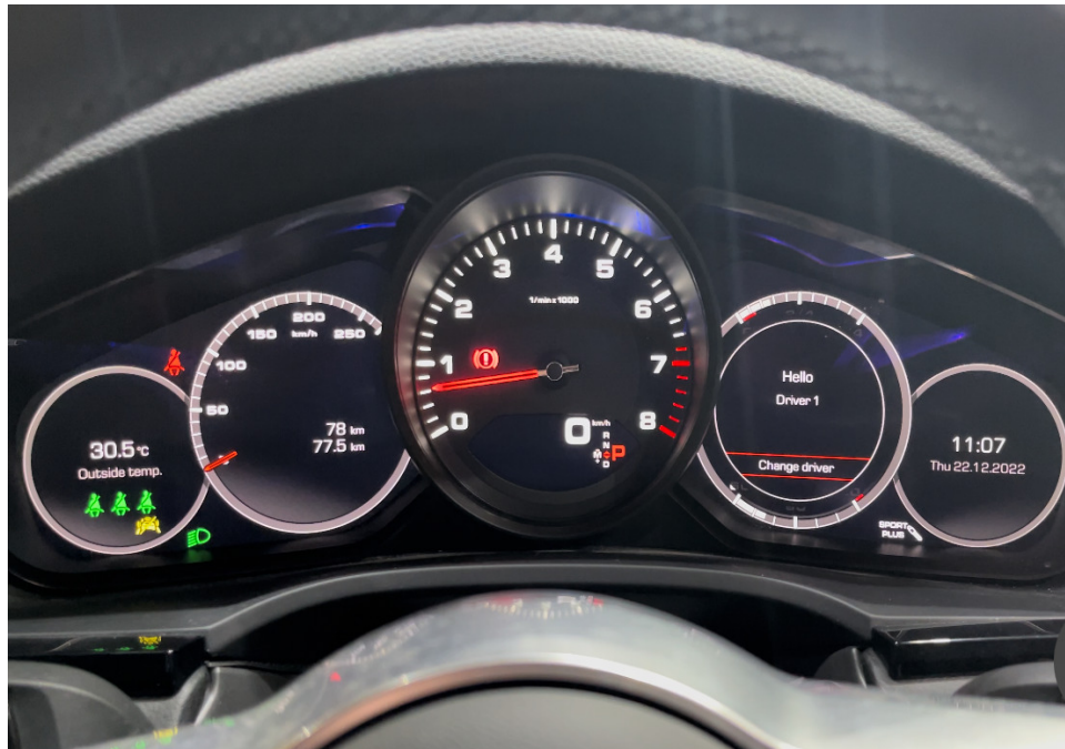
Photo 22 shows the respective warning lights no longer illuminated, indicating that there is no fault detected to the ABS, SRS, TPM, EPS and TCS systems of the Motor Car during the self-test. These electronic systems were hence in working condition at the time of my inspection.
