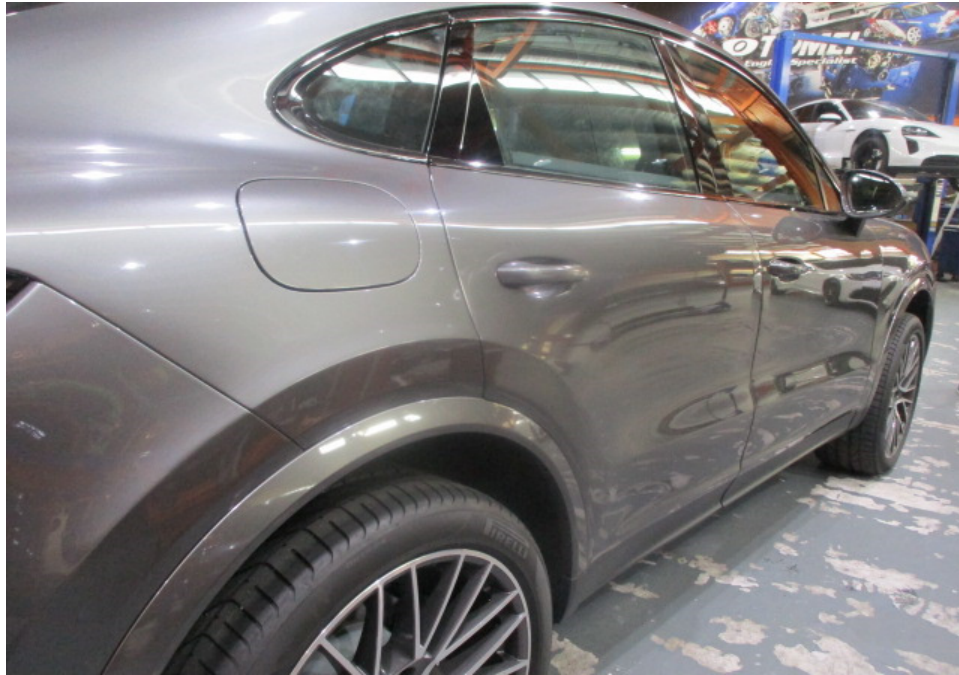
Photo 15 shows a closer view of the Motor Car's rear bumper, rear right fender, rear right fender wheel arc garnish, rear right door and fuel filler outer cover. The body parts at the right side rear portion of the Motor Car were visually examined and it was observed that the repair/restoration works carried out to the damaged area of the Motor Car (refer to photograph 3 above) were reasonably adequate and in order.
