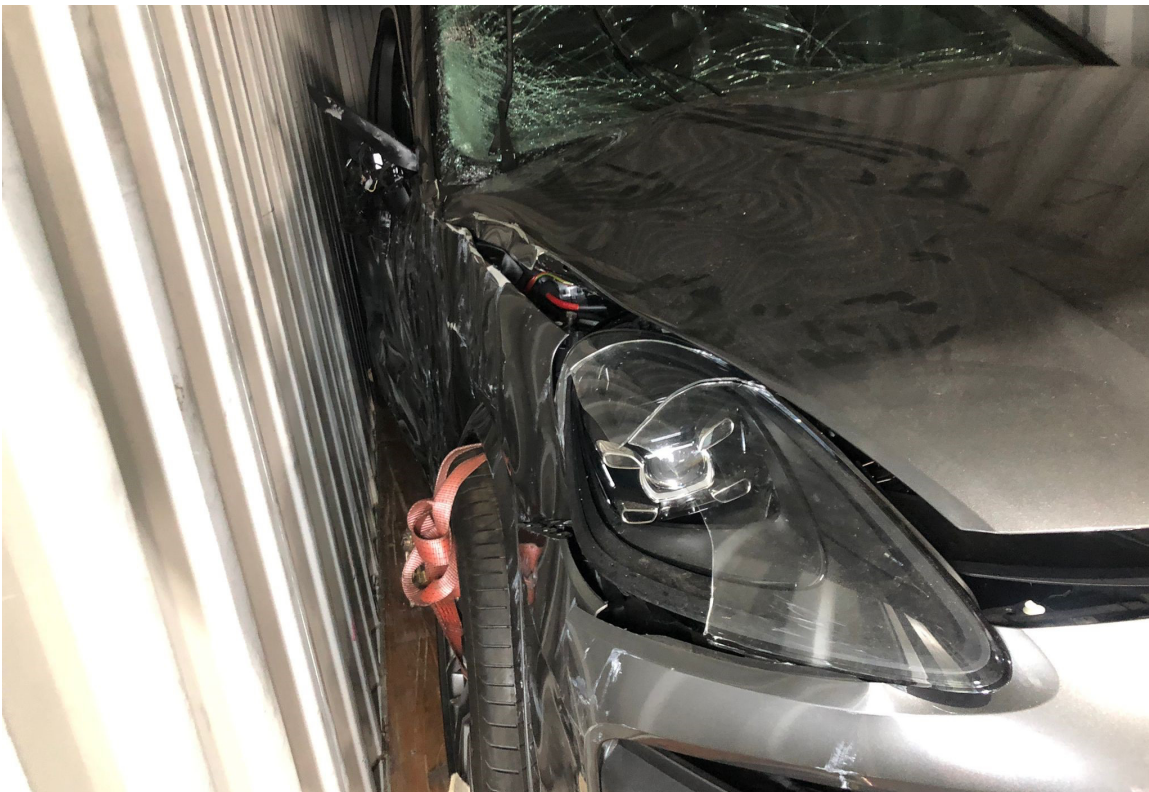
Photo 2 shows the right side front body of the Motor Car (photograph provided to me). The front bonnet, front bumper, front right headlamp, front right fender, front right fender wheel arc garnish, front right door, front right door window and front windscreen were amongst the body parts that were observed to have been damaged.
