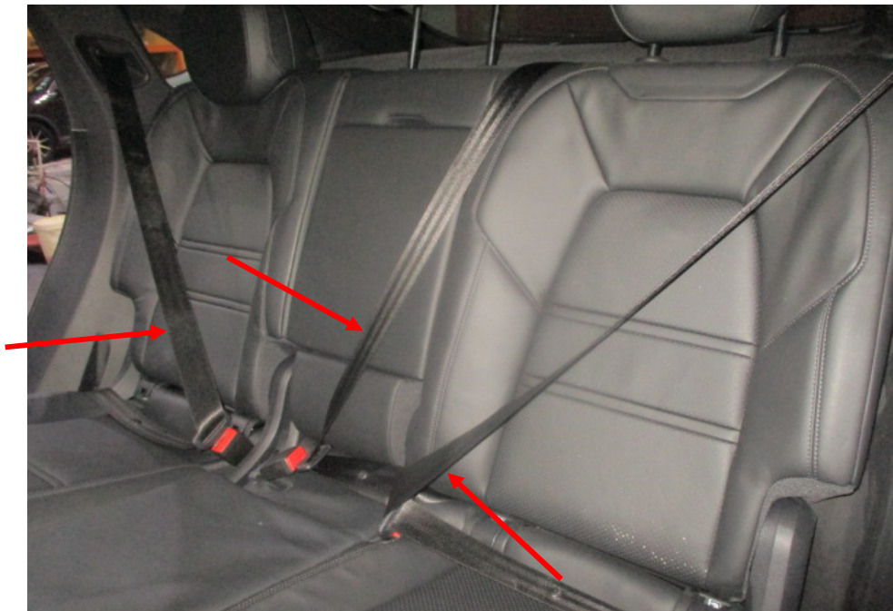
Photo 20 shows the rear seats of the Motor Car. All the seats of the Motor Car were secured via seat rails to the floorboard. They were also fitted with a retractable seat belt reel and a pre-tensioner. The seat belts (arrowed) were tested and were able to be fastened into the respective pre-tensions that were fitted on the side of each individual seat.
