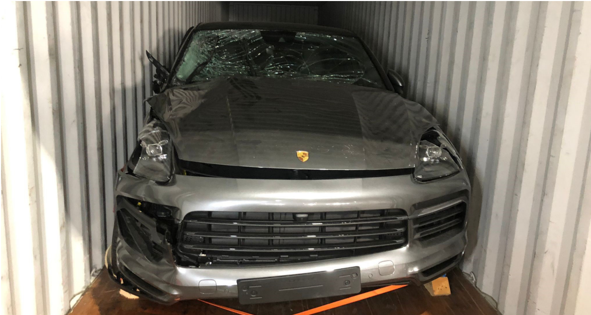
Photo 1 shows the frontal body of the Motor Car (photograph provided to me). The Motor Car was observed to have sustained damage at its right side front portion and left side front portion. The front bumper, front bumper lower cover, front bumper right upper grille, front right day light, front right headlamp, front radiator grille, front bonnet and front windscreen were amongst the body parts that were observed to have been damaged at the right side front portion of the Motor Car.
