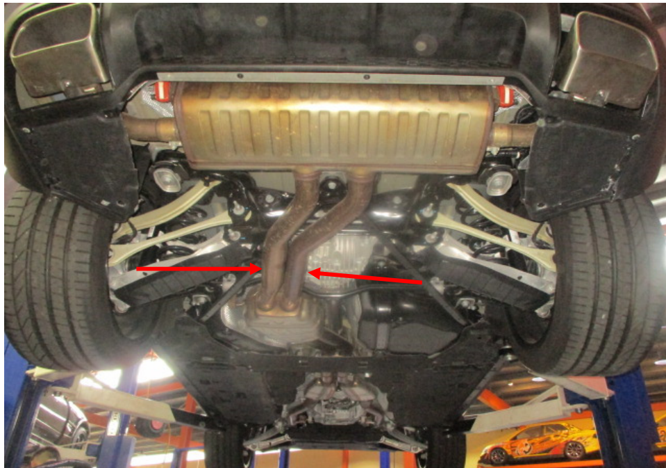
Photo 28 shows the rear section of the Motor Car's exhaust system. My examination of the Motor Car's exhaust system revealed no sign(s) or indication(s) of any cut or weld marks along its exhaust pipes (arrowed), on its rear muffler, on its centre resonator boxes and on its catalytic converters.
