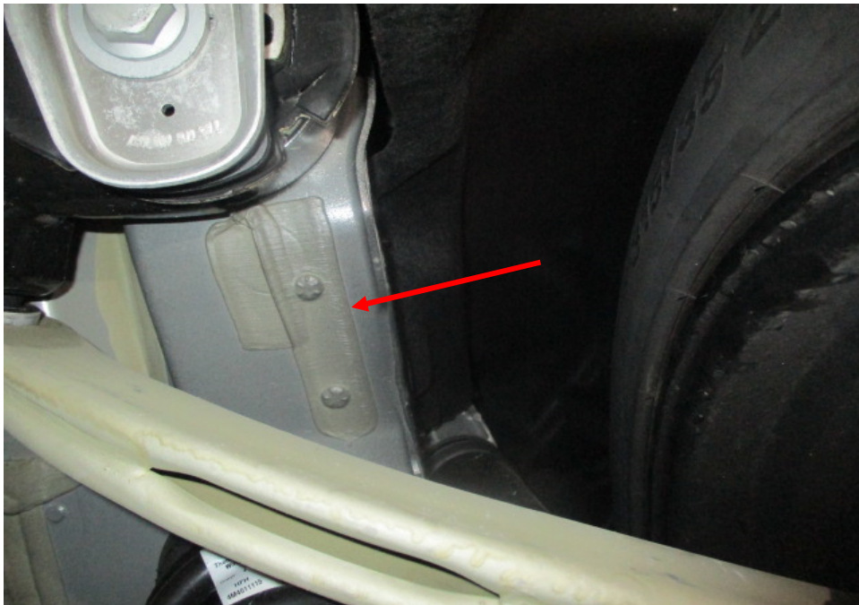
Photo 30 shows the chassis/structural body at the underside rear right of the Motor Car. I did not find any weld marks other than original spot weld marks on the chassis/structural body of the Motor Car. The original factory sealant (arrowed) at the joints along the chassis/structural body was untouched, indicating no work was done on the chassis/structural body of the Motor Car and that the chassis/structural body was originally fitted.
