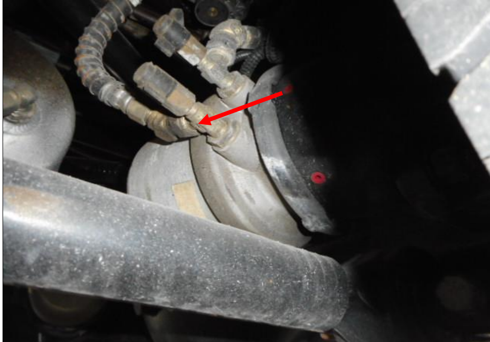
Photo 18 shows the brake pipe (arrowed) at the rear right wheel of the Motor Bus. I did not observe any leakage of brake fluid at the time of my inspection of the Motor Bus. My static tests of the Motor Bus's braking system, along with my visual examination of the various mechanical components in the braking system, had indicated that there was no internal leakage of pressure/vacuum. Hence the braking system of the Motor Bus was likely to be in serviceable condition at the material time of accident.
