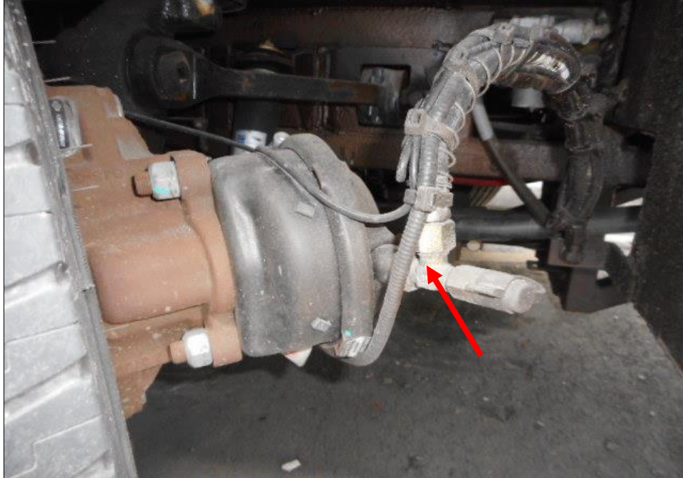
Photo 20 shows the brake pipe (arrowed) at the front right wheel of the Motor Bus. I did not observe any leakage of brake fluid at the time of my inspection of the Motor Bus. My static tests of the Motor Bus's braking system, along with my visual examination of the various mechanical components in the braking system, had indicated that there was no internal leakage of pressure/vacuum. Hence the braking system of the Motor Bus was likely to be in serviceable condition at the material time of accident.
