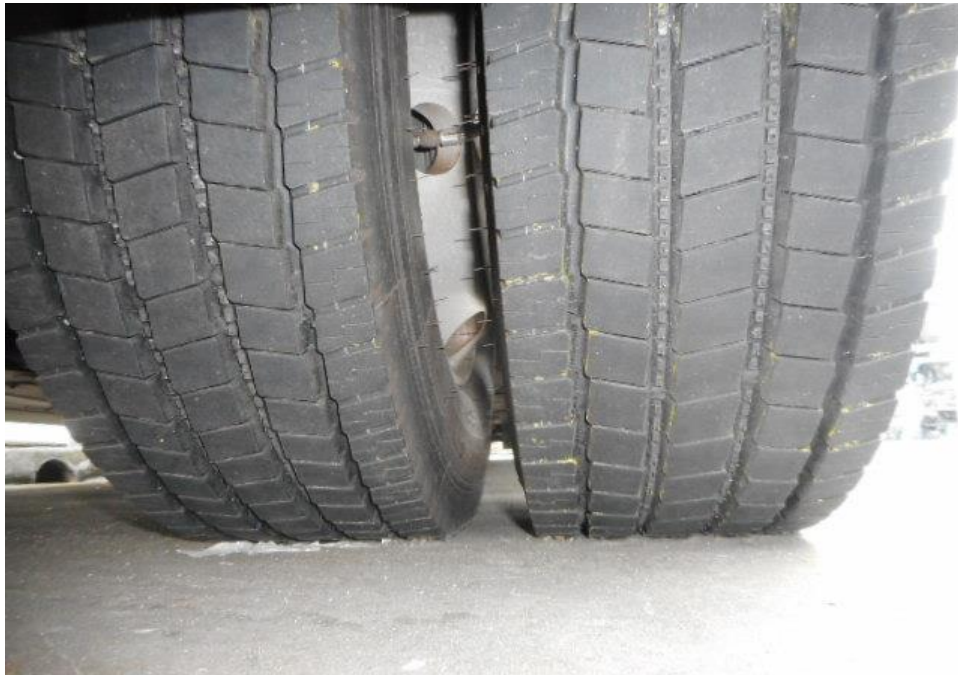
Photo 10 shows the condition of the rear right tyre of the Motor Bus, which was observed to be in serviceable condition with remaining tread depth of approximately 11.1mm. The tyre, which was wrapped around standard steel wheel rim, was also observed to be sufficiently inflated for vehicular operation.
