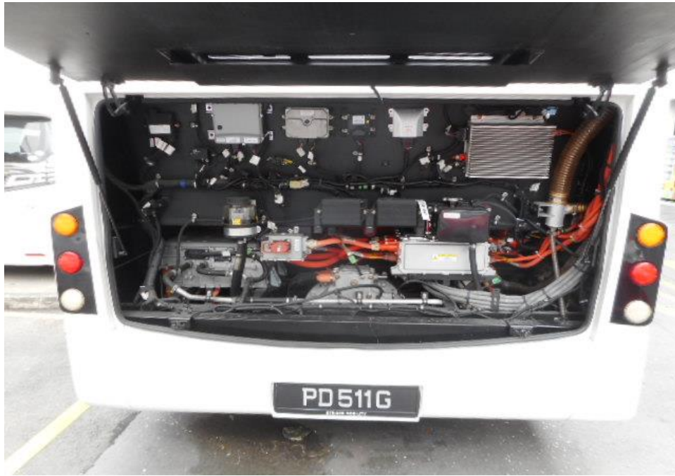
Photo 13 shows a general view of the Motor Bus's electric motor compartment, which was accessed by lifting the rear cabin of the Motor Bus. The various parts and components inside the electric motor compartment were unaffected by the accident. There was also no sign(s) or indication(s) of fresh fluid leakage and/or fluid stain within the electric motor compartment
