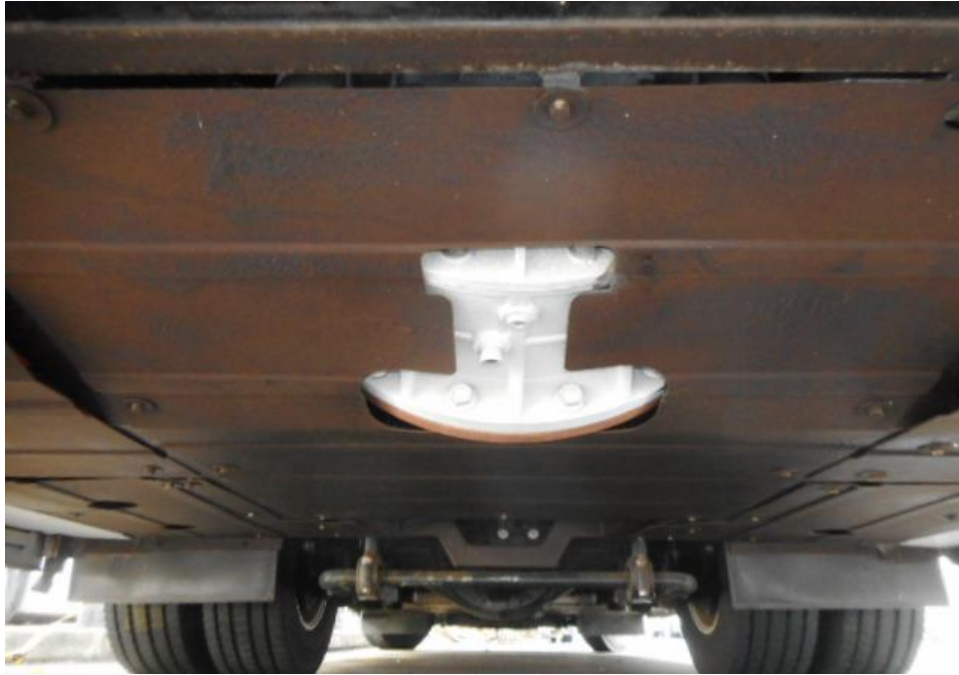
Photo 17 shows the undercarriage of the Motor Bus, at the area where the electric motor housing located. I did not find any sign(s) or indication(s) of fluid leak on the underside of the Motor Bus.
