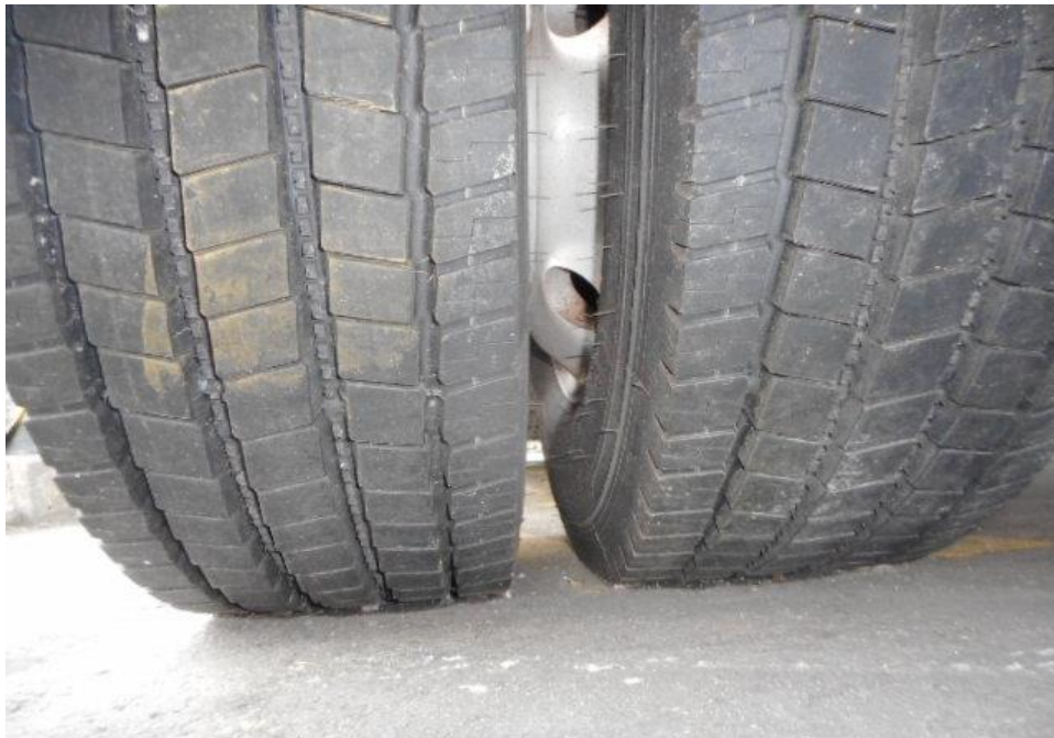
Photo 11 shows the condition of the rear left tyres of the Motor Bus, which was observed to be in serviceable condition with remaining tread depth of approximately 11.2mm. The tyres, which were wrapped around standard steel wheel rim, were also observed to be sufficiently inflated for vehicular operation. There was also no damage found on all 6 steel wheel rims of the Motor Bus.
