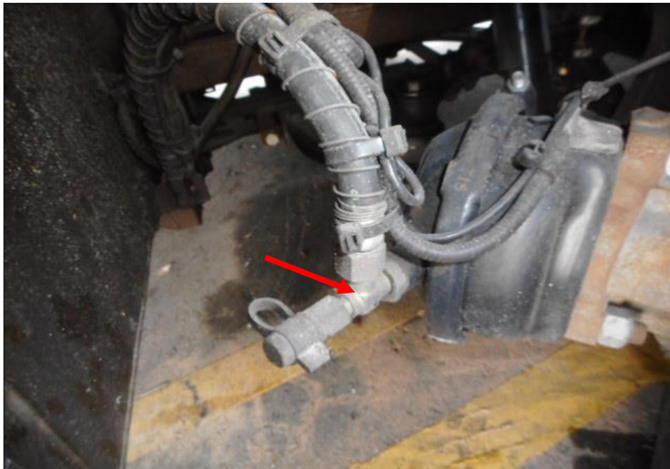
Photo 21 shows the brake pipe (arrowed) at the front left wheel of the Motor Bus. I did not observe any leakage of brake fluid at the time of my inspection of the Motor Bus. My static tests of the Motor Bus's braking system, along with my visual examination of the various mechanical components in the braking system had indicated that there was no internal leakage of pressure/vacuum. Hence the braking system of the Motor Bus was likely to be in serviceable condition at the material time of accident.
