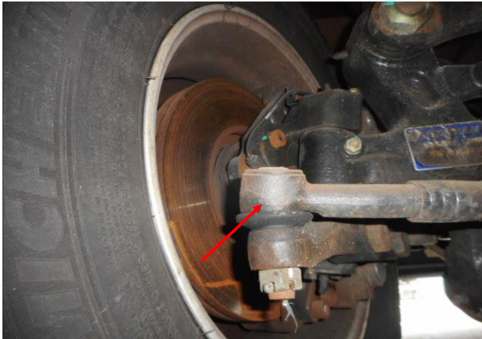
Photo 24 shows the various undercarriage components at the front left wheel of the Motor Bus, in particular the steering tie rod end (arrowed). The various undercarriage components of the Motor Bus were all found to be intact without any visible damage. There was also no sign of fluid stain(s) observed on the various undercarriage components.
