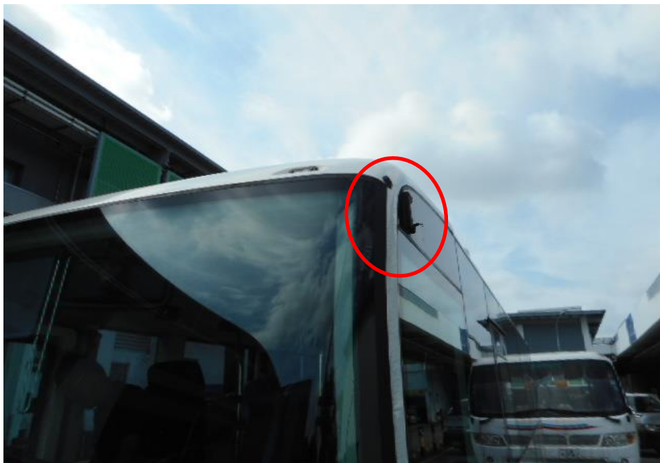
Photo 5 shows a close up view of the right body of the Motor Bus at the time of my inspection. The front portion of the Motor Bus was observed to sustained damage at the time of inspection. Its left rear view mirror (circled) was amongst the body parts that were damaged as a result of the accident.
