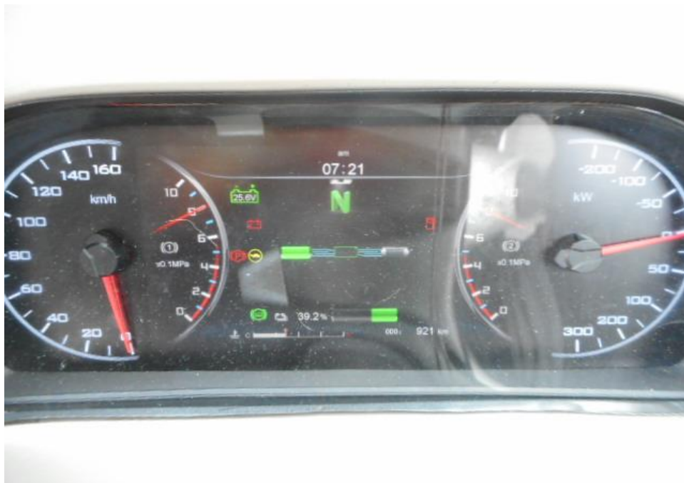
Photo 28 shows no warning lights illuminated on the instrument panel of the Motor Bus after the electric motor was cranked. This would suggest that there was no abnormality to the electronic operating system of the Motor Bus, like the ABS and etc.
