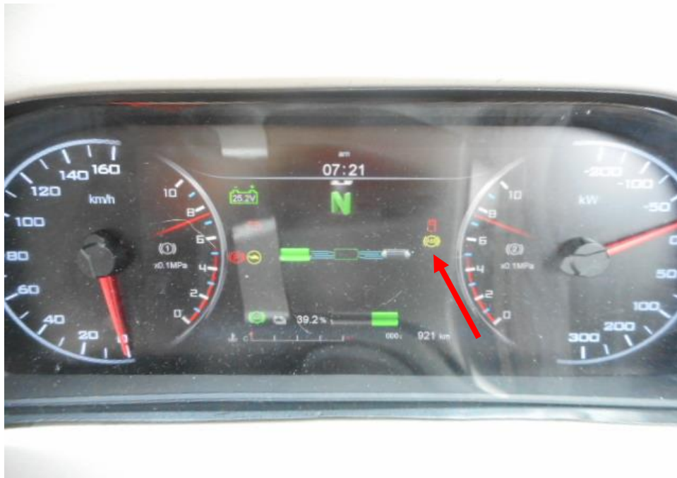
Photo 27 shows the warning light for Anti-Lock Brake System (ABS) (arrowed) appearing on the instrument panel of the Motor Bus during the self-test of its various electronic operating systems when its electric motor was cranked.
