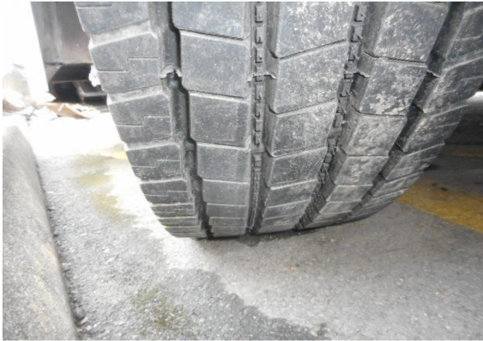
Photo 12 shows the condition of the front left tyres of the Motor Bus, which were observed to be in serviceable condition with remaining tread depth of approximately 10.3mm. There was also no tear, cut or burst mark(s) on the outer and the inner sidewalls as well as across the tread of the 6 tyres that were fitted on the Motor Bus.
