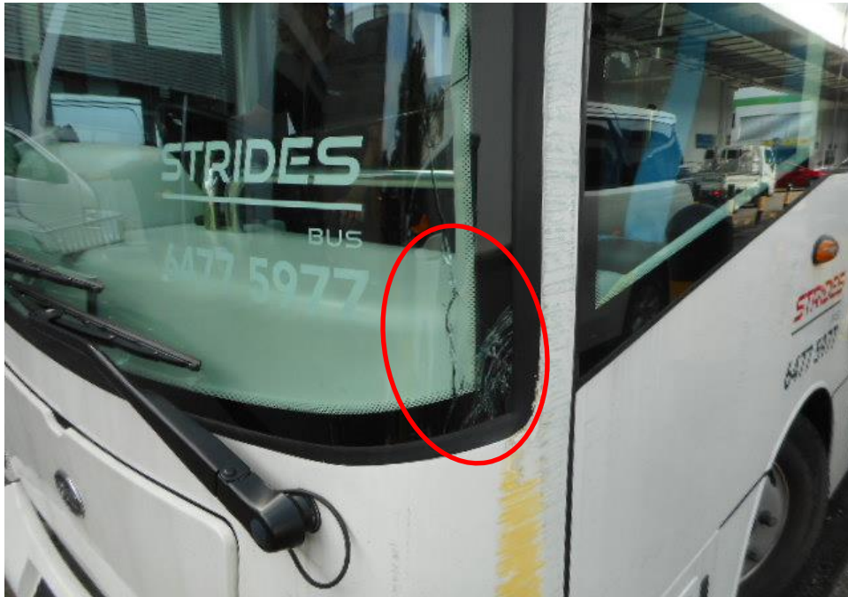
Photo 4 shows a close up view of the right body of the Motor Bus at the time of my inspection. The front portion of the Motor Bus was observed to sustained damage at the time of inspection. Its front windscreen (circled) was amongst the body parts that were damaged as a result of the accident.
