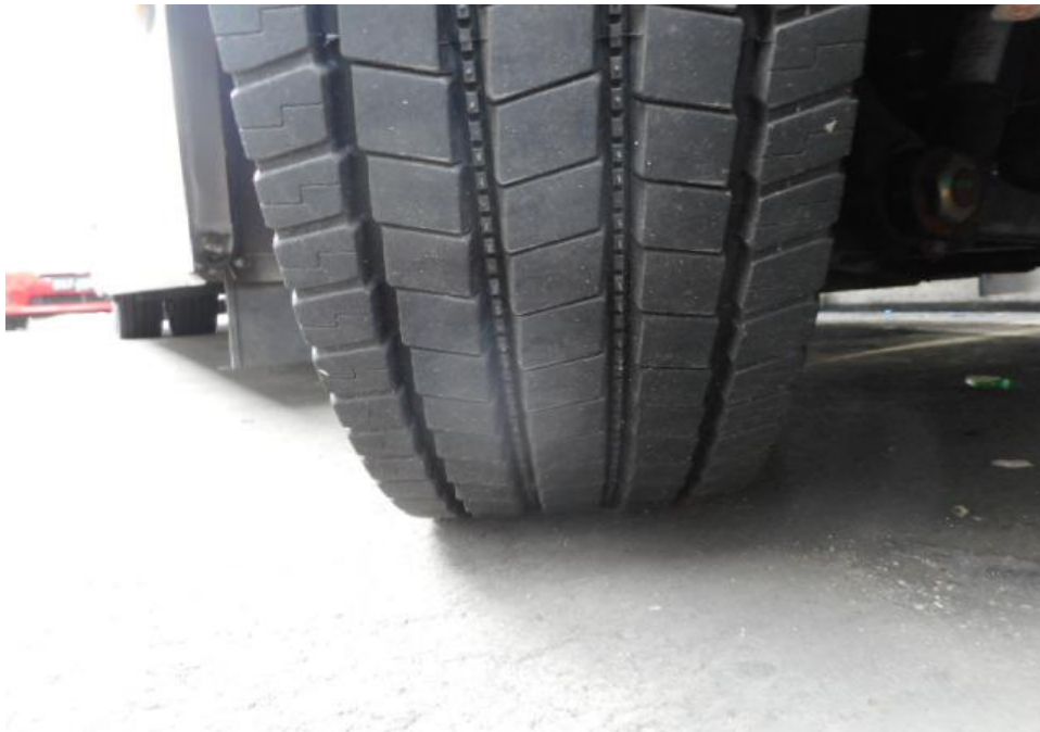
Photo 9 shows the condition of the front right tyre of the Motor Bus, which was observed to be in serviceable condition with remaining tread depth of approximately 10.1mm. The tyre, which was wrapped around standard steel wheel rim, was also observed to be sufficiently inflated for vehicular operation. There was no tear, cut or burst mark(s) on the outer and the inner sidewalls as well as across the tread of the 6 tyres that were fitted on the Motor Bus.
