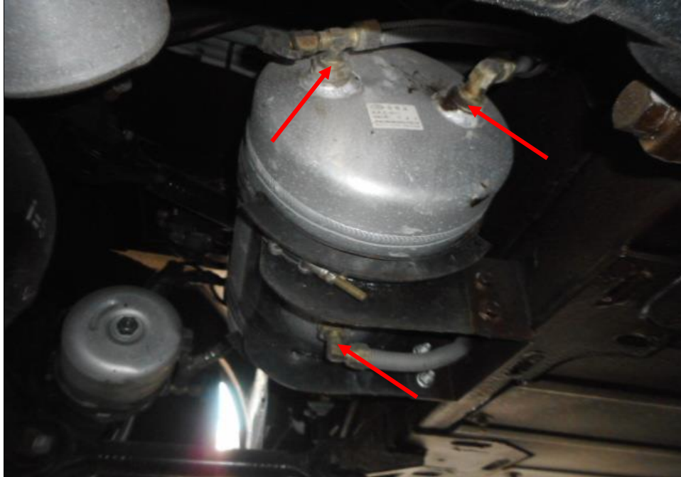
Photo 22 shows the air brake cylinders (arrowed) at the undercarriage of the Motor Bus. I did not observe any leakage of air brake fluid at the time of my inspection of the Motor Bus. My static tests of the Motor Bus's braking system, along with my visual examination of the various mechanical components in the braking system had indicated that there was no internal leakage of pressure/vacuum. Hence the braking system of the Motor Bus was likely to be in serviceable condition at the material time of accident.
