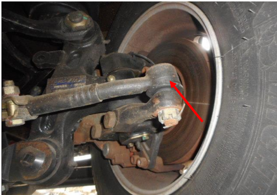
Photo 23 shows the various undercarriage components at the front right wheel of the Motor Bus, in particular the steering tie rod end (arrowed). The various steering components were all found to be intact, suggesting that the steering system of the Motor Bus was likely to be in serviceable condition at the material time of accident. There was also no sign of fluid stain(s) observed on the various undercarriage components.
