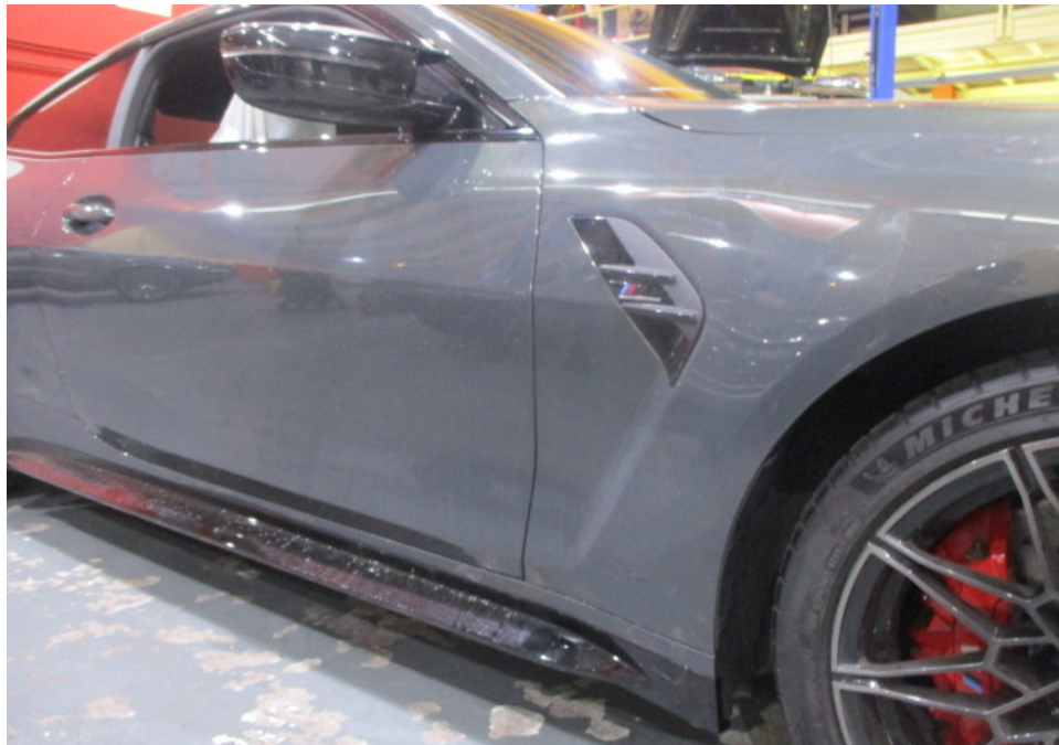
Photo 8 shows a closer view of the Motor Car's front right fender, front right door, right side wing mirror and right side rocker panel garnish. The body parts at the right side portion of the Motor Car were visually examined and it was observed that the repair/restoration works carried out to the damaged area of the Motor Car (refer to photograph 1 above) were reasonably adequate and in order.
