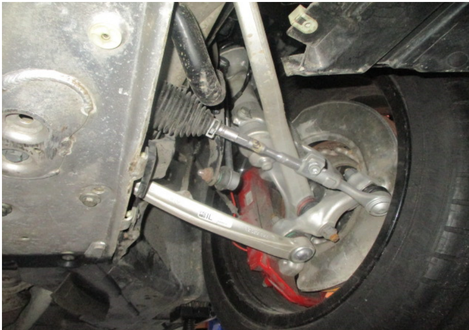
Photo 24 shows a general view of the control arms and linkages at the front left wheel of the Motor Car. I did not observe any fluid leak and/or fluid stain on the underside of the Motor Car. All of the Motor Car's undercarriage components were observed to be intact and secured in an appropriate manner.
