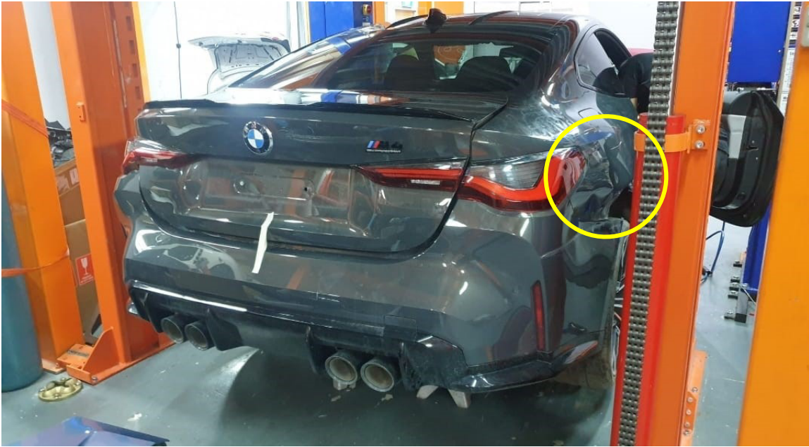
Photo 4 shows the rear right body of the Motor Car (photograph provided to me). The rear right body panel was observed to be damaged (circled).
