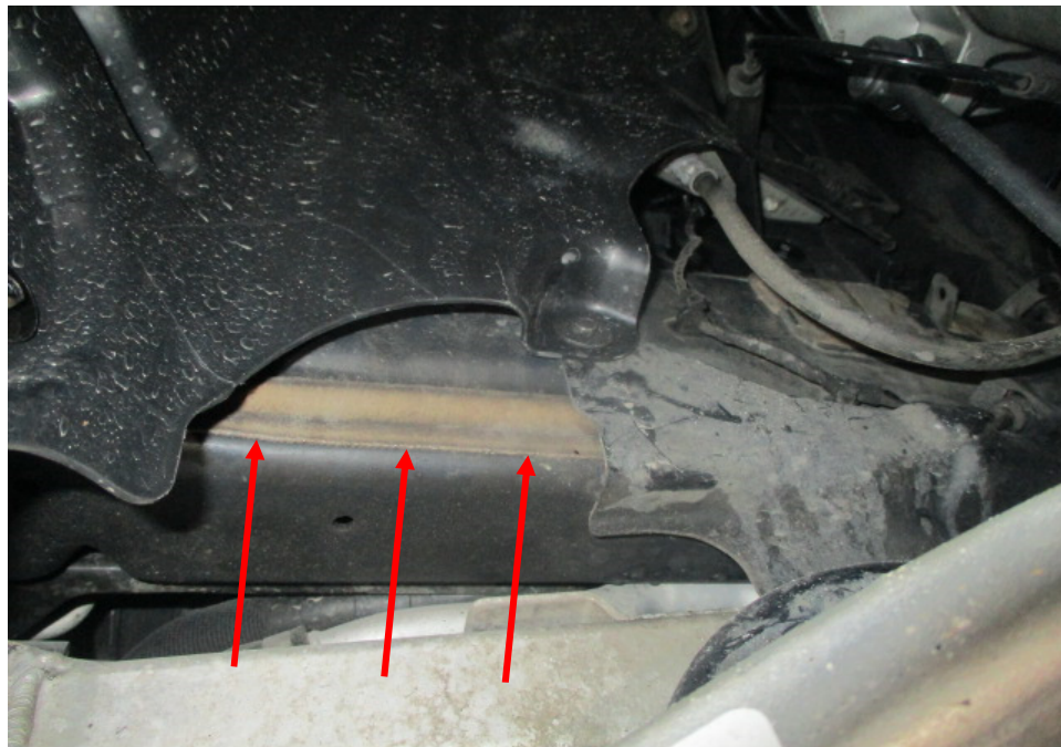
Photo 30 shows the chassis/structural body at the underside front left of the Motor Car. The original factory sealant (arrowed) at the joints along the chassis/structural body was observed to be untouched. In general, I had found no work was carried out on the chassis/structural body of the Motor Car. The chassis/structural body of the Motor Car was originally fitted.
