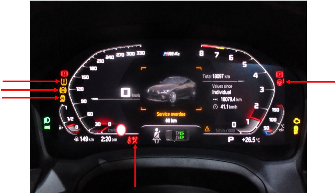
Photo 19 shows the warning lights for the various electronic safety features appearing on the instrument panel of the Motor Car during its self-test when the engine is cranked, in particular the ABS, SRS, IAS, TPM and DSC lights (arrowed).
