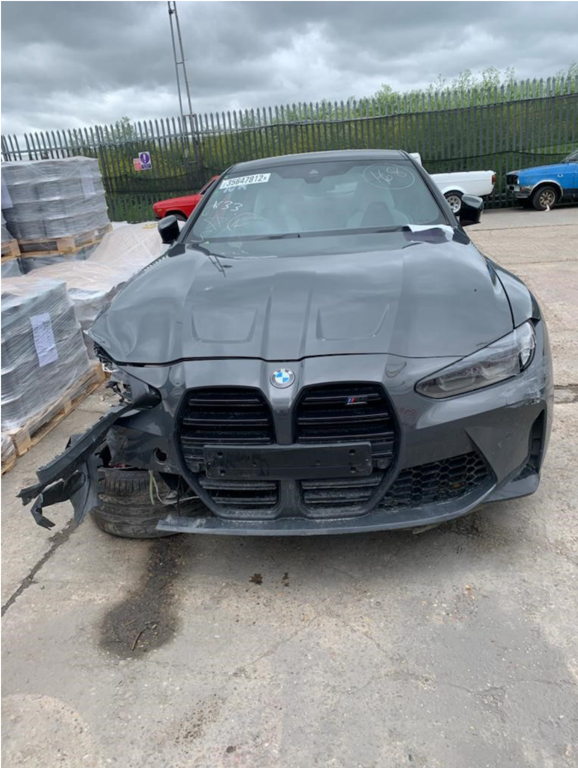
Photo 3 shows the frontal body of the Motor Car (photograph provided to me). The Motor Car was observed to have sustained damage at its front right portion. The front bumper, front bumper right lower grille, front bumper right sensor, front bumper right corner air guide, front bonnet, front right headlamp and front left headlamp were amongst the body parts that were observed to have been damaged. The airbag(s) of the Motor Car was not deployed as seen from the photographs that were provided to me.
