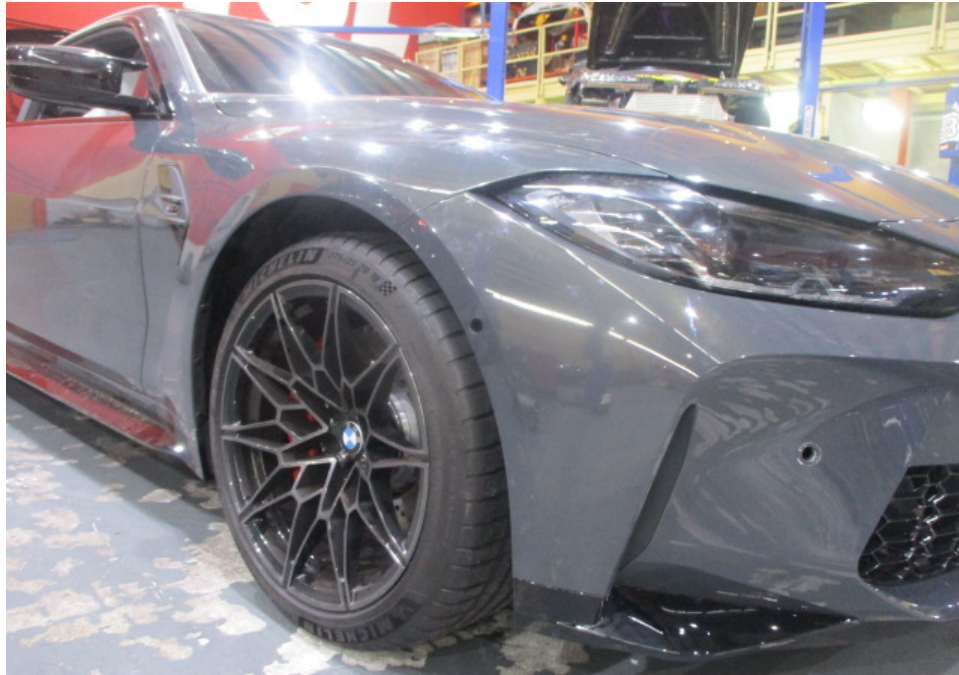
Photo 7 shows a closer view of the Motor Car's front bumper, front right headlamp, front right fender, front right wheel rim and front right tyre. The body parts at the right side front portion of the Motor Car were visually examined and it was observed that the repair/restoration works carried out to the damaged area of the Motor Car (refer to photograph 1 above) were reasonably adequate and in order.
