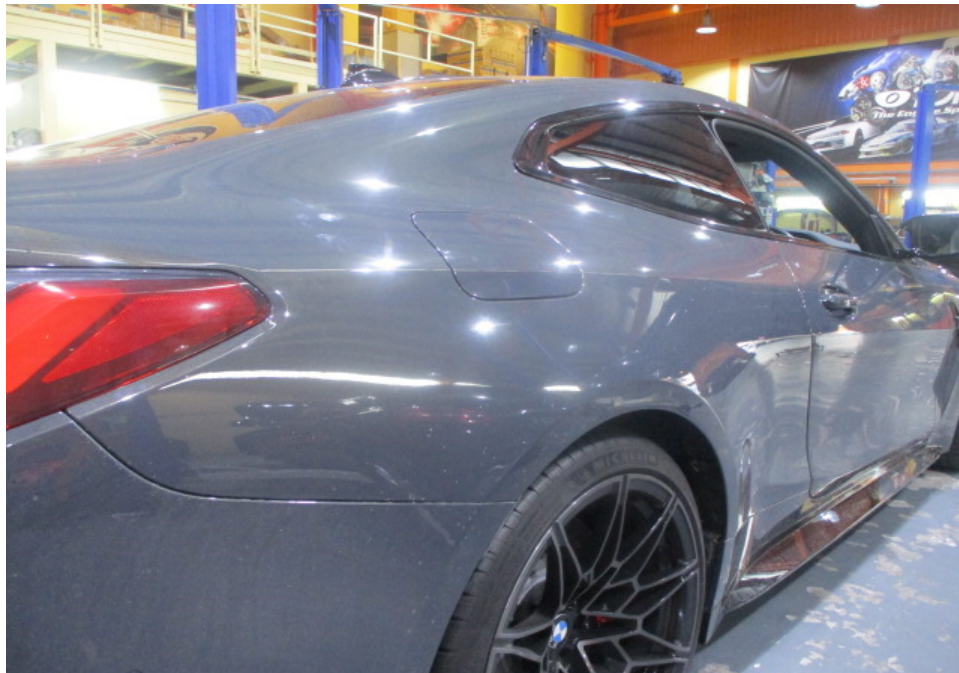
Photo 14 shows a closer view of the Motor Car's rear bumper, rear right taillamp and rear right body panel. The body parts at the rear right portion of the Motor Car were visually examined and it was observed that the repair/restoration works carried out to the damaged area of the Motor Car (refer to photograph 4 above) were reasonably adequate and in order.
