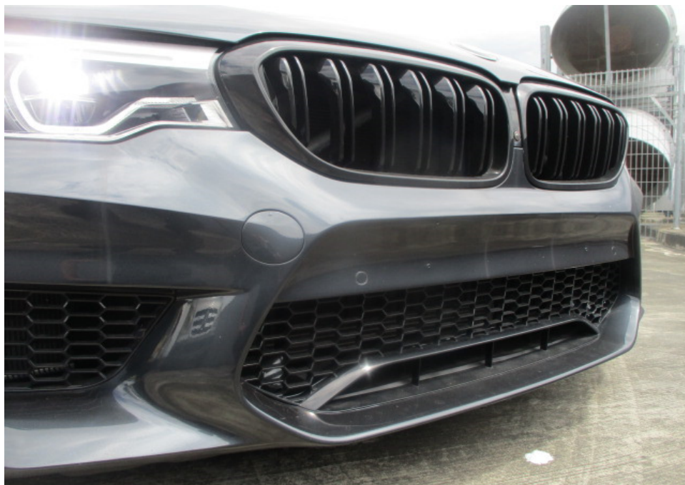
Photo 12 shows a closer view of the Motor Car's front bumper, front bumper centre lower grille, front bumper sensors, front bumper tow cover and front radiator grilles. The body parts at the front right portion of the Motor Car were visually examined and it was observed that the repair/restoration works carried out to the damaged area of the Motor Car (refer to photograph 1 - 2 above) were reasonably adequate and in order.
