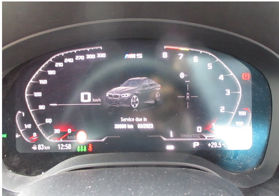
Photo 24 shows the respective warning lights no longer illuminated, indicating that there is no fault detected to the ABS, SRS, IAS, TPM and DSC systems of the Motor Car during the self-test. These electronic systems were hence in working condition at the time of my inspection.
