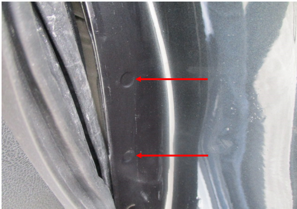
Photo 38 shows the right side "A" pillar of the Motor Car. I did not find any weld marks other than original spot weld marks (arrowed) on the right side "A" pillar of the Motor Car, which indicates that there was no re-welding works carried out. In general, I had found all the non-detachable body panels of the Motor Car to be originally fitted at the time of my inspection.
