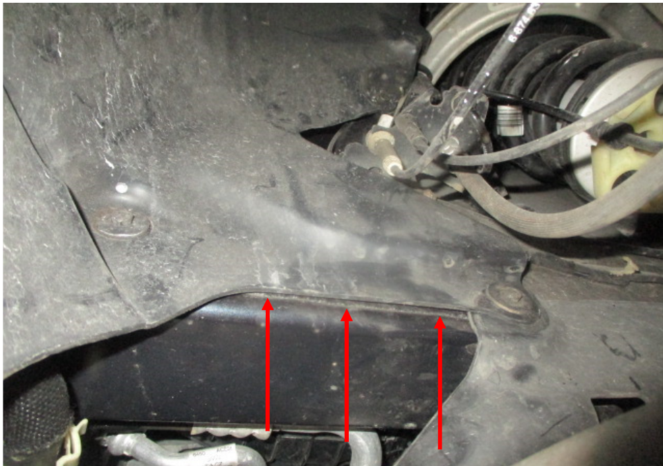
Photo 34 shows the chassis/structural body at the underside front left of the Motor Car. The original factory sealant (arrowed) at the joints along the chassis/structural body was observed to be untouched. In general, I had found no work was carried out on the chassis/structural body of the Motor Car. The chassis/structural body of the Motor Car was originally fitted.
