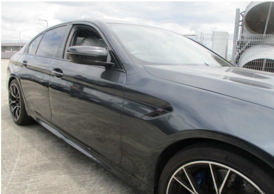
Photo 10 shows a closer view of the Motor Car's front right fender, front right door and right side wing mirror. The body parts at the right side front portion of the Motor Car were visually examined and it was observed that the repair/restoration works carried out to the damaged area of the Motor Car (refer to photograph 2 above) were reasonably adequate and in order.
