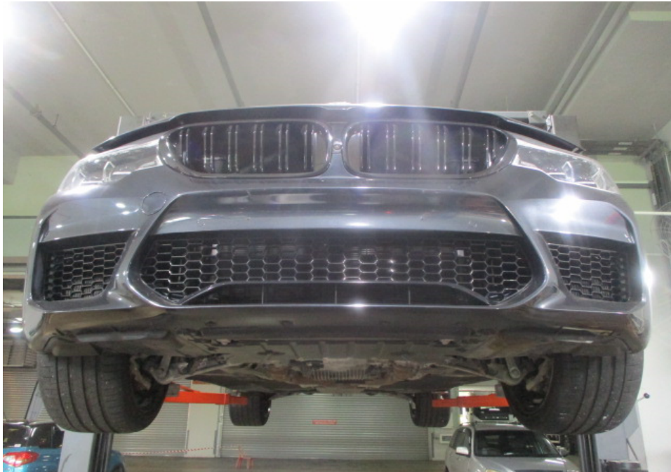
Photo 25 shows the Motor Car hoisted up for checks on its undercarriage. There was no sign(s) or indication(s) of fluid leakage and/or fluid stain(s) on the underside of the Motor Car. The undercarriage components of the Motor Car were also all observed to be intact and secured in an appropriate manner.
