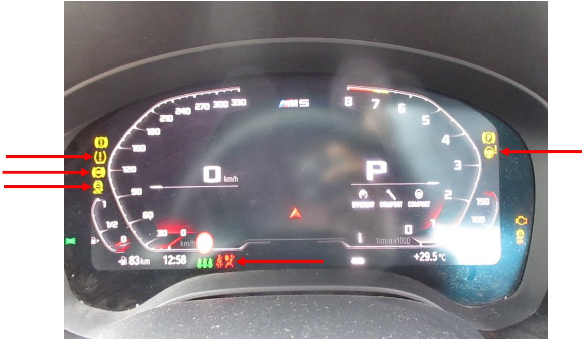
Photo 23 shows the warning lights for the various electronic safety features appearing on the instrument panel of the Motor Car during its self-test when the engine is cranked, in particular the ABS, SRS, IAS, TPM and DSC lights (arrowed).
