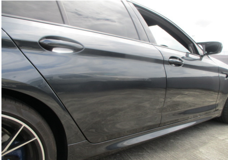
Photo 17 shows a closer view of the Motor Car's rear right door, rear right door handle, front right door, front right door handle and right side rocker panel garnish. The body parts at the right side centre portion of the Motor Car were visually examined and it was observed that the repair/restoration works carried out to the damaged area of the Motor Car (refer to photograph 2 & 4 above) were reasonably adequate and in order.
