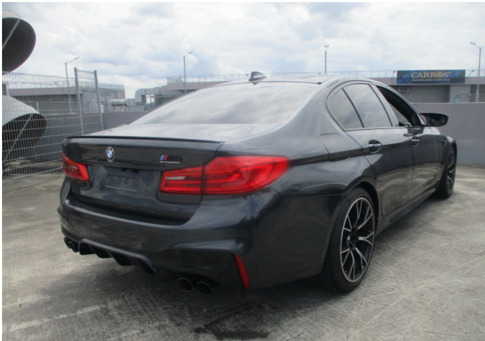
Photo 14 shows a general view of the rear right body of the Motor Car at the time of my inspection. The Motor Car was observed to be in a relatively good general condition with no loose exterior fittings observed. The body parts at the right side portion of the Motor Car were visually examined and it was observed that the repair/restoration works carried out to the damaged area of the Motor Car (refer to photograph 3 & 4 above) were reasonably adequate and in order.
