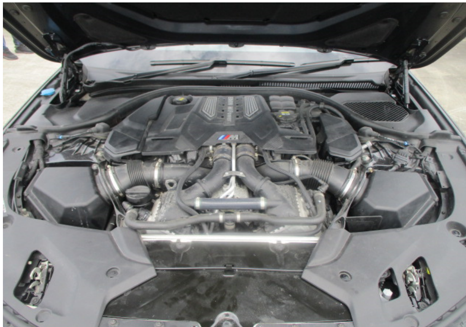
Photo 20 shows a general view of the Motor Car's engine compartment at the time of my inspection. The various parts and components inside the engine compartment were all observed to be intact and properly fitted. There was also no sign(s) or indication(s) of fluid leak and/or fluid stain found inside the engine compartment.
