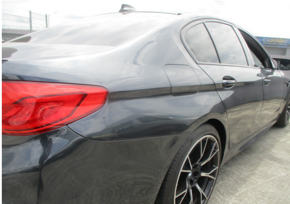
Photo 15 shows a closer view of the Motor Car's rear bumper, rear right taillamp and rear right fender. The body parts at the right side rear portion of the Motor Car were visually examined and it was observed that the repair/restoration works carried out to the damaged area of the Motor Car (refer to photograph 3 & 4 above) were reasonably adequate and in order.
