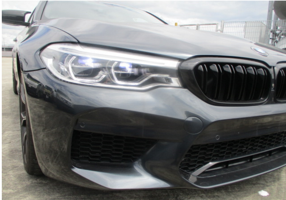
Photo 11 shows a closer view of the Motor Car's front bumper, front bumper right lower grille and front right headlamp. The body parts at the front right portion of the Motor Car were visually examined and it was observed that the repair/restoration works carried out to the damaged area of the Motor Car (refer to photograph 1 - 2 above) were reasonably adequate and in order.
