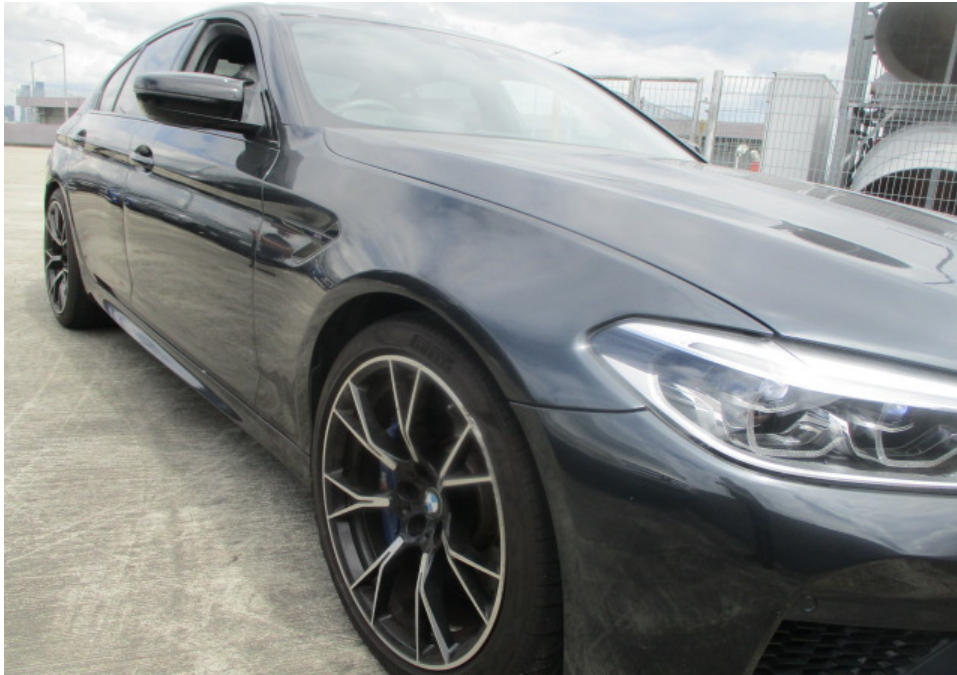
Photo 9 shows a closer view of the Motor Car's front right headlamp, front right wheel rim and front right fender. The body parts at the front right portion and right side front portion of the Motor Car were visually examined and it was observed that the repair/restoration works carried out to the damaged area of the Motor Car (refer to photograph 1 - 2 above) were reasonably adequate and in order.
