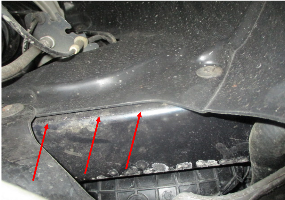
Photo 35 shows the chassis/structural body at the underside front right of the Motor Car. I did not find any weld marks other than original spot weld marks on the chassis/structural body of the Motor Car. The original factory sealant (arrowed) at the joints along the chassis/structural body was untouched, indicating no work was done on the chassis/structural body of the Motor Car and that the chassis/structural body was originally fitted.
