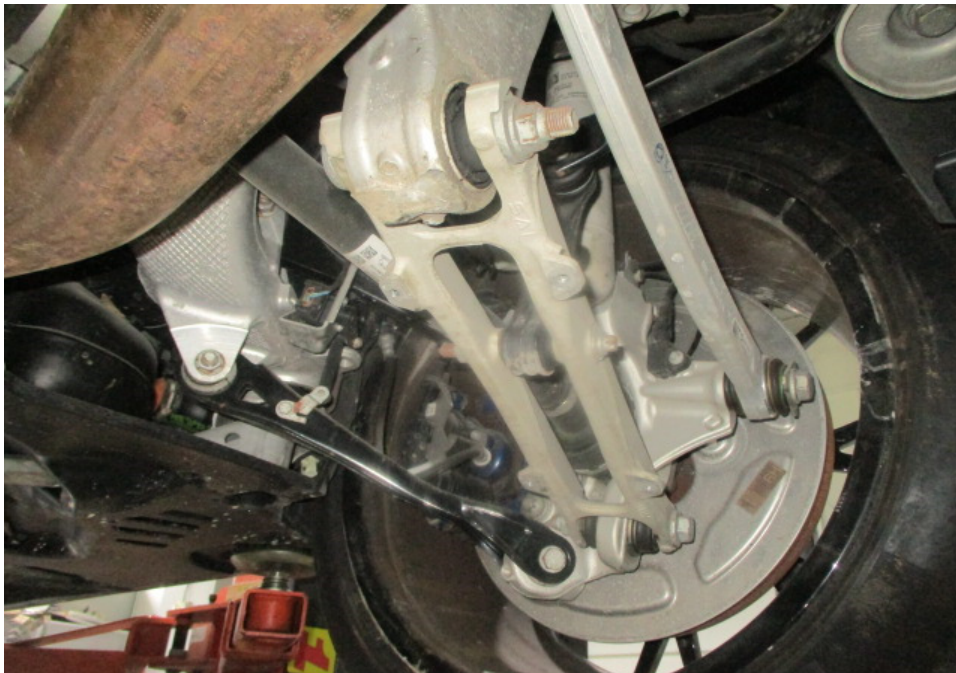
Photo 26 shows a general view of the control arms and linkages at the rear right wheel of the Motor Car. I did not observe any fluid leak and/or fluid stain on the underside of the Motor Car. All of the Motor Car's undercarriage components were observed to be intact and secured in an appropriate manner.
