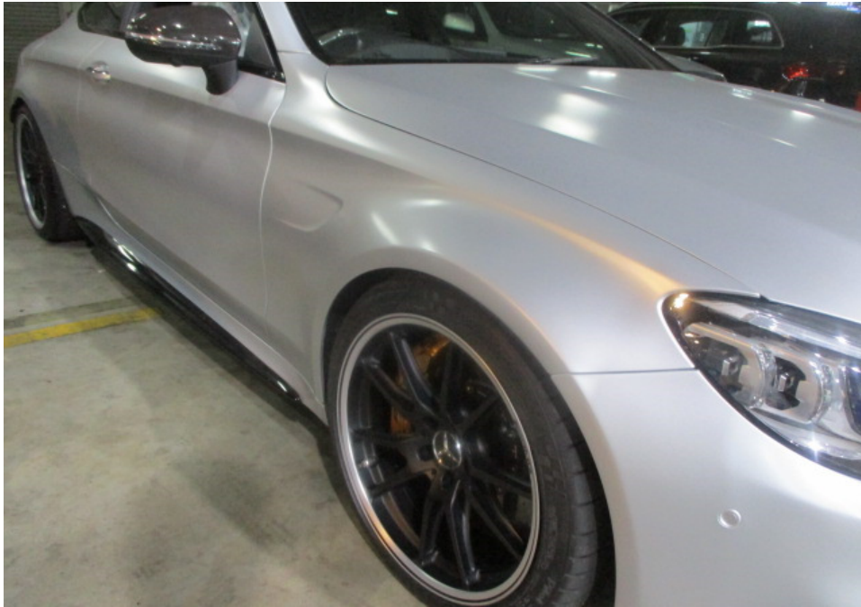
Photo 6 shows a closer view of the Motor Car's front bonnet, front right headlamp, front right wheel rim and front right fender. The body parts at the frontal portion of the Motor Car were visually examined and it was observed that the repair/restoration works carried out to the damaged area of the Motor Car (refer to photograph 1 & 2 above) were reasonably adequate and in order.
