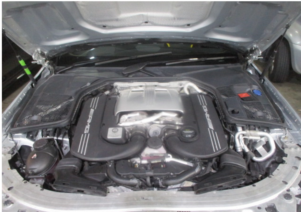
Photo 15 shows a general view of the Motor Car's engine compartment at the time of my inspection. The various parts and components inside the engine compartment were all observed to be intact and properly fitted. There was also no sign(s) or indication(s) of fluid leak and/or fluid stain found inside the engine compartment.
