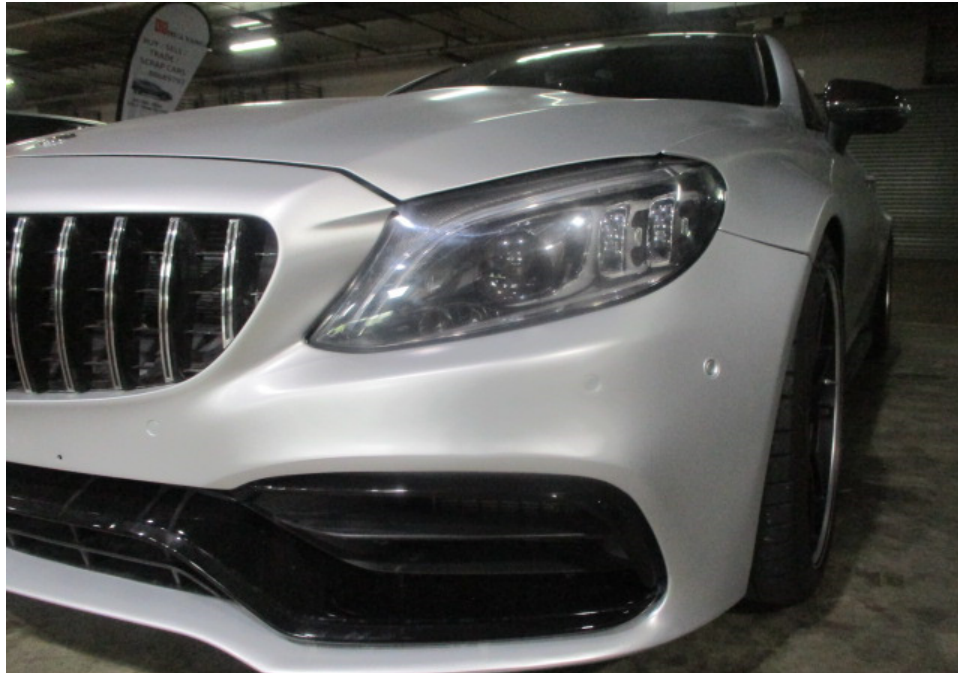
Photo 10 shows a closer view of the Motor Car's front bumper, front bumper left lower grille, front bumper sensors and front left headlamp. The body parts at the frontal portion of the Motor Car were visually examined and it was observed that the repair/restoration works carried out to the damaged area of the Motor Car (refer to photograph 1 & 2 above) were reasonably adequate and in order.
