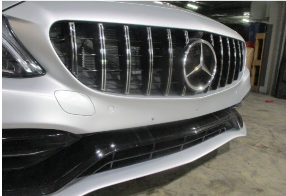
Photo 8 shows a closer view of the Motor Car's front bumper, front bumper centre lower garnish, front bumper centre lower grille, front bumper sensors, front radiator grille and front emblem. The body parts at the frontal portion of the Motor Car were visually examined and it was observed that the repair/restoration works carried out to the damaged area of the Motor Car (refer to photograph 1 & 2 above) were reasonably adequate and in order.
