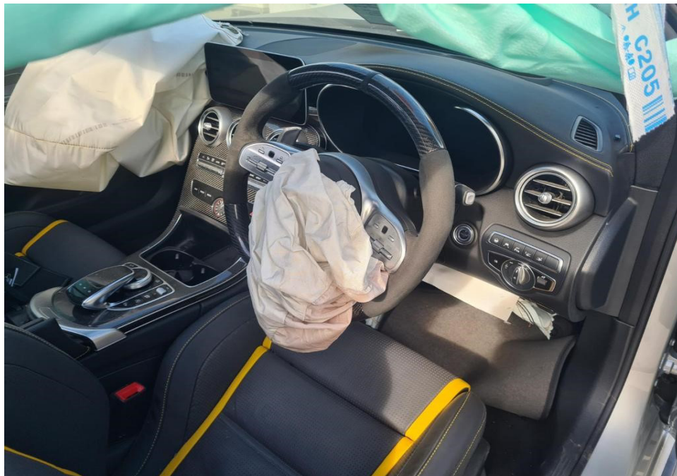
Photo 4 shows the interior compartment of the Motor Car (photograph provided to me). The driver's airbag, driver's knee airbag, front left passenger airbag and right curtain airbag were deployed.
