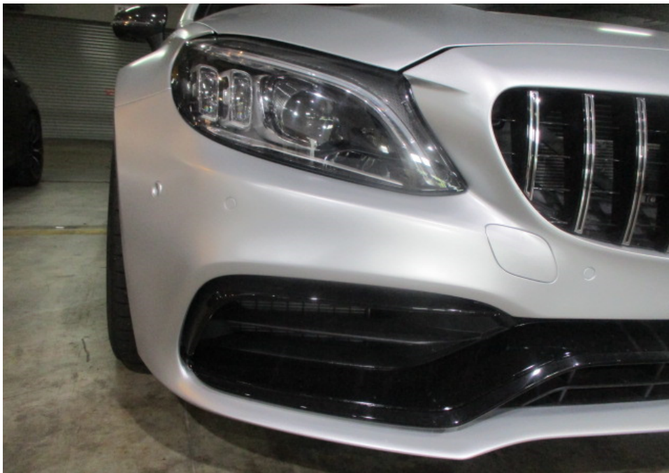
Photo 7 shows a closer view of the Motor Car's front bumper, front bumper right lower grille, front bumper tow cover and front right headlamp. The body parts at the frontal portion of the Motor Car were visually examined and it was observed that the repair/restoration works carried out to the damaged area of the Motor Car (refer to photograph 1 & 2 above) were reasonably adequate and in order.
