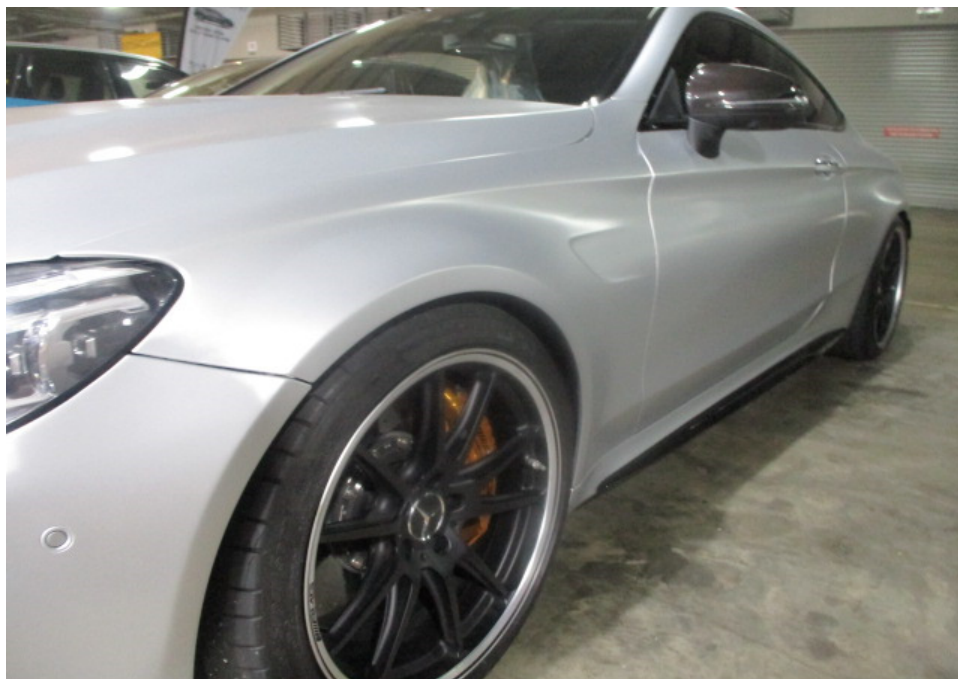
Photo 11 shows a closer view of the Motor Car's front left headlamp, front left fender, front left wheel rim, front left door and left side rocker panel garnish. The body parts at the frontal portion of the Motor Car were visually examined and it was observed that the repair/restoration works carried out to the damaged area of the Motor Car (refer to photograph 1 & 2 above) were reasonably adequate and in order.
