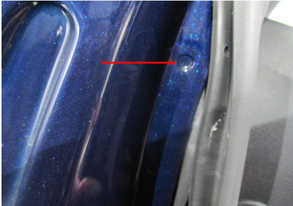
Photo 32 shows the left side "A" pillar of the Motor Car. I did not find any weld marks other than original spot weld marks (arrowed) on the left side "A" pillar of the Motor Car, which indicates that there was no re-welding works carried out. In general, I had found all the non-detachable body panels of the Motor Car to be originally fitted at the time of my inspection.
