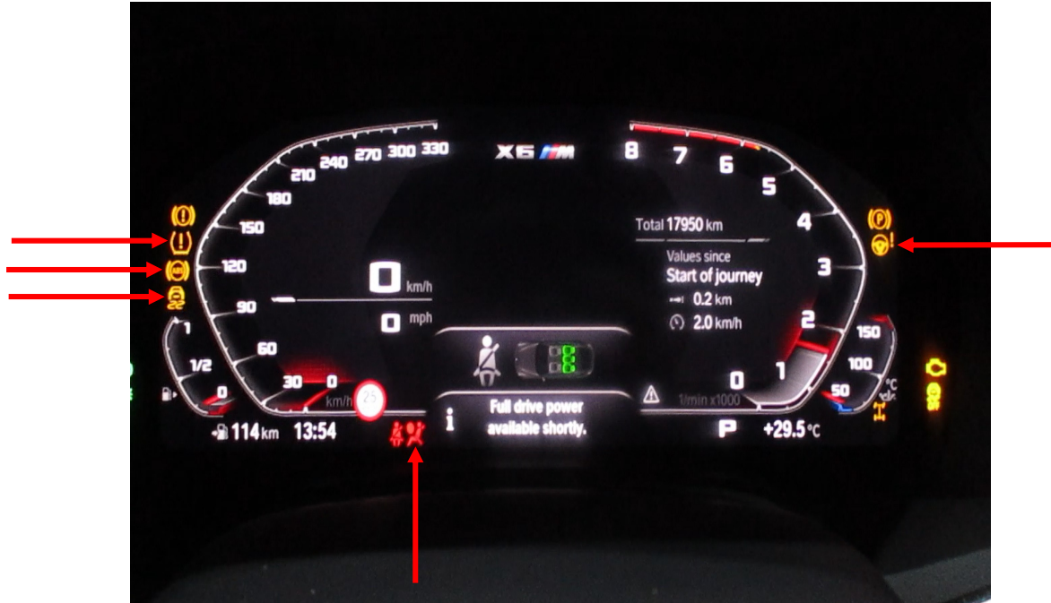
Photo 18 shows the warning lights for the various electronic safety features appearing on the instrument panel of the Motor Car during its self-test when the engine is cranked, in particular the ABS, SRS, IAS, TPM and DSC lights (arrowed).
