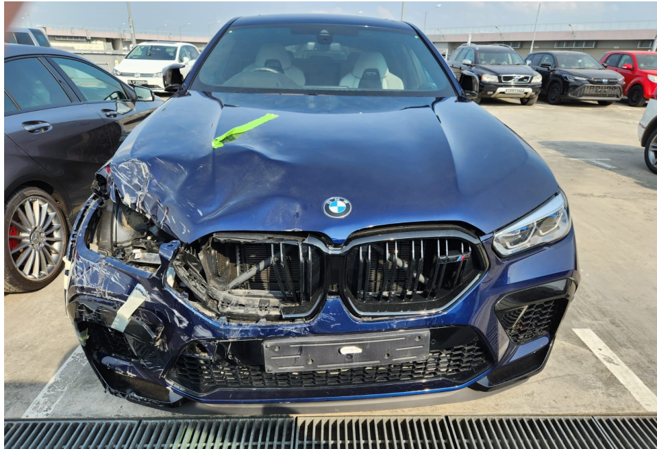
Photo 1 shows the frontal body of the Motor Car (photograph provided to me). The photographs provided to me had showed damage to the front right portion of the Motor Car. The front bumper, front bumper centre garnish, front bumper centre lower grille, front bumper right sensors, front number plate garnish, front right headlamp, radiator grilles and front bonnet were amongst the body parts that were observed to have been damaged.
