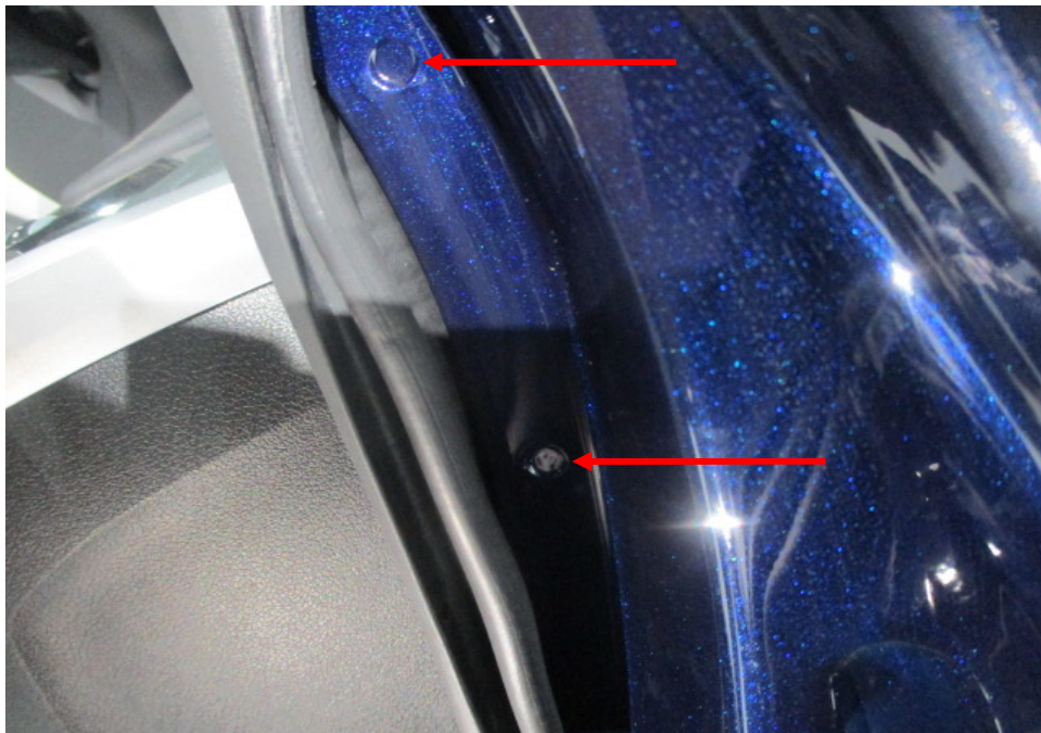
Photo 33 shows the right side "A" pillar of the Motor Car. I did not find any weld marks other than original spot weld marks (arrowed) on the right side "A" pillar of the Motor Car, which indicates that there was no re-welding works carried out. In general, I had found all the non-detachable body panels of the Motor Car to be originally fitted at the time of my inspection.
