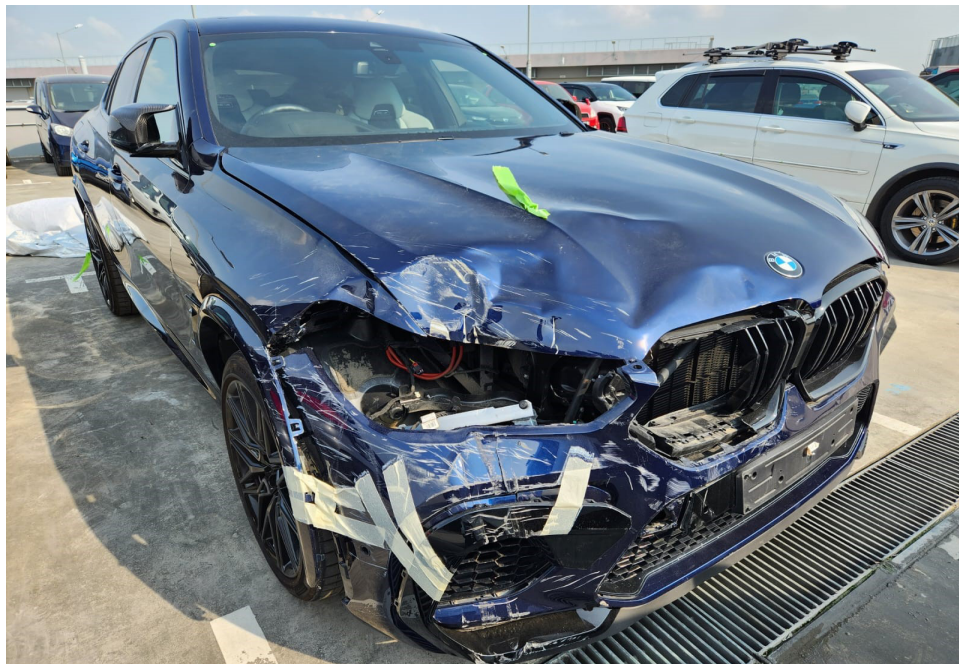
Photo 2 shows the front right body of the Motor Car (photograph provided to me). The photographs provided to me had showed damage to the front right portion of the Motor Car. The front bumper, front bumper lower lip, front bumper right lower garnish, front bumper right lower grille, front bumper right reflector, front right headlamp, front right fender, front right fender wheel arc garnish and front bonnet were amongst the body parts that were observed to have been damaged.
