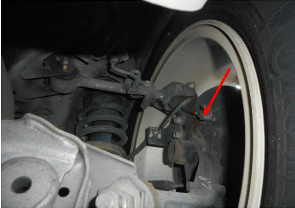
Photo 28 shows the brake hose/pipe (arrowed) at the rear right wheel of the Motor Car. No leakage of brake fluid was observed. Visual examination of the various components of the braking system like the drum brake, brake booster, brake pedal etc. had revealed all to be intact and without visible damage.
