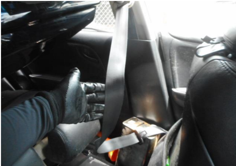
Photo 30 shows that the seat belt on the left seat was worn at the material time of accident as the safety pre-tensioners was activated at the moment of impact and caused the seat belt to be locked into the last position.
