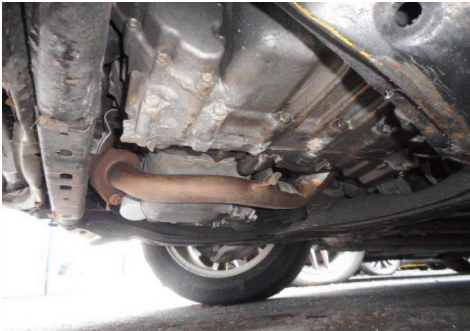
Photo 21 shows the undercarriage of the Motor Car, at the area where the engine housing and transmission housing are located. I did not find any sign(s) or indication(s) of fluid leak and/or fluid stain(s) on the underside of the Motor Car.
