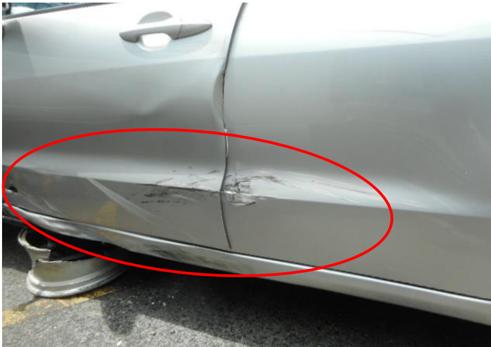
Photo 8 shows a close up view of the Motor Car's left body at the time of my inspection. The Motor car was observed to have sustained damage at its left portion. Its left door (circled) was damaged as a result of the accident.
