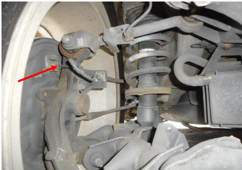
Photo 27 shows the brake hose/pipe (arrowed) at the rear left wheel of the Motor Car. No leakage of brake fluid was observed. Visual examination of the various components of the braking system like the drum brake, brake booster, brake pedal etc. had revealed all to be intact and without visible damage.
