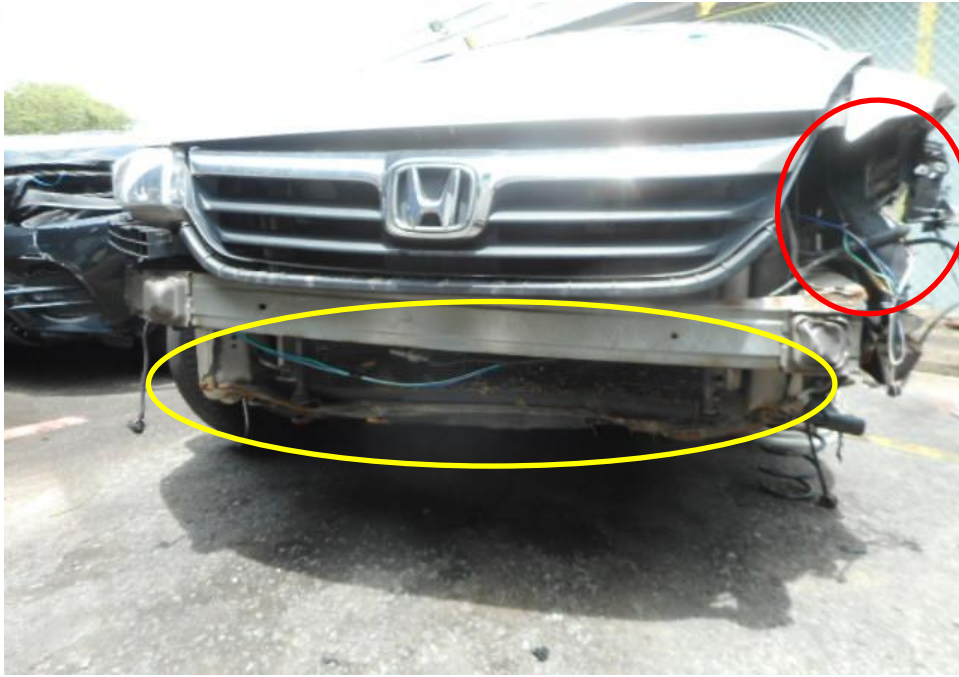
Photo 5 shows the close up view of the Motor Car's front body at the time of my inspection. The Motor car was observed to have sustained damage at its front portion. Its front bumper (yellow circle) and its front left headlamp (red circle) was damaged as a result of the accident.
