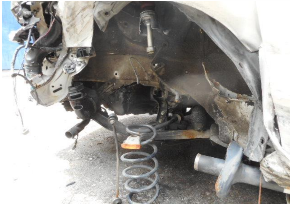
Photo 11 shows the location of where the front left tyre and wheel rim of the Motor Car should be, however observed that the wheel rim was broken off and tyre was missing as a result of the accident.
