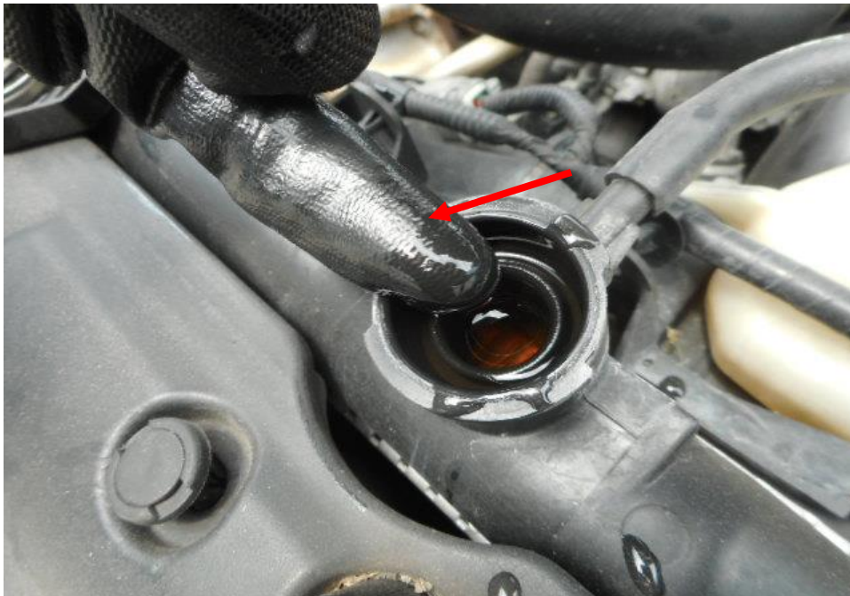
Photo 19 shows the engine coolant reservoir of the Motor Car at the time of my inspection. The coolant was observed to be of sufficient level (arrowed) and without any visible contamination.
