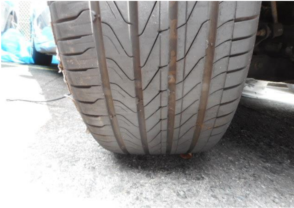
Photo 15 shows the condition of the front right tyre of the Motor Car, which was observed to be in serviceable condition with remaining tread depth of approximately 5.6mm. The tyre was also observed to be sufficiently inflated for vehicular operation with no tear, cut or burst mark(s).
