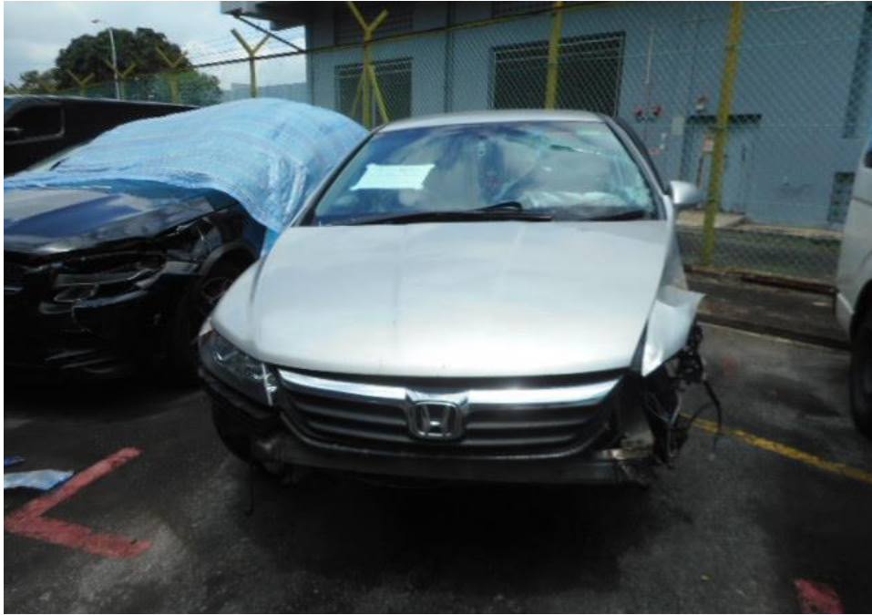
Photo 3 shows a general view of the Motor Car's front body at the time of my inspection. The Motor car was observed to have sustained damage at its front portion. Its front windscreen, front bumper, front left fender, front left headlamp was the body parts that were damaged as a result of the accident.
