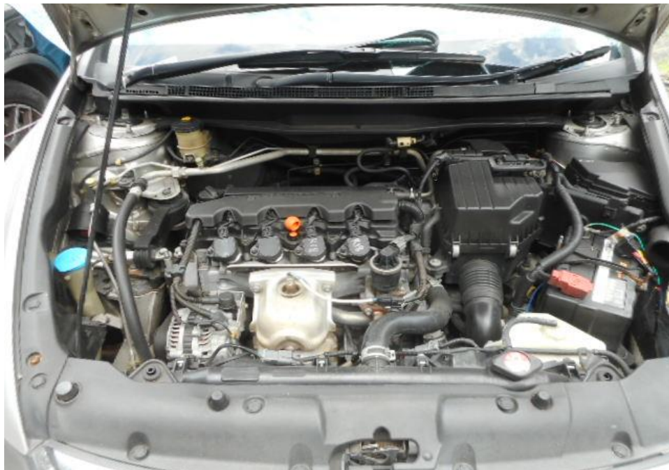
Photo 17 shows a general view of the Motor Car's engine compartment. Only the brake fluid in the reservoir was observed to be insufficient due to the missing brake caplier and broken brake hose at the front left wheel as a result of the accident. The other various parts and components inside the engine compartment were unaffected by the accident. There was also no sign(s) or indication(s) of fluid leakage and/or fluid stain within the engine compartment.
