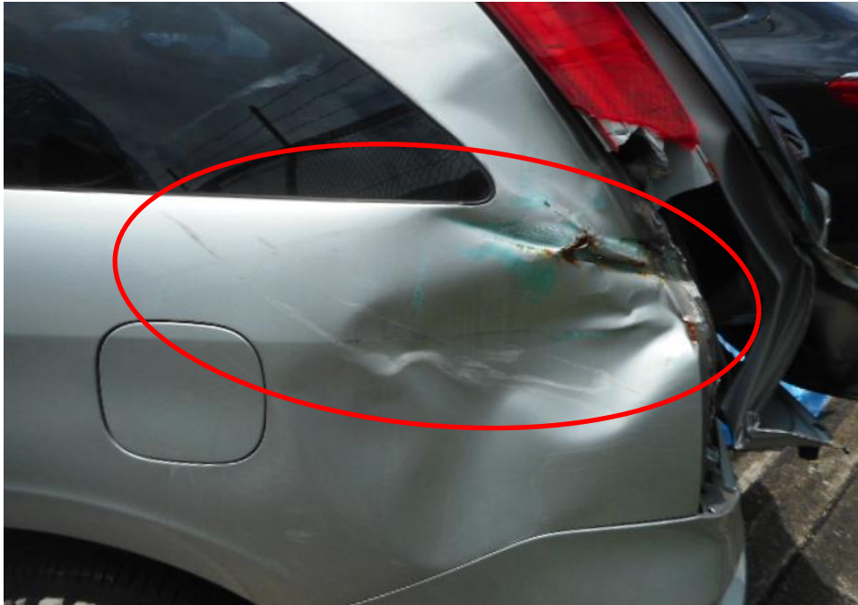
Photo 9 shows a close up view of the Motor Car's left body at the time of my inspection. The Motor car was observed to have sustained damage at its left portion. Its left body panel (circled) was damaged as a result of the accident.
