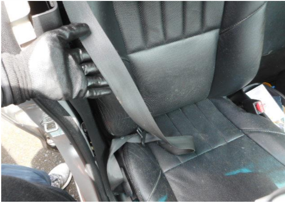
Photo 29 shows that the seat belt on the right seat was worn at the material time of accident as the safety pre-tensioners was activated at the moment of impact and caused the seat belt to be locked into the last position.
