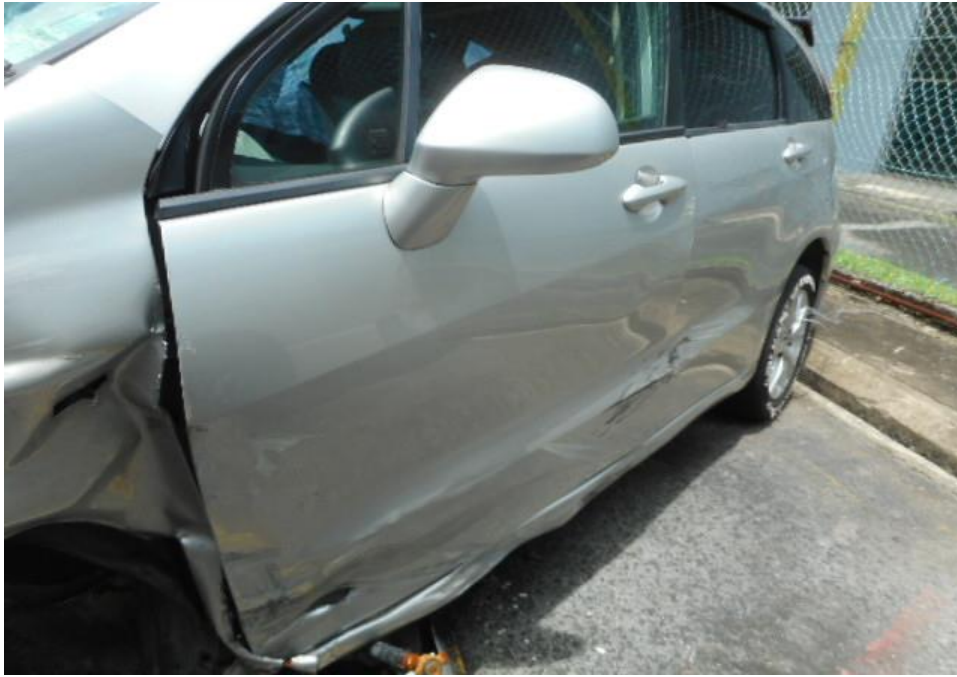
Photo 7 shows a general view of the Motor Car's left body at the time of my inspection. The Motor car was observed to have sustained damage at its left portion. Its left door and left body panel was damaged as a result of the accident.
