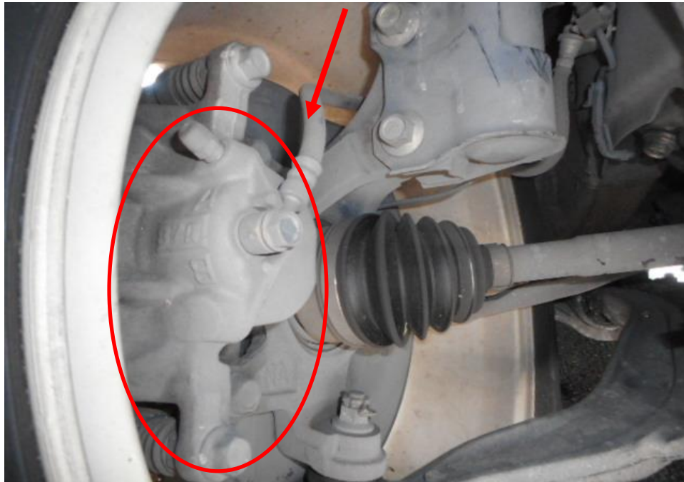
Photo 26 shows the brake hose/pipe (arrowed) at the front right wheel of the Motor Car. No leakage of brake fluid was observed. Visual examination of the various components of the braking system like the brake caliper (circled), brake booster, brake pedal etc had revealed all to be intact and without visible damage.
