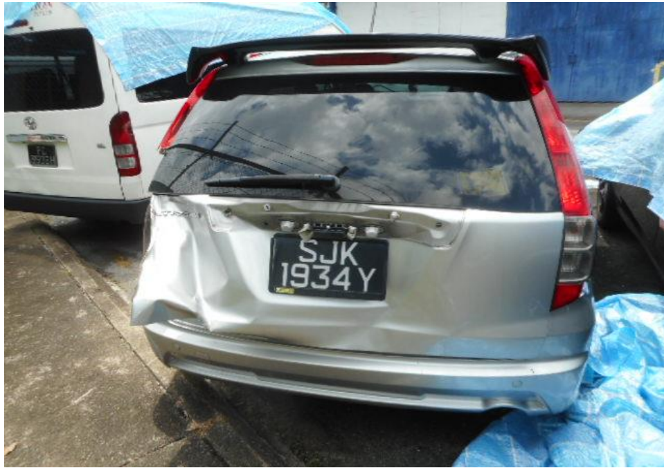
Photo 1 shows a general view of the Motor Car's rear body at the time of my inspection. The Motor car was observed to have sustained damage at its rear portion. Its rear boot and rear left brake lamp was the body parts that were damaged as a result of the accident.
