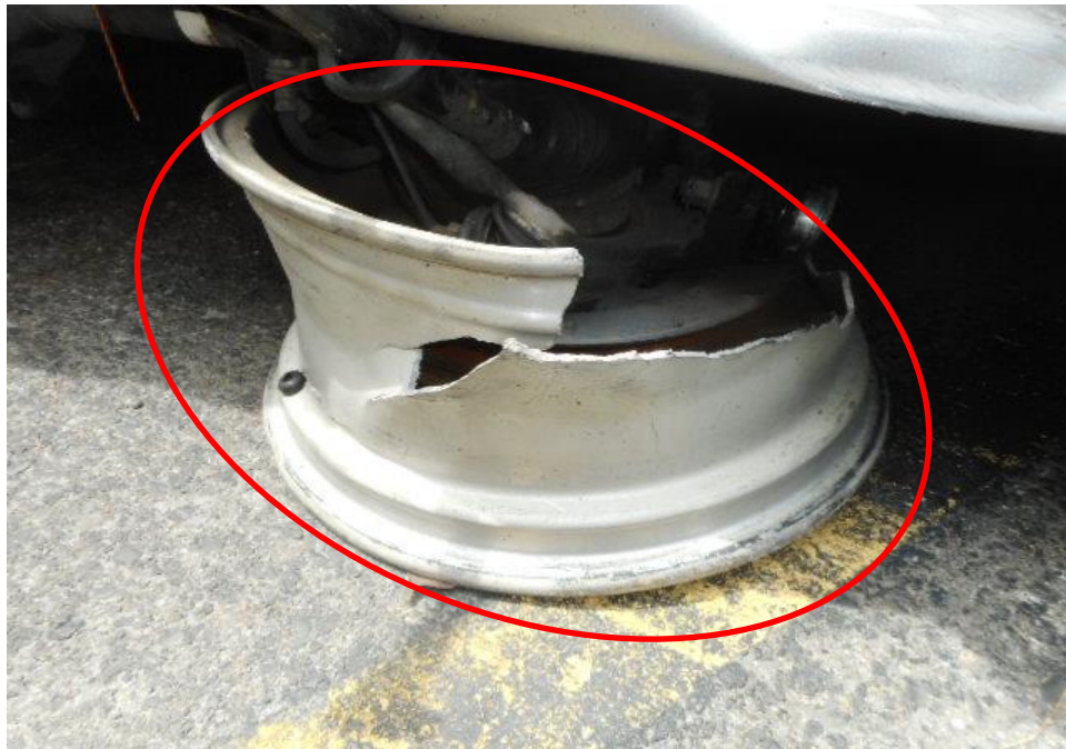
Photo 12 shows the front left wheel rim of the Motor Car observed that the wheel rim was broken off and damaged (circled) and the tyre was missing as a result of the accident.
