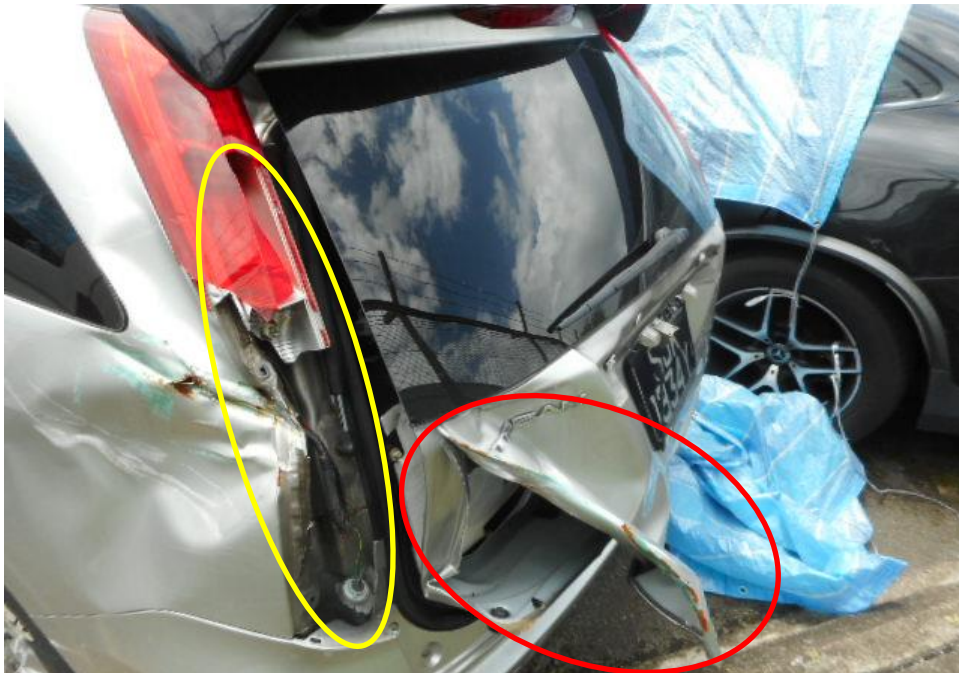
Photo 2 shows the close up view of the Motor Car's rear body at the time of my inspection. The Motor car was observed to have sustained damage at its rear portion. Its rear boot (red circle) and its rear left brake lamp (yellow circle) was damaged as a result of the accident.
