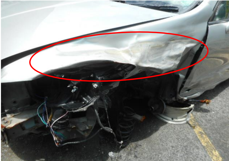
Photo 6 shows the close up view of the Motor Car's front body at the time of my inspection. The Motor car was observed to have sustained damage at its front portion. Its front left fender (red circle) was damaged as a result of the accident.
