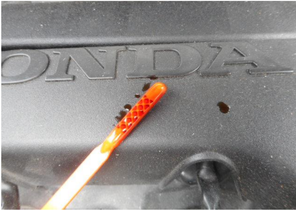
Photo 20 shows the engine oil level dipstick of the Motor Car at the time of my inspection. The engine oil was observed to be of sufficient level and without any visible contamination.
