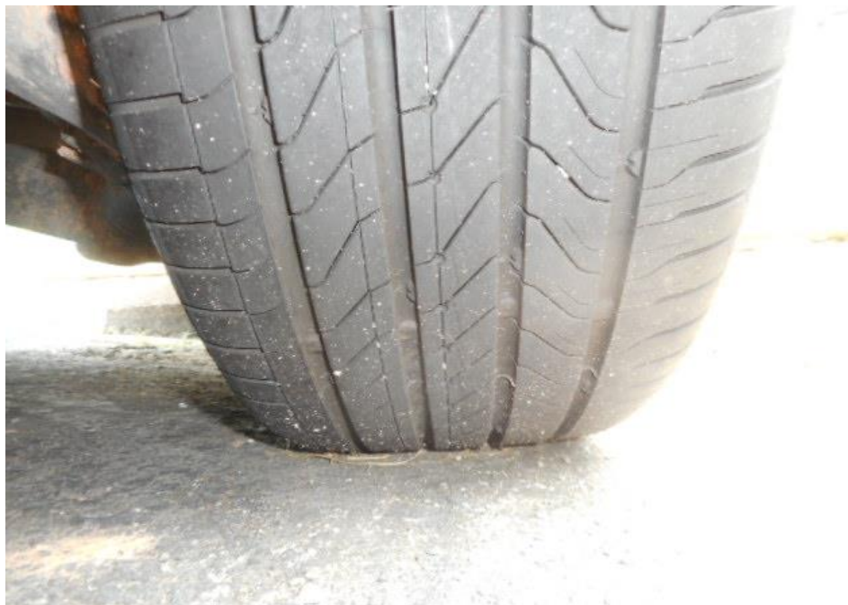
Photo 14 shows the condition of the rear right tyre of the Motor Car, which was observed to be in serviceable condition with remaining tread depth of approximately 4.7mm. The tyre was also observed to be sufficiently inflated for vehicular operation with no tear, cut or burst mark(s).
