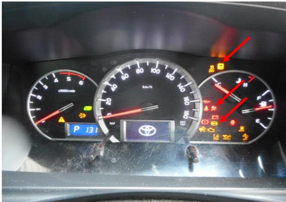
Photo 24 shows the warning light for Anti-Lock Brake System (ABS), Traction Control System (TCS) and Supplemental Restraint System (SRS) (arrowed) appearing on the instrument panel of the Motor Van during the self-test of its various electronic operating systems when its engine was cranked.
