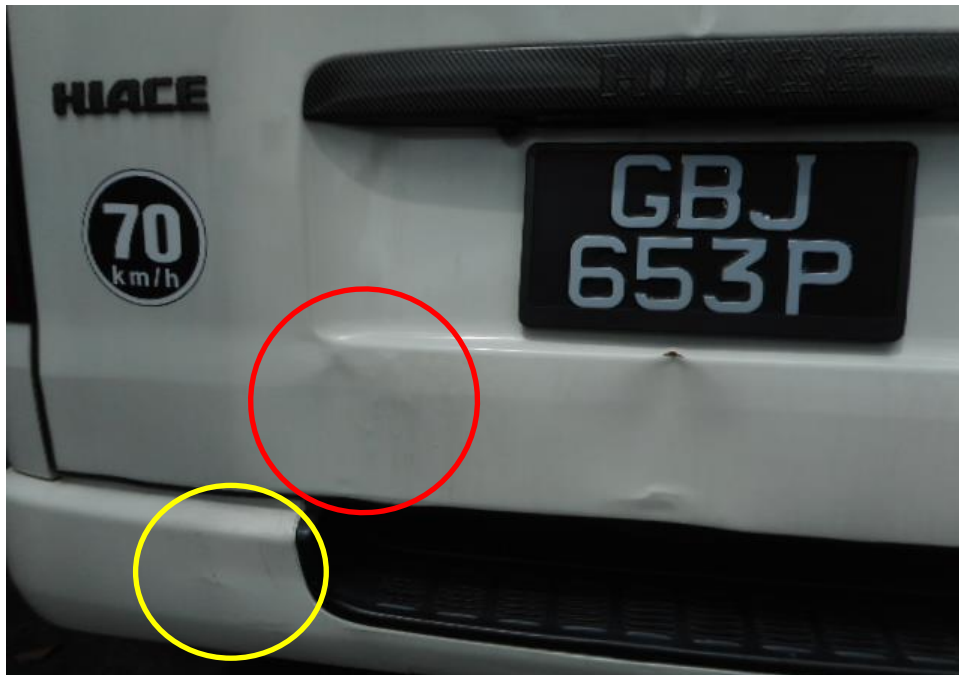
Photo 3 shows a close up view of the Motor Van's rear portion at the time of my inspection. It appeared to have sustained damage at its rear portion. Its rear bumper (yellow circle) and rear body panel (red circle) was damage at the time of my inspection as a result of the accident.
