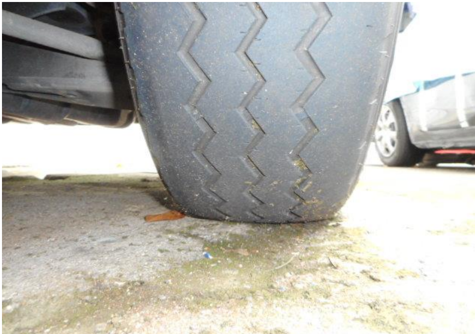
Photo 7 shows the condition of the front right tyre of the Motor Van, which was observed to be in serviceable condition with remaining tread depth of approximately 2.8mm. The tyre, which was wrapped around standard steel wheel rim, was also observed to be sufficiently inflated for vehicular operation. There was no tear, cut or burst mark(s) on the outer and the inner sidewalls as well as across the tread of the 4 tyres that were fitted on the Motor Van.
