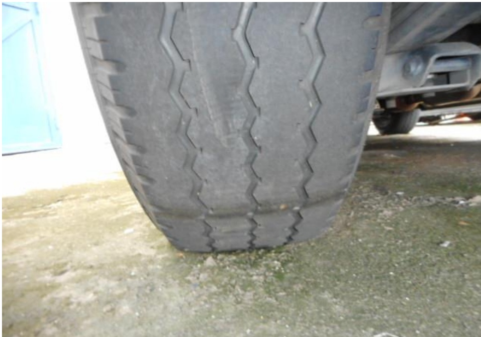
Photo 9 shows the condition of the rear left tyres of the Motor Van, which was observed to be in serviceable condition with remaining tread depth of approximately 2.4mm. The tyres, which were wrapped around standard steel wheel rim, were also observed to be sufficiently inflated for vehicular operation. There was also no damage found on all 4 steel wheel rims of the Motor Van.
