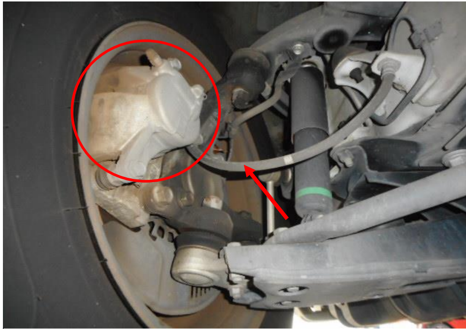
Photo 22 shows the brake hose/pipe (arrowed) at the front left wheel of the Motor Van. No leakage of brake fluid was observed. Visual examination of the various components of the braking system like the brake caliper (circled), brake booster, brake pedal etc had revealed all to be intact and without visible damage at the time of accident. There was also no sign of fluid stain(s) observed on the various undercarriage components.
