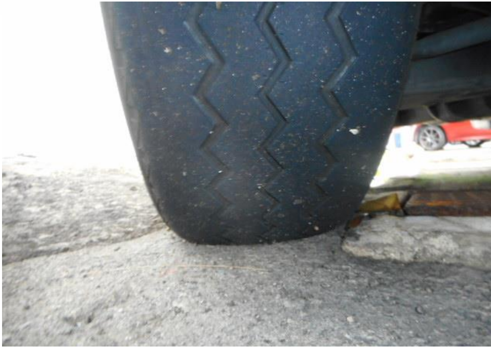
Photo 10 shows the condition of the rear right tyres of the Motor Van, which were observed to be in serviceable condition with remaining, tread depth of approximately 2.8mm. There was also no tear, cut or burst mark(s) on the outer and the inner sidewalls as well as across the tread of the 4 tyres that were fitted on the Motor Van.
