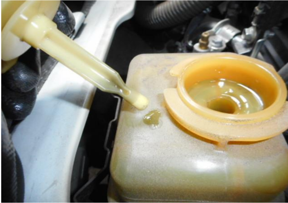
Photo 15 shows the power steering fluid dip stick of the Motor Van at the time of my inspection. The steering fluid was observed to be of sufficient level and without any visible contamination.
