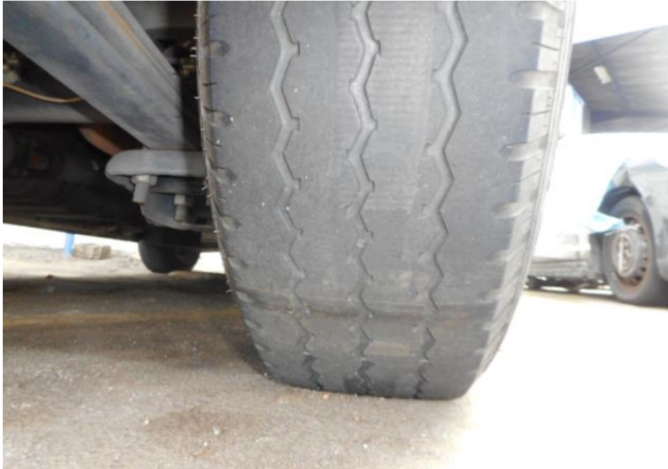
Photo 8 shows the condition of the rear right tyre of the Motor Van, which was observed to be in serviceable condition with remaining tread depth of approximately 1.9mm. The tyre, which was wrapped around standard steel wheel rim, it was observed to be sufficiently inflated for vehicular operation.
