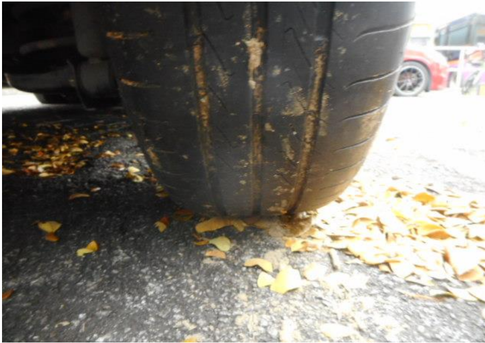
Photo 8 shows the condition of the rear right tyre of the Motor Car, which was observed to be in serviceable condition with remaining tread depth of approximately 4.6mm. The tyre was also observed to be sufficiently inflated for vehicular operation with no tear, cut or burst mark(s).
