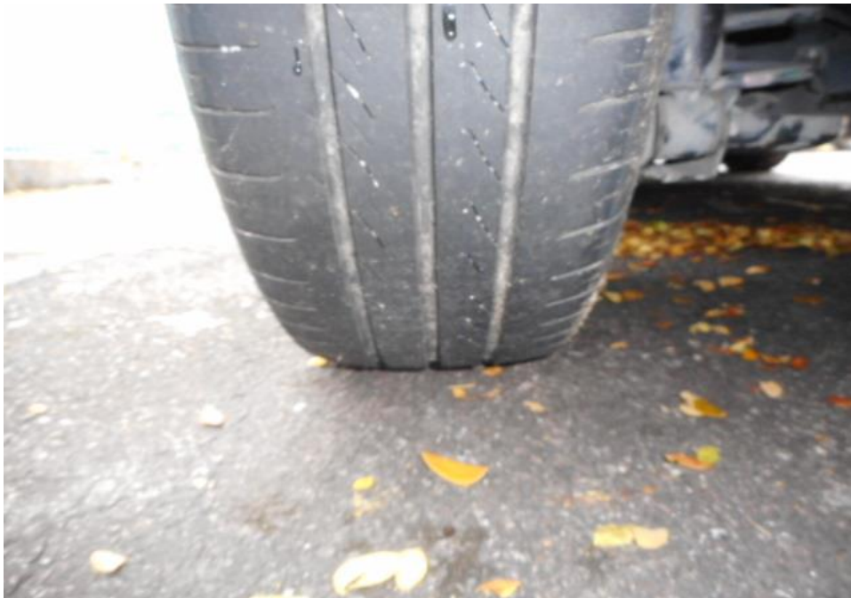
Photo 9 shows the condition of the rear left tyre of the Motor Car, which was observed to be in serviceable condition with remaining tread depth of approximately 4.1mm. The tyre, which was wrapped around steel wheel rim, was also observed to be sufficiently inflated for vehicular operation. The 3 tyres of the Motor Car were wrapped around standard steel wheel rims.
