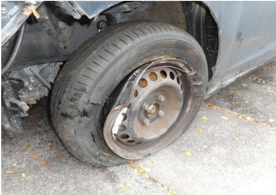
Photo 10 shows the general condition of the front left tyre of the Motor Car, which was observed to be in unserviceable condition with remaining tread depth of approximately 6mm. There was also cut mark(s) on the outer sidewalls of the Motor Car's tyre and the wheel rim was also damaged as a result of the accident.
