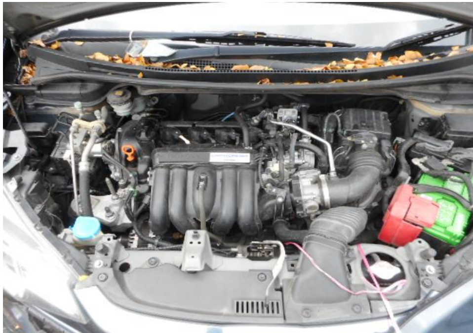
Photo 12 shows a general view of the Motor Car's engine compartment. The various parts and components inside the engine compartment were unaffected by the accident. There was also no sign(s) or indication(s) of fluid leakage and/or fluid stain within the engine compartment.
