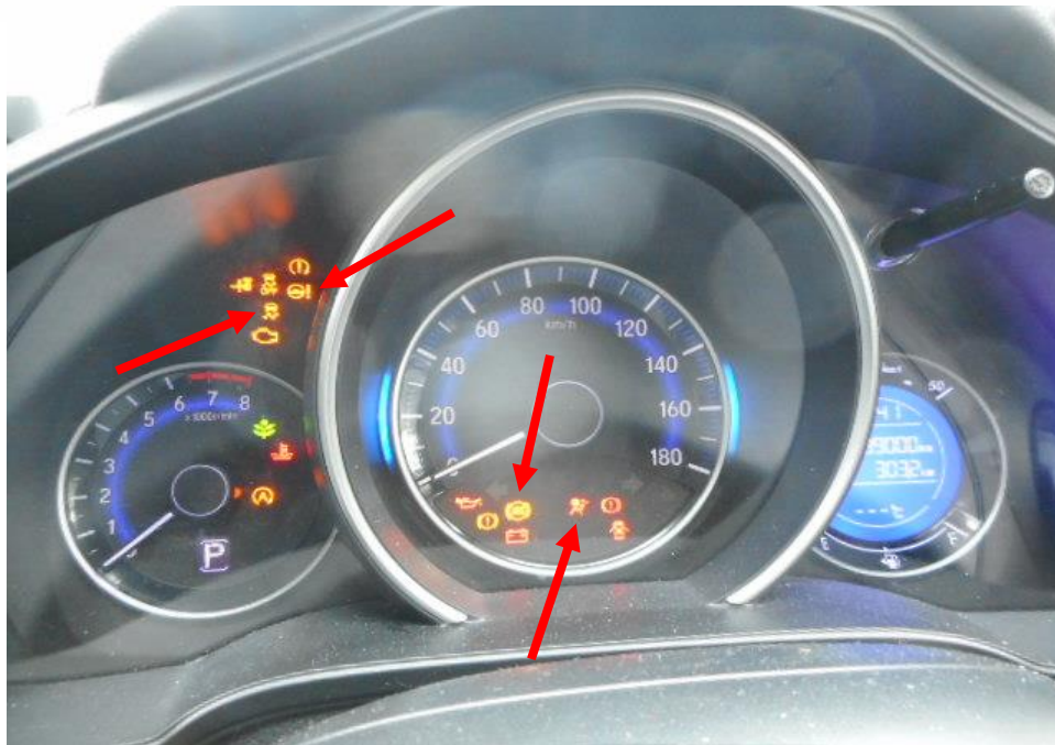
Photo 23 shows the warning light for Anti-Lock Brake System (ABS), Traction Control System (TCS), Electric Power Steering System (EPS) and Supplemental Restraint System (SRS) (arrowed) appearing on the instrument panel of the Motor Car during the self-test of its various electronic operating systems when its engine was cranked.
