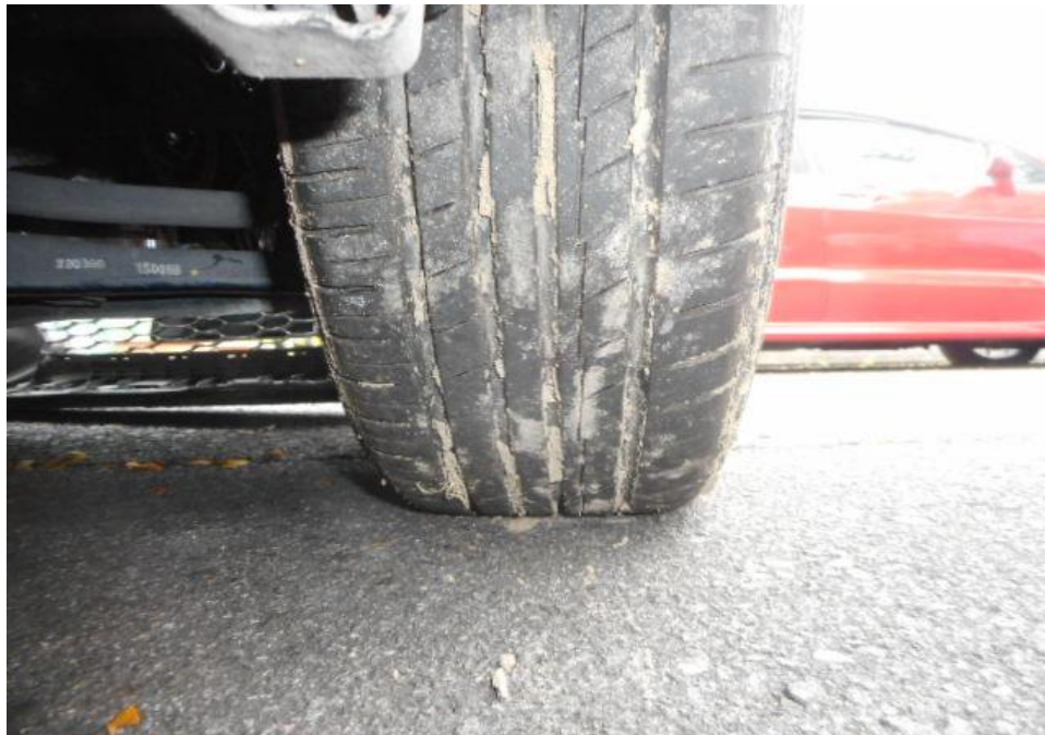
Photo 7 shows the condition of the front right tyre of the Motor Car, which was observed to be in serviceable condition with remaining tread depth of approximately 5.6mm. The tyre was sufficiently inflated for vehicular operation with no tear, cut or burst mark(s) on the outer and the inner sidewalls as well as across the tread. The 3 tyres of the Motor Car were wrapped around standard steel wheel rims without any damage.
