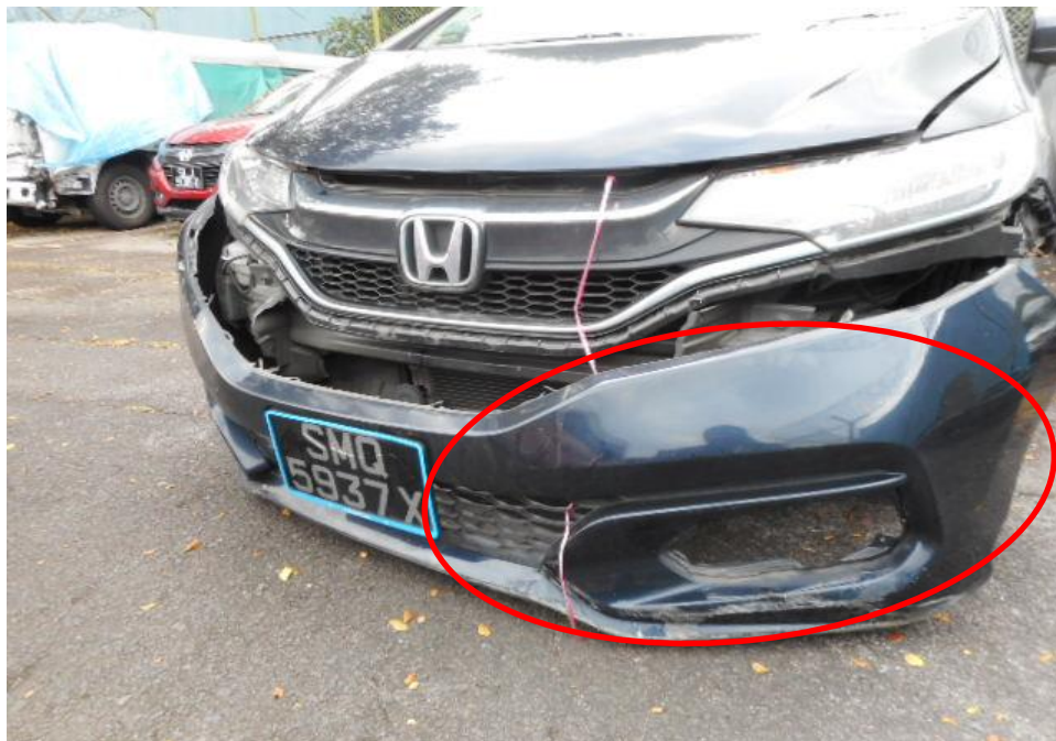
Photo 3 shows a close up view of the Motor Car's front body at the time of my inspection. The front portion of the Motor Car was observed to have sustained damage. Its front bumper (circled) was the body parts that were damaged as a result of the accident.
