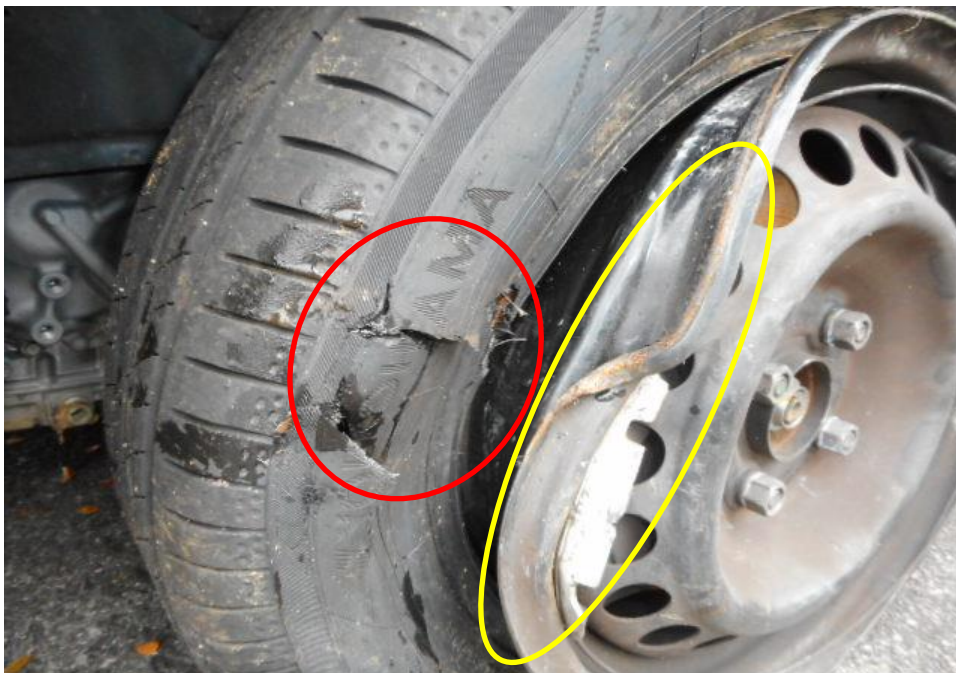
Photo 11 shows the close up condition of the front left tyre of the Motor Car, which was observed to be in unserviceable condition with remaining tread depth of approximately 6mm. There was also cut mark (red circle) on the outer sidewalls of the Motor Car's tyre and the wheel rim (yellow circle) was also damaged as a result of the accident.
