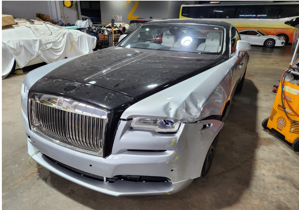
Photo 1 shows the front left body of the Motor Car (photograph provided to me). The photographs provided to me had showed damage to the front left portion of the Motor Car. The front bumper, front bumper left reflector, front left headlamp, front left fender and front bonnet were amongst the body parts that were observed to have been damaged. The front bumper sensors, front bumper left lower chrome moulding and front left day light were also observed to be missing/dislodged/damaged.
