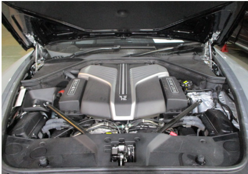
Photo 13 shows a general view of the Motor Car's engine compartment at the time of my inspection. The various parts and components inside the engine compartment were all observed to be intact and properly fitted. There was also no sign(s) or indication(s) of fluid leak and/or fluid stain found inside the engine compartment.
