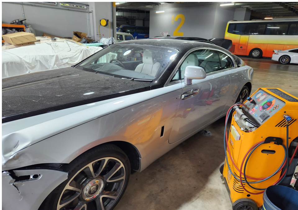
Photo 2 shows the left side front portion of the Motor Car (photograph provided to me). The front bumper, front bumper left reflector and front left fender were amongst the body parts that were observed to have been damaged. The front left fender emblem was also observed to be missing/dislodged/damaged.
