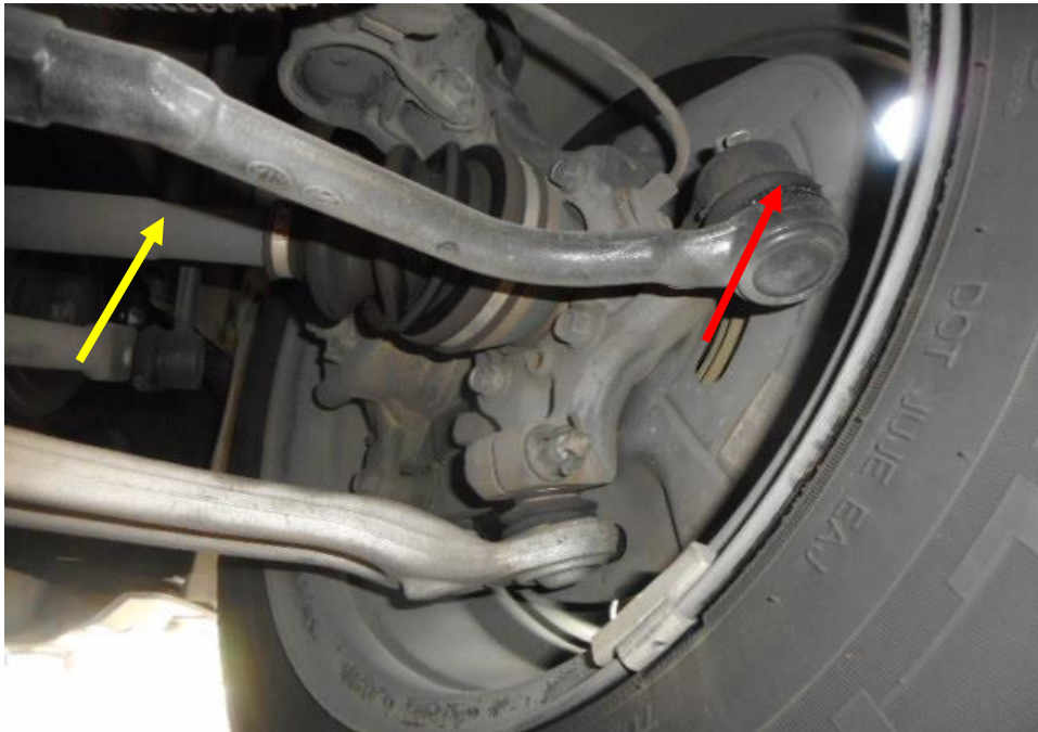
Photo 24 shows the various undercarriage components at the front right wheel of the Motor Taxi, in particular the steering tie rod (red arrow) and drive shaft (yellow arrow). The various steering components were all found to be intact, suggesting that the steering system of the Motor Taxi was likely to be in serviceable condition at the material time of accident. There was also no sign of fluid stain observed on the various undercarriage components at the front right wheel of the Motor Taxi.
