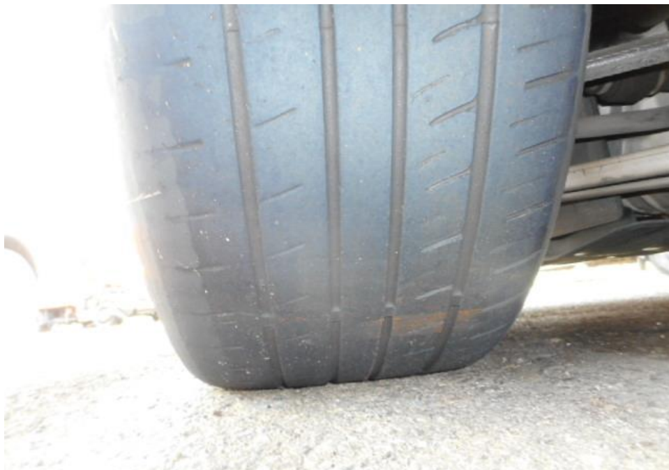
Photo 13 shows the condition of the front left tyre of the Motor Taxi, which was observed to be in serviceable condition with remaining tread depth of approximately 2.4mm. There was also no tear, cut or burst mark(s) on the outer and the inner sidewalls as well as across the tread of the Motor Taxi's 4 tyres.
