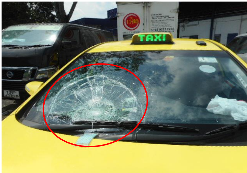
Photo 3 shows a close up view of the Motor Taxi's front body at the time of my inspection. The front portion of the Motor Taxi was observed to have sustained damage. Its front windscreen (circled) was the body parts that were damaged as a result of the accident.
