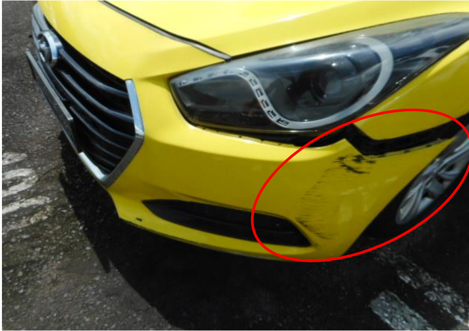
Photo 6 shows a close up view of the Motor Taxi's front body at the time of my inspection. The front portion of the Motor Taxi was observed to have sustained damage. Its front bumper (circled) was the body parts that were damaged as a result of the accident.
