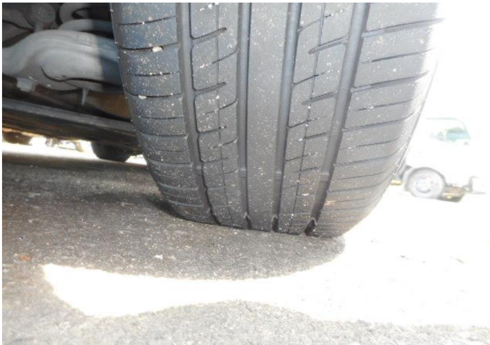
Photo 11 shows the condition of the rear right tyre of the Motor Taxi, which was observed to be in serviceable condition with remaining tread depth of approximately 6.1mm. The tyre was also observed to be sufficiently inflated for vehicular operation with no tear, cut or burst mark(s).
