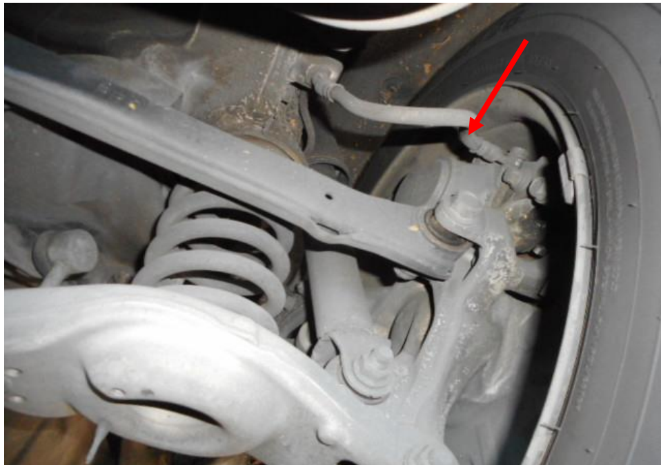
Photo 19 shows the brake hose/pipe (arrowed) at the rear right wheel of the Motor Taxi. No leakage of brake fluid was observed. Visual examination of the various components of the braking system like the drum brake, brake booster, brake pedal etc. had revealed all to be intact and without visible damage.
