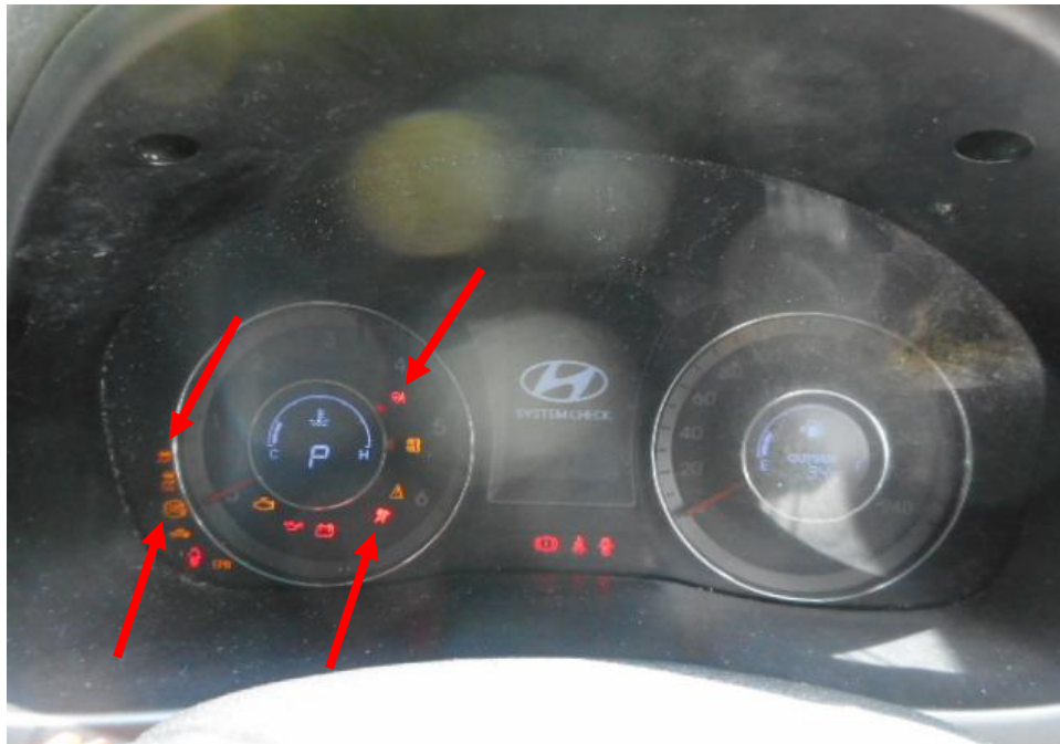
Photo 26 shows the warning light for Anti-Lock Brake System (ABS), Electric Power Steering System (EPS), Traction Control System (TCS) and Supplemental Restraint System (SRS) (arrowed) appearing on the instrument panel of the Motor Taxi during the self-test of its various electronic operating systems when its engine was cranked.
