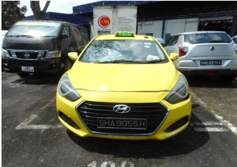
Photo 2 shows a general view of the Motor Taxi's front body at the time of my inspection. The front portion of the Motor Taxi was observed to have sustained damage. Its front windscreen, front bonnet, front bumper and front grille was amongst the body parts that were damaged as a result of the accident.
