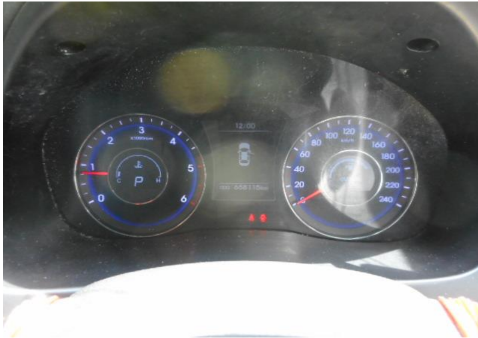
Photo 27 shows no warning lights illuminated on the instrument panel of the Motor Taxi after the engine was cranked. This would suggest that there was no abnormality to the electronic operating system of the Motor Taxi, like the ABS, EPS, TCS and SRS etc.
