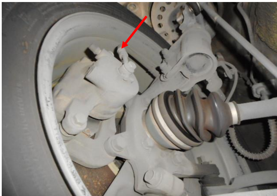
Photo 21 shows the brake hose/pipe (arrowed) at the front right wheel of the Motor Taxi. I did not observe any leakage of brake fluid at the time of my inspection of the Motor Taxi. Static tests of the Motor Taxi's braking system had indicated that there was no internal leakage of pressure/vacuum. The undercarriage components of the Motor Taxi were also all found to be intact and without any visible damage.
