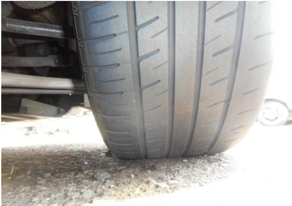
Photo 10 shows the condition of the front right tyre of the Motor Taxi, which was observed to be in serviceable condition with remaining tread depth of approximately 3.2mm. The tyre was sufficiently inflated for vehicular operation with no tear, cut or burst mark(s) on the outer and the inner sidewalls as well as across the tread. The 4 tyres of the Motor Taxi were wrapped around standard steel wheel rims without any damage.
