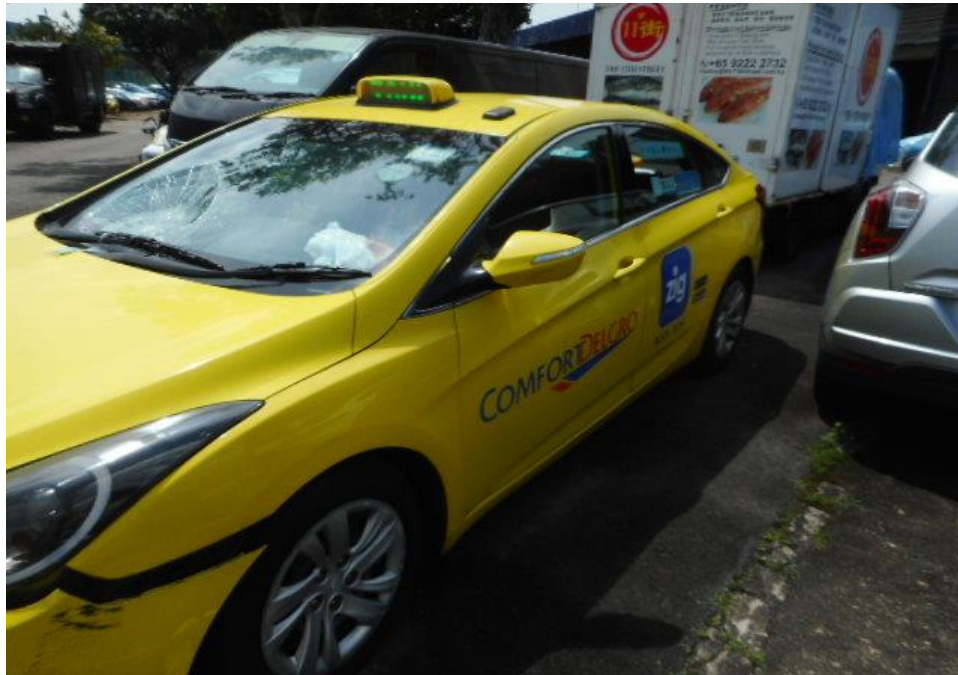
Photo 8 shows a general view of the Motor Taxi's left body at the time of my inspection. The left portion of the Motor Taxi was observed to have been unaffected by the accident.
