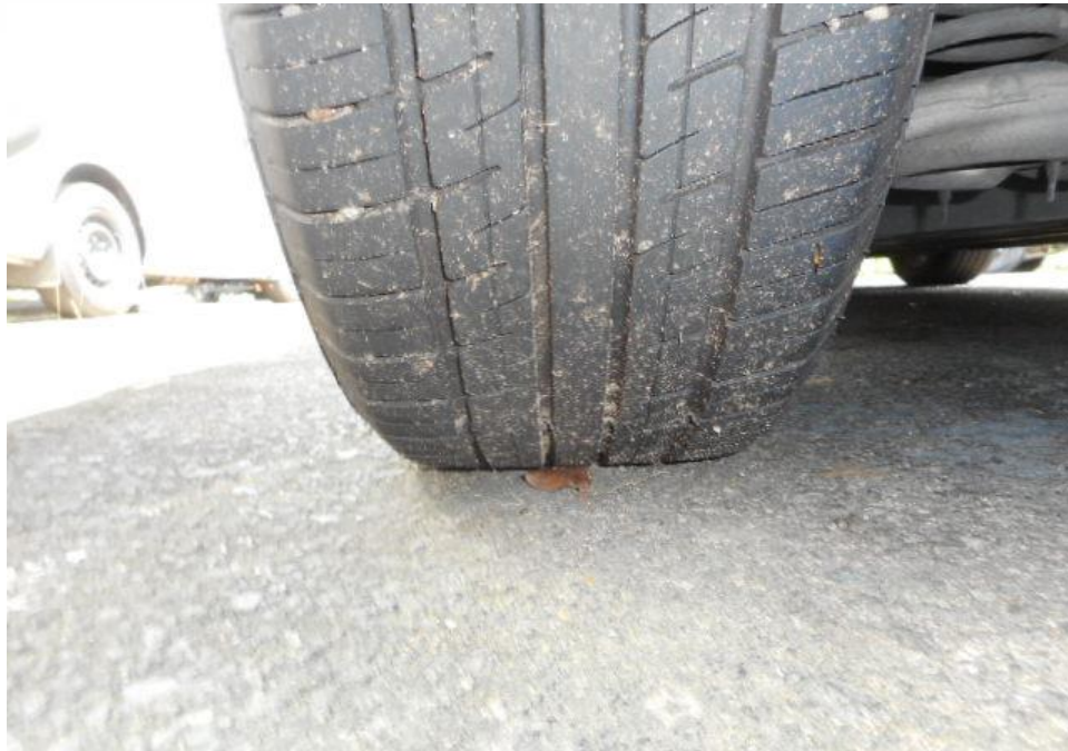
Photo 12 shows the condition of the rear left tyre of the Motor Taxi, which was observed to be in serviceable condition with remaining tread depth of approximately 5.6mm. The tyre, which was wrapped around steel wheel rim, was also observed to be sufficiently inflated for vehicular operation. The 4 tyres of the Motor Taxi were wrapped around standard steel wheel rims.
