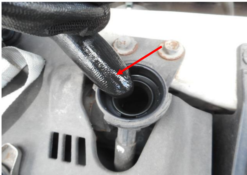
Photo 14 shows checks being carried out to the engine coolant of the Motor Car at the time of my inspection. The engine coolant was observed to be of sufficient level (arrowed) and without any visible contamination.
