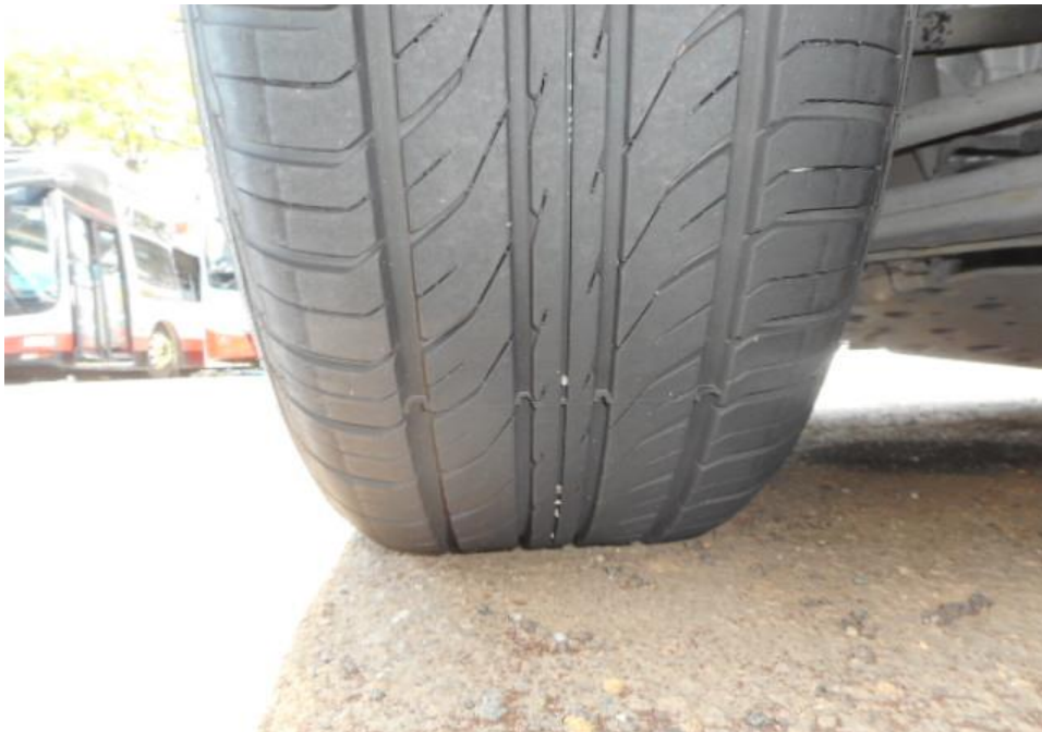
Photo 11 shows the condition of the front left tyre of the Motor Car, which was observed to be in serviceable condition with remaining tread depth of approximately 5.6mm. There was also no tear, cut or burst mark(s) on the outer and the inner sidewalls as well as across the tread of the Motor Car's 4 tyres.
