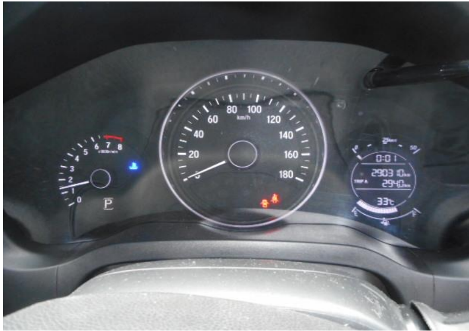
Photo 25 shows no warning lights illuminated on the instrument panel of the Motor Car after the engine was cranked. This would suggest that there was no abnormality to the electronic operating system of the Motor Car, like the ABS, EPS, TCS and SRS etc.
