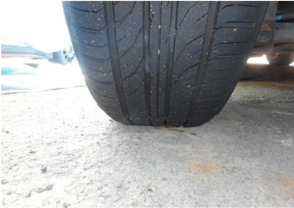
Photo 10 shows the condition of the rear left tyre of the Motor Car, which was observed to be in serviceable condition with remaining tread depth of approximately 4.4mm. The tyre, which was wrapped around alloy wheel rim, was also observed to be sufficiently inflated for vehicular operation. The 4 tyres of the Motor Car were wrapped around standard alloy wheel rims.
