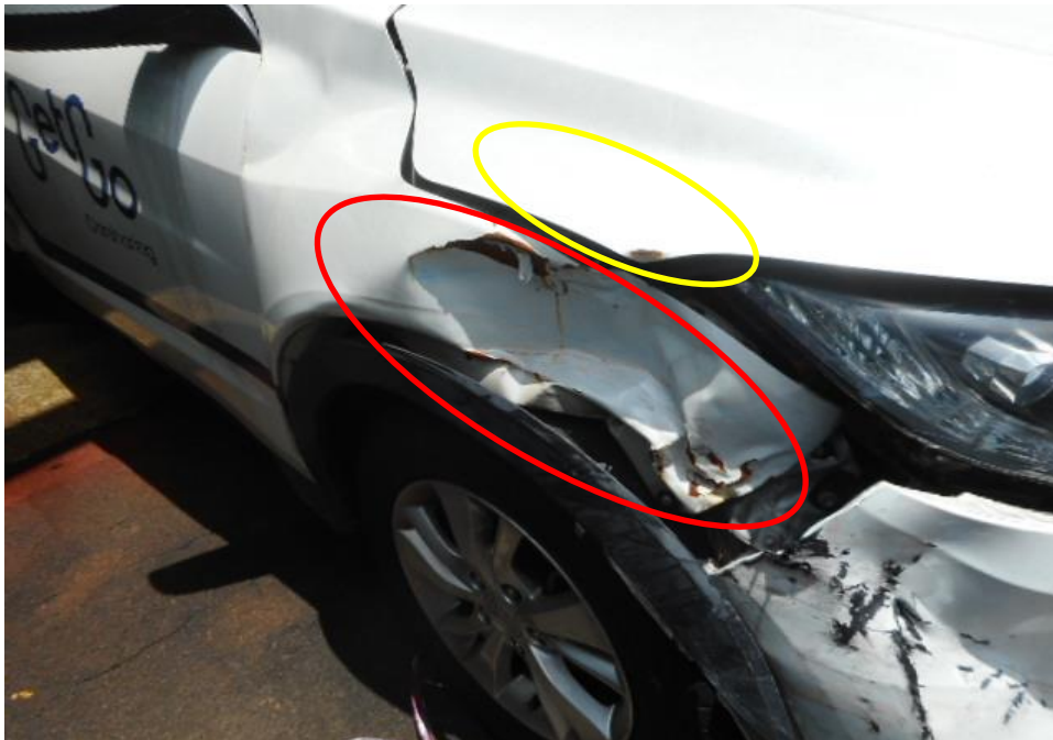
Photo 3 shows a close up view of the Motor Car's front body at the time of my inspection. The front portion of the Motor Car was observed to have sustained damage. Its front bonnet (yellow circle) and front right fender (red circle) was the body parts that were damaged as a result of the accident.
