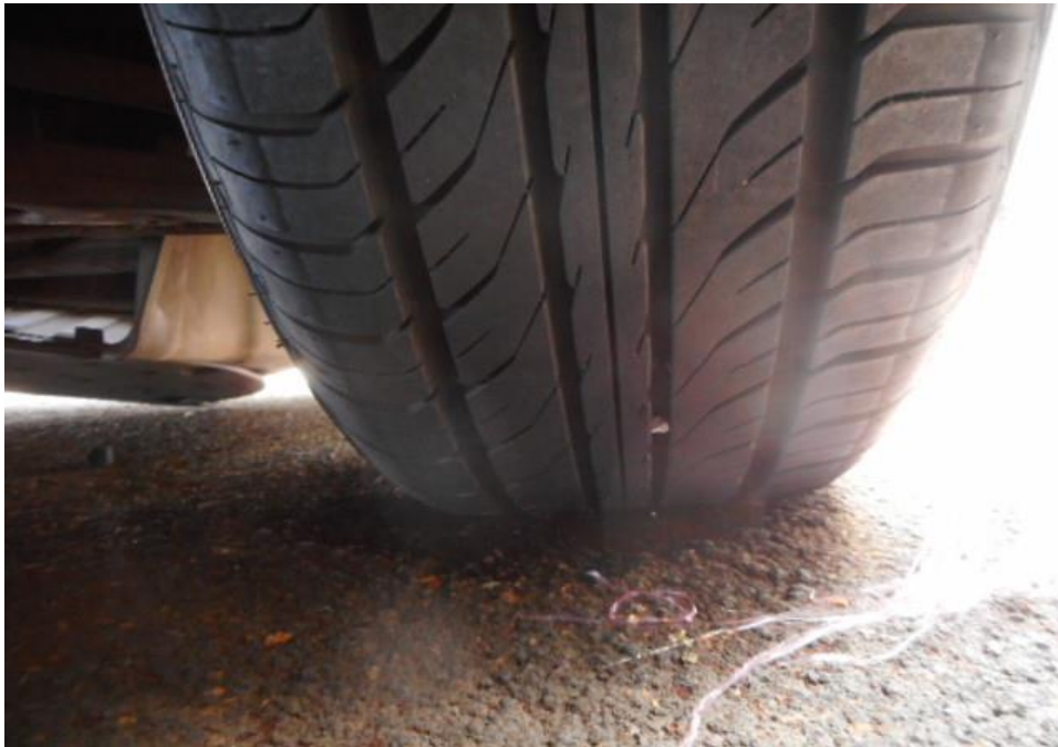
Photo 8 shows the condition of the front right tyre of the Motor Car, which was observed to be in serviceable condition with remaining tread depth of approximately 5.6mm. The tyre was sufficiently inflated for vehicular operation with no tear, cut or burst mark(s) on the outer and the inner sidewalls as well as across the tread. The 4 tyres of the Motor Car were wrapped around standard alloy wheel rims without any damage.
