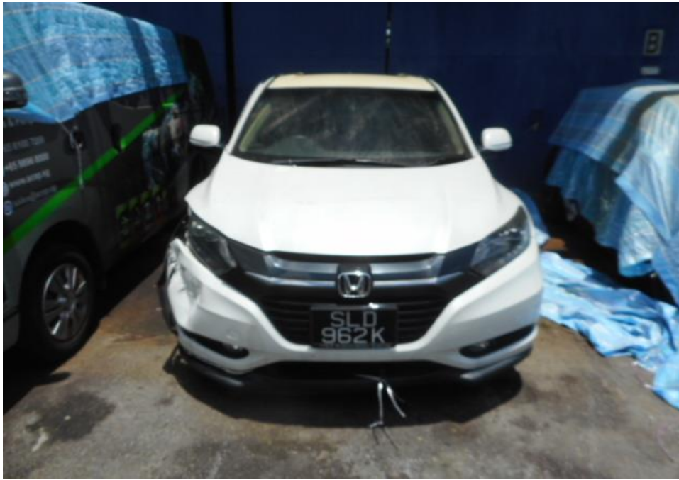
Photo 2 shows a general view of the Motor Car's front body at the time of my inspection. The front portion of the Motor Car was observed to have sustained damage. Its front bonnet, front bumper, front right fender was amongst the body parts that were damaged as a result of the accident.
