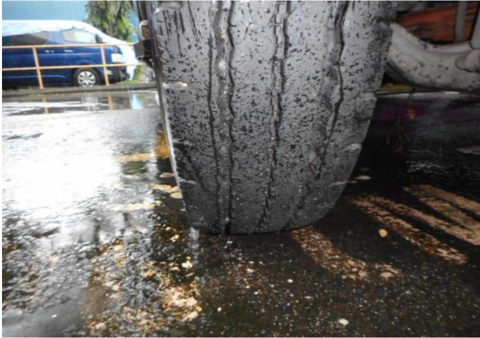
Photo 8 shows the condition of the front right tyre of the Motor Lorry, which was observed to be in serviceable condition with remaining tread depth of approximately 10.6mm. The tyre, which was wrapped around standard steel wheel rim, was also observed to be sufficiently inflated for vehicular operation. There was no tear, cut or burst mark(s) on the outer and the inner sidewalls as well as across the tread of the 6 tyres that were fitted on the Motor Lorry.
