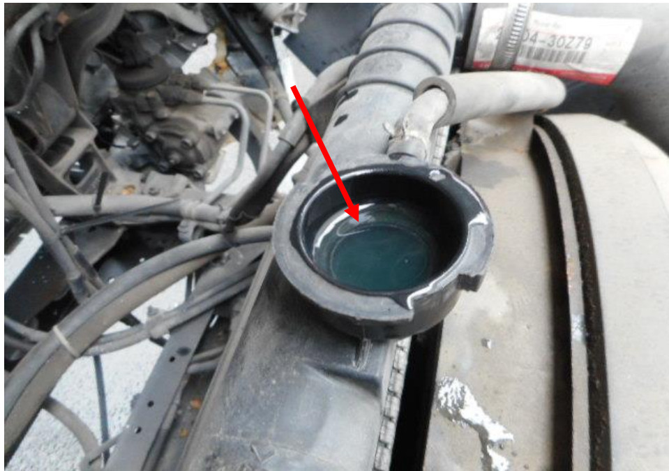
Photo 14 shows the engine coolant reservoir of the Motor Lorry at the time of my inspection. The engine coolant was observed to be of sufficient level (arrowed) and without any visible contamination.
