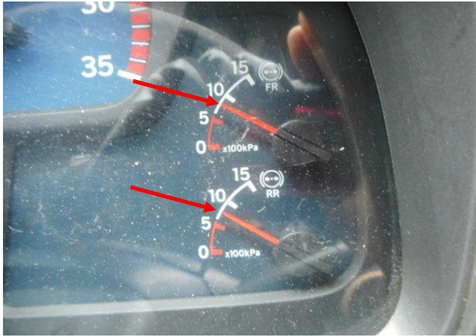
Photo 13 shows the air in the air brake cylinders of the Motor Lorry at the time of my inspection. The air in the cylinder was observed to be of sufficient level & serviceable at the time of the accident.
