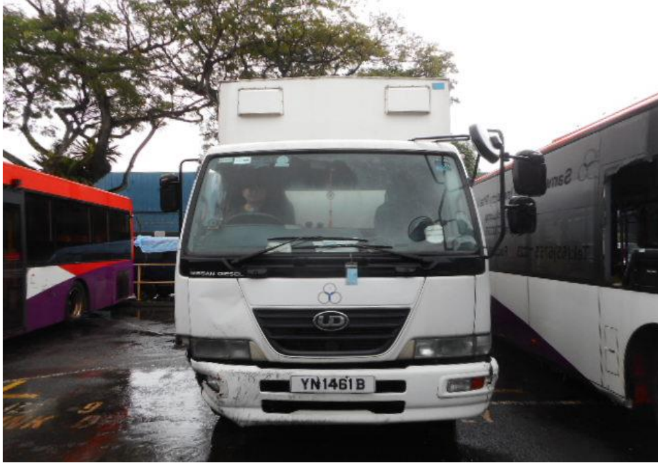
Photo 2 shows a general view of the front body of the Motor Lorry at the time of my inspection. It appeared to have sustained damage at its front portion. Its front bumper was damage at the time of my inspection as a result of the accident.
