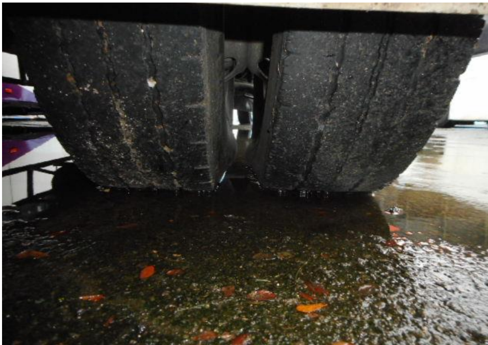
Photo 9 shows the condition of the rear right tyres of the Motor Lorry, which was observed to be in serviceable condition with remaining tread depth of approximately 3.3mm. The tyre, which was wrapped around standard steel wheel rim, it was observed to be sufficiently inflated for vehicular operation.
