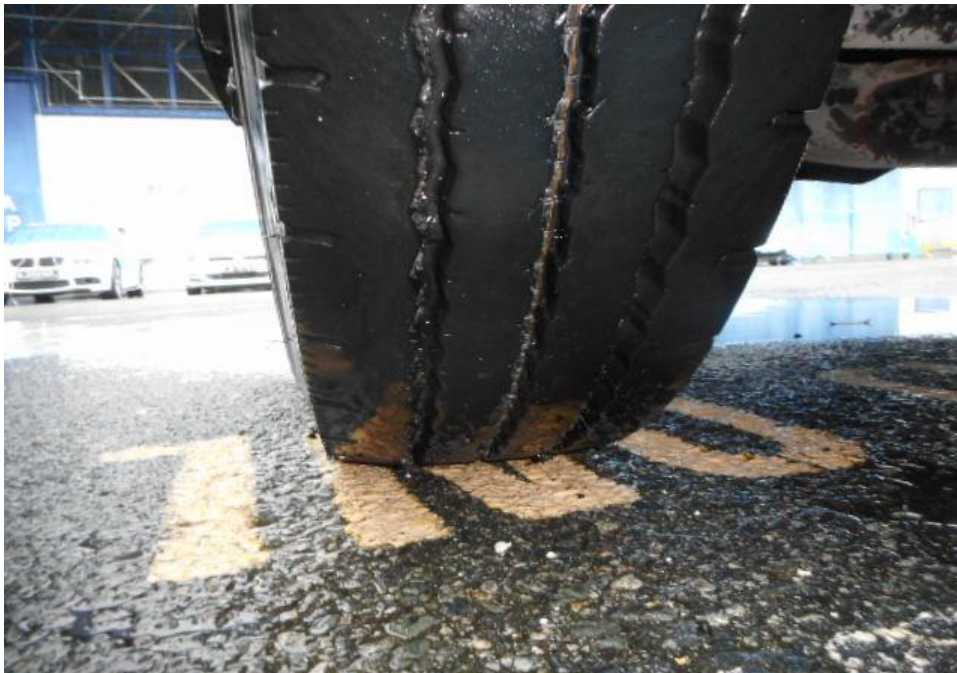
Photo 11 shows the condition of the front left tyre of the Motor Lorry, which were observed to be in serviceable condition with remaining, tread depth of approximately 10.9mm. There was also no tear, cut or burst mark(s) on the outer and the inner sidewalls as well as across the tread of the 6 tyres that were fitted on the Motor Lorry.
