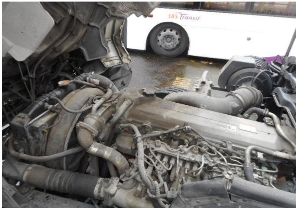
Photo 12 shows a general view of the Motor Lorry's engine compartment, which was accessed by lifting the front cabin of the Motor Lorry. The various parts and components inside the engine compartment were unaffected by the accident. There was also no sign(s) or indication(s) of fresh fluid leakage and/or fluid stain within the engine compartment.
