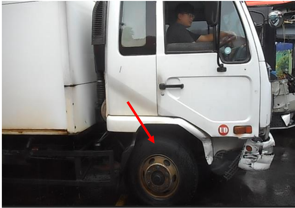
Photo 26 shows the front right wheel of the Motor Lorry turning to its left (arrowed) however, during my steering system test, I experience resistance when I turned the steering wheel towards the left and the steering would be jammed in the midst of turning towards the left.
