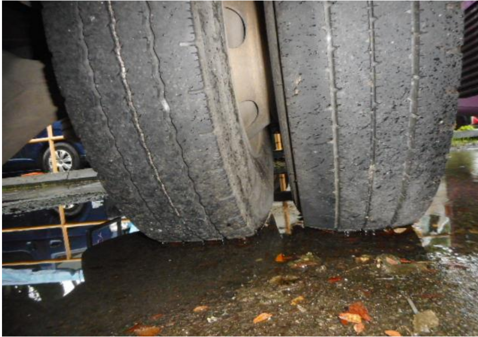
Photo 10 shows the condition of the rear left tyres of the Motor Lorry, which was observed to be in serviceable condition with remaining tread depth of approximately 5.7mm. The tyres, which were wrapped around standard steel wheel rim, were also observed to be sufficiently inflated for vehicular operation.
