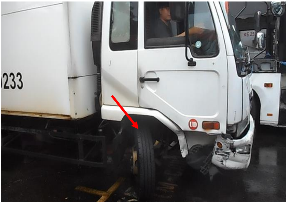
Photo 25 shows the front right wheel of the Motor Lorry turned to its full right (arrowed). During my steering system test, I did not experience any abnormal free play and/or resistance when I had turned the steering wheel towards full right.
