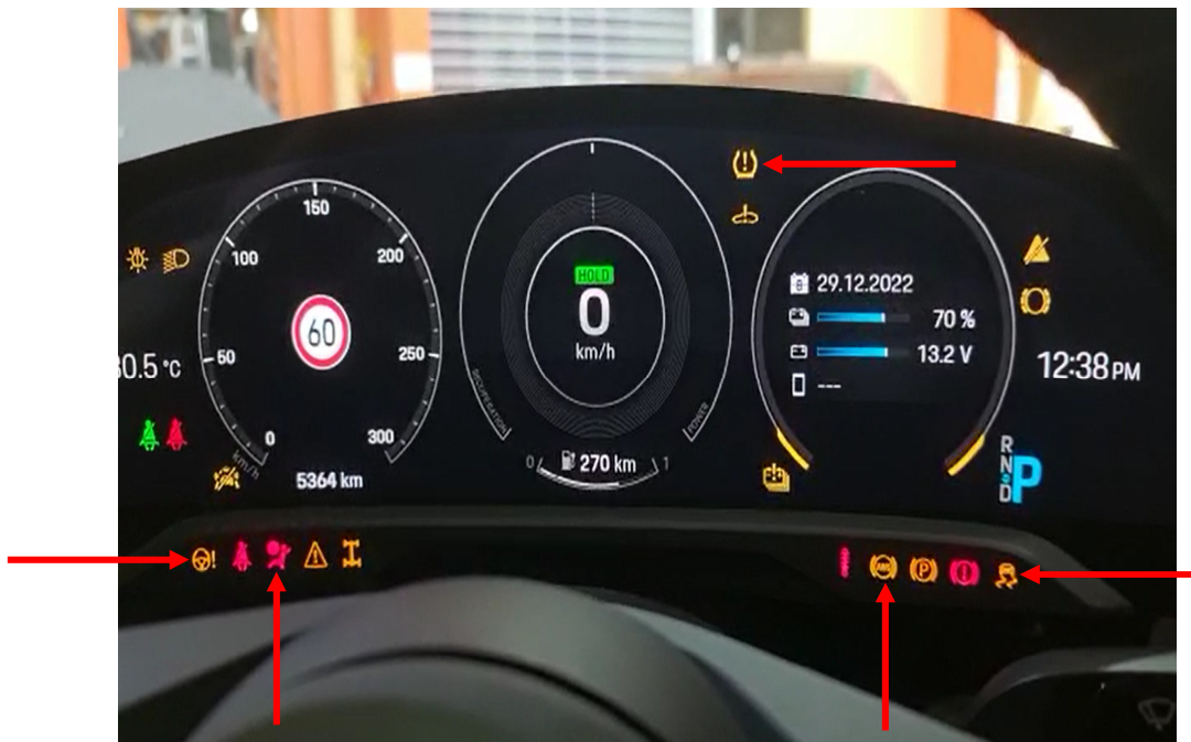
Photo 22 shows the warning lights for the various electronic safety features appearing on the instrument panel of the Motor Car during its self-test when the engine is cranked, in particular the ABS, SRS, EPS, TPM and SCS lights (arrowed).
