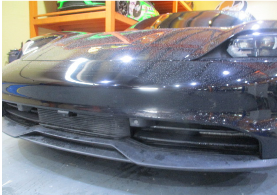
Photo 11 shows a closer view of the Motor Car's front bumper, front bumper lower lip, front bumper sensors, front bumper centre frame and front bonnet. The body parts at the frontal portion of the Motor Car were visually examined and it was observed that the repair/restoration works carried out to the damaged area of the Motor Car (refer to photograph 1 - 3 above) were reasonably adequate and in order.
