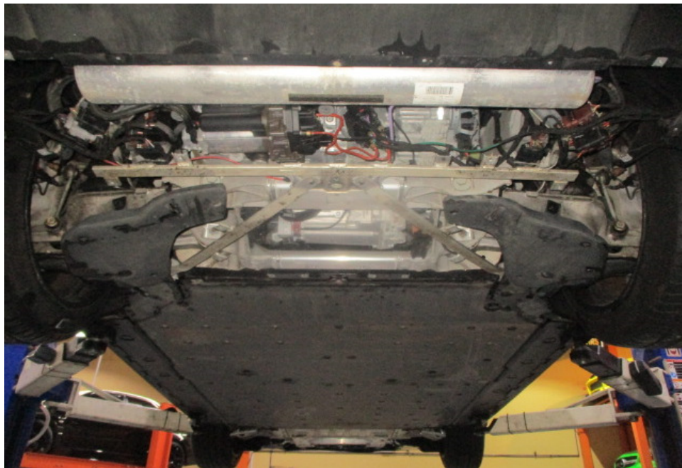
Photo 30 shows the underside centre of the Motor Car, at the location where the high voltage battery is fitted. The high voltage system of the Motor Car was visually checked, and it was observed that the various high voltage parts and components like the high voltage battery, inverter unit, converter unit, high voltage cables, electric motors and electric aircon compressor amongst others, were properly secured and without any physical damage.
