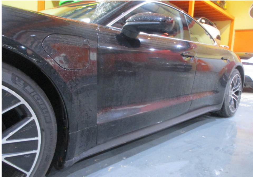
Photo 13 shows a closer view of the Motor Car's left side high voltage charging port cover, front left door, left side wing mirror and left side rocker panel garnish. The body parts at the frontal portion of the Motor Car were visually examined and it was observed that the repair/restoration works carried out to the damaged area of the Motor Car (refer to photograph 1 - 3 above) were reasonably adequate and in order.
