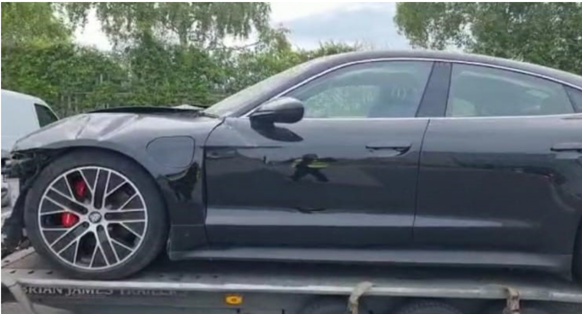
Photo 3 shows the left side body of the Motor Car (photograph provided to me). The Motor Car was observed to have sustained damage at its frontal portion. The front left fender and front left door were amongst the body parts that were observed to have been damaged.
