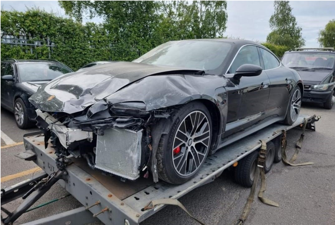
Photo 2 shows the front left body of the Motor Car (photograph provided to me). The Motor Car was observed to have sustained damage at its frontal portion. The front bumper, front bumper lower lip, front bumper left air guide, front bumper left lower grille, front bumper sensors, front bonnet, front bonnet left hinge, front left headlamp, front left signal lamp, front left fender, front left fender inner shield, front left radiator and front left door were amongst the body parts that were observed to have been damaged.
