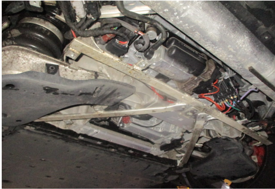
Photo 29 shows the underside rear of the Motor Car, at the location where the rear electric motor is fitted. The high voltage system of the Motor Car was visually checked, and it was observed that the various high voltage parts and components like the high voltage battery, inverter unit, converter unit, high voltage cables, electric motors and electric aircon compressor amongst others, were properly secured and without any physical damage.
