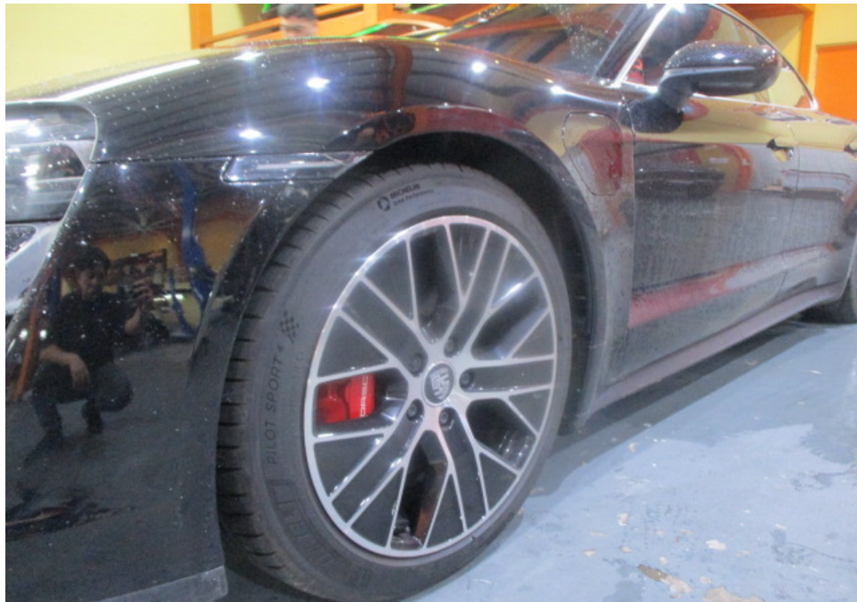
Photo 12 shows a closer view of the Motor Car's front left signal lamp, front left fender and front left wheel rim. The body parts at the frontal portion of the Motor Car were visually examined and it was observed that the repair/restoration works carried out to the damaged area of the Motor Car (refer to photograph 1 - 3 above) were reasonably adequate and in order.
