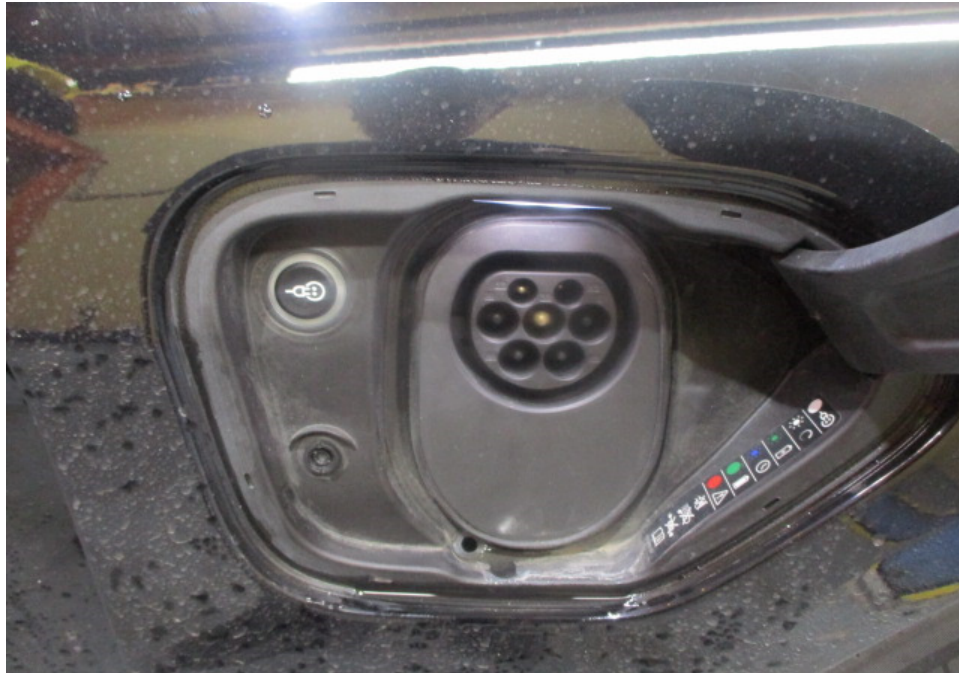
Photo 19 shows the high voltage charging port located at the front right fender of the Motor Car at the time of my inspection. A JS 1772 (Type 2) for alternating current (AC) charging was fitted on the front right fender of the Motor Car. No physical damage was observed to the charging head.
