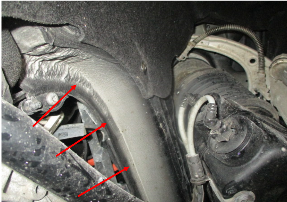
Photo 35 shows the chassis/structural body at the underside front right of the Motor Car. The original factory sealant (arrowed) at the joints along the chassis/structural body was observed to be untouched. In general, I had found no work was carried out on the chassis/structural body of the Motor Car. The chassis/structural body of the Motor Car was originally fitted.
