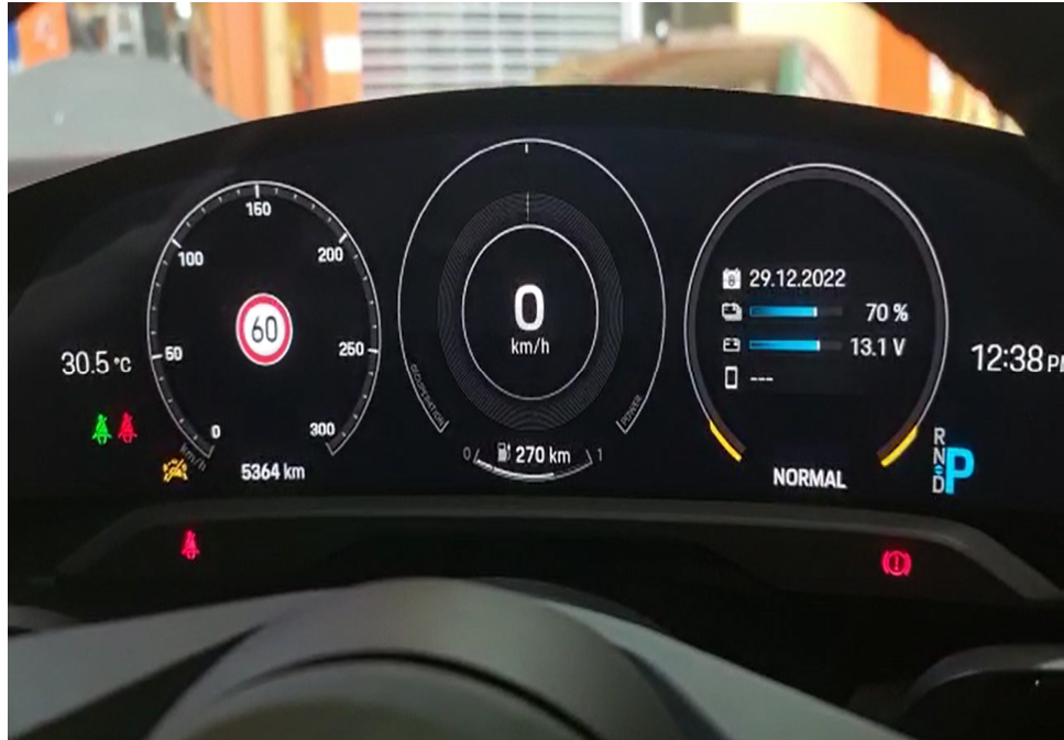
Photo 23 shows the respective warning lights no longer illuminated, indicating that there is no fault detected to the ABS, SRS, EPS, TPM and SCS systems of the Motor Car during the self-test. These electronic systems were hence in working condition at the time of my inspection.
