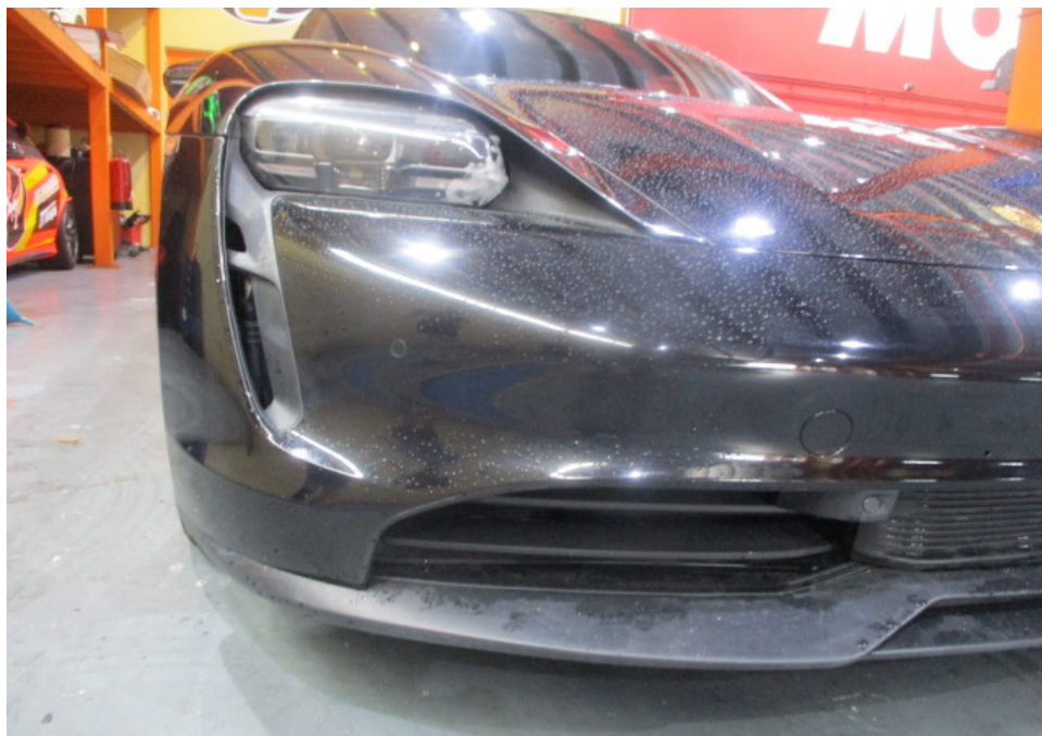
Photo 8 shows a closer view of the Motor Car's front bumper, front bumper lower lip, front bumper right air guide, front bumper right lower grille and front right headlamp. The body parts at the frontal portion of the Motor Car were visually examined and it was observed that the repair/restoration works carried out to the damaged area of the Motor Car (refer to photograph 1 - 3 above) were reasonably adequate and in order.
