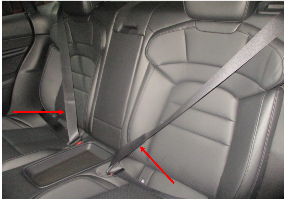
Photo 21 shows the rear seats of the Motor Car. All the seats of the Motor Car were secured via seat rails to the floorboard. They were also fitted with a retractable seat belt reel and a pre-tensioner. The seat belts (arrowed) were tested and were able to be fastened into the respective pre-tensions that were fitted on the side of each individual seat.
