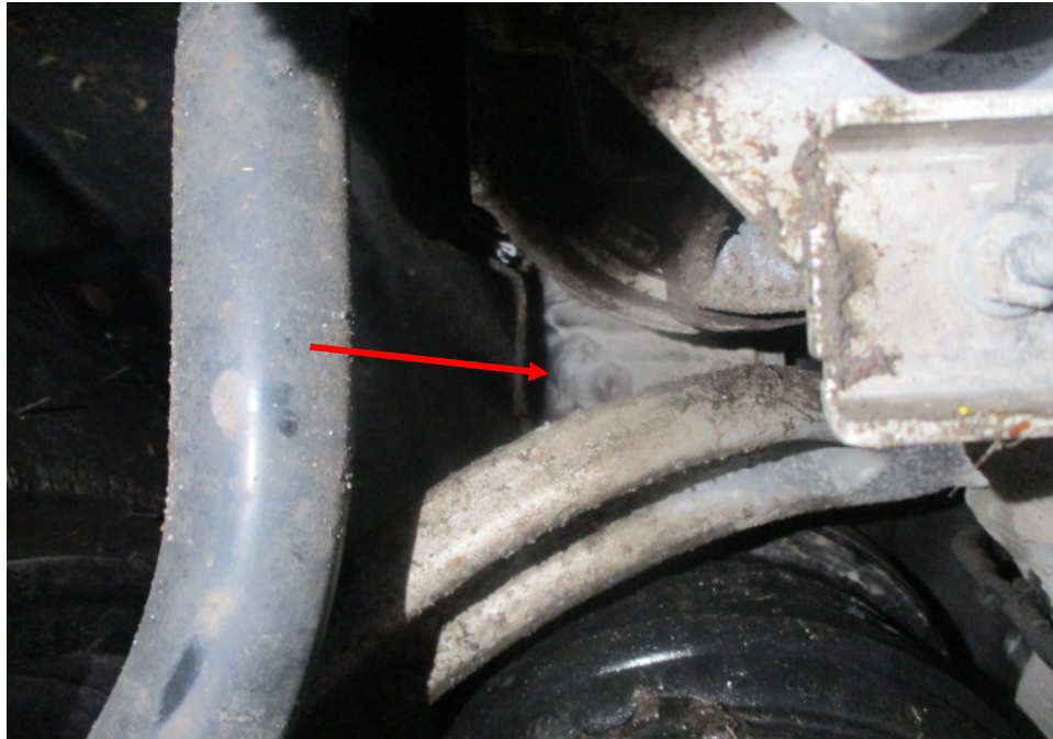
Photo 33 shows the chassis/structural body at the underside rear left of the Motor Car. The original factory sealant (arrowed) at the joints along the chassis/structural body was observed to be untouched. In general, I had found no work was carried out on the chassis/structural body of the Motor Car. The chassis/structural body of the Motor Car was originally fitted.
