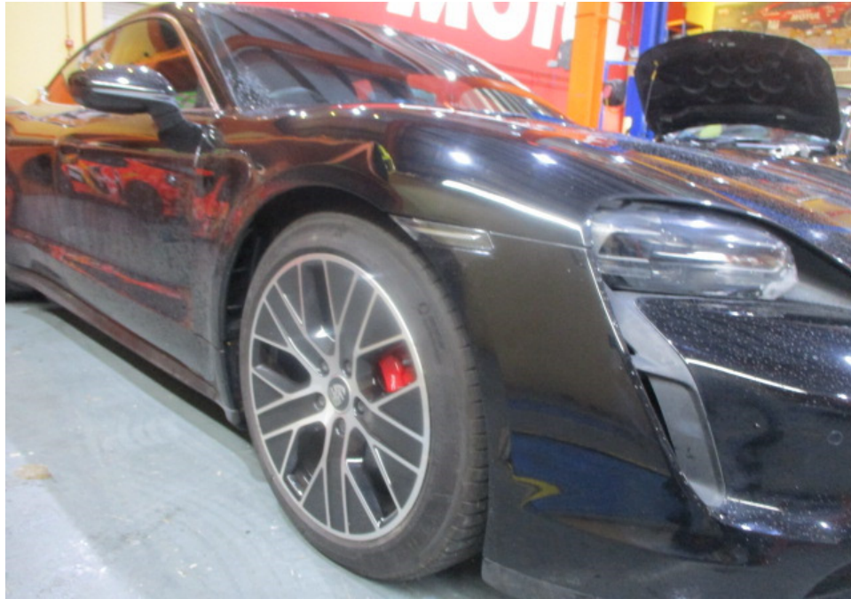
Photo 7 shows a closer view of the Motor Car's front right headlamp, front right signal lamp, front right fender and front right wheel rim. The body parts at the frontal portion of the Motor Car were visually examined and it was observed that the repair/restoration works carried out to the damaged area of the Motor Car (refer to photograph 1 - 3 above) were reasonably adequate and in order.
