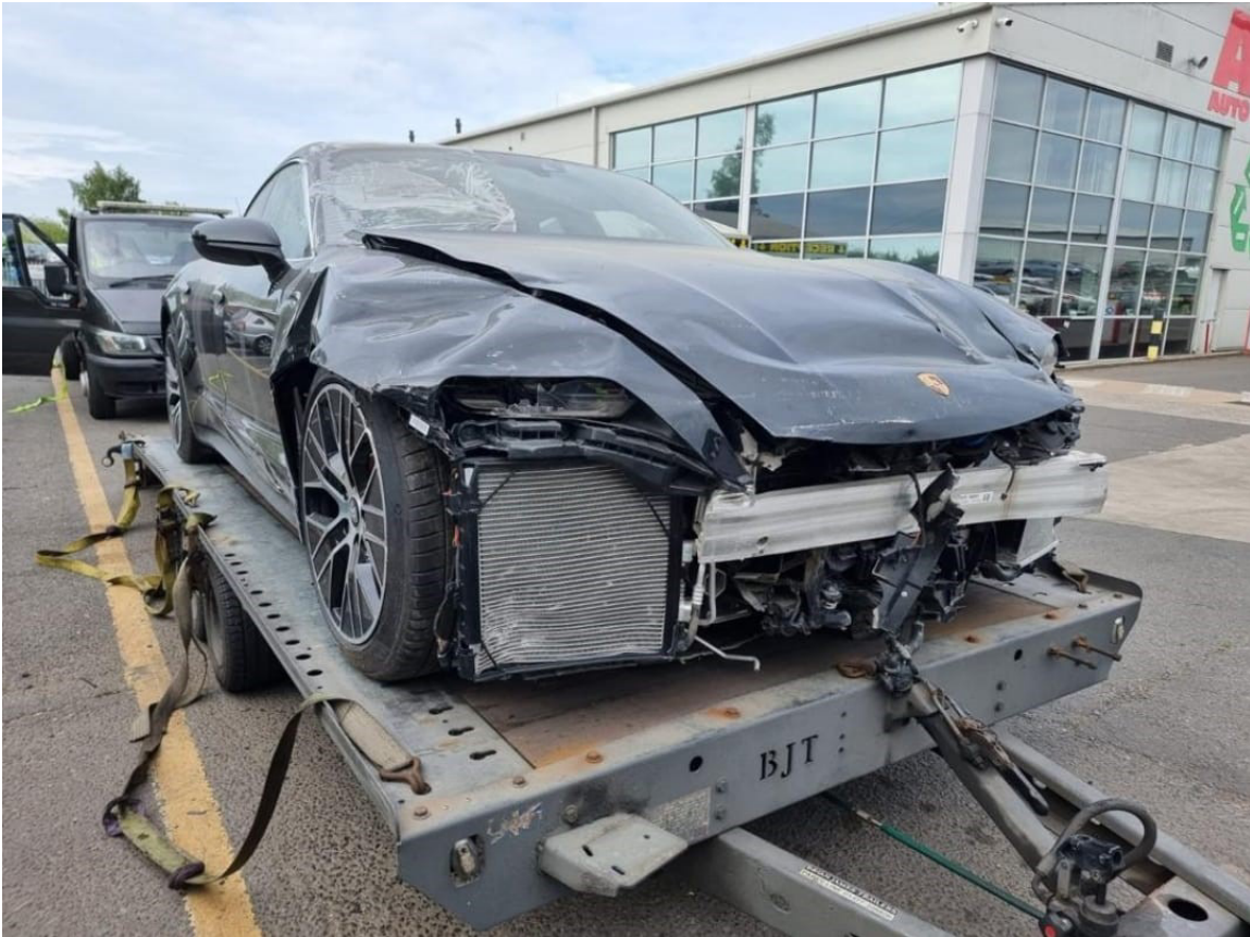
Photo 1 shows the front right body of the Motor Car (photograph provided to me). The Motor Car was observed to have sustained damage at its frontal portion. The front bumper, front bumper reinforcement, front bumper centre frame, front bumper lower lip, front bumper right air guide, front bumper right lower grille, front bumper sensors, front bonnet, front bonnet right hinge, front right headlamp, front right signal lamp, front right fender, front right fender inner shield, front right aircon condenser and front windscreen were amongst the body parts that were observed to have been damaged.
