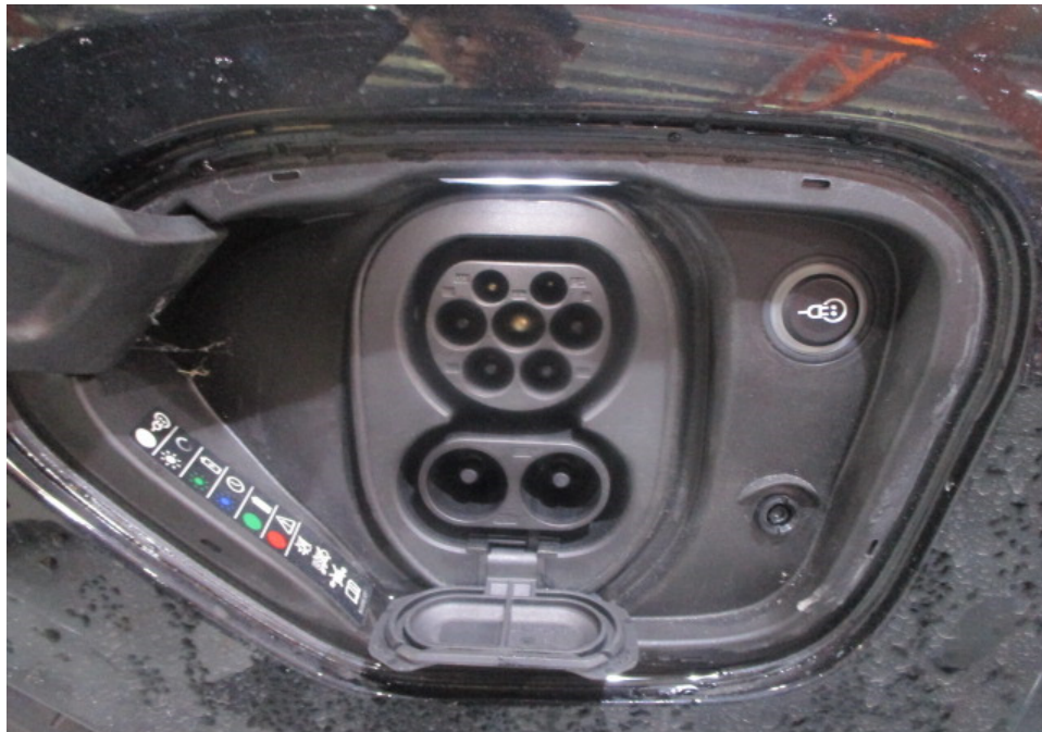
Photo 18 shows the high voltage charging port located at the front left fender of the Motor Car at the time of my inspection. A Combined Charging Standard 2 (CCS 2) for direct current (DC) charging was fitted on the front left fender of the Motor Car. No physical damage was observed to the charging head.
