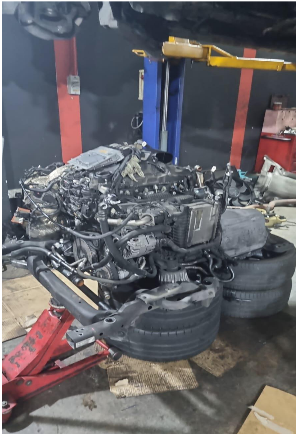
Photo 6 shows the general view of the engine unit of the Insured Vehicle at the start of the dismantling. The exterior of the engine unit is observed to be unaffected and by any signs of accident.
