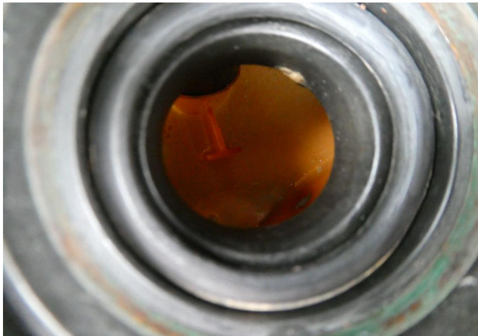
Photo 5 shows the close up view of inside the coolant reservoir of the Insured Vehicle at the time of our inspection. The coolant reservoir is observed to be unaffected and by any signs of accident, however the coolant was observed to be insufficient.
