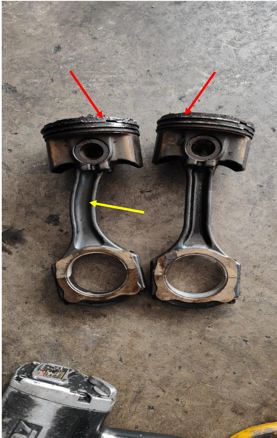
Photo 8 shows the general view of the piston and connecting rod of the Insured Vehicle at the time of our inspection. We observed that the piston (red arrow) and connecting rod (yellow arrow) was damaged as a result of the engine coolant which had resulted in the damage to the engine.
