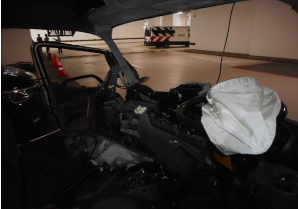
Photo 17 shows the deployment of the Supplemental Restraint System (SRS) airbag in the Motor Lorry as a result of the accident.
