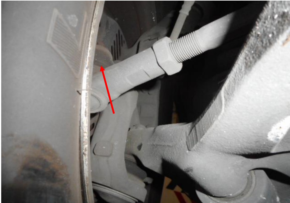
Photo 21 shows the various undercarriage components at the front right wheel of the Motor Lorry, in particular the steering tie rod end (arrowed). The various steering components were all found to be intact.
