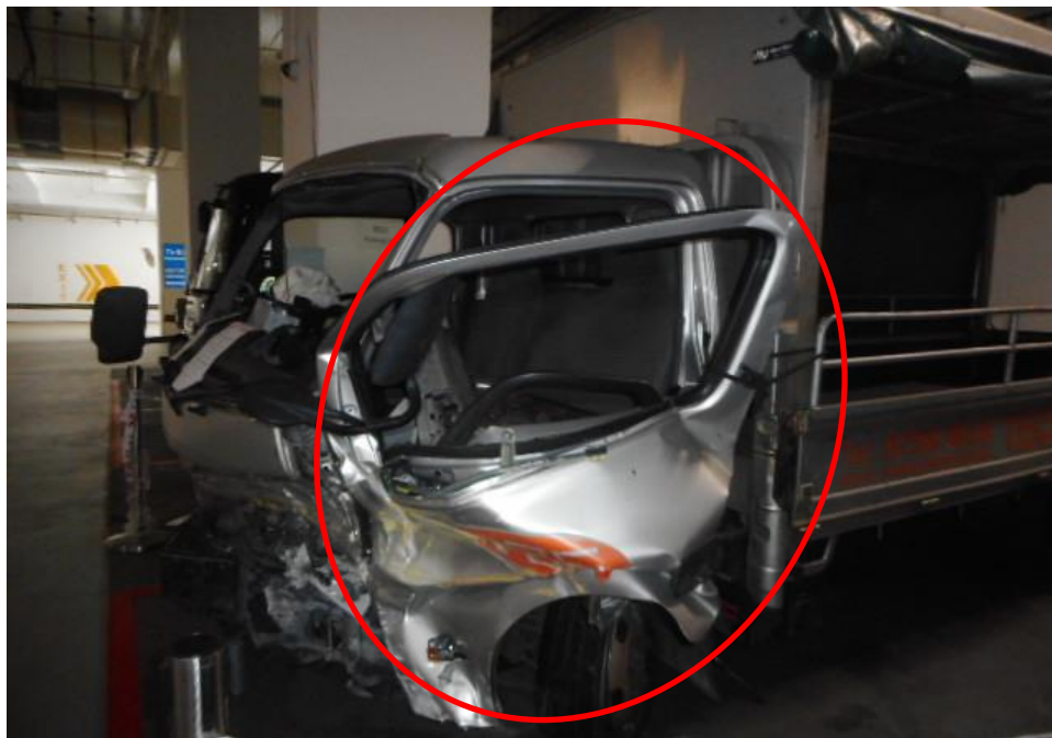
Photo 8 shows the close up view of the left door of the Motor Lorry at the time of our inspection. The Motor Lorry was observed to have sustained damages to its left door (circled) as a result of the accident.
