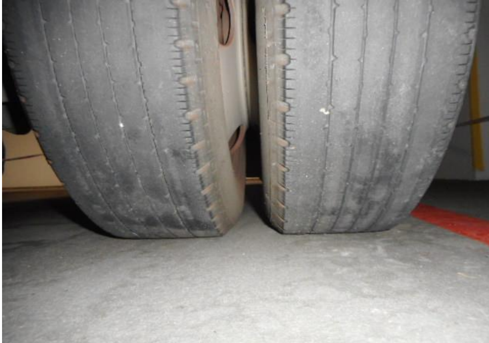
Photo 15 shows the condition of the rear right tyres of the Motor Lorry, which were observed to be in serviceable condition with remaining, tread depth of approximately 2.1mm. The tyres, which was wrapped around standard steel wheel rim, it was observed to be sufficiently inflated for vehicular operation.
