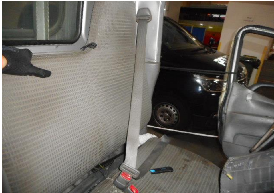
Photo 30 shows that the seat belt on the left seat was able to be fastened securely into the respective pre-tensioners that were fitted at the sides of each seat.
