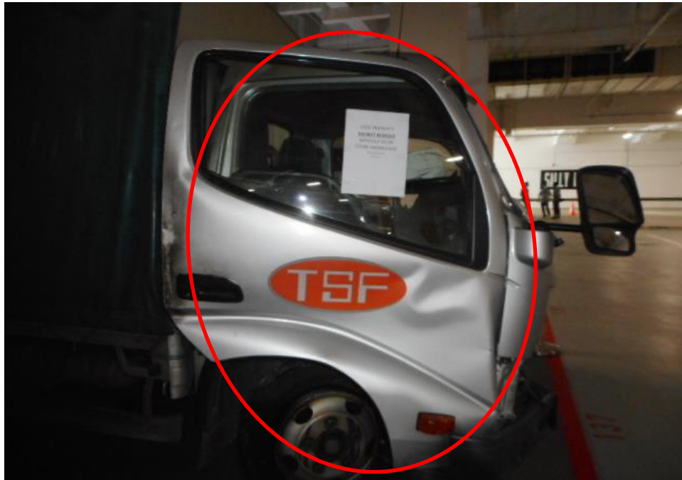
Photo 7 shows the close up view of the right door of the Motor Lorry at the time of our inspection. The Motor Lorry was observed to have sustained damages to its right door (circled) as a result of the accident.
