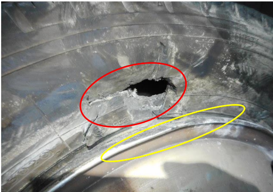
Photo 14 shows the condition of the outer side of the front left tyre of the Motor Lorry, which was observed to be in unserviceable condition with remaining tread depth of approximately 6.5mm. The steel wheel rim, was observed damage (yellow circle) and the tyre was observed to be cut and deflated (red circle) as a result of the accident.
