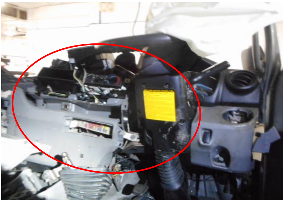
Photo 4 shows the close up view of the front portion of the Motor Lorry at the time of our inspection. The Motor Lorry was observed to have sustained major damages to its dashboard (circled) that was crushed due to the accident's impact.
