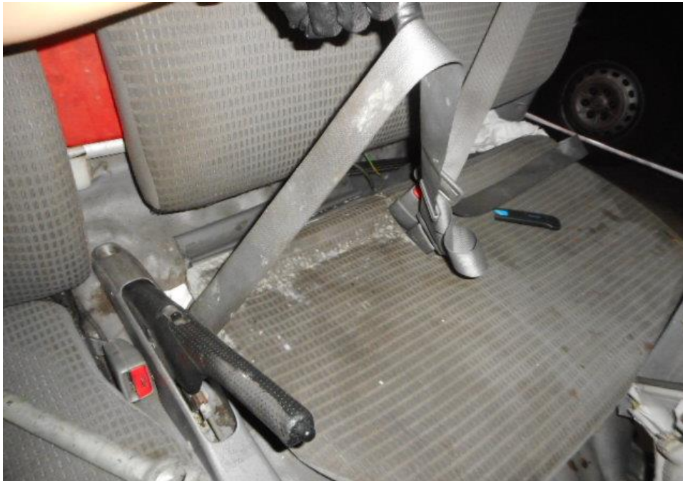
Photo 29 shows that the seat belt on the centre seat was able to be fastened securely into the respective pre-tensioners that were fitted at the sides of each seat
