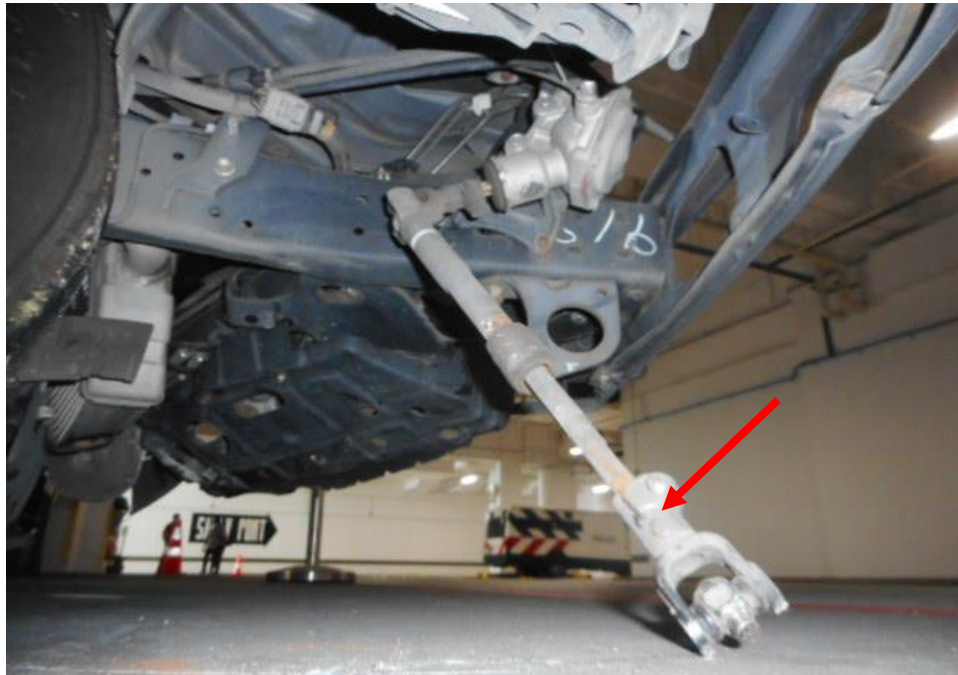
Photo 27 shows the various undercarriage components of the Motor Lorry, in particular the steering shaft (arrowed) was observed to be broken off as a result of the accident.
