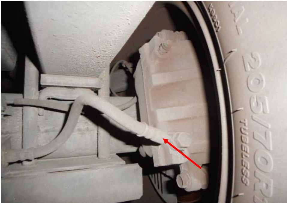
Photo 23 shows the brake pipe (arrowed) at the rear right wheel of the Motor Lorry. I did not observe any leakage of brake fluid at the time of my inspection of the Motor Lorry. My visual examination of the various mechanical components in the braking system were all found to be intact without any visible damage.
