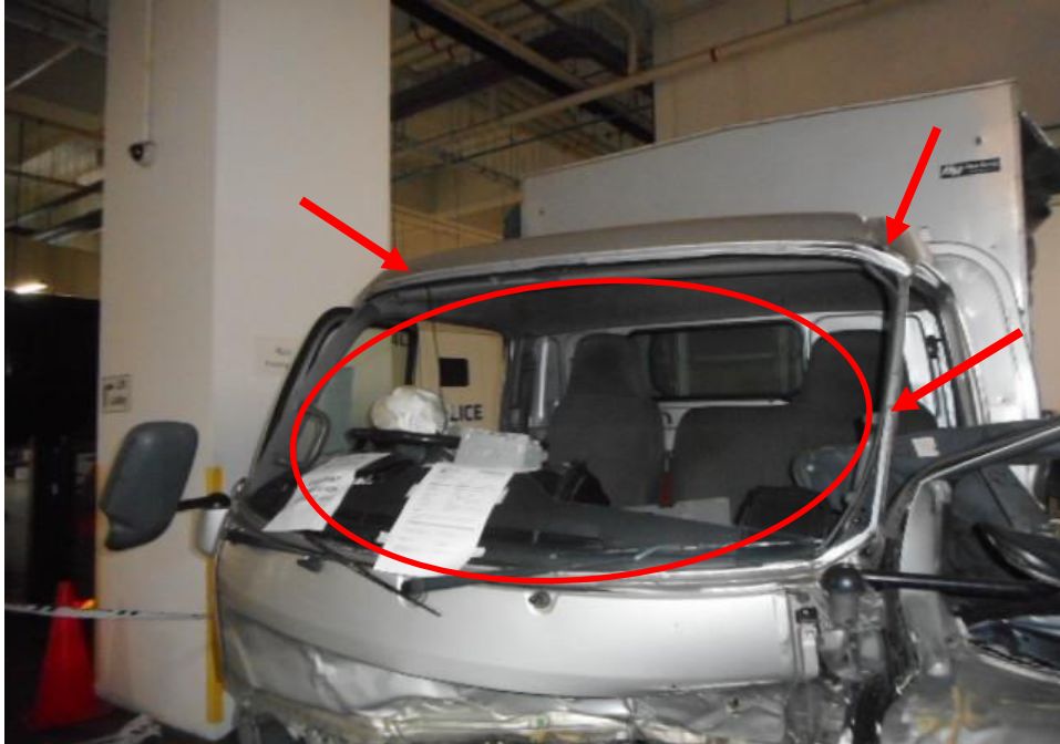
Photo 5 shows the close up view of the front portion of the Motor Lorry at the time of our inspection. The Motor Lorry was observed to have sustained major damages to its front windscreen (red circle) and its front cabin (arrowed) that was crushed due to the accident's impact.
