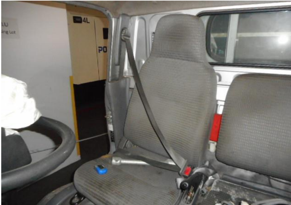
Photo 28 shows that the seat belt on the right seat was able to be fastened securely into the respective pre-tensioners that were fitted at the sides of each seat
