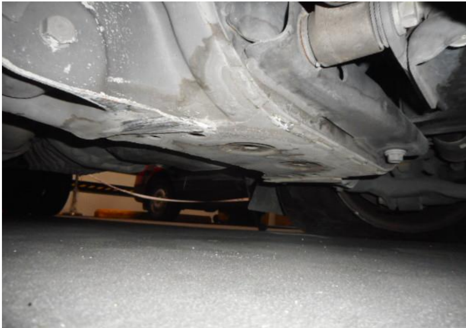
Photo 20 shows the undercarriage of the Motor Lorry, at the area where the engine housing and transmission housing are located. I did not find any sign(s) or indication(s) of fluid leak and/or fluid stain(s) on the underside of the Motor Lorry.
