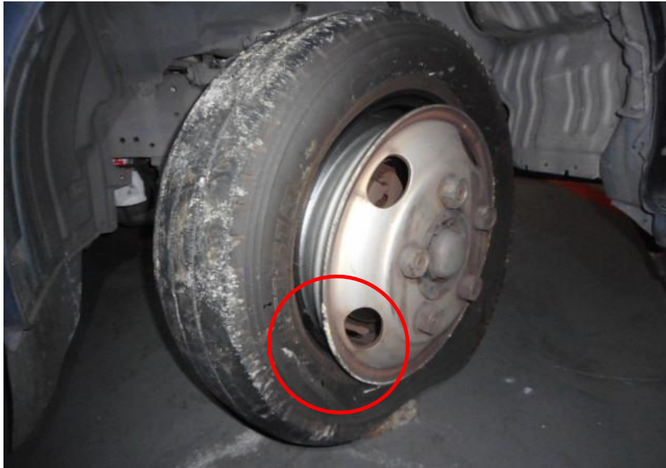
Photo 11 shows the condition of the outer side of the front right tyre of the Motor Lorry, which was observed to be in unserviceable condition with remaining tread depth of approximately 6.5mm. The steel wheel rim, was observed damage (circled) and the tyre was observed to be cut and deflated as a result of the accident.
