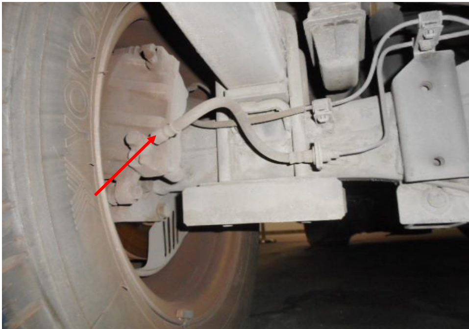
Photo 24 shows the brake pipe (arrowed) at the rear left wheel of the Motor Lorry. I did not observe any leakage of brake fluid at the time of my inspection of the Motor Lorry. My visual examination of the various mechanical components in the braking system were all found to be intact without any visible damage.
