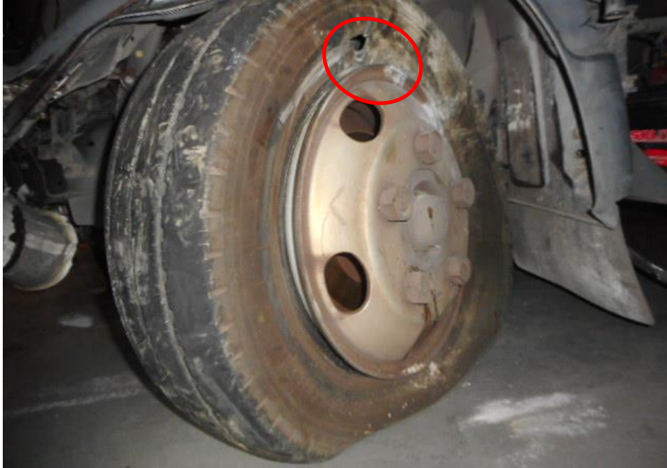
Photo 13 shows the condition of the outer side of the front left tyre of the Motor Lorry, which was observed to be in unserviceable condition with remaining tread depth of approximately 6.5mm. The steel wheel rim, was observed damage (circled) and the tyre was observed to be cut and deflated as a result of the accident.
