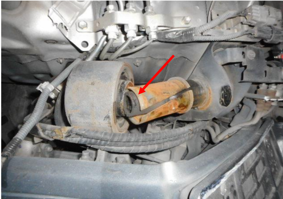
Photo 18 shows the induced damage to the front cabin opening mechanism (arrowed) of the Motor Lorry's which had immobilised the opening and viewing of the various parts and components inside the engine compartment a result of the accident.
