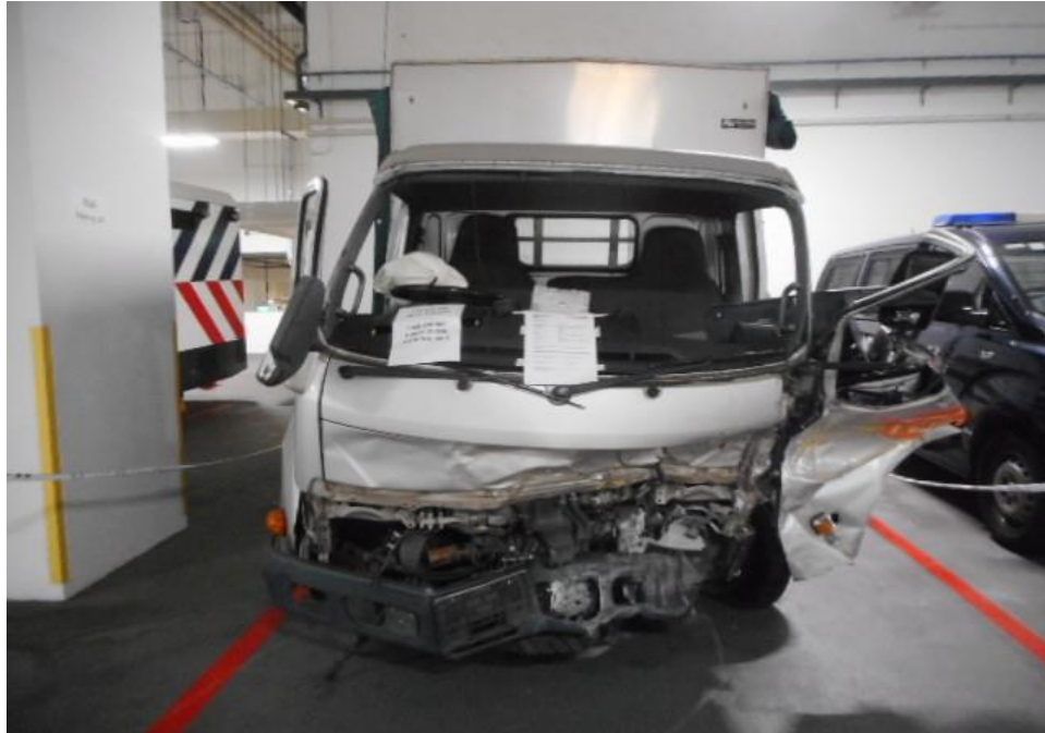
Photo 3 shows a general view of the front portion of the Motor Lorry at the time of our inspection. The Motor Lorry was observed sustained major damages to its front and rear portion. Its front cabin, front windscreen, front bumper and front body panel and its both doors as a result of the accident. The Supplemental Restraint System (SRS) was activated as a result of the accident.
