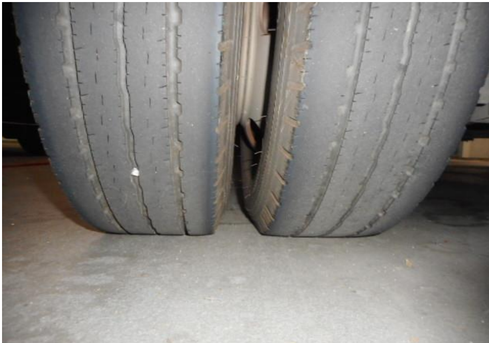
Photo 16 shows the condition of the rear left tyres of the Motor Lorry, which were observed to be in serviceable condition with remaining, tread depth of approximately 5.7mm. The tyres, which was wrapped around standard steel wheel rim, it was observed to be sufficiently inflated for vehicular operation.
