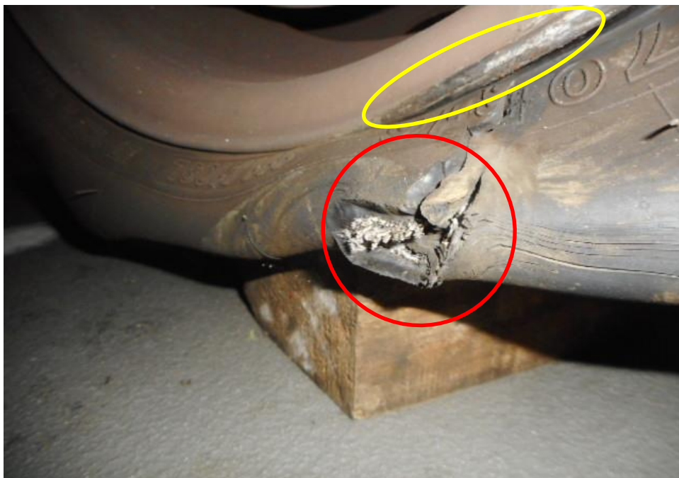
Photo 12 shows the condition of the inner side of the front right tyre of the Motor Lorry, which was observed to be in unserviceable condition with remaining tread depth of approximately 6.5mm. The steel wheel rim, was observed damage (yellow circle) and the tyre was observed to be cut and deflated (red circle) as a result of the accident.
