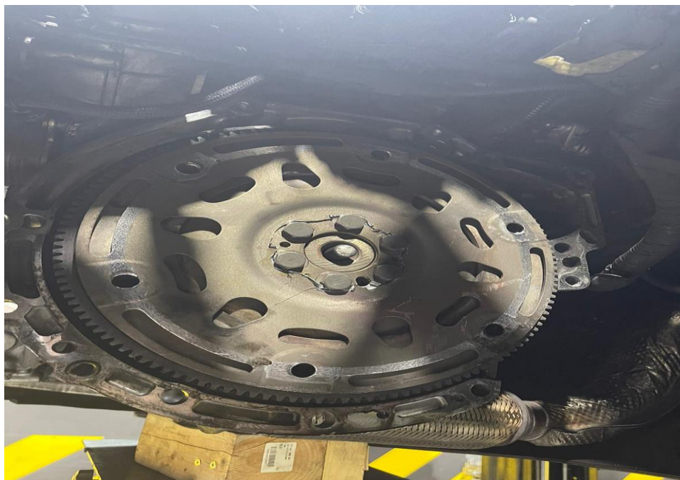
Photo 5 shows the general view of the engine flywheel of the Insured Vehicle at the time of our inspection. The engine flywheel was observed to have free play and also sustained damages on it.
