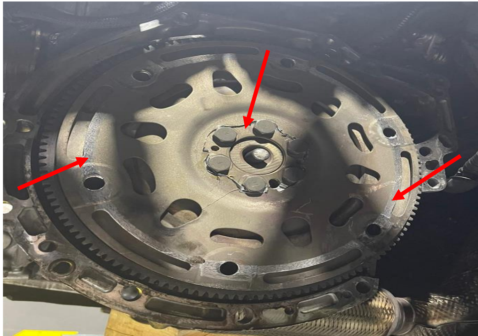
Photo 6 shows the close up view of the engine flywheel of the Insured Vehicle at the time of our inspection. The engine flywheel (arrowed) was observed to have free play and also sustained damages on it.
