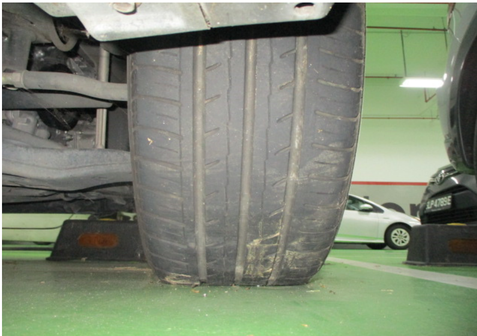
Photo 8 shows the width of the front right tyre that was fitted on the Insured Vehicle at the material time of accident. The width of the other 3 tyres that were fitted on the Insured Vehicle was wider as compared to the narrower width of the spare tyre that was fitted on the front left wheel of the Insured Vehicle (refer to photograph 7 above).
