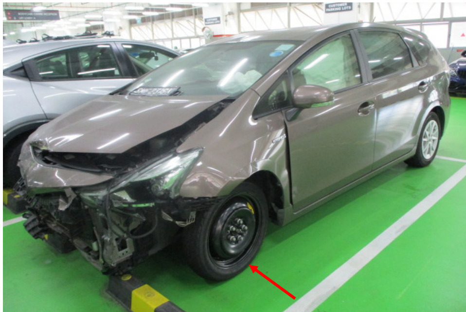
Photo 1 shows a general view of the front left body of the Insured Vehicle at the time of my inspection on 27 June 2022. The Insured Vehicle was observed to have sustained impact damages at its frontal portion. The driver's airbag, driver's seat airbag, driver's knee airbag and front left passenger airbag were deployed. The front left tyre fitted on the Insured Vehicle was a spare tyre (arrowed).
