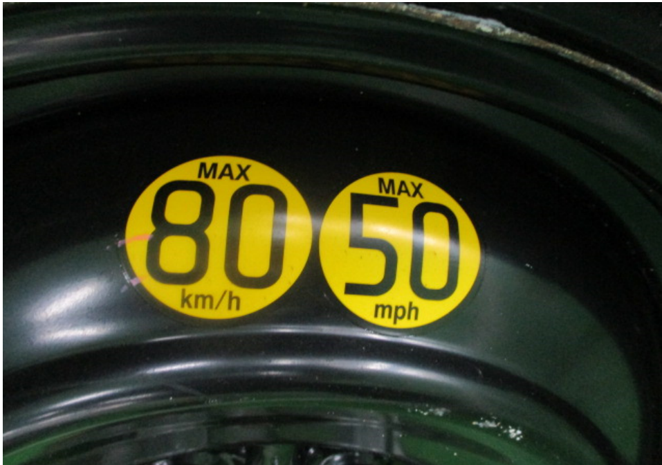
Photo 6 shows a closer view of the 2 bright coloured yellow stickers that were pasted on the wheel rim of the spare tyre. The stickers indicate that the maximum safe travelling speed of a vehicle that is fitted with this spare tyre is 80km per hour or 50 miles per hour.
