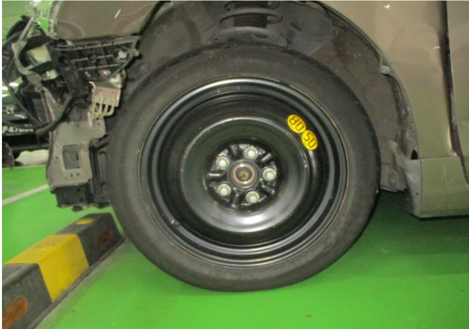
Photo 5 shows the spare tyre that was fitted at the front left wheel of the Insured Vehicle. The spare tyre was observed to be sufficiently inflated with relatively good remaining tread depth and tread pattern for vehicular operation. 2 bright coloured yellow stickers were pasted on the wheel rim of the spare tyre, which had indicated the maximum speed of 80km per hour and 50miles per hour.
