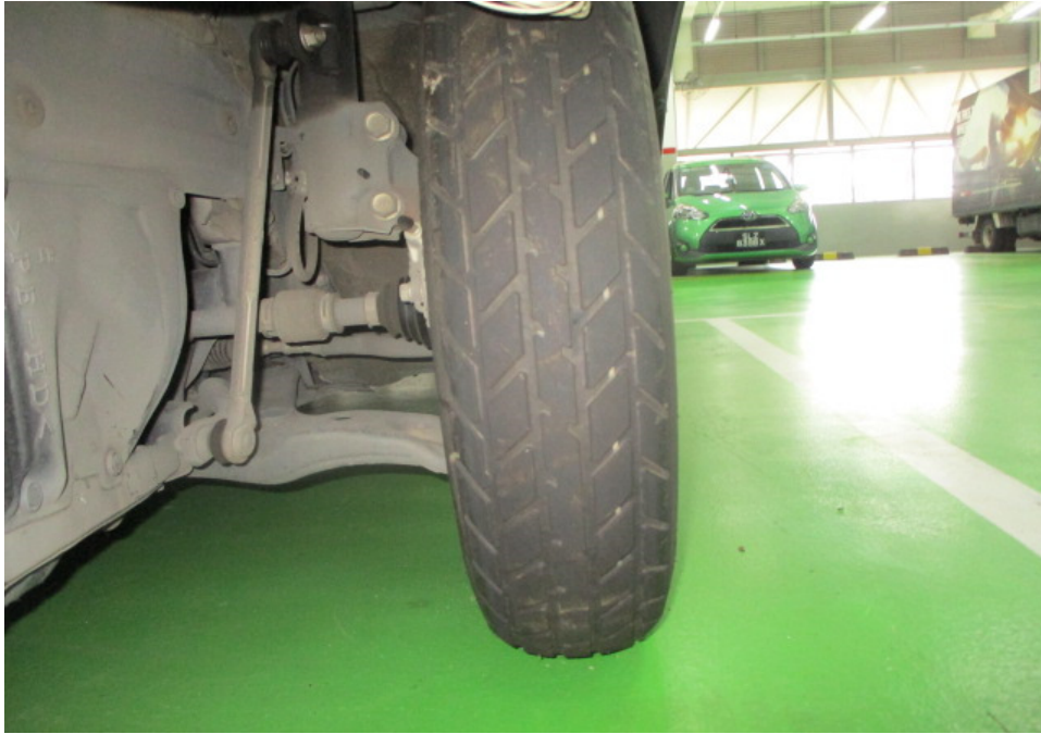
Photo 7 shows the narrower width of the spare tyre that was fitted on the Insured Vehicle as compared to the wider width of the other 3 tyres (refer to photograph 8 below) that were fitted on the Insured Vehicle at the material time of accident. A narrower width equates to lesser contact area between tyre and ground.
